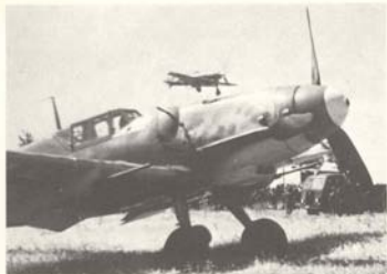
On a Sardinian airfield Axis air force personnel watch an Italian Macchi C.202 fighter come in to land. In the foreground is a Bf109G-6 of either II/JG 51 or III/JG 77, heavily armed with additional underwing 20mm cannon for anti-bomber work.
