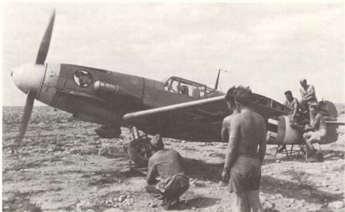
By late 1941, I/JG 27 had been re-equipped with Bf109Fs. An aircraft of this Gruppe undergoes undercarriage retraction tests with the engine running. Note the ground crew holding down the tail.
