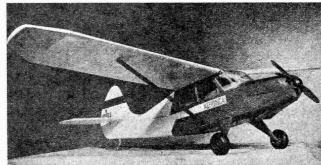
Fine example of British kits: Aeronca Sedan of 65.5" span. Designed to take 2.5 cc motors for free flight or radio control. This one has an Elfin 2.40 cc engine. Boasts scale flight characteristics.
