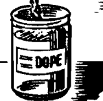
Silver powder, added to clear dope, gives "body" to fill pores of silk and nylon covering —
