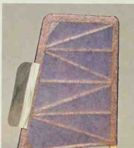
Top: Wiping an inlaid sheet balsa panel into place with a metal rule. Second: Use books or blocks to hold wingtips at correct height for dihedral; note centre panel pinned flat. Third: Easing tissue in place and pressing on wet clear dope or paste. Bottom left: Remove tissue surplus by sanding with fine paper when dry. Bottom right: Use balsa strip for turn adjustment, or fit tab – both shown.
