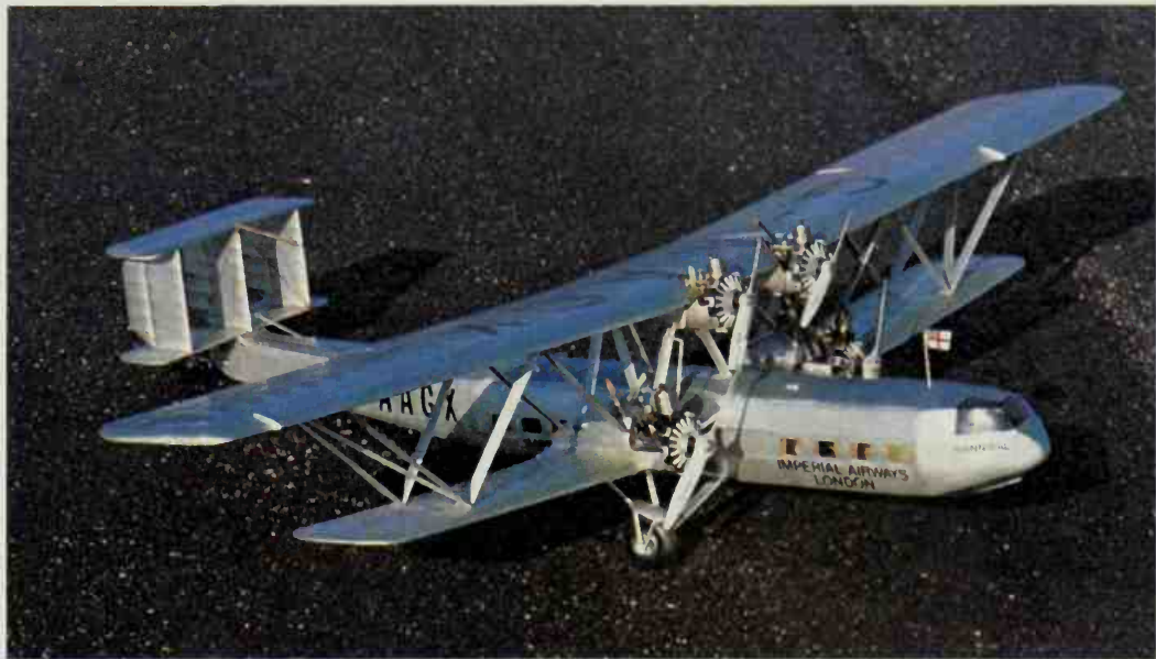
Right: A 66in Handley Page 42 Hannibal by J. Shelley. Two 1.3cc and two 0.75cc diesels, radio-controlled.
