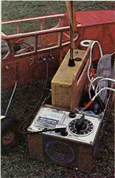
Above: A neat field-box carrying transmitter and test and charging equipment. Fast re-charge cells allow many flights during a session at the flying field.
