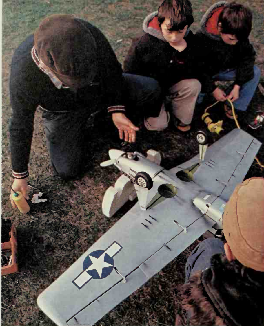
Left: World War 2 fighters are popular. This Mustang has retracting undercarriage, flaps, and an inverted engine. Flooding of the plug is avoided when starting by turning the model over. Diagram below shows basic layout of fuel system.
