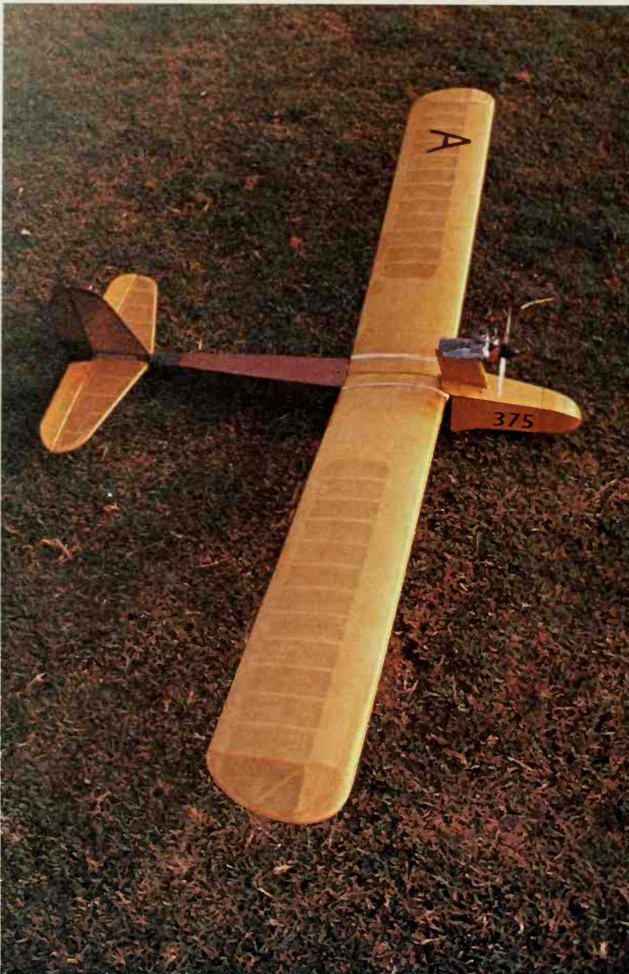
Above: A simple boxy model equipped with a power pod. The engine is a means of gaining height in place of a towline.
