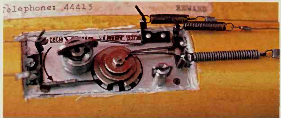
Top: Dethermaliser details, essential to all high performance free-flight models. Above: Operation of engine cut-out, variable incidence tail, rudder trim and D/T can all be carried out by one clockwork timer.
