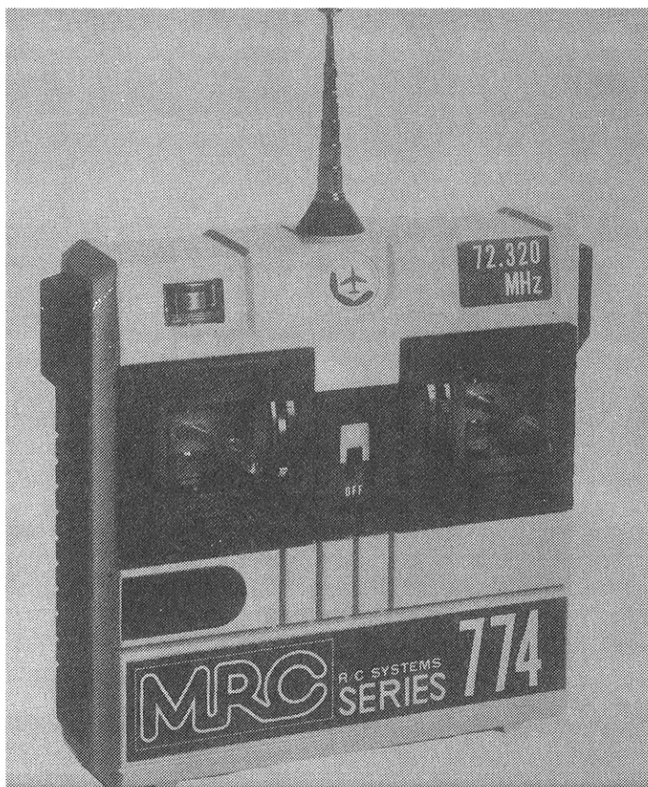
Fig. 3-15. A modern digital transmitter with sliding antenna.
