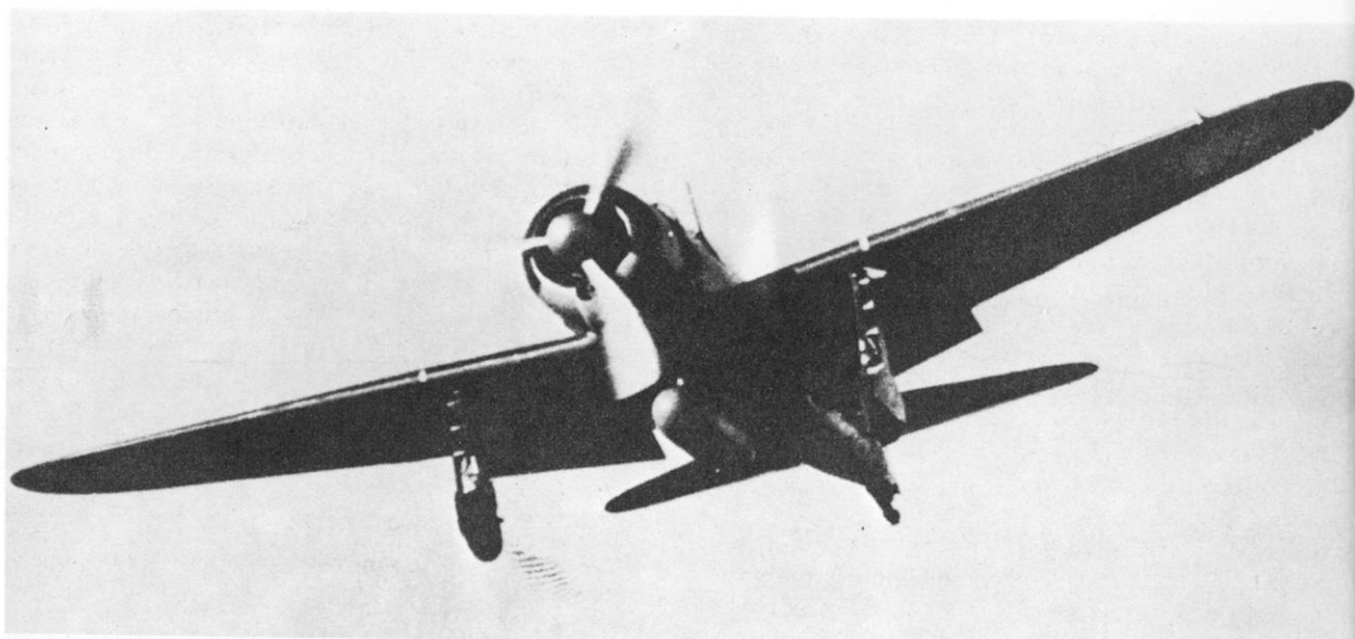
Mitsubishi A6M2 (Navy Type O Carrier Fighter Model 21) in landing configuration. Note flaps and ventral drop tank.
