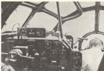
Men at work: a B-29 bombardier bends over his sight in front of the instrument panel and control wheel of the 'Airplane Commander'. Of interest is the bombardier's steel helmet, which appears to be of standard infantry pattern, hanging conveniently above his left shoulder.
