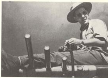
Sqn. Ldr. L. Hawkins of No. 135 Sqn. on the wing of his Thunderbolt Mk I, showing well how the four .50 cal. machine-guns were set horizontally rather than following the dihedral angle. (L. Hawkins)
