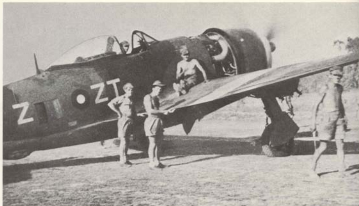
Playing a unique combat role in RAF hands in SEAC was the Republic Thunderbolt, over 800 of which were delivered in two main marks—I (P-47D razorback) and II (P-47D-25 and subsequent models with bubble hood). Pictured at Ratnap in late 1944 was HD244/HT-Z of No. 258 Sqn. in green/earth camouflage and SEAC identity bands common to the type.
