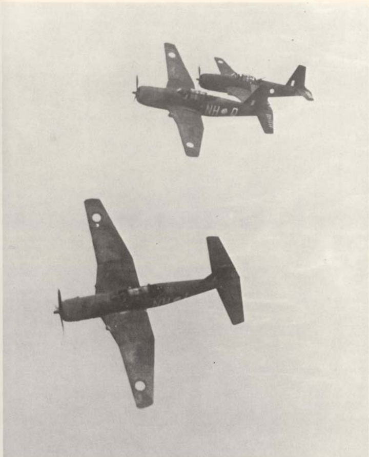
Peel off by Vengeances of No. 12 Sqn. RAAF, code 'NH'. The two aircraft in the background have white bars on the elevators, which may have been sighting aids for the rear gunner.
