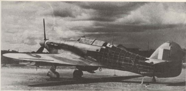
A No. 135 Sqn. Hurricane under repair at Yelahanka. The size of the wing roundel and proportions of the fin flash are of interest, as are the exposed structural details. (C. A. C. Stone)
