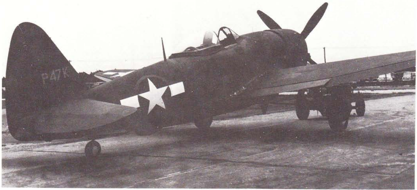
Fig. 12 The P-47K was radically modified from the last P-47D-5-RE, 42-8702, to have a bubble canopy, cut-down rear fuselage decking and repositioned radio equipment. It was completed 3 July 1943. Its star and bar markings had the current red surround. [Republic via R. A. Freeman]
