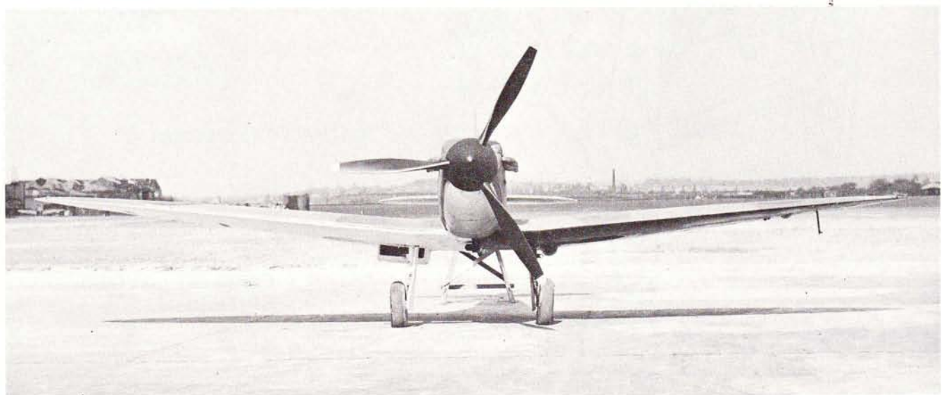
Fig. 12 Head-on view of a Spitfire I with a three-bladed DH two-speed propeller, showing to good effect the Spit's low frontal area, including the extremely thin wing. Narrow-track undercarriage was one of the Spit's least desirable features as it caused handling problems, especially during taxiing when the pilot's difficulties were further increased by the long nose which completely blocked the forward view.
