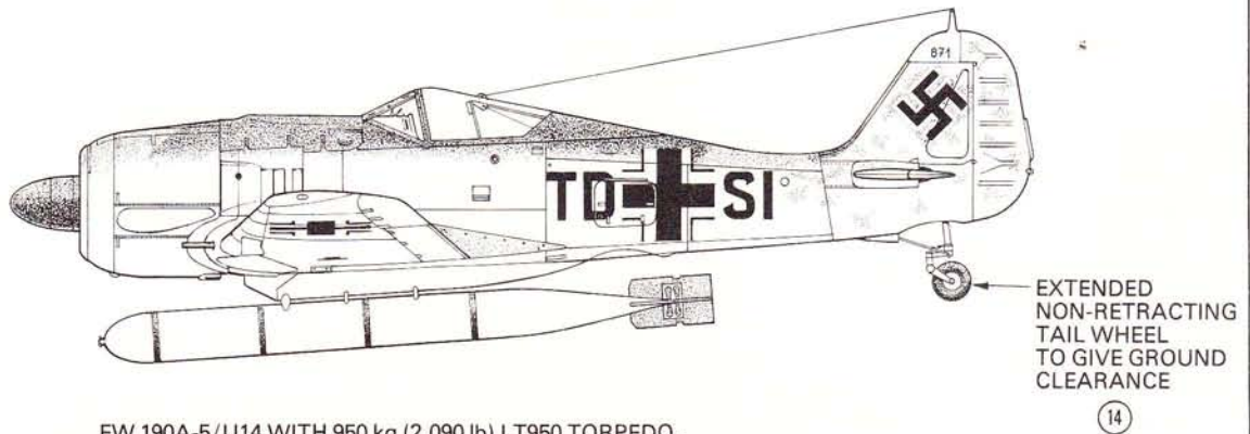
FW 190A-5/U14 WITH 950 kg (2,090 lb) LT950 TORPEDO. SIMILAR WAS THE FW 190A-5/U15 WHICH HAD PROVISION FOR TWO 300 LITRE FUEL TANKS UNDER THE WINGS. (13)
