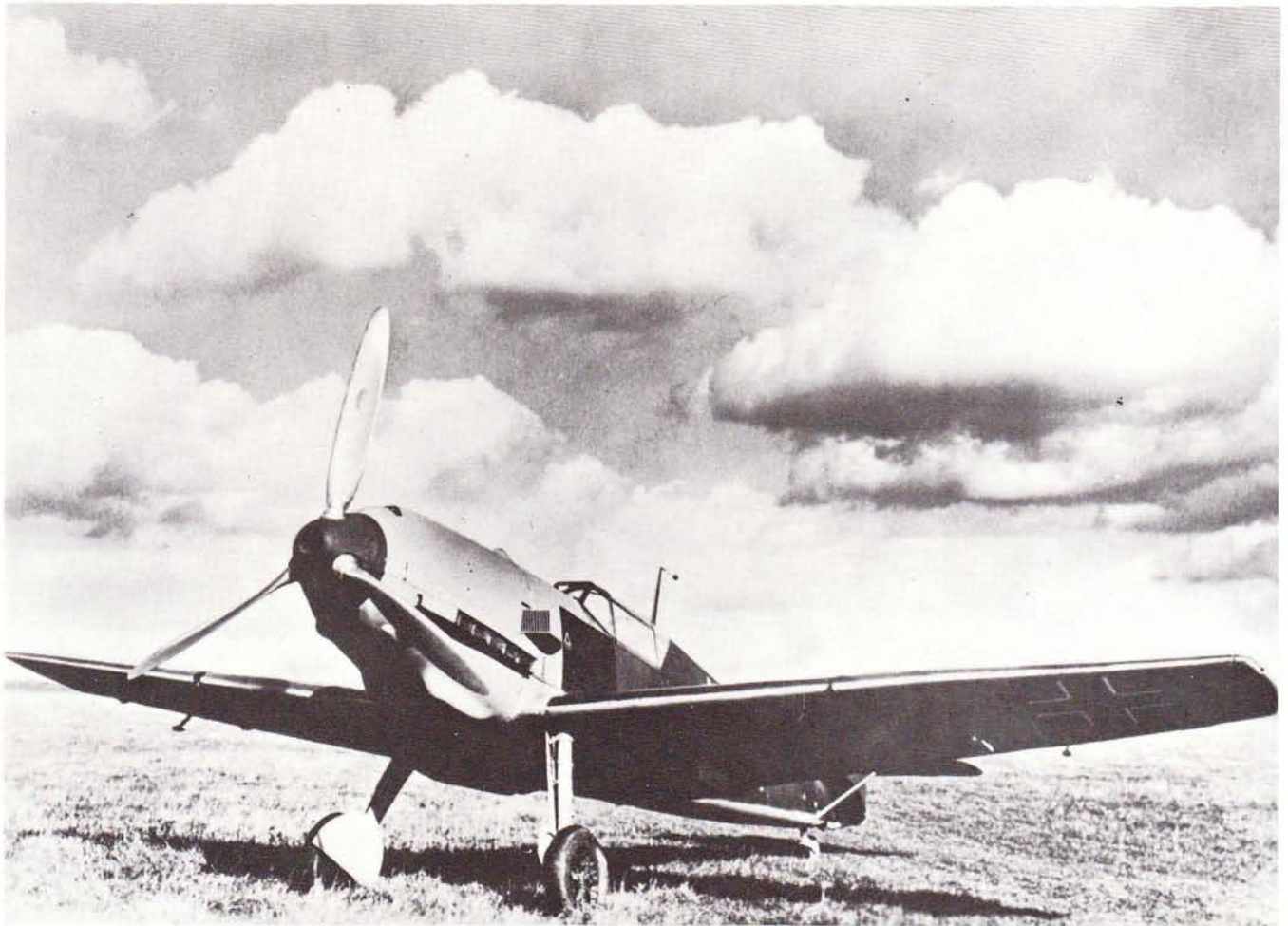
Fig. 4 First development aircraft for the E-series was the Me 109 V14, which began flight trials in the summer of 1938 and was eventually registered D-IRTT.
