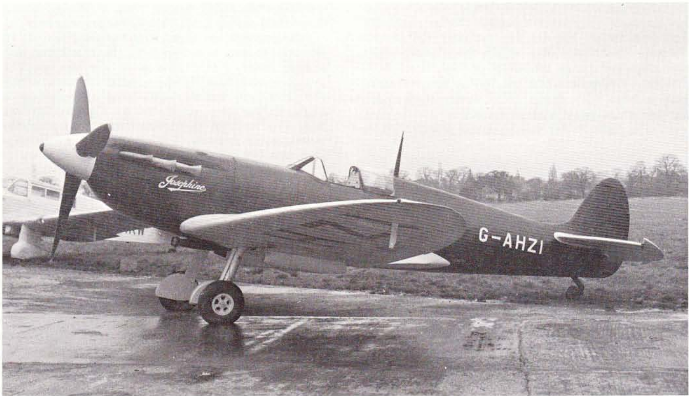
Fig. 23 This "civilianised" Spitfire II (ex P8727) was re-engined in 1946 with a 1,440hp Merlin 45 for a private owner. Painted black and cream, and named "Josephine", it crashed on take-off from Kastrup, Copenhagen in April 1947. [E. J. Riding.]
