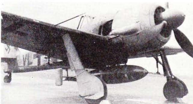
Fig. 26 FW 190A-4 VL+FG carrying a Blohm and Voss Bv 246 glider bomb.
