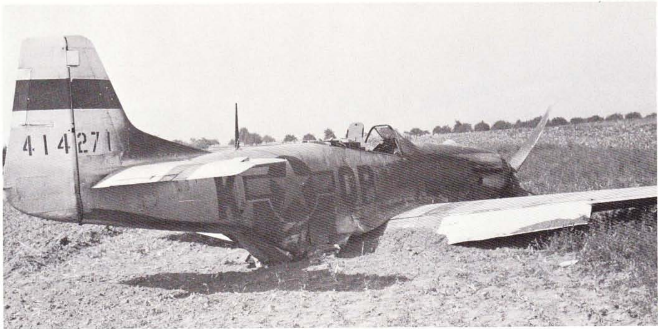
Fig. 4 A coolant leak forced this 4th FG P-51D to crash-land in Germany on 12 September 1944—on only its second mission.
