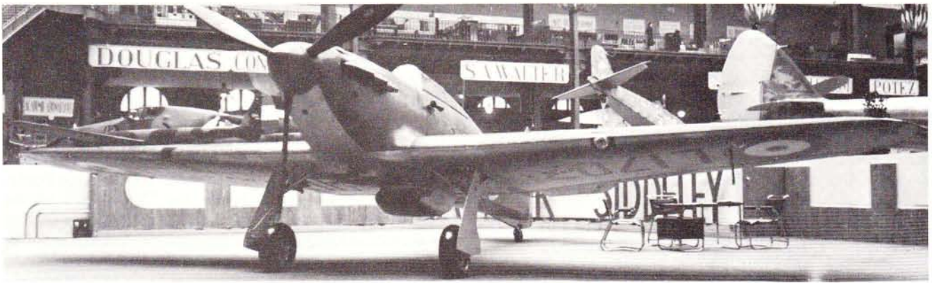
Fig. 9 Hurricane I L1707 was displayed on Hawker Siddeley's stand at the 1938 Paris Air Show, afterwards being allotted to No 79 Squadron at Biggin Hill. Note triple ejector exhaust manifolds and ventral fin. Latter was introduced on production aircraft from March 1938 and at the same time the hitherto retractable tailwheel was fixed.
