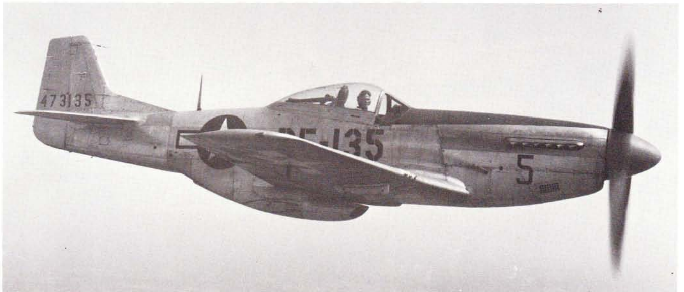
Fig. 17 After WW2, military aircraft in the United States were allocated “buzz numbers” to aid identification. These numbers consisted of a large two-letter code and the last three digits of the aircraft’s serial. The Mustang was coded PF and the application can be seen in the photograph.
