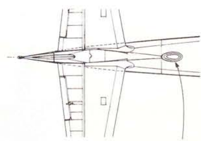
ENCLOSED HOMING DEVICE FITTED TO POSTWAR AIRCRAFT ⑦
