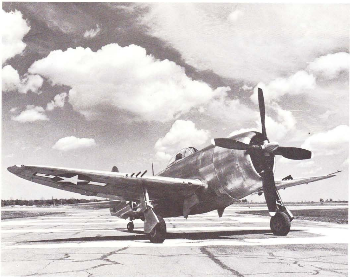
Fig. 13 A bubble canopy P-47D-26-RA in natural metal finish and uncluttered by underwing pylons. Curtiss Electric propeller. [Republic via R. A. Freeman]
