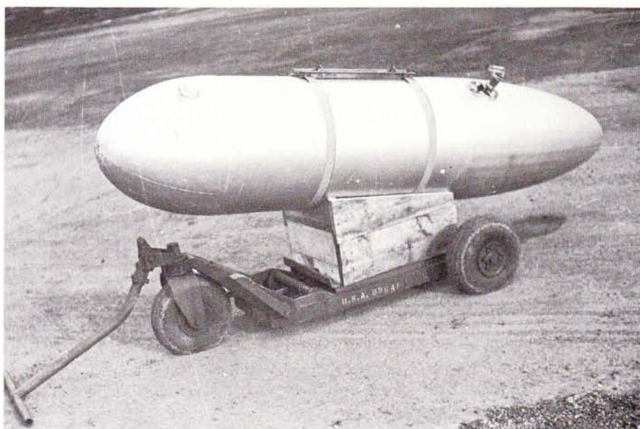
Fig. 8 The 108 US gallon (409 litre) "paper" drop tank manufactured in England for the 8th Air Force.
