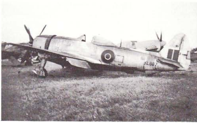
Fig. 18 The very last RAF Thunderbolt II, KL887, a P-47D-40-RA (USAAF No 44-90335) in stained natural metal finish but with 'duck egg' fuselage band, shallow dorsal fin fillet and underwing rocket clips, which was finally scrapped at RAF Lichfield in 1947. [Author]
