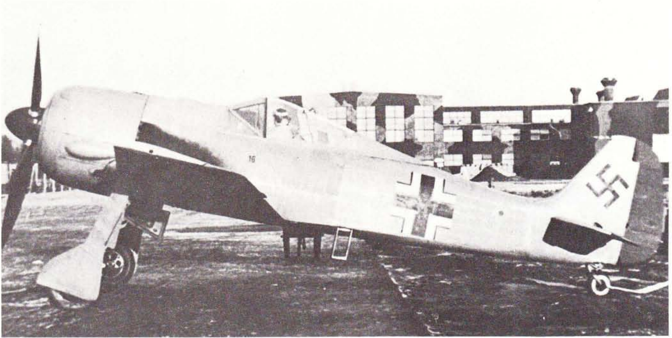
Fig. 6 The first pre-production batch of the FW 190 were known as A-Os, and from the eighth one onwards they featured an enlarged wing, as seen on this example, to improve manoeuvrability.
