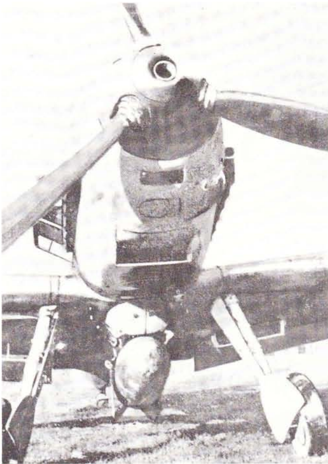
Fig. 19 A 250kg bomb-carrying Me 109E-4B of III/JG1. Fig. 20 Head-on view of an E-4B with a 250kg bomb slung from the ETC 500 belly rack.
