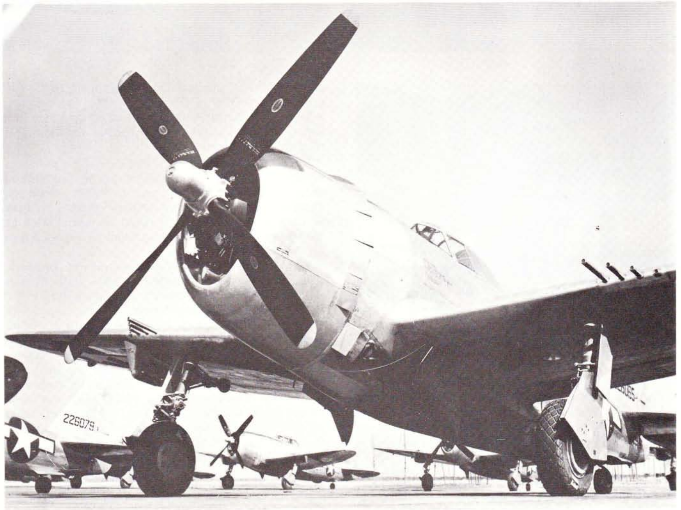
Fig. 6 More P-47D-22-REs at Farmingdale including 42-25974, 42-26065 and 42-26079. Blunt hub of the Hamilton Standard propeller and underwing stores pylons show in this photograph. [Republic via R. A. Freeman]
