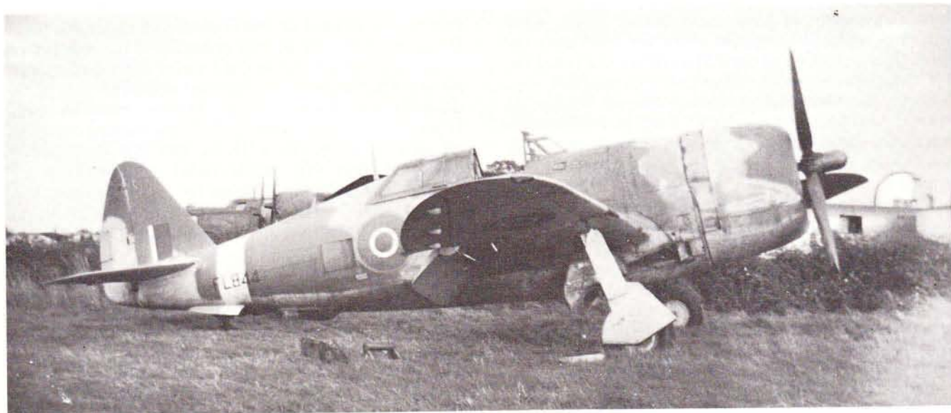
Fig. 17 A razorback RAF Thunderbolt I, FL844 (USAAF No 42-25792) was a P-47D-22-RE retained in the United Kingdom for evaluation. It wore standard Fighter Command colours and is seen here in 1946 at RAF Lichfield awaiting scrapping. [Author]
