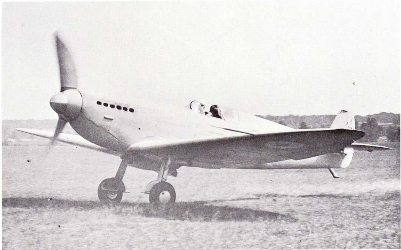
Fig. 4 Take-off shot of K5054 when fully painted and fitted with hinged wheel fairings and redesigned rudder with smaller horn balance. Pilot is Jeffrey Quill.
