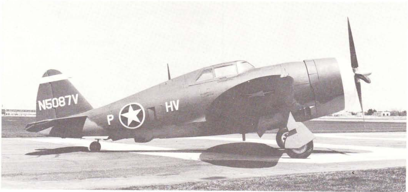
Figs. 10 & 11 In the uppermost of these two additional views of 42-23278 the machine is seen to have a D/F aerial "egg" under its belly. [Republic via R. A. Freeman]
