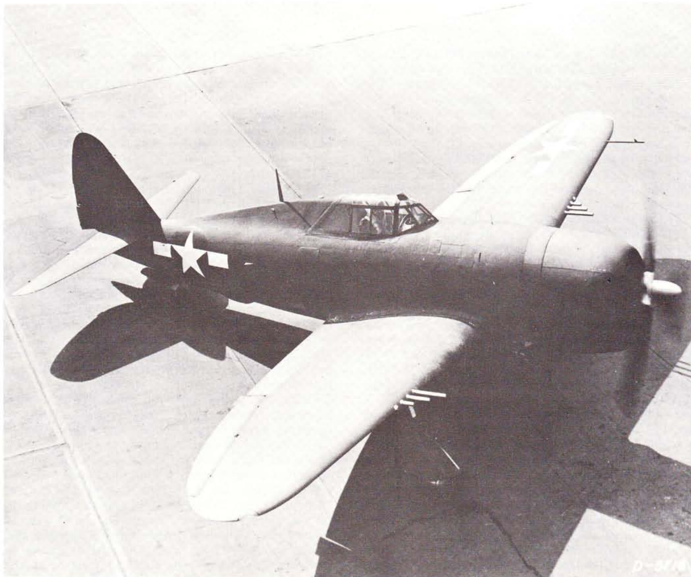
Fig. 3 In this view a P-47D-11-RE, 42-75568, clearly portrays the elliptical planform wing, pointed windscreen, framed sliding cockpit canopy and sharp rear fuselage spine. The wing guns and pointed hub of the Curtiss Electric propeller stand out sharply. (Republic via R. A. Freeman)
