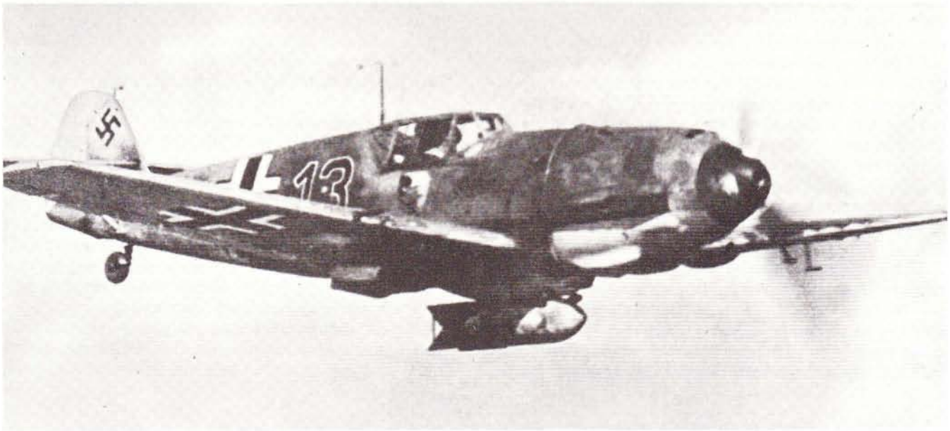
Fig. 19 A 250kg bomb-carrying Me 109E-4B of III/JG1. Fig. 20 Head-on view of an E-4B with a 250kg bomb slung from the ETC 500 belly rack.
