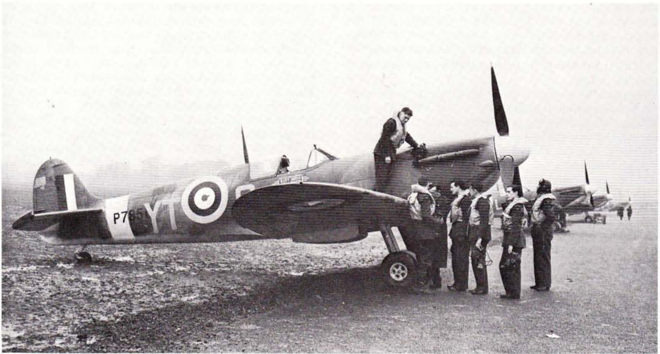
Fig. 19 Sole external distinguishing feature of the Spitfire II was the small blister over the Coffman cartridge starter on the starboard side of the nose immediately behind the propeller, as seen on this IIA of No 65 Squadron.
