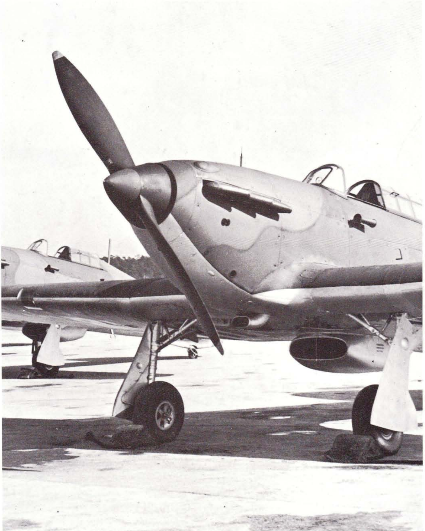
Fig. 1 Brand new Hurricanes at Brooklands aerodrome before the war. They have the original Watts two-bladed wooden propellers but instead of the early "kidney" type exhaust stubs they have Rolls-Royce exhaust ejector stubs. Note the flight instrument venturis on the aircrafts' cockpit walls.
