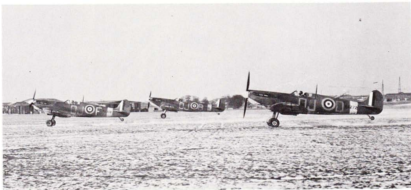
Fig. 22 Two of No 92 Squadron's trial cannon/machine-gun Spitfire IBs (R6908 QJ-F and X4272 QJ-D) take off from Manston, Kent, in company with an unmodified Mk IA (X4561 QJ-B) in December 1940.
