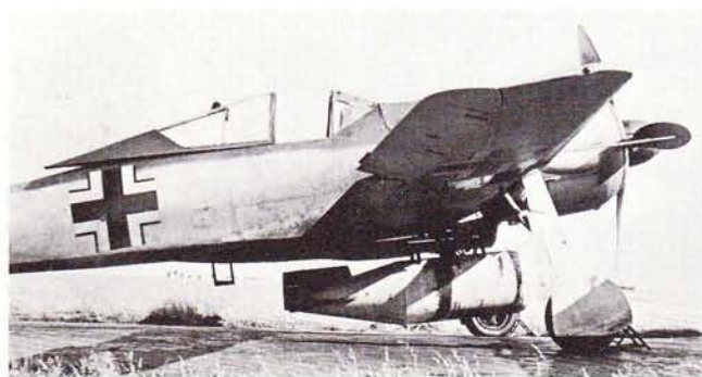
Fig. 22 An A-4/U8 long-range fighter-bomber with two 300-litre drop tanks and a SC 500 bomb. Fig. 23 An A-5/U8 long-range fighter-bomber with a 1000kg SB 1000 bomb, lower fin of which has been removed for ground clearance.
