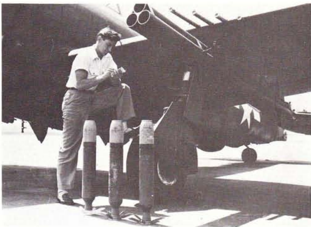
Figs. 7 & 8 Close-ups of a Republic P-47D-20-RA fitted with three launcher tube clusters for 4.5in (11.43mm) folding fin rockets under each wing. [Republic via R. A. Freeman]
