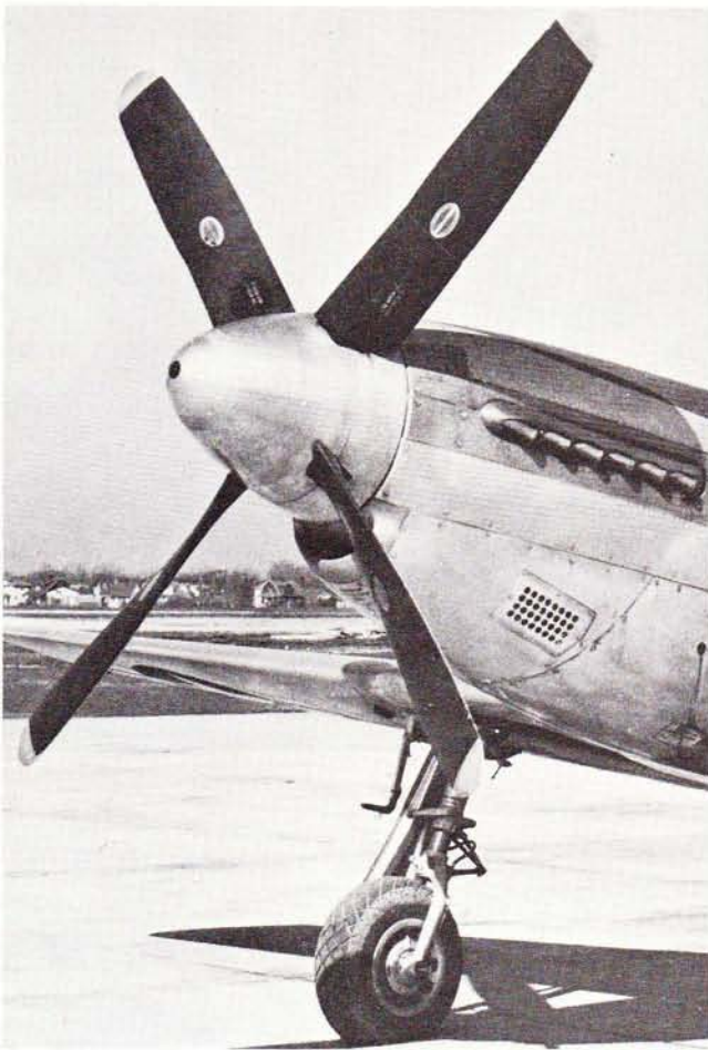
Fig. 25 P-51D close-up showing the Hamilton Standard 4-blade hydromatic propeller of 11ft 2in (3403.6mm) diameter.
