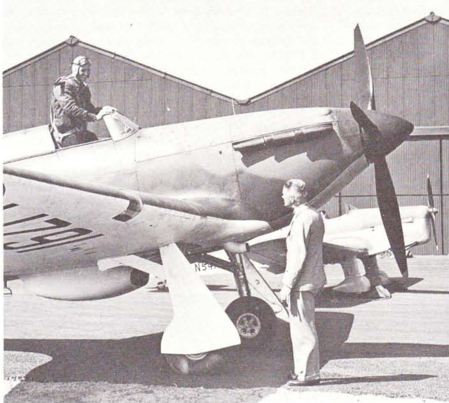
Fig. 9 Hurricane I L1707 was displayed on Hawker Siddeley's stand at the 1938 Paris Air Show, afterwards being allotted to No 79 Squadron at Biggin Hill. Note triple ejector exhaust manifolds and ventral fin. Latter was introduced on production aircraft from March 1938 and at the same time the hitherto retractable tailwheel was fixed.
