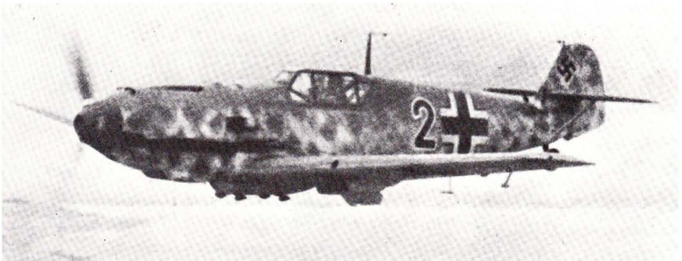
Fig. 16 The Me 109E-7. Except for having provision for either a 300 litre drop tank or a bomb load varying from a single 50kg bomb to one of 250kg, this model was identical to the E-4N.
