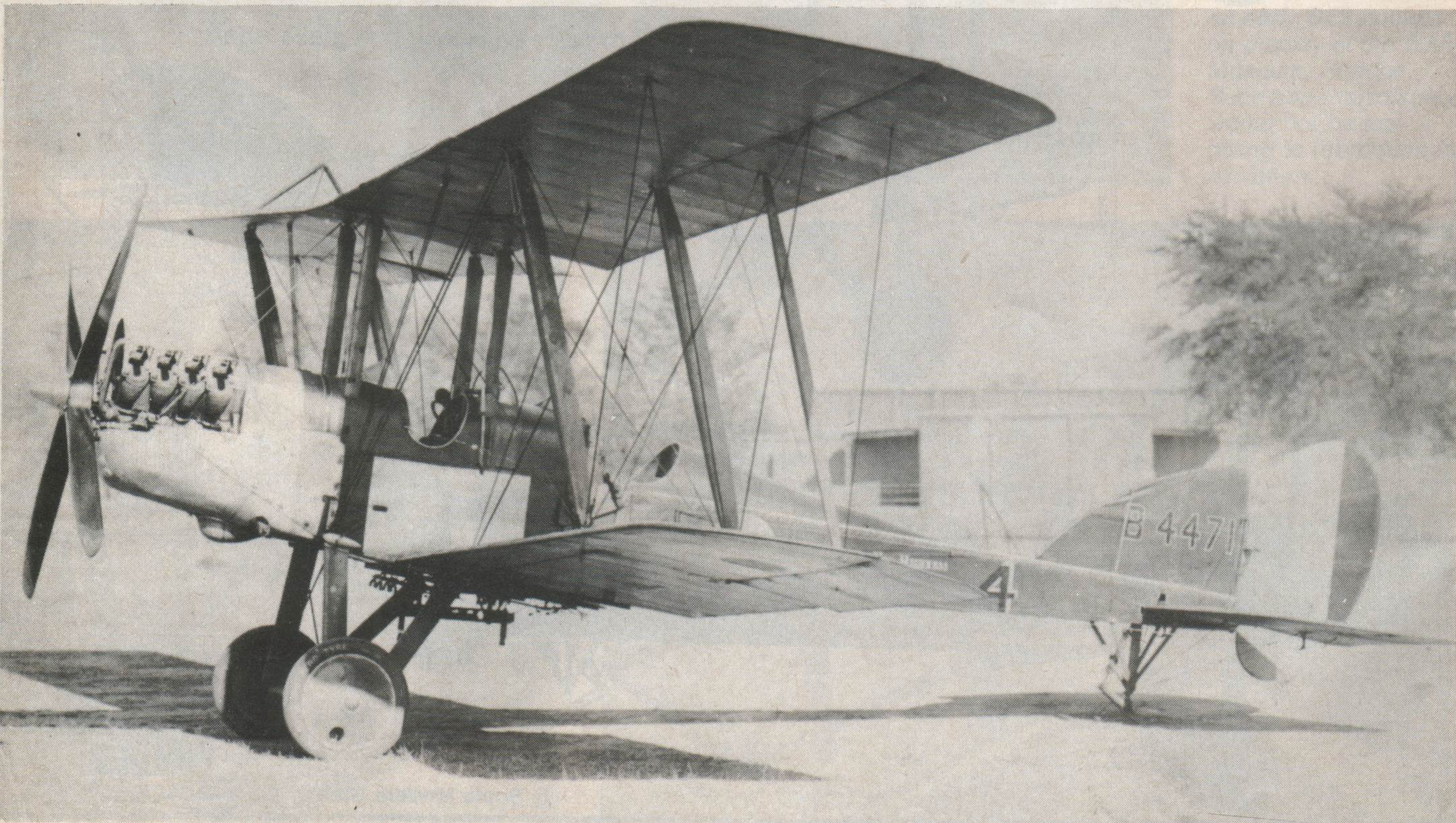
10. BE2e of No. 50 HDS bearing the squadron's skull and crossbones on fuselage sides and under upperwing surfaces outboard of struts. (See drawing on previous page). 11. BE2e B4471, built by the British and Colonial Aeroplane Co. Ltd., Filton. Note extra protection for observer in front cockpit by use of bolt-on metal plate! Plenty of modelling reference is afforded by close study of this excellent period photograph.
