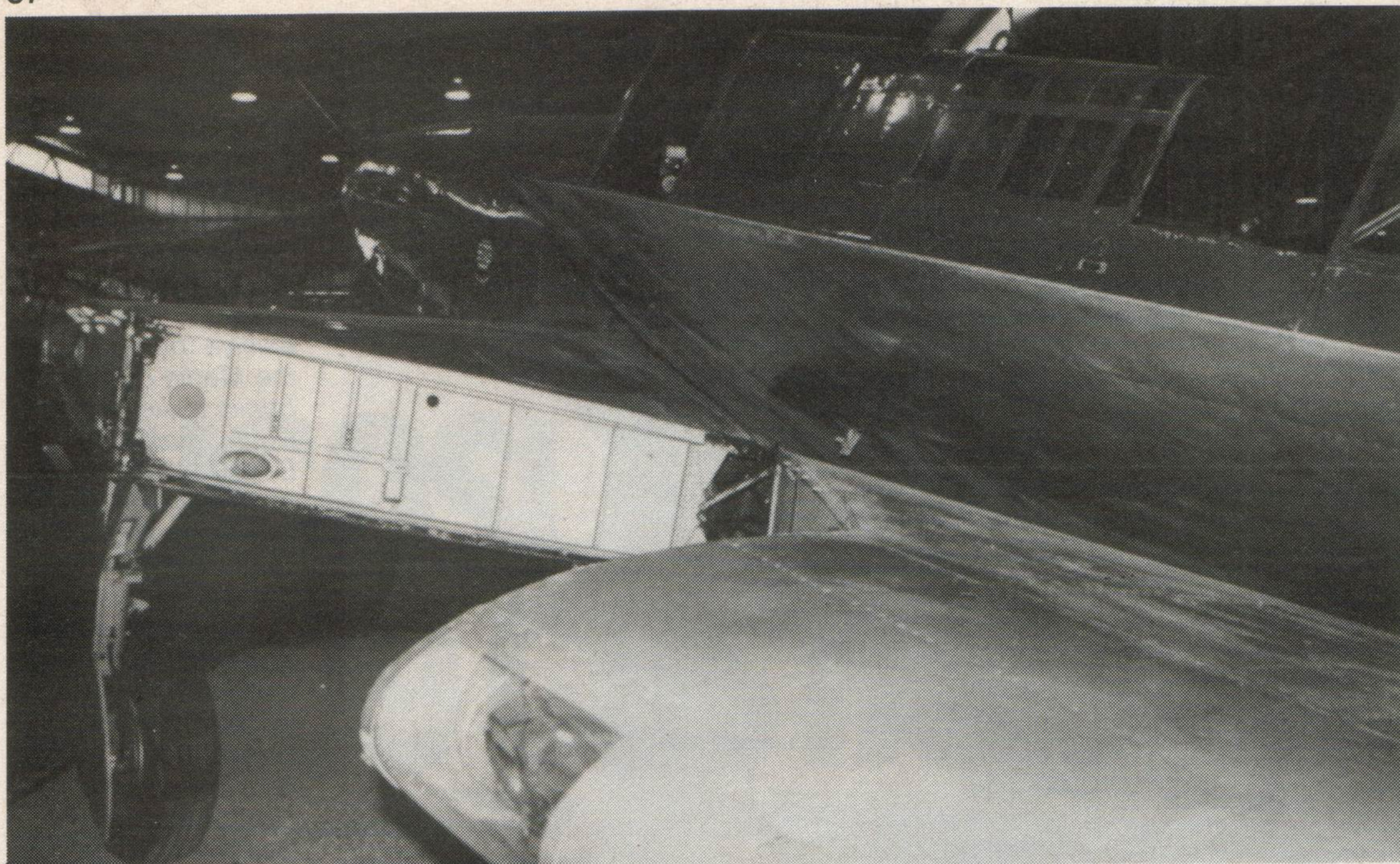
57. Wing-fold mechanism detail of the preserved prototype – note large leading-edge lamp and casing. 58. Prototype N1854 modified to Mk II standard and in non-standard 1942 type finish as revealed by the Sky Grey Spinner. 59. N1858 development airframe with yellow undersides. A large gas-detecting square was applied to the port tailplane of the aircraft.
