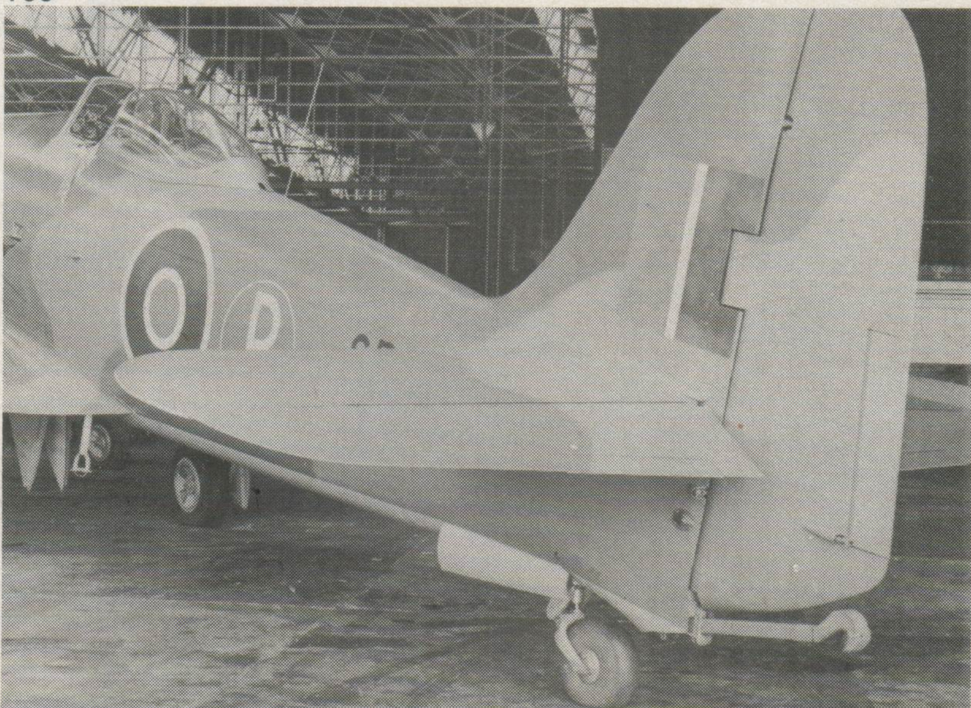
109. Prototype Sea Fury shows that neat installation of the extending sting-type arresting hook.
