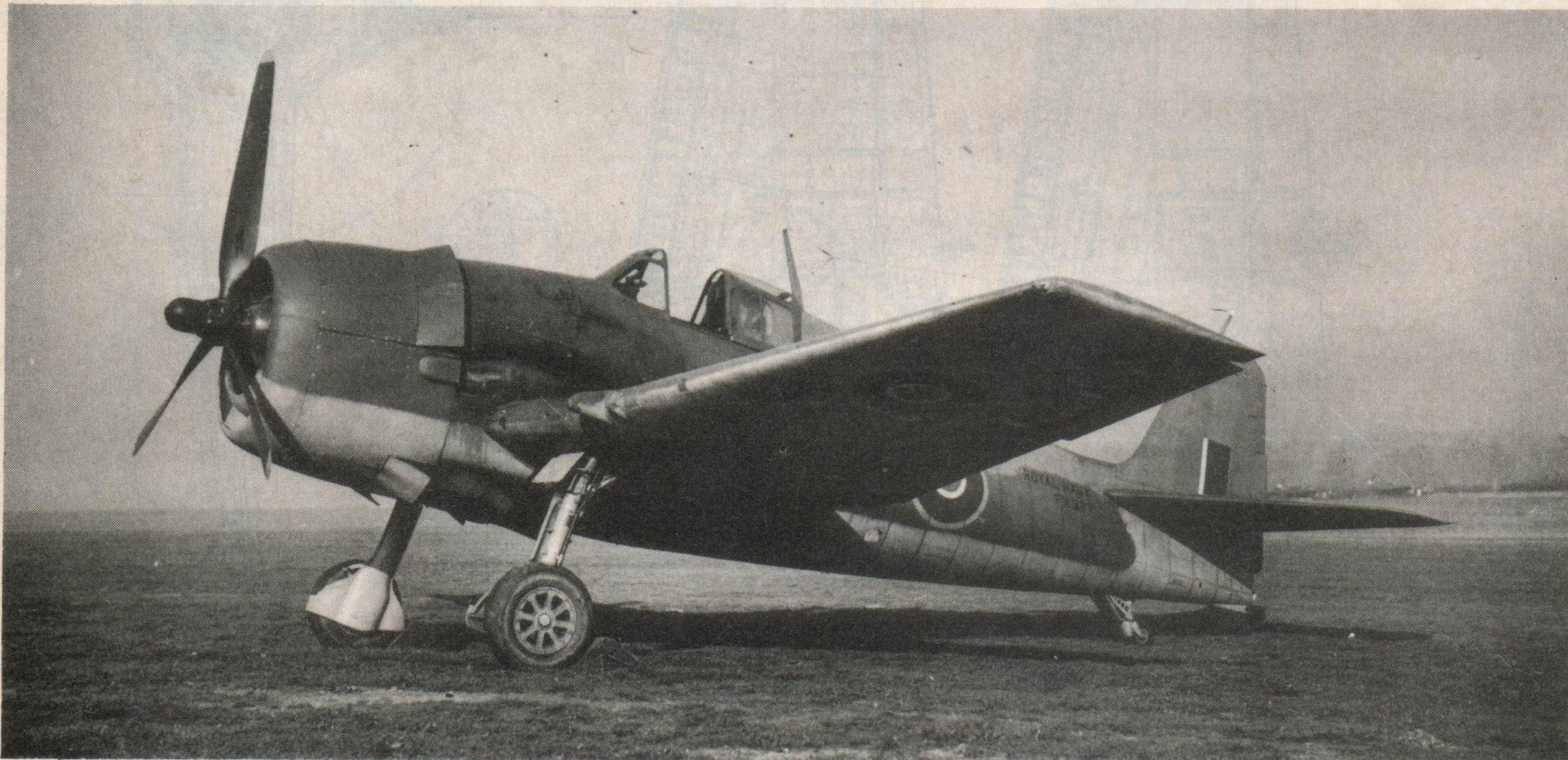
78. Grumman F6F-5N nightfighter with wing-mounted radar and flame-damped exhausts.
