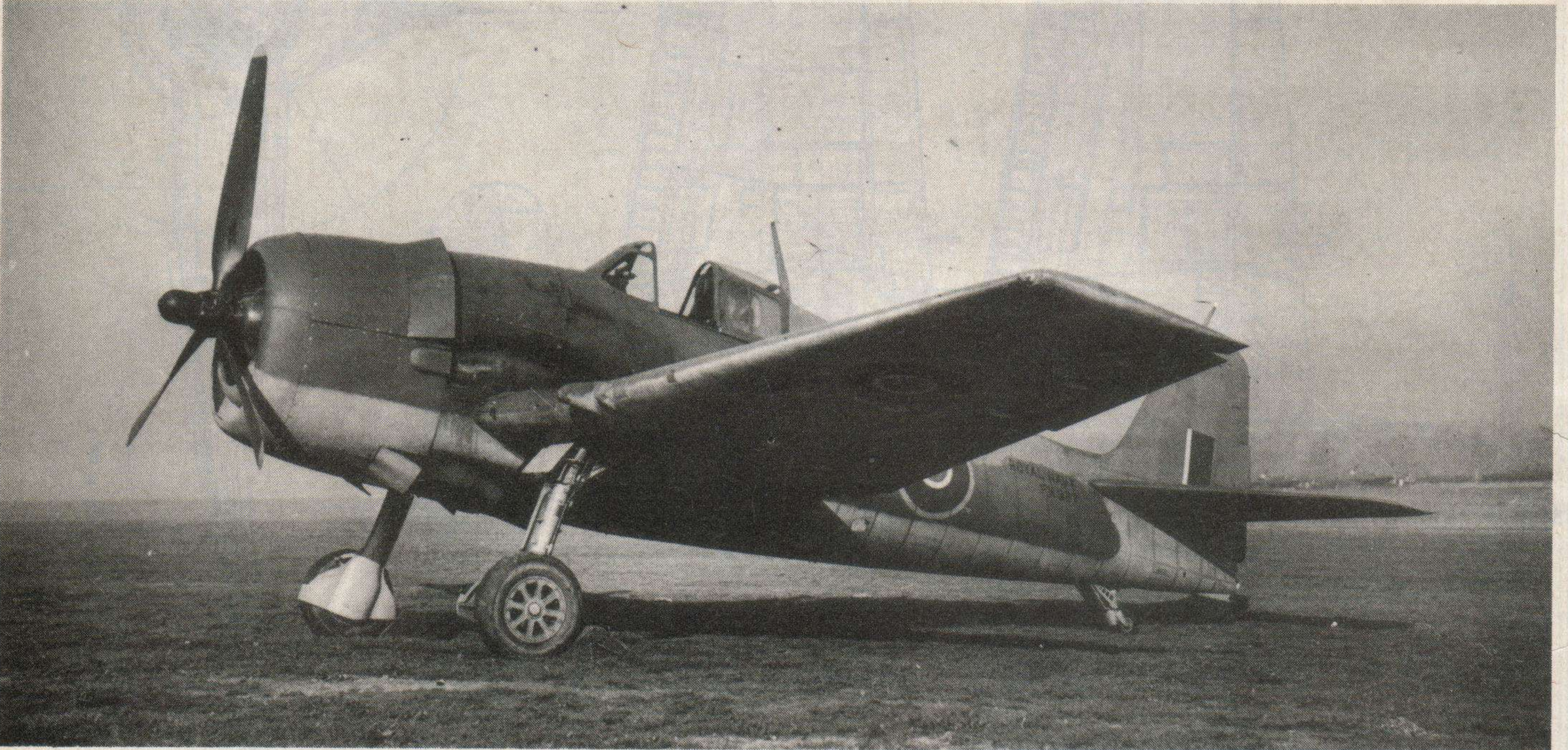
78. Grumman F6F-5N nightfighter with wing-mounted radar and flame-damped exhausts.
