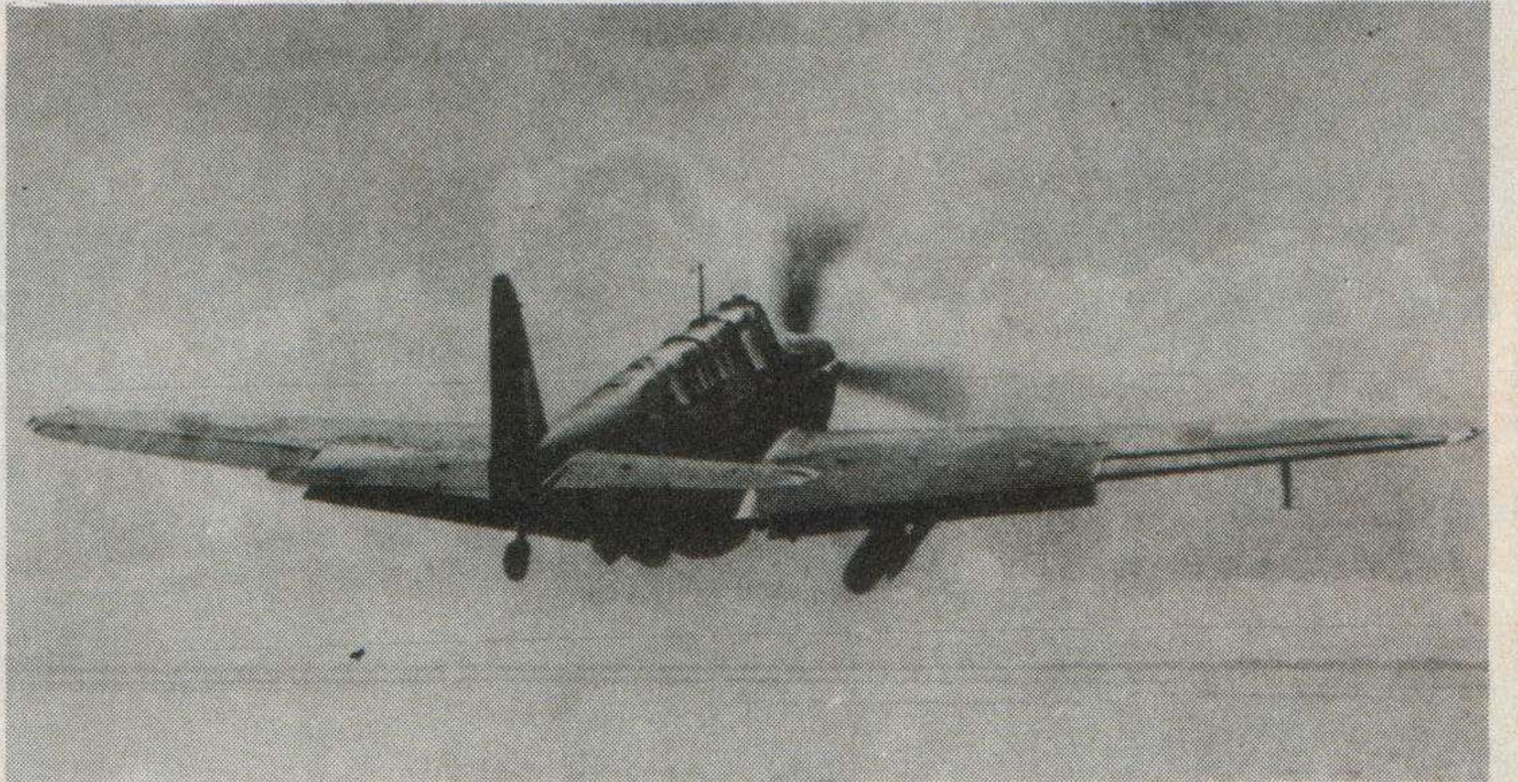
45. A Fairey Fulmar clears the flight deck of HMS Victorious in August 1942. Although of poor quality, this wartime photo illustrates the asymmetrical-retracting undercarriage to advantage. 46 and 47. Views of the prototype Fulmar preserved at the Fleet Air Arm Museum at Yeovilton. Particularly noteworthy is the fuselage shape beyond the air intake aperture (below) and its bulged cheeks (Photo 47). See drawing opposite.
