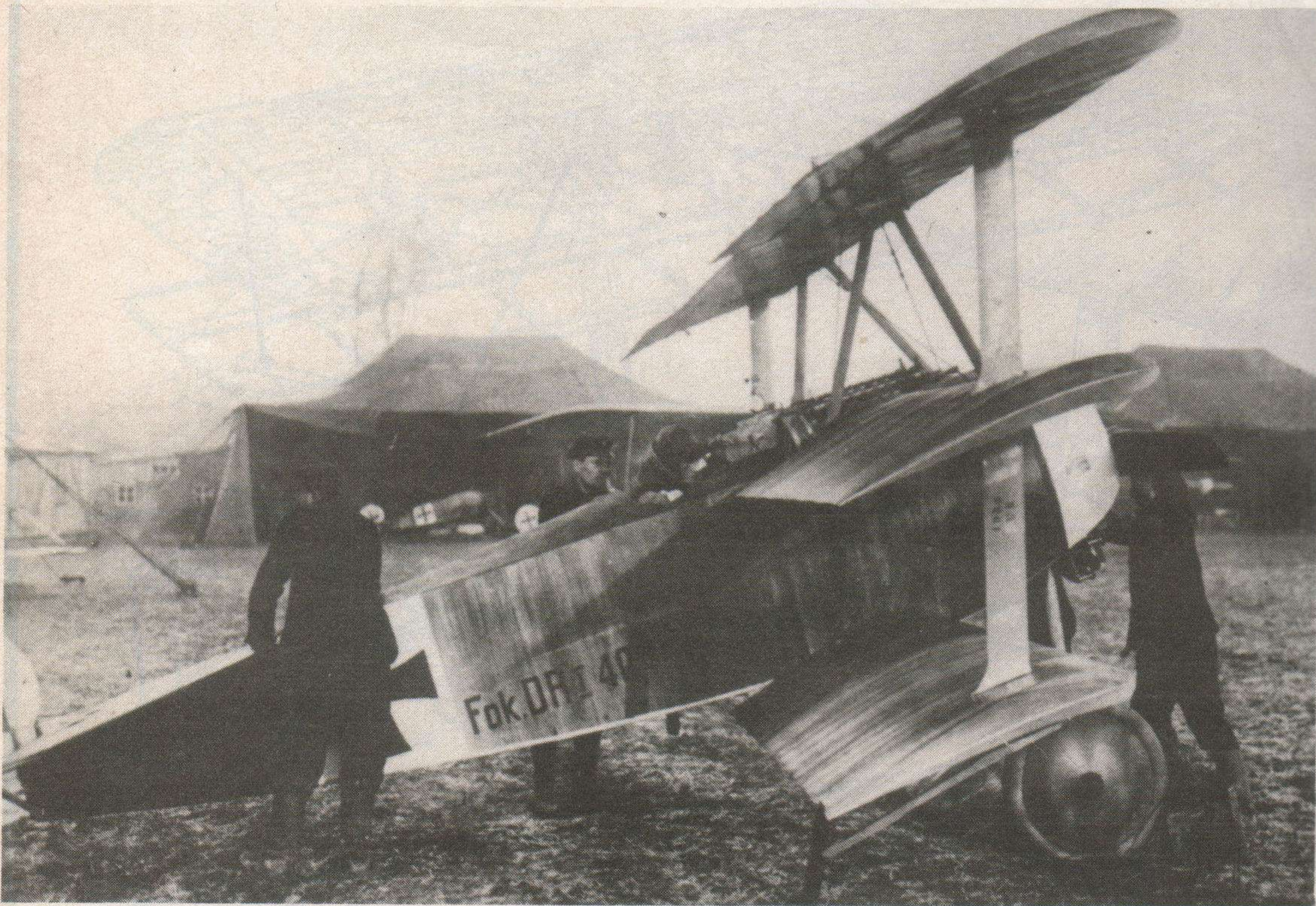
17. Leutnant Paul Rothe (five victories) stands before a Fokker Dri of Jasta 14, in the spring of 1918. Close study of this photo reveals the streaky Fokker camouflage to good effect. Not easy to reproduce accurately in miniature, this method of colour application was a time-saving and simple operation for Fokker factory workers. The turquoise blue undersurface colour was much more solid and here the outlining use of this colour can be plainly seen.
