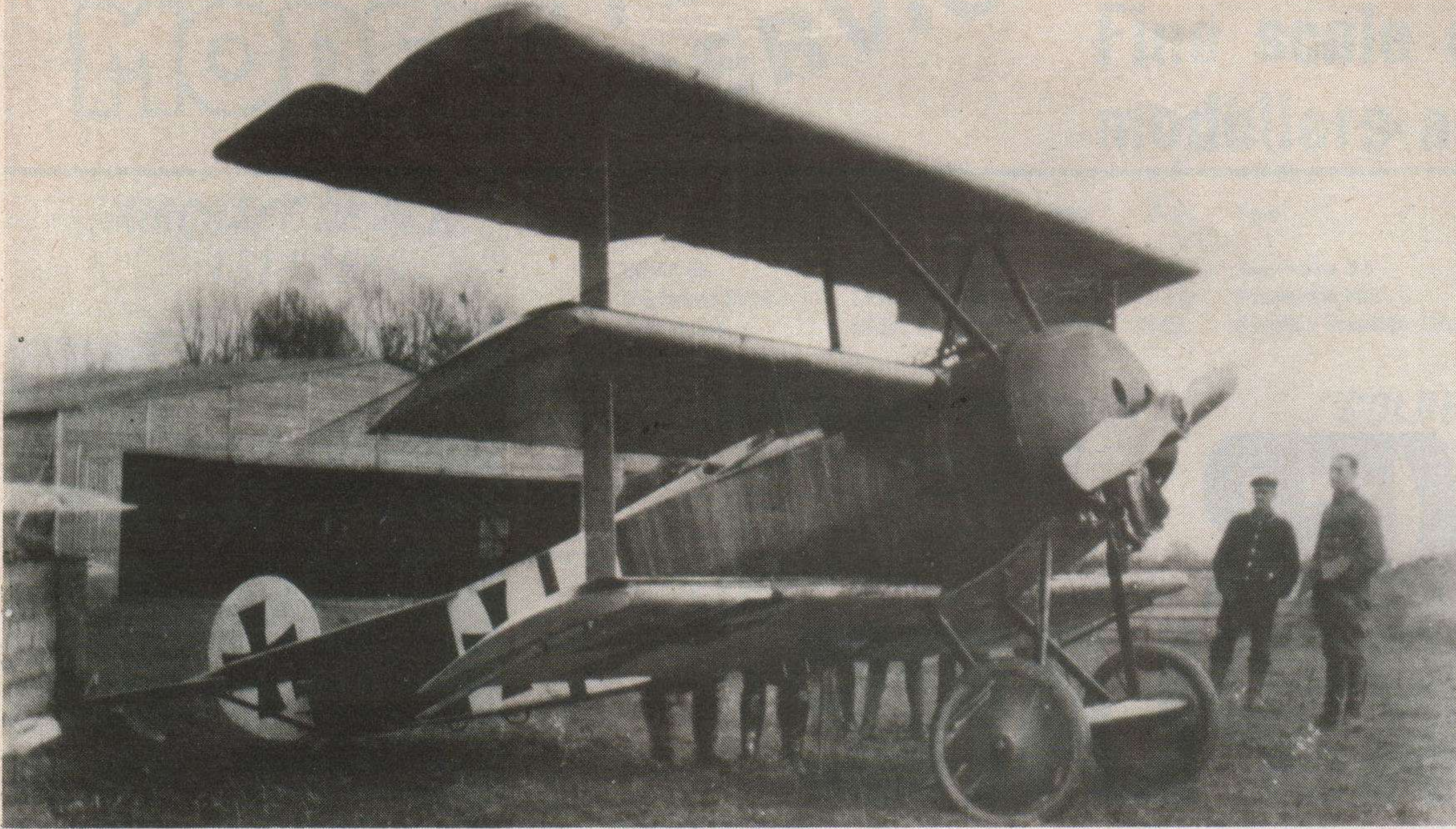
13. A standard production Fokker DrI with late-type ailerons. Note how the lower surface turquoise dope overlaps the lower fuselage longeron even continuing over the white cross panel in many instances – as here.
