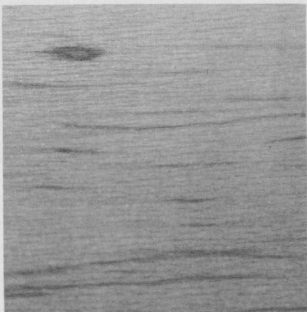
Above, left: straight grained balsa and above right: quarter grain, characteristic 'fleck' to the surface distinguishes this cut.
