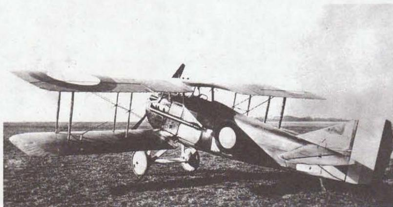
V-type engines which at first delivered 200 hp and were soon improved to 220 hp at sea level. Among the most streamlined of WW I airplanes, it had a top speed of 134.5 mph. It could climb to 6,500 feet in 5 minutes 17 seconds and could reach a ceiling of slightly over 22,000 feet.
