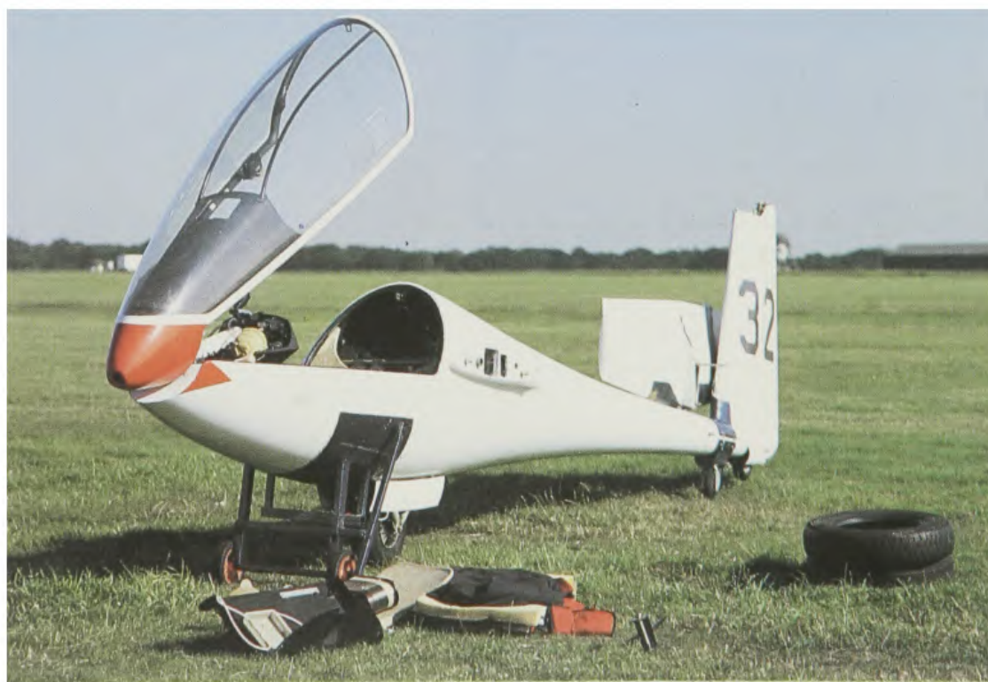
Top A fuselage support to help rigging with only two people.
