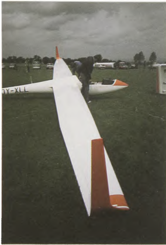
Winglets on an ASW-20 to help reduce induced drag.
