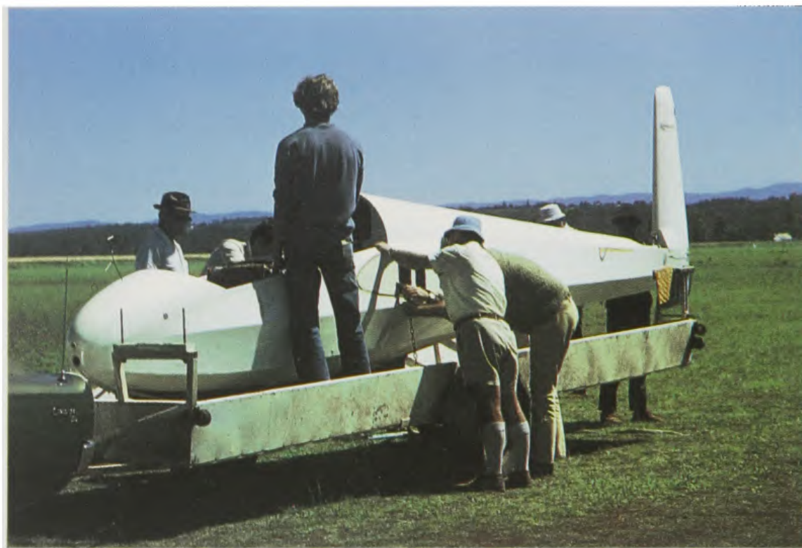
A typical club open trailer which can be persuaded to carry different types of glider.
