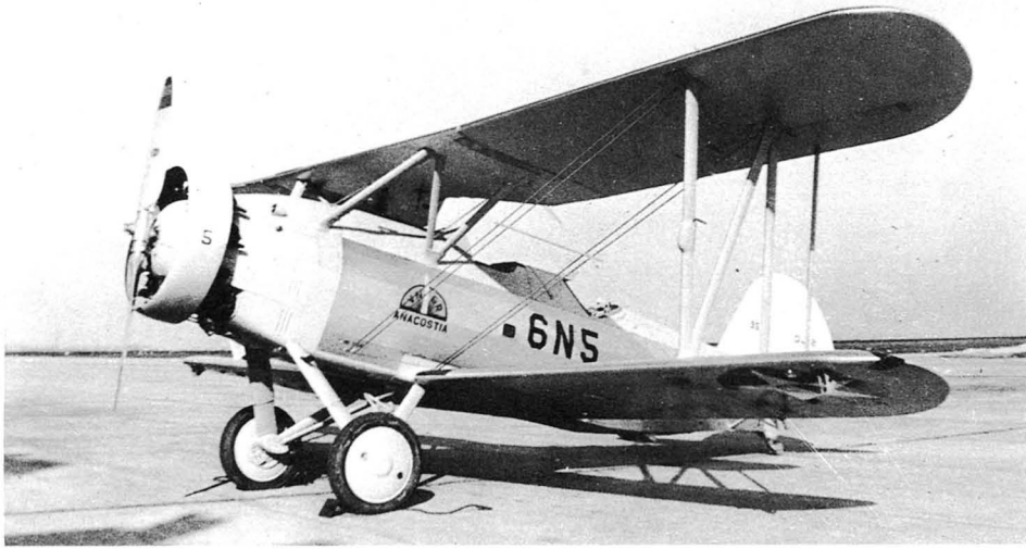
Left: A Berliner Joyce OJ-2 reserve aircraft shows the squadron insignia and designation on the side of the fuselage. Note the color shift from metal to fabric areas.
