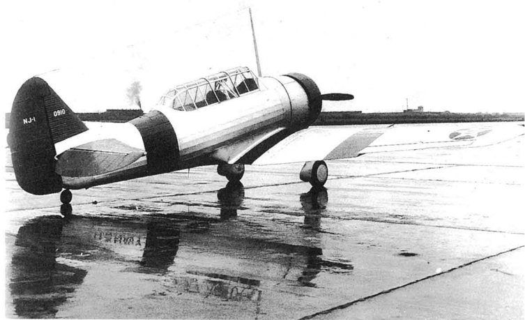
Above: This photo of October 13, 1937, shows a North American NJ-1, assigned to the training command for instrument training. Note the red bands around the wing and fuselage denoting an instrument trainer. It is believed that the tail and engine cowl are also Insignia Red. Above right: The number four aircraft of VS-9S assigned to the heavy cruiser Salt Lake
