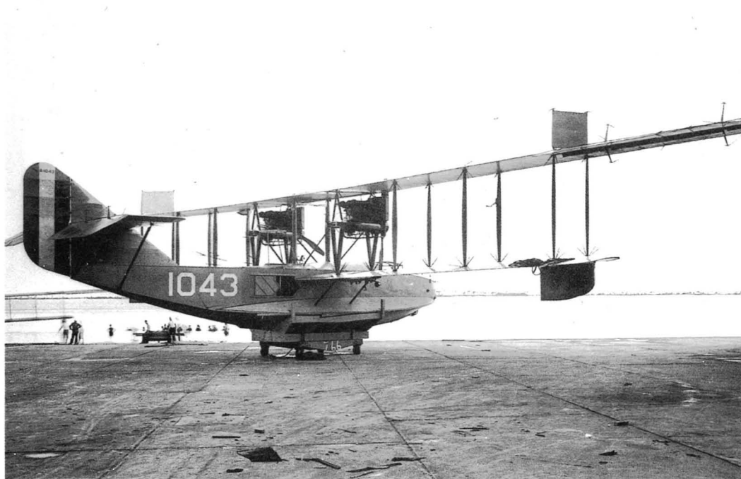
Left: This Curtiss H-16, photographed on August 23, 1918, is a good example of the inconsistency of the early markings. Note that the aircraft serial number on the white rudder stripe has the letter A prefix while the fuselage designation does not.
