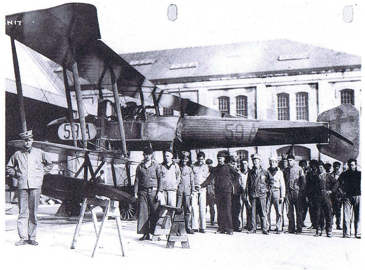
Right: The Gallaudet AH-61 is shown in January 1917, with the aircraft serial number applied to both the front and rear fuselage. This should read A-59. Note the midship position of the propeller on this unusual aircraft.
