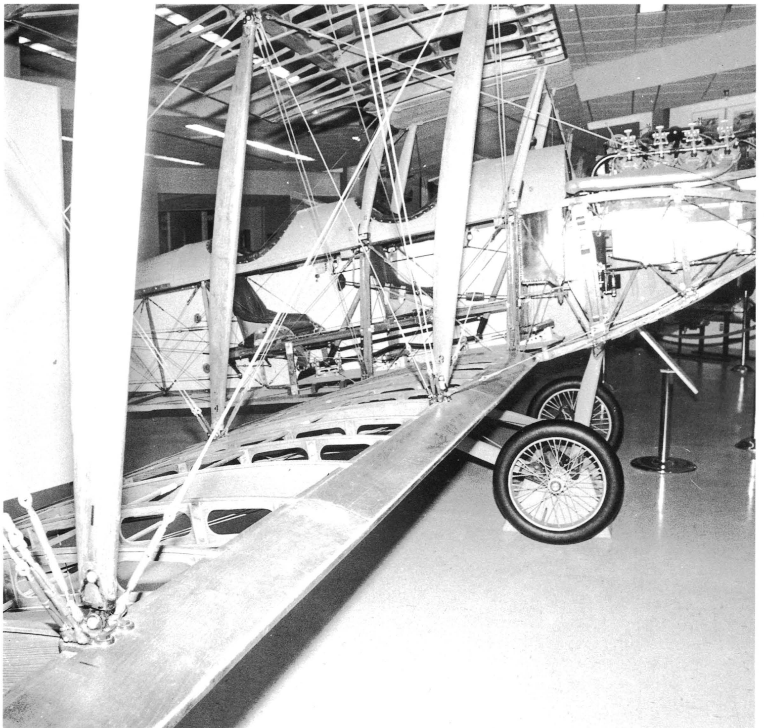
Right: Wing strut numbers have been applied to the restored Curtiss JN-4D at the US Naval Aviation Museum, Pensacola, Florida, in accordance with Aeronautical Specification No. 49. Below: Overall view of the same aircraft as shown in the close-up view.
