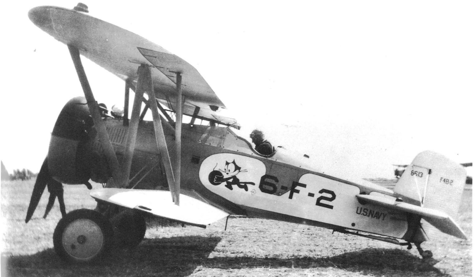
Above: A Boeing F4B-2 is shown assigned to the Commanding Officer of Fighting Squadron Six (VF-6B). The full cowl and section leader fuselage band are Insignia Red. Note the variation between the gray metal and aluminum fabric. Below: This shows another Boeing F4B-2 of VF-6B assigned to the
