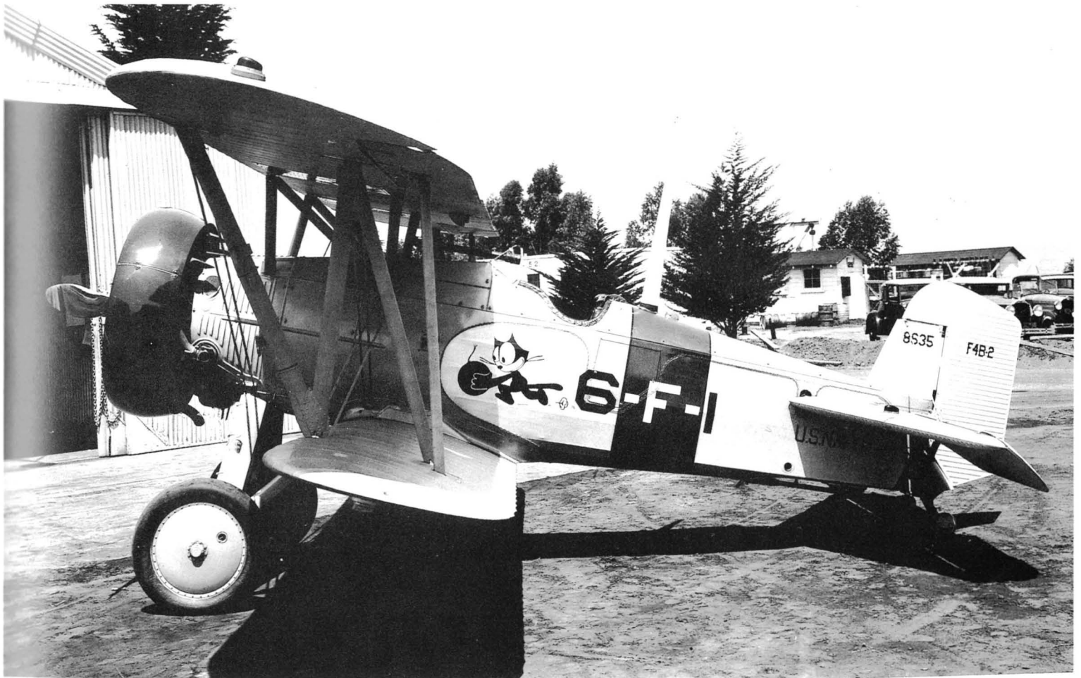
Above: A Boeing F4B-2 is shown assigned to the Commanding Officer of Fighting Squadron Six (VF-6B). The full cowl and section leader fuselage band are Insignia Red. Note the variation between the gray metal and aluminum fabric. Below: This shows another Boeing F4B-2 of VF-6B assigned to the
