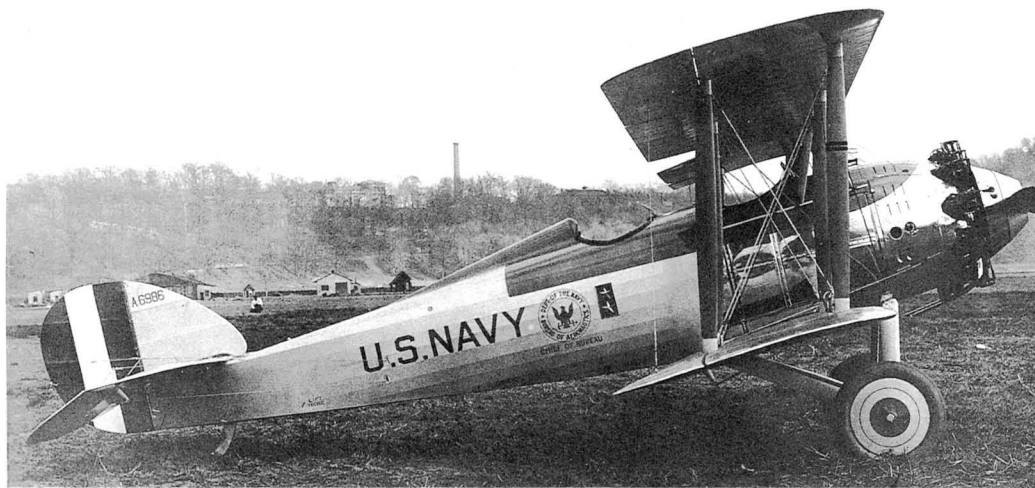
Left: This UO-1 (A-6986) was assigned to the Chief of the Bureau of Aeronautics, Admiral W.A. Moffett. The highly polished cowling and Dark Blue cockpit area is believed to be the first of the special staff aircraft paint schemes with Bureau approval. Opposite lower: The fuselage of this De Havilland DH-4B (A-6371) was painted blue in the manner of an Admiral's barge. This particular machine was assigned to LCdr. Millington B. McComb, Commanding Officer of Naval Air Station Pearl Harbor.
