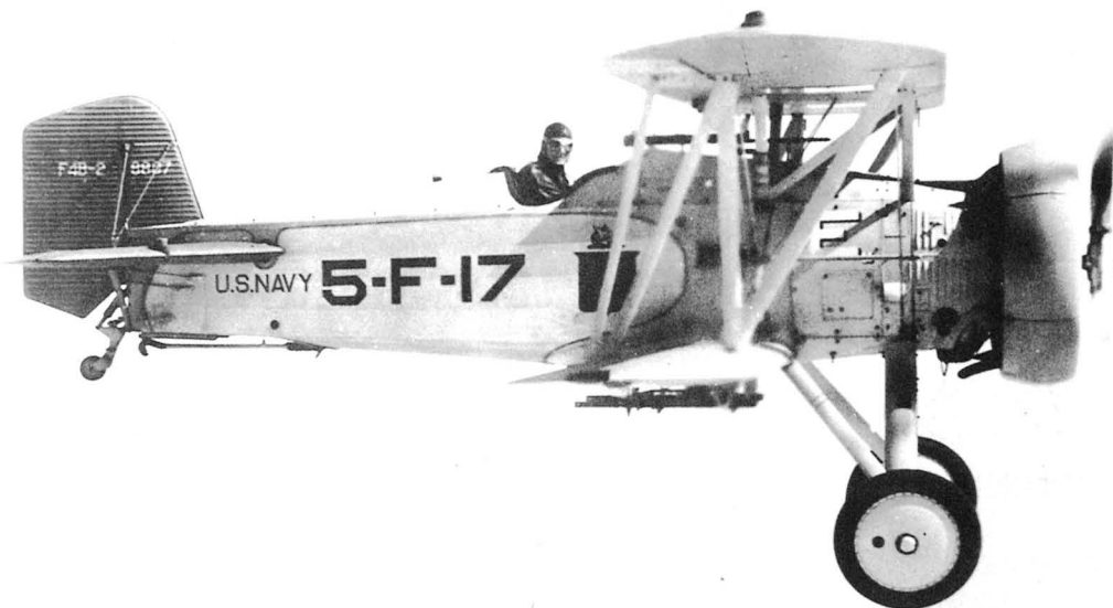
Left: Squadron missions changed frequently and the "Red Rippers" are once again a fighting squadron in 1932 flying Boeing F4B-2s. The Navy "E" has a shadow outline to make it more prominent against the Light Gray of the forward fuselage. Flying from the USS Lexington the tail color is True Blue.
