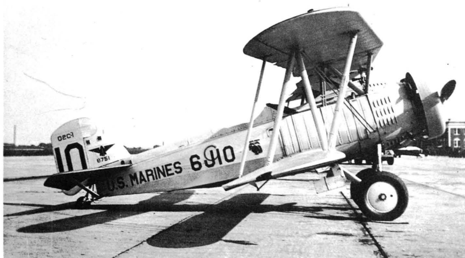
Left: This is a Curtiss O2C-1 of VJ-6M, Aircraft One, Quantico, Virginia. The large aircraft number on the rudder and Aircraft One insignia on the vertical fin are unusual.
