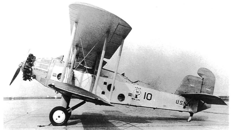
since they were flown on alternate weekends by the different squadrons assigned to the base. Below: This Curtiss F8C-4 also was assigned to the Naval Reserve Air Base in New York. The chevron on the upper wing appears to be white, outlined with black, but the upper half of the cowl shows that it should be a dark color. What appears to be a letter "C" behind the station insignia is an inspection panel, not a marking.
