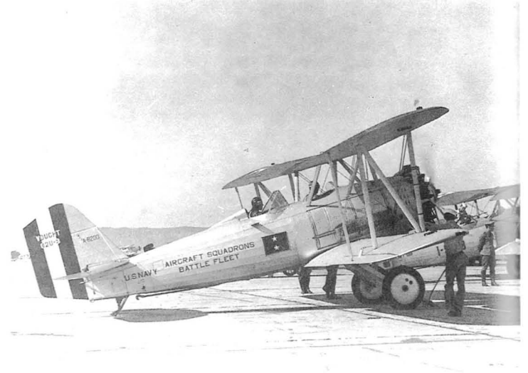
Three (VF-3B) is shown here. The horizontal stripe on the tail appears to be a special marking for use in a maneuver as no such markings are known to have been in general use at this time. The metal surfaces appear to be far too dark. Note that the aircraft serial number 7720 is painted vertically on the fin due to its narrow width.
