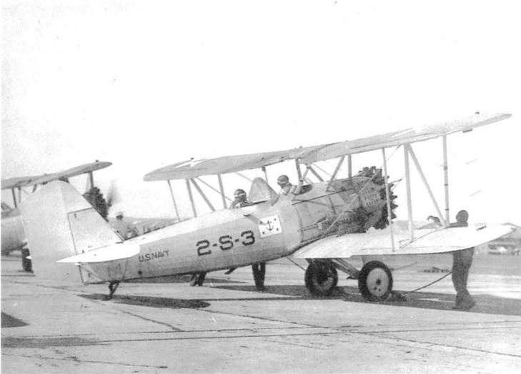
Above: The Assistant Secretary of the Navy for Air is being flown in this Vought O2U-2 of VS-2B during October 1929. Note his flag on the side of the fuselage. Above right: The Rear Admiral commanding Aircraft Squadrons, Battle Fleet is being flown in his staff aircraft from NAS North Island, San Diego, in October 1929. Note the oversize windscreen and headrest provided for additional comfort. Below: A Boeing F3B-1 of Fighting
