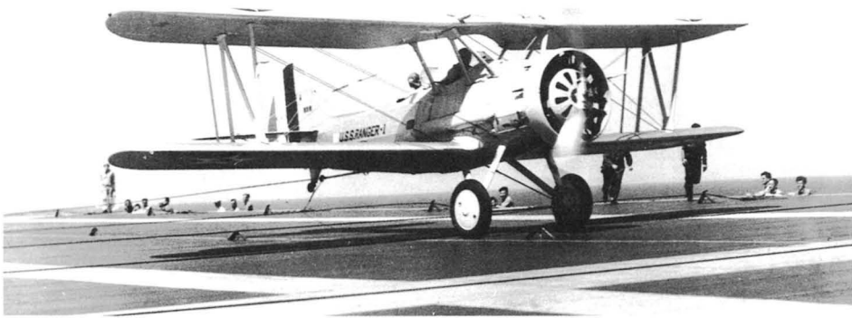
Left: This Vought O3U-3 number 1 utility aircraft is shown aboard the USS Ranger. It is an unusual photo for the period, showing the arresting cables being held off the deck by the fiddle bridges so that the aircraft's tail hook can engage them. Below: A Bellanca JE-1 utility transport assigned to the Naval Air Station Anacostia, Washington, DC shows the base name in the location normally used for the squadron number, type, and aircraft number.
