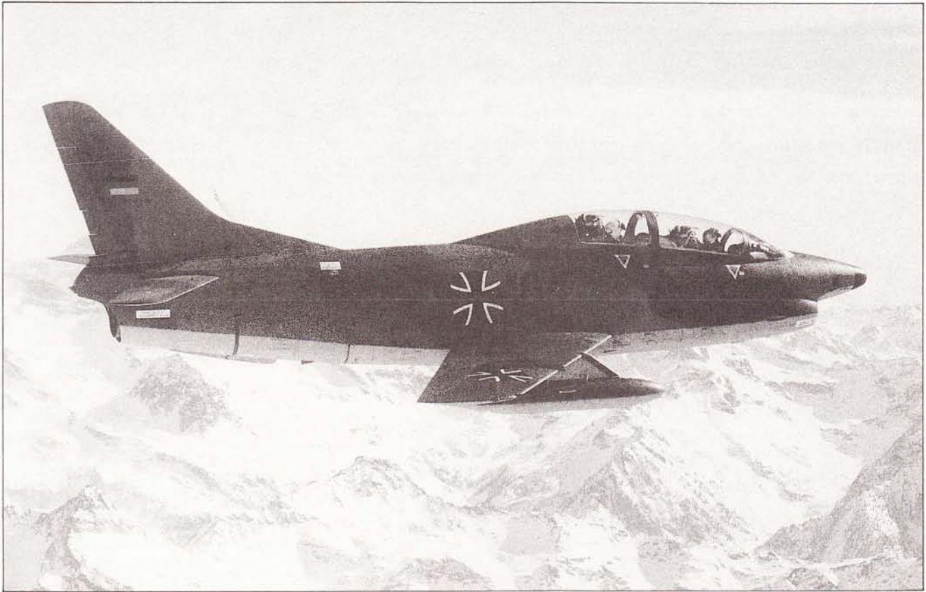
▲ Fiat (now Aeritalia) G91T two-seat trainer in Luftwaffe service. The general similarity of the G91 design to that of the F-86 Sabre was no accident.
