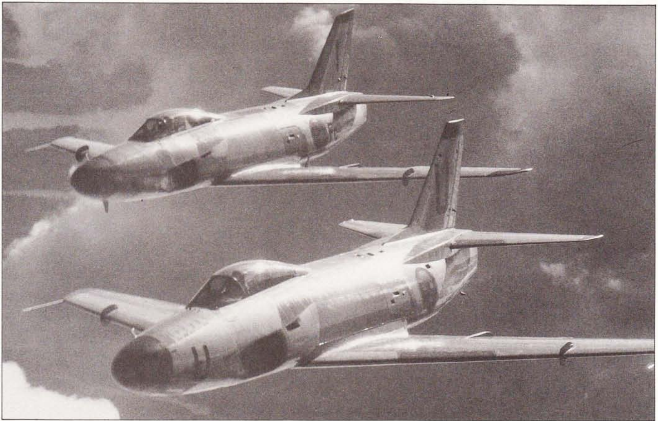
▲ Early Lansens had a rounded tip to the fin leading edge, modified on production aircraft to the square contours seen here. 'Lansen' is Swedish for 'Lance'.
