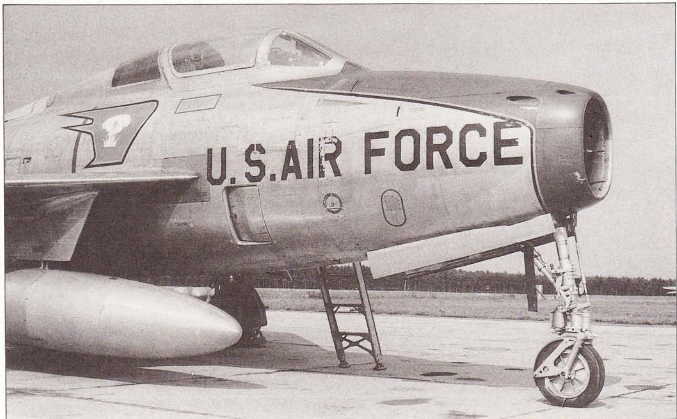
Close-in view of the 'Streak's nose shows complex undercarriage gear and cannon ports above intake.
