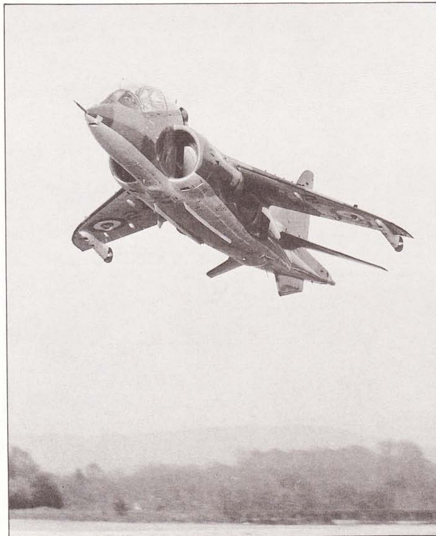
◀ T.2 take-off. Note long 'sting' at tail, to counterbalance the extension of the forward fuselage in the trainer version.
