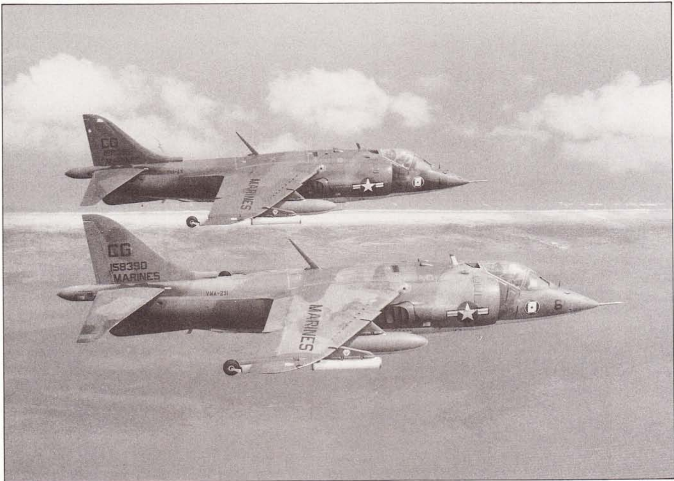
▲ US Marine Corps AV-8As were broadly similar to the GR.1 but, externally, had a prominent dorsal antenna. These two are from VMA-231.
