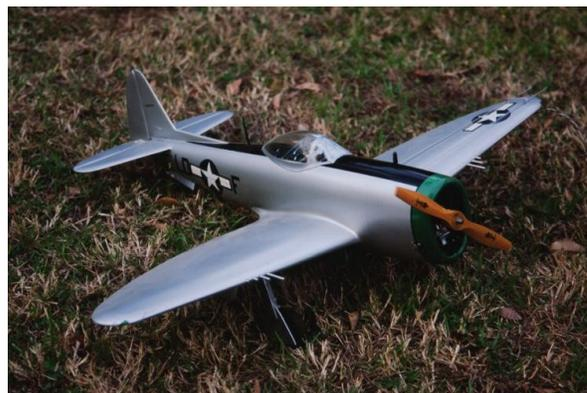
Once you break into the .40 sized model with a wingspan of 50" or more then you get a model with a sufficient amount of wing area to carry some options. Notice the bottom line, wing area. If you look at the electronics, flaps, retracts, bomb drop and the other options we like to install in our models, they are heavy. A 2-ounce servo in a 2-LB model represents 6% of the total model weight. That same 2-ounce servo in a larger model, let's say that weighs 12 lbs represents 1% of the model weight.
