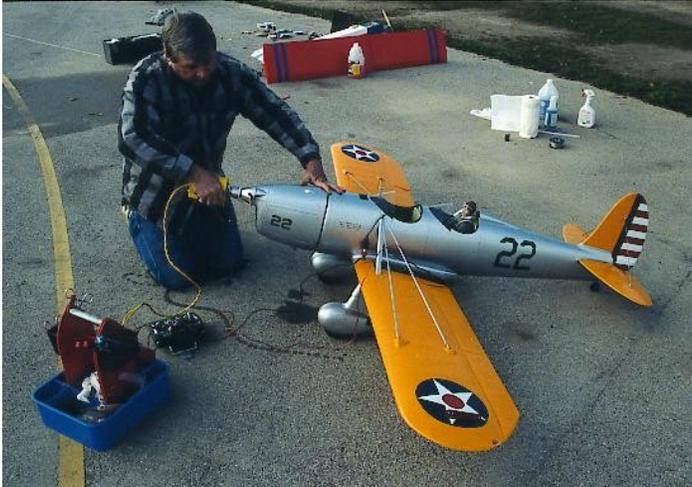
**Photograph 9.2** - Test run motor with handle, transmitter or servo plugged directly into the airplane. The lines have not been rolled out yet. Steve has brakes on this model. For additional safety you should have a friend hold the model while you start and adjust the needle valve.
