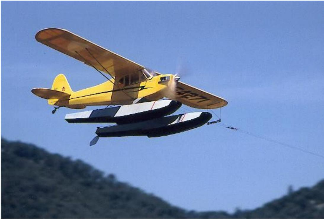
**Plate #18-** Author's Hanger Nine Cub with floats flying from the Roseburg, Oregon float pond. The floats were built from Great Planes float kit (balsa).
