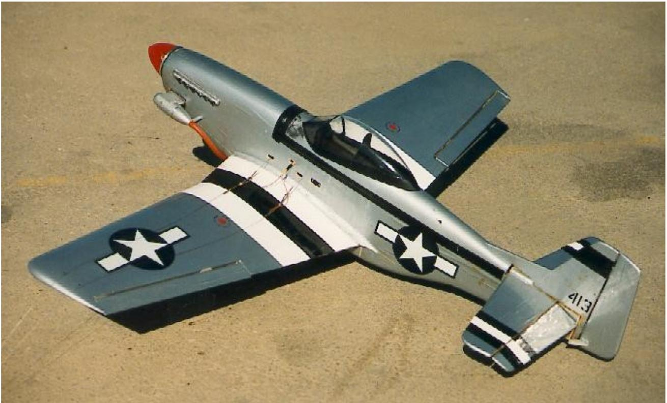
**Plate #13-** This model is not shown for its good looks. This was the prototype used to test the converted ACE radio that became the Multi-Channel electronic controls. The basic system was crude at this point, but proved that it could be done. 48" span, OS-35FP for power. This model weighs 4 lbs in this configuration. The lines used on this model were normal flying lines coated with Clear dope, we later switched to the fishing leader.
