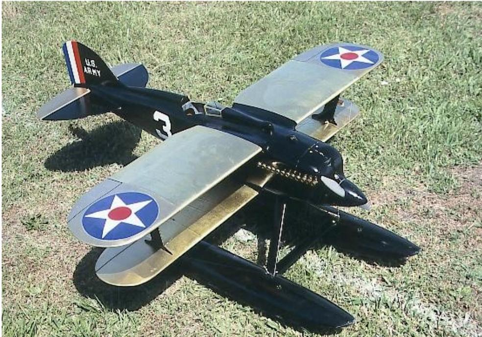
**Plate #15-** Curtiss R3C-2 Seaplane built by Dave Shrum of Roseburg, Oregon. 3-line control for throttle control with an .60 glow engine for power
