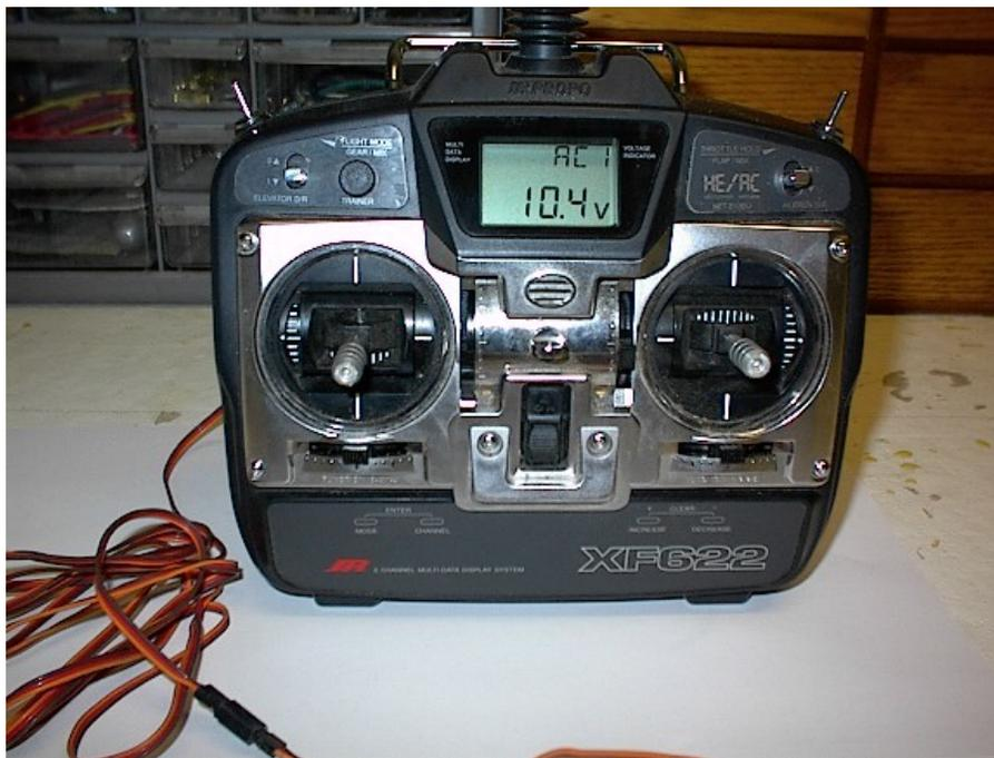
**Photograph 5.11** -Typical JR computer radio with DSC. Toggles on top left and right are great for retractable landing gear, bomb drop. Left stick is used for throttle control. The right stick, which is normally used for elevator on RC models, can be used for flaps if the spring is removed. At the time of printing the XP652 was available.
