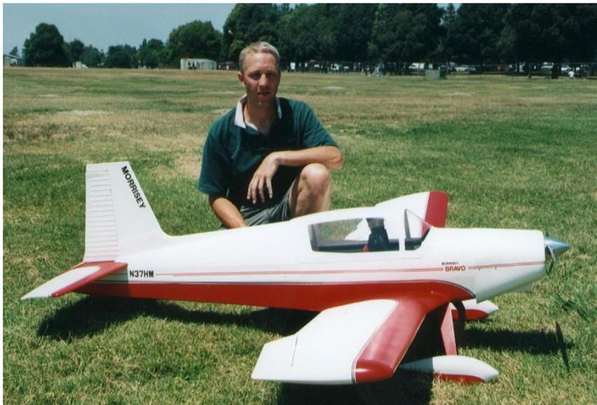
**Photograph 18.1** - Author's 1/4 scale Bravo flown in Sport Scale from the Sig kit. Powered with a Saito .91 four stroke, featured flaps and throttle using a converted Airtronics radio in as described in the Multi-channel chapter. This model weighed 17 lbs and spanned 87"
