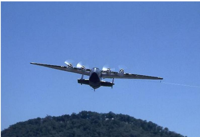
**Plate #14-** Grant Hiestand built this 88" span Boeing 314 Clipper from white foam and covered it with Econokote and then painted it. Powered with four electric motors, this airplane used DSC electronic controls and was flown off of the Roseburg, Oregon float pond in 1999.
