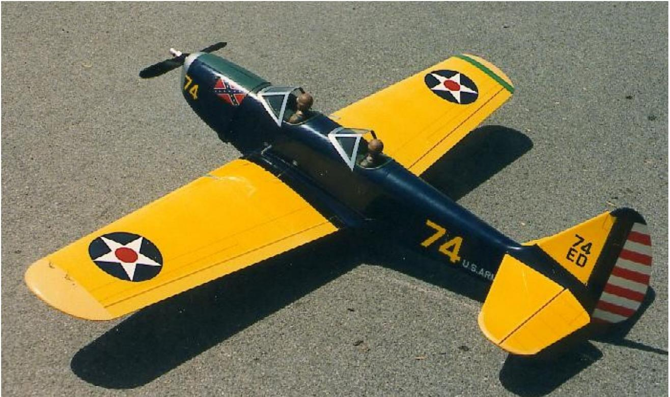
**Plate #11-** This is an ARF model that was used to test the Prototype single channel electronic control system by Fred Cronenwett. 63" span, Fox Eagle 60 for power and this model was a blast to fly. Grant later flew this model for several years with an Astro 40 geared electric motor. A lot of valuable lessons were learned from this model flying it on a daily basis.
