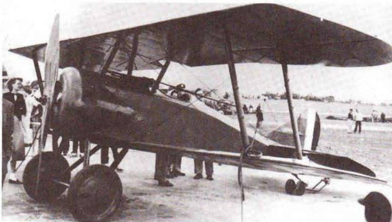
Designed as an advanced single-seat trainer for WW I fighter pilots, over 1,000 "Tommys" were built. This is the S-4B. Photo courtesy of Leonard Opdycke, WW I Aeroplanes.
