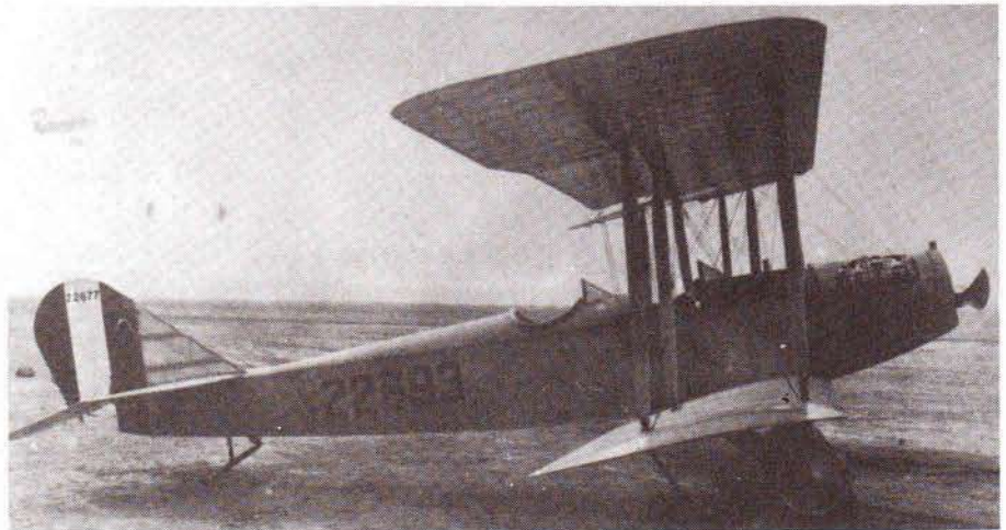
Standard J-1 with Curtiss OX5 engine. Photos courtesy of Leonard Opdycke, WW I Aeroplanes.
