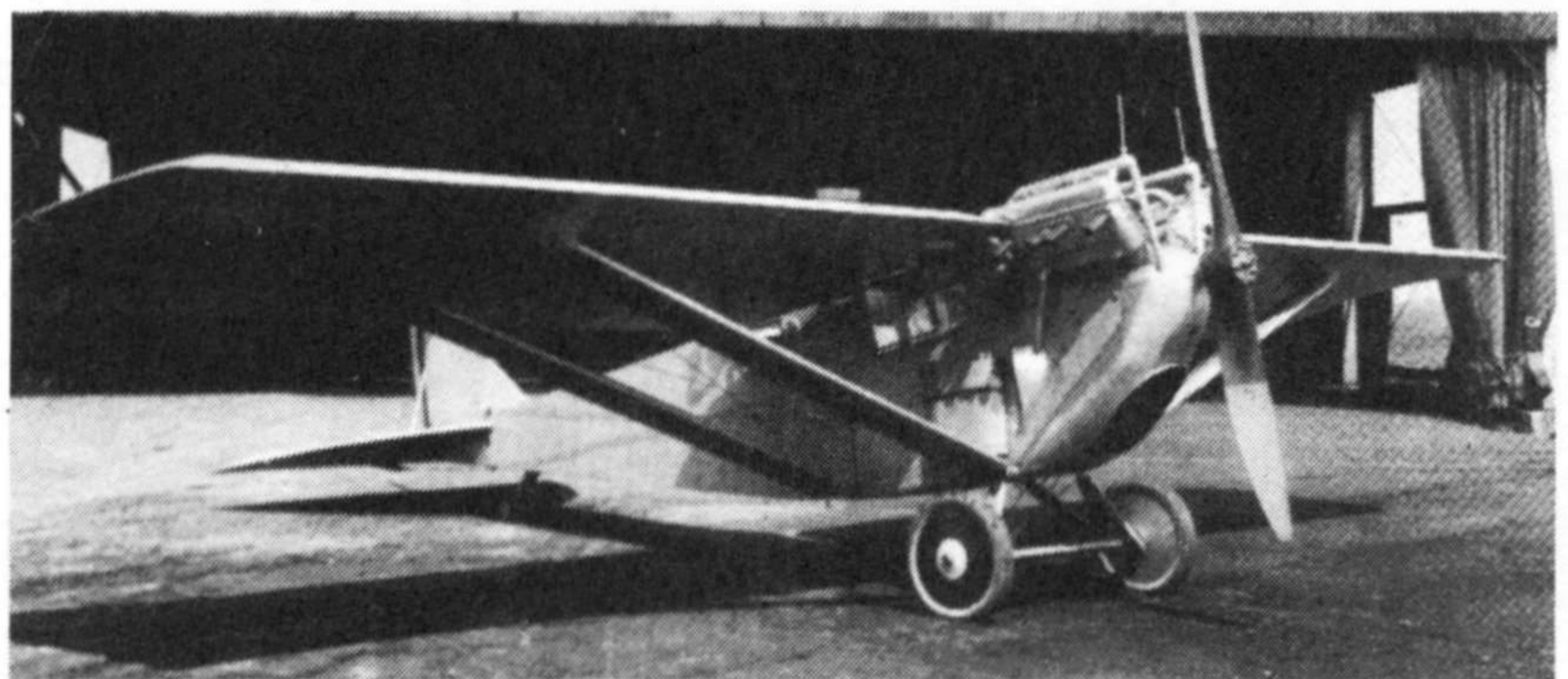
Lifting strut wing braces designed for the M-8 were a breakthrough that has been carried over into lightplane designs of current manufacturing.
