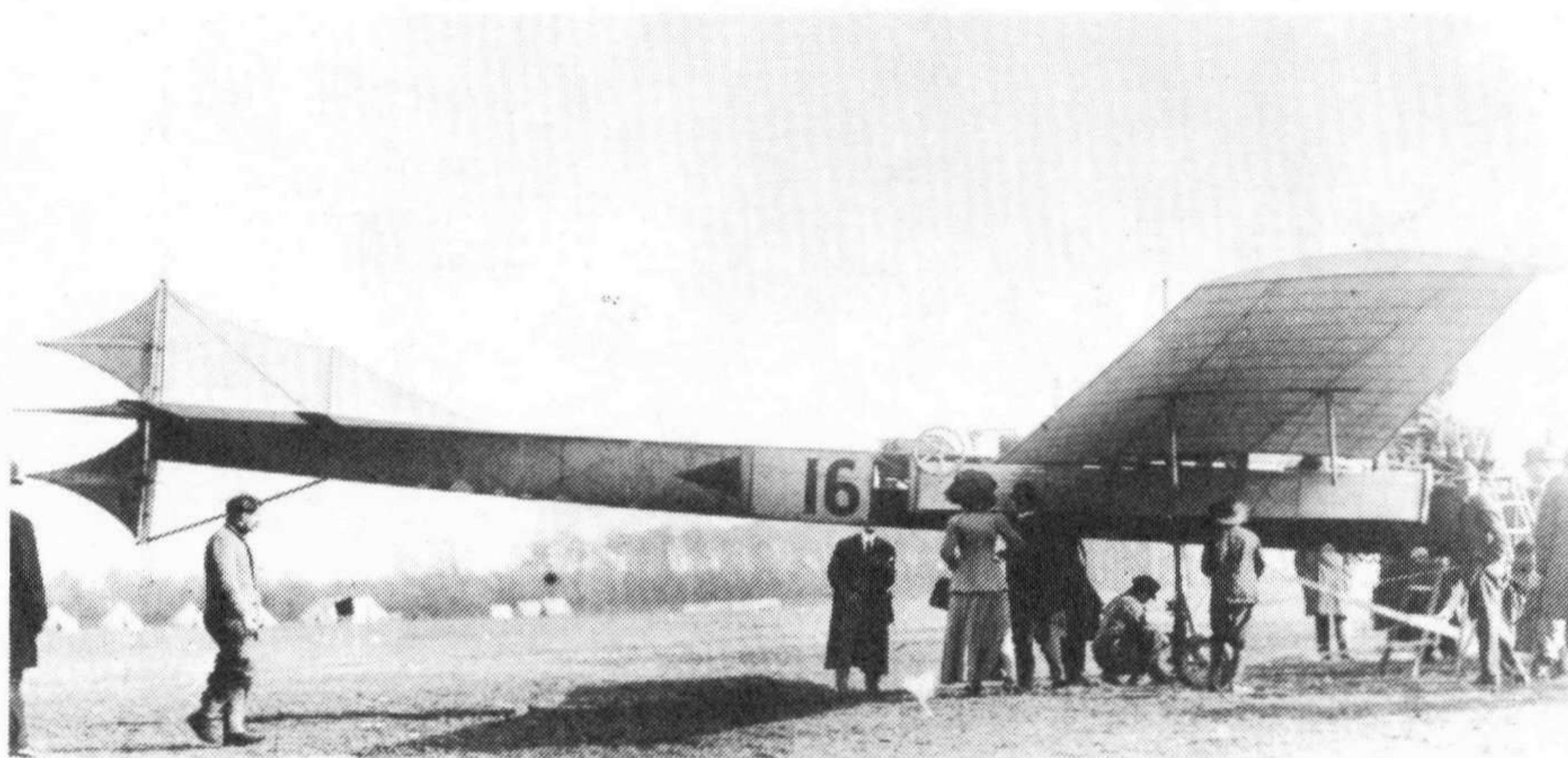
The advancement in aircraft design exhibited here in 1908 was quite revolutionary. Note rudder and elevator control surfaces. The entire wing panels were moved for lateral control. Photos courtesy of Leonard Opdycke, WW I Aeroplanes.
