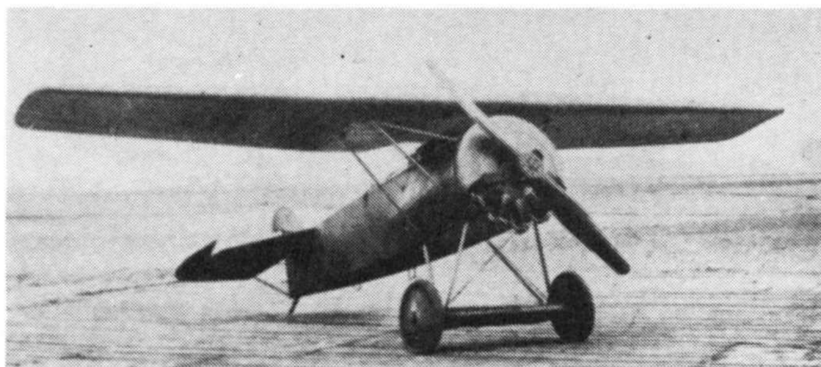
The 110-hp Oberursel rotary, Siemens-Halske, Goebel, and Le Rhone engines were used on various versions of the D.VIII.
