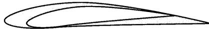
Wash Out Aerofoil at wingtip always has less Angle of Attack then main wing body
