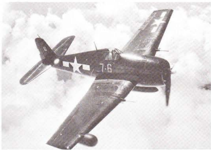
Shown above is an F6F-3 with the short-lived red-bordered insignia and the new (since February 1943) camouflage that used dark blue-gray for top surfaces and graduated to glossy white for undersurfaces. Below: an F6F-5N (with a 20mm cannon and a wing-tip radar pod) that shows off the glossy, overall sea-blue camouflage that was adopted for carrier-based fighters in February 1944 and later expanded to cover most U.S. Navy tactical planes and some support planes.
