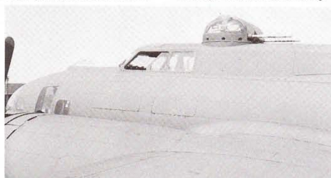
A top-powered gun turret and forward navigator's astrodome were added to the B-17E and retained through subsequent models.
