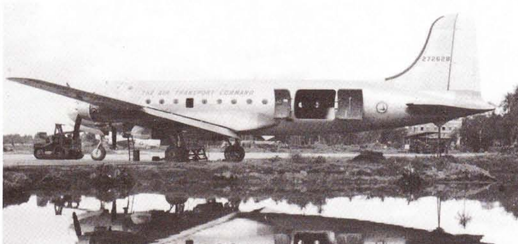
This view of a C-54D shows the large, two-section cargo doors fitted to all C-54s from the C-54A on. Note the Army Air Transport Command insignia on the rear fuselage.
