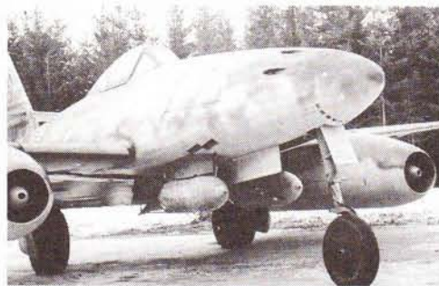
■ Above: Me 262 nose details. At left, an Me 262A-2a with two 250kg (550-pound) bombs under the fuselage. At right, an Me 262A-1a fighter. Note the ports for the 30mm cannon in the upper nose.
