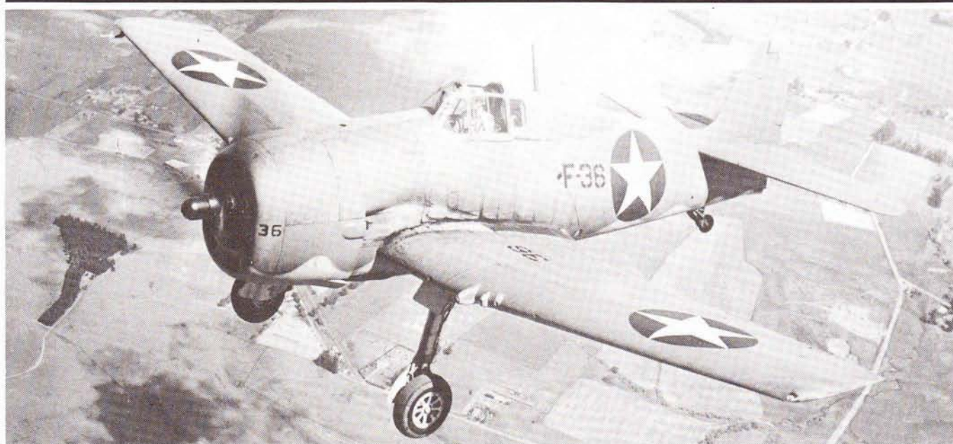
An early production F6F-3 Hellcat with the two-tone gray camouflage that was still used in early 1943. Note the use of stars on both wings and the use of fairings around the muzzles of the six wing guns (later deleted).
