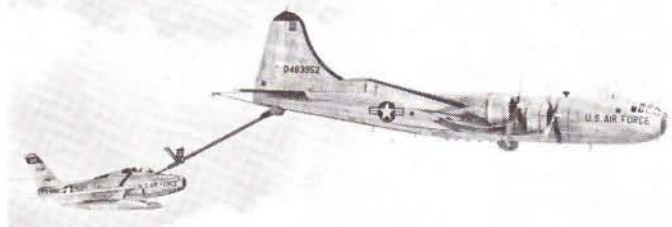
Major postwar use of the B-29 after Korea was as an aerial refueling tanker fitted with Boeing's "flying boom" refueling system. Here, a KB-29P refuels a Republic F-84F.
