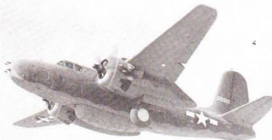
At left: an early Douglas A-20A. Note the DB-7B-type nose, external pack for nose machine guns and use of rudder stripes and two wing stars before the marking change of February 1941. At right: an A-20G-40 with four .50-caliber nose machine guns and a long-range ferry tank under the belly.
