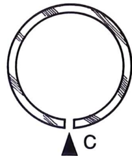
(A) is the Piston Ring in the liner. Use a feeler gauge (B) to measure the Piston Ring gap (C).
