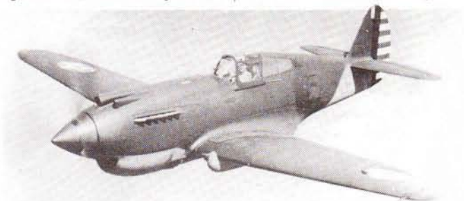
(Figure 1) The early Curtiss P-40 (shown) and Douglas A-20A were the only camouflaged U.S. Army airplanes delivered with the distinctive Army rudder stripes and star insignia on both wing tips. Rudder stripes were eliminated from camouflaged airplanes in February 1942, and the star configuration changed to one on the upper left wing, one on the lower right wing and one on each side of the rear fuselage.
