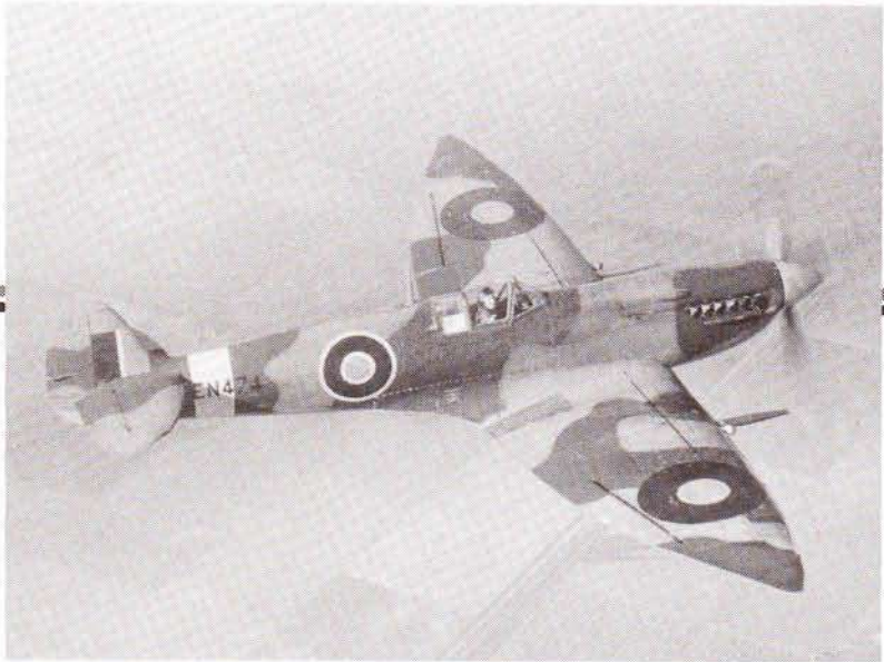
A Spitfire H.F. VII with extended triangular wing tips (above) and a Spitfire VB with clipped wing tips (below).
