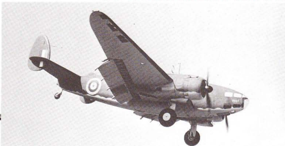
A Hudson V without a turret on a factory test flight in June 1941. Compare the cowling for the Pratt & Whitney engines with those of Wright-powered models in the drawing and other photos. Also note the rearward as well as the downward extension of the Fowler flaps.
