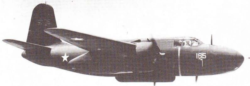
Sixty of the U.S. Army Douglas A-20s were completed as radar-equipped night fighters armed with four 20mm cannon in a belly pack. Note the overall matte-black finish and undersize national insignia.
