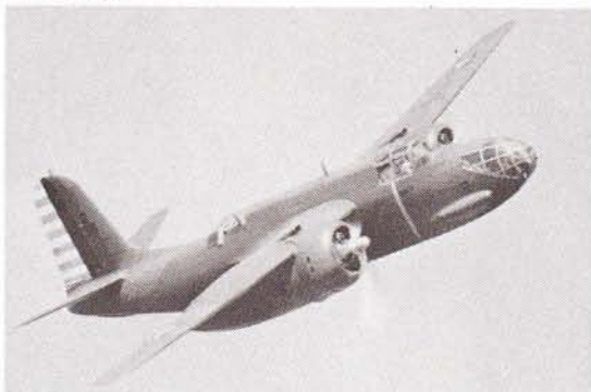
At left: an early Douglas A-20A. Note the DB-7B-type nose, external pack for nose machine guns and use of rudder stripes and two wing stars before the marking change of February 1941. At right: an A-20G-40 with four .50-caliber nose machine guns and a long-range ferry tank under the belly.
