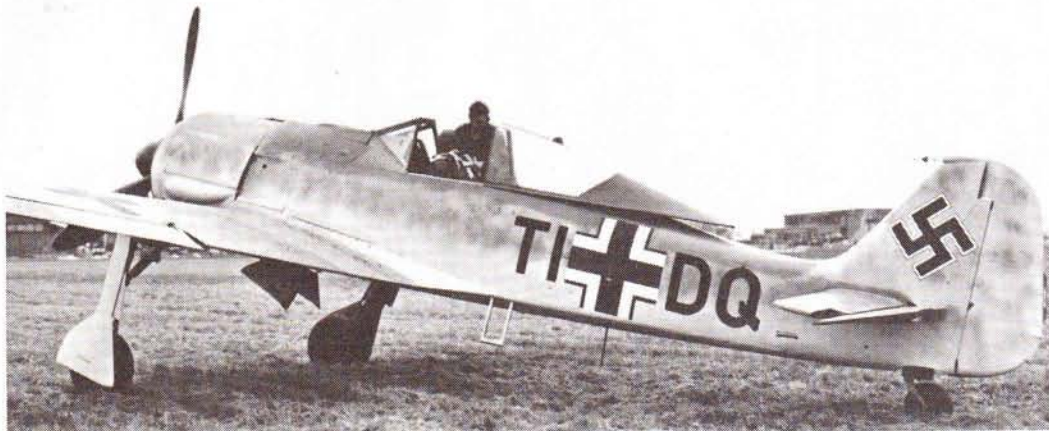
A "factory-fresh" FW-190A-1. Note the distinctive rear-sliding canopy and the wide-track landing gear. The unit markings on the fuselage are black.
