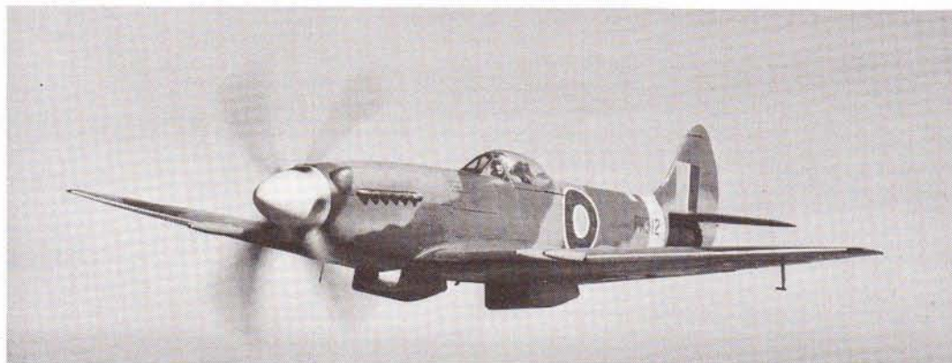
The first Spitfire Mk 22, with a Griffon engine, five-blade propeller, bubble canopy and enlarged tail. Note the bulges in the nose to cover the cylinder banks of the larger engine.
