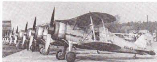
Line-up of nine Gladiator Is in prewar, all-silver finish. Note the large, fixed-pitch wooden propellers, (later replaced with three-blade metal models), and the hinge-down door for cockpit access.
