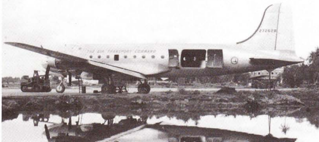
This view of a C-54D shows the large, two-section cargo doors fitted to all C-54s from the C-54A on. Note the Army Air Transport Command insignia on the rear fuselage.
