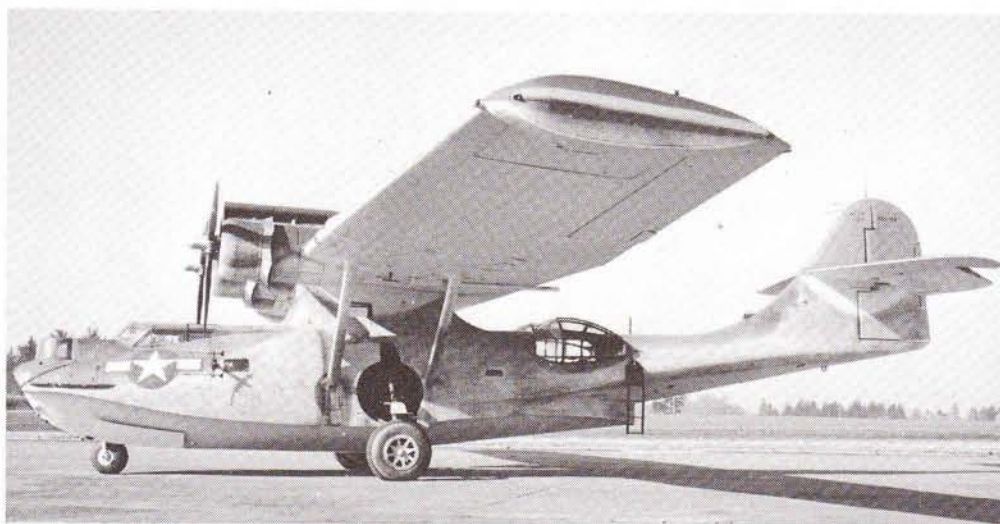
A Consolidated PBY-5A ashore. Note the ram air scoops on the tops of the engines (not shown on drawing) and the hook-on access ladder at the side blister. Sea-blue camouflage on top of the wing is carried around to the bottom of the retracted wing-tip float.
