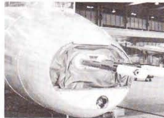
Tail-gunner's station from the B-17E midway through B-17G production. Late Gs had a revised design that was developed at United Air Lines' modification center, site of earlier modifications.
