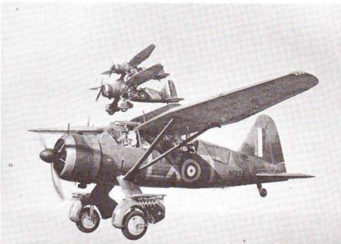
Lysander IIs with stub wings in place on the landing gear; the wheel covers have been removed. Note the far-aft location of the fuselage bomb racks and the early form of the narrow tin flash that was adopted in mid-1940.
