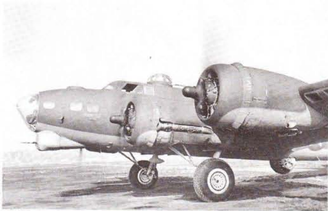
This B-17G-15-BO was delivered without the additional nose guns that were added to early B-17Gs at modification centers. Note that the exhausts for inboard engines are on the outer sides of nacelles; exhausts on the outboard engines are on the bottoms of nacelles. Also note the camouflage pattern on engine cowlings.
