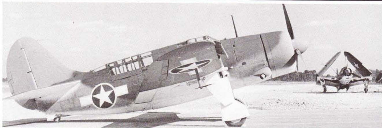
An SB2C-1C with its retractable, leading-edge wing-slats open. Note the short-lived red border around the insignia as used in July/August 1942, and the use of topside camouflage on the outer (folding) panels of the wing. The plane in the background has folded wings and open bomb-bay doors.
