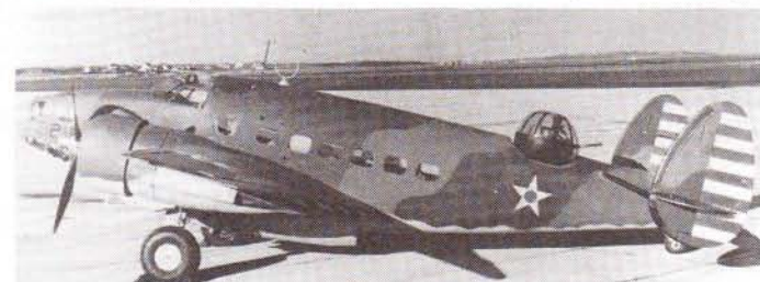
This U.S. Navy PBO-1, formerly a Hudson IIIA, carries early 1942 Navy markings, is fitted with the British Boulton & Paul gun turret and retains its original British "Sand and Spinach" camouflage.
