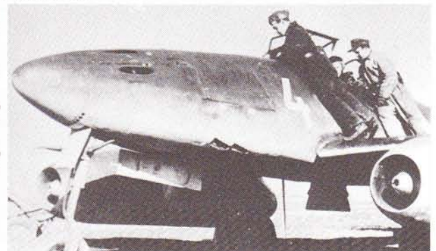
Me 262 nose details. At left, an Me 262A-2a with two 250kg (550-pound) bombs under the fuselage. At right, an Me 262A-1a fighter. Note the ports for the 30mm cannon in the upper nose.
