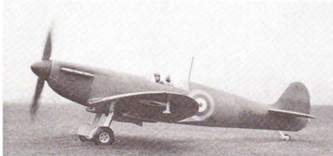
An early Spitfire I with a fixed-pitch wooden propeller and a straight top canopy. Note the Type A roundel under the wing and the Type A.1 roundel on the fuselage.
