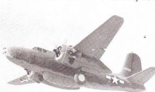
At left: an early Douglas A-20A. Note the DB-7B-type nose, external pack for nose machine guns and use of rudder stripes and two wing stars before the marking change of February 1941. At right: an A-20G-40 with four .50-caliber nose machine guns and a long-range ferry tank under the belly.
