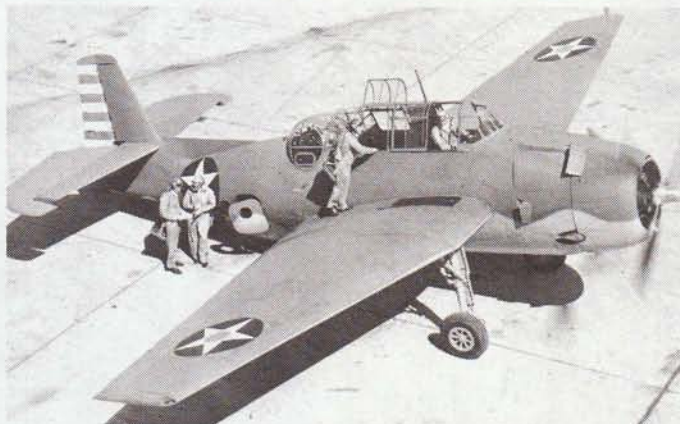
A Grumman TBF-1 with two-tone camouflage and the Navy rudder stripes used only from January 4, 1942, through May 15, 1942.
