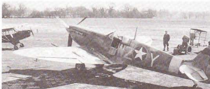
A Spitfire Mk VB of the 309th Fighter Squadron, 31st Fighter Group, with U.S. insignia. Note the bulge on the wing over the cannon breech and the hinge-down door necessary for pilot access to the narrow cockpit.
