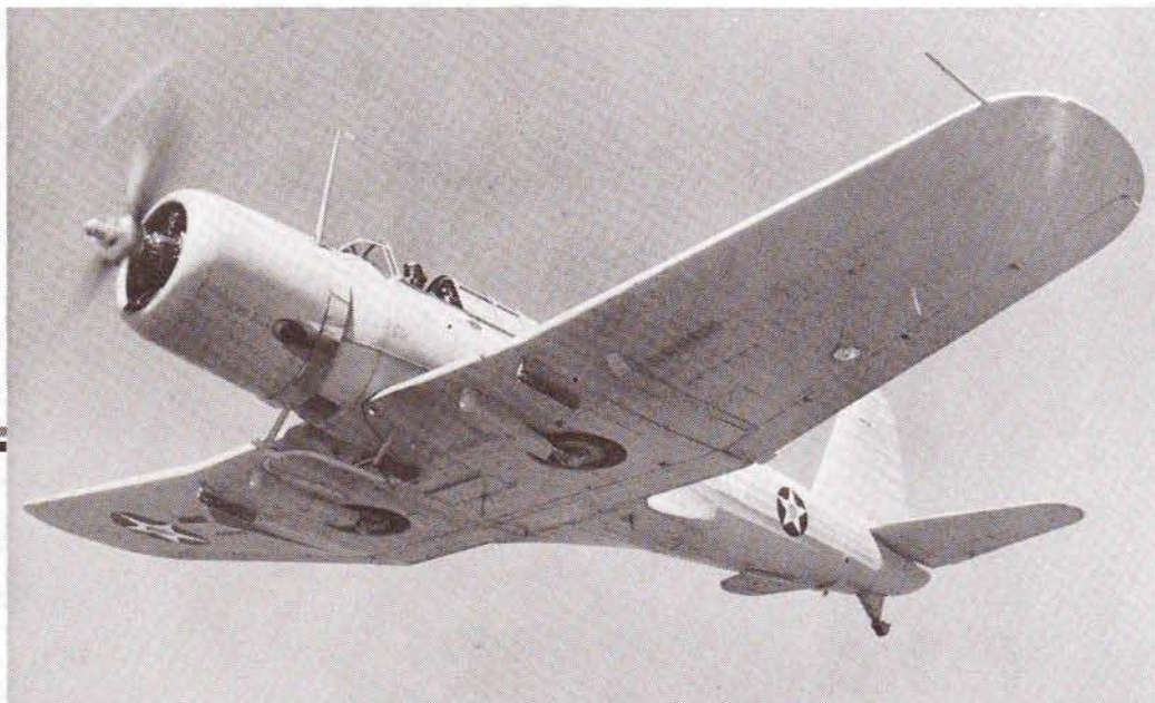
This underside view of the SB2U-3 1-S-16 shows the retracted landing gear and racks for 100-pound bombs. Note the star on the lower right wing.
