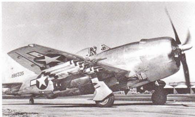
This is the final "Jug" model, the P-47N, with a lengthened and square-tipped wing. This plane is in fighter-bomber configuration, with two 1,000-pound bombs and 10 rockets.
