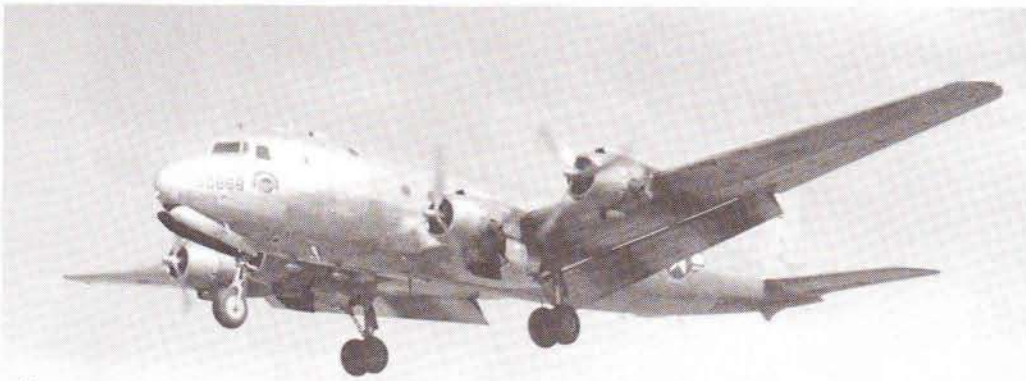
This U.S. Navy R5D-2 was originally a C-54B built for the Army. Note the large, single-wing, trailing-edge flaps and the application of a U.S. Navy serial number and Naval Air Transport Service insignia to the nose.
