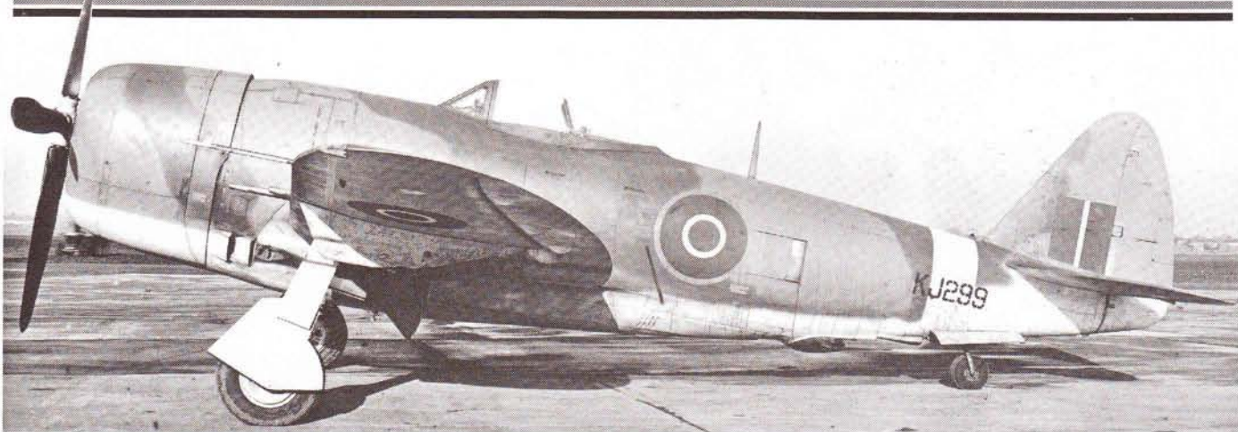
A Republic P-47D-25 in service with the Royal Air Force as "Thunderbolt II." The streamlined shape under the wing is a rack for either a drop tank or a 500- or 1,000-pound bomb. Note the absence of a dorsal fin.
