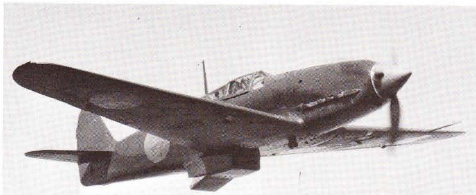
A flight view of a Kawasaki Ki 61-I Tony that was captured by the Allies and tested after being repainted with non-standard coloring. The restored Japanese insignia was used for publicity purposes. Note the extremely clean design and radiator installation similar to the North American P-51.
