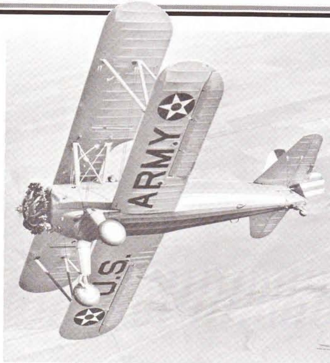
A Stearman PT-13A banked over to reveal the underside detail. The U.S. Army lettering is 24 inches high; the star insignia is 30 inches in diameter under the wing and 42 inches above.
