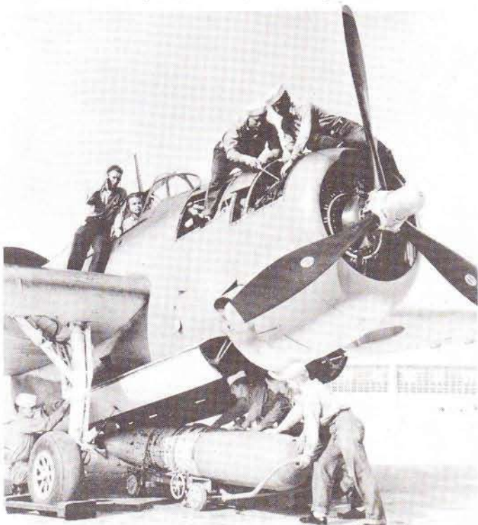
In a typical WW II publicity photo, Navy crewmen load a torpedo into the bomb bay of a TBM-1.
