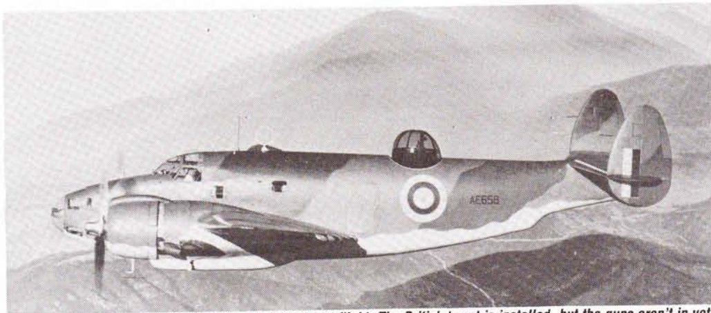
The first Ventura I ordered by Britain on a factory test flight. The British turret is installed, but the guns aren't in yet. Note the step-up forward of the tail for the ventral gunner's station.
