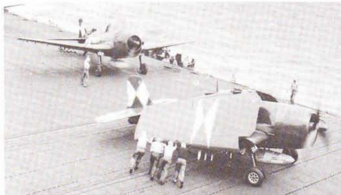
F6F-3s on the deck of the USS Essex in April 1945. Note the belly tanks and underwing rockets on both airplanes, and the deck crew manually folding one plane's wing (center). The various white markings shown here were adopted in late 1943 to identify airplanes from different aircraft carriers.
