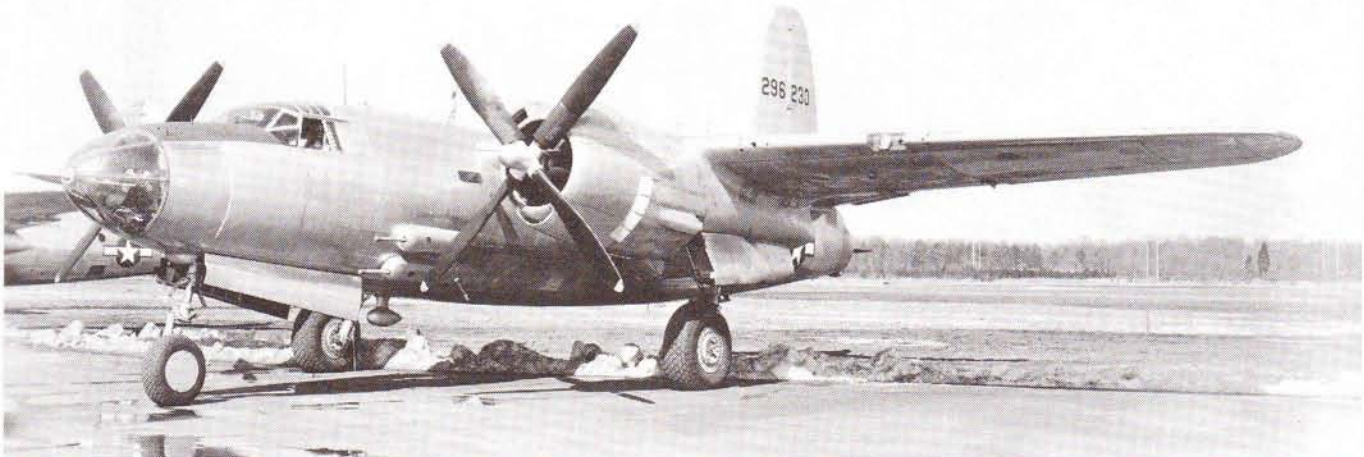
A B-26F-1-MA in the natural metal finish adopted for most U.S. Army combat planes early in 1944. Note the external "package guns" on the lower fuselage.
