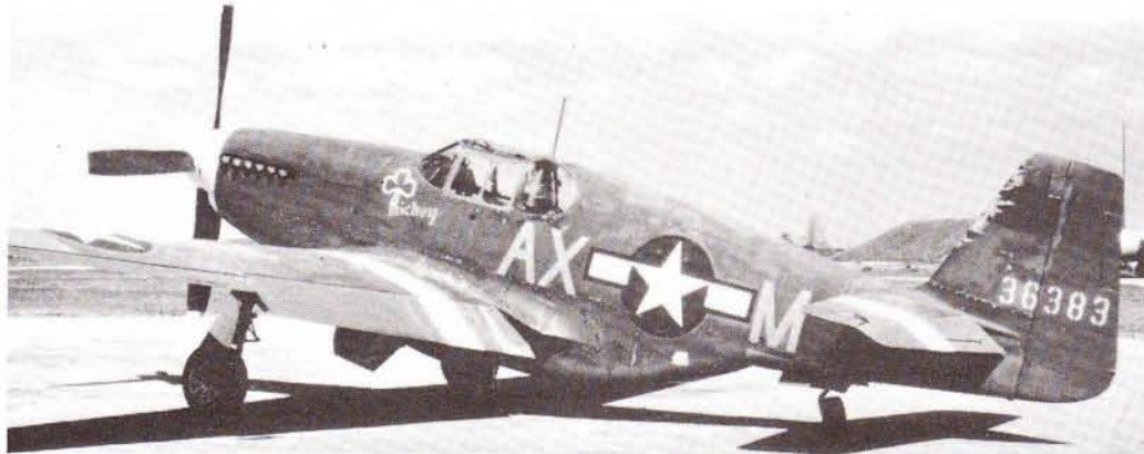
A camouflaged P-51B-5-NA Mustang, photographed with the Ninth Air Force in England. The letters "AX" identify the 12th Squadron of the 67th Reconnaissance Group, identified by the letter "M."
