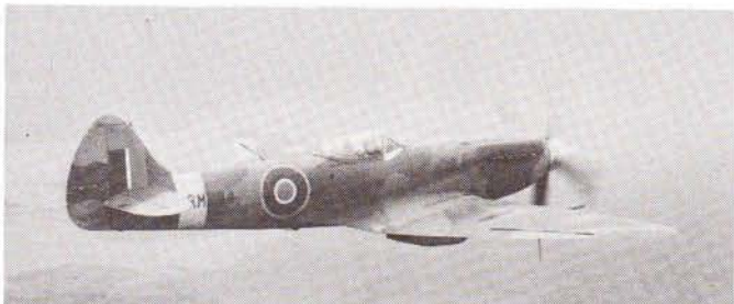
A Spitfire F.Mk XIV with a Rolls-Royce Griffon engine, four-blade propeller, cut-down rear fuselage with bubble canopy, and an enlarged vertical tail.
