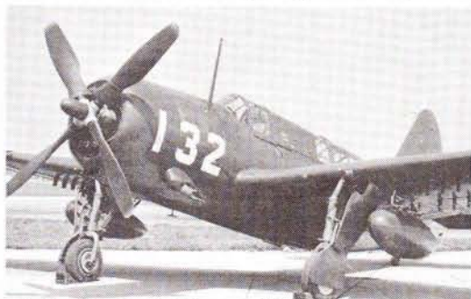
The final Curtiss Helldiver model—the SB2C-5. Note the four-blade propeller, the 100-gallon drop tanks on wing bomb racks, the mounts for 5-inch rockets and the overall midnight-blue finish adopted for carrier-based airplanes early in 1944.
