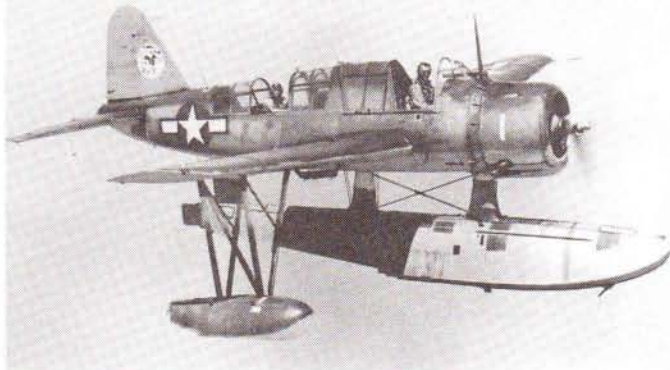
A Vought OS2U-3 Kingfisher seaplane, with 1943-44 dark blue-gray camouflage on the upper surfaces graduating to white undersides. The hook under the float was used to snag a retrieval net before the seaplane was hoisted aboard the mother ship.
