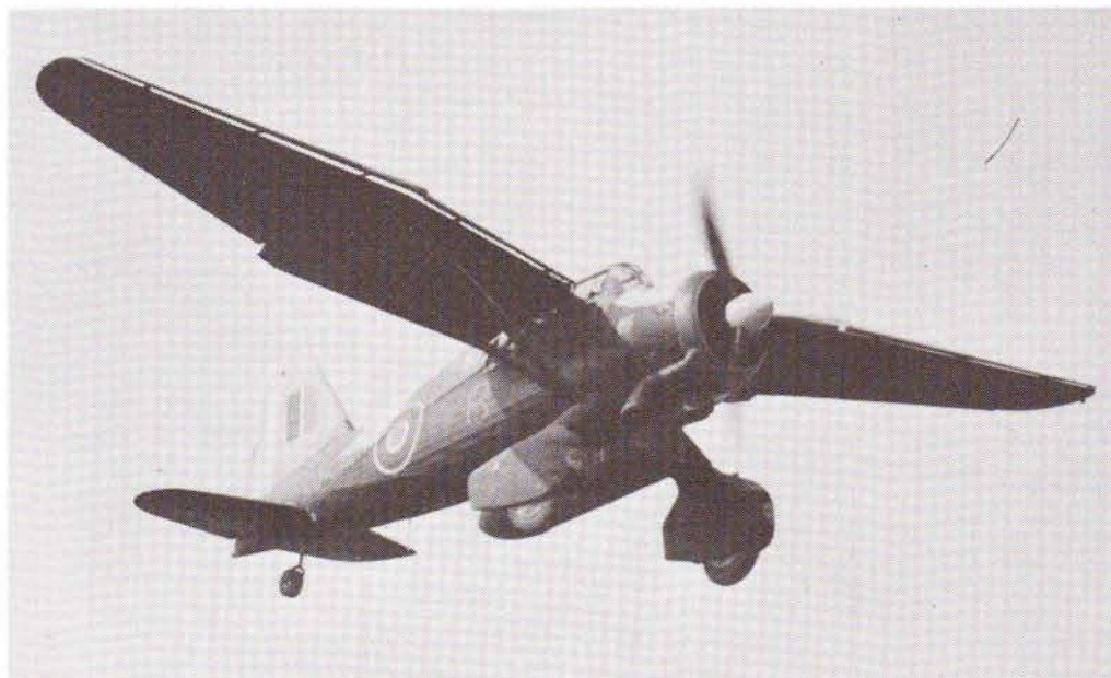
This view of a Lysander III with a belly-mounted auxiliary fuel tank shows the full-span wing slats open during a landing approach.
