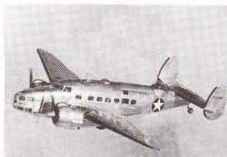
A U.S. Army AT-18 gunnery trainer with a molded Plexiglas Martin gun turret. The rubber de-icer boots on the wings and tail are prominent on this unpainted airplane.
