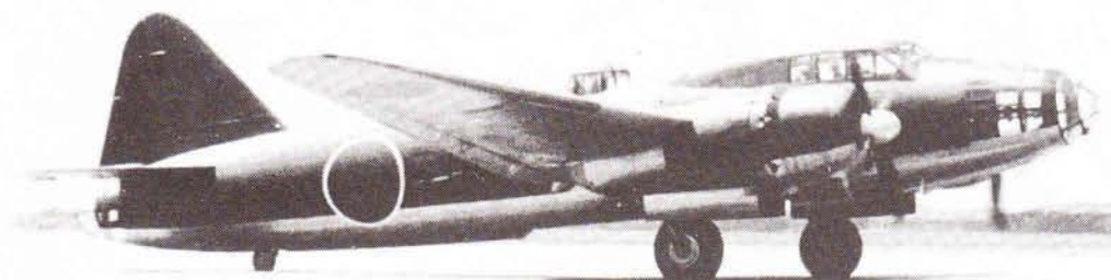
This view of the Mitsubishi G4M-2 Betty bomber shows the powered upper turret and four-blade propellers added to this model. The color is dark green on the upper surfaces and silvery gray underneath.
