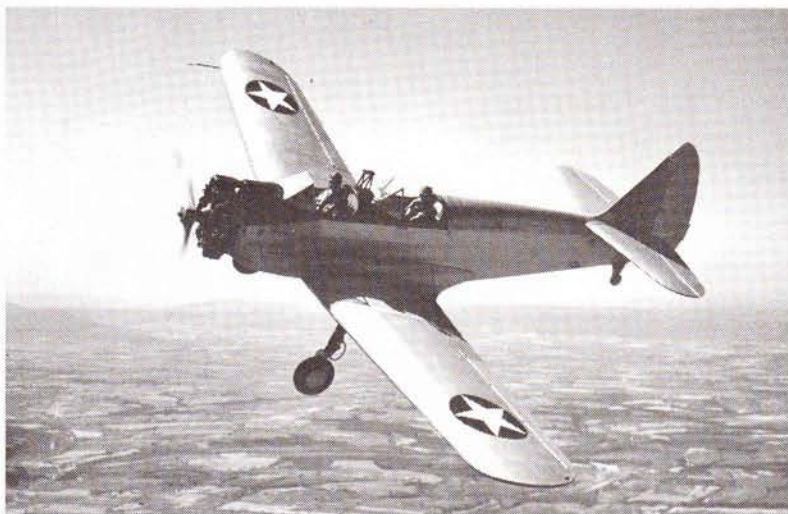
A silver Fairchild-built PT-23 with 220hp Continental Radial engine and 1942-43 star markings.
