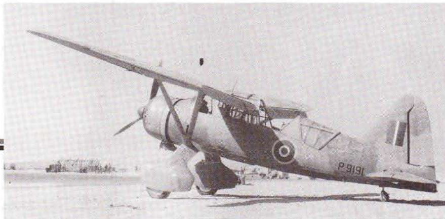
Side view of the Lysander II. Note how the rear portion of the cabin enclosure slides straight aft.
