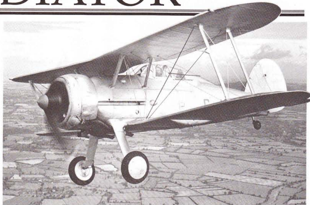
This restored Gladiator I has the postwar British civil registration G-AMRK. The prewar R.A.F. serial number was L8032. Note the absence of guns from fuselage troughs and underwing pods.
