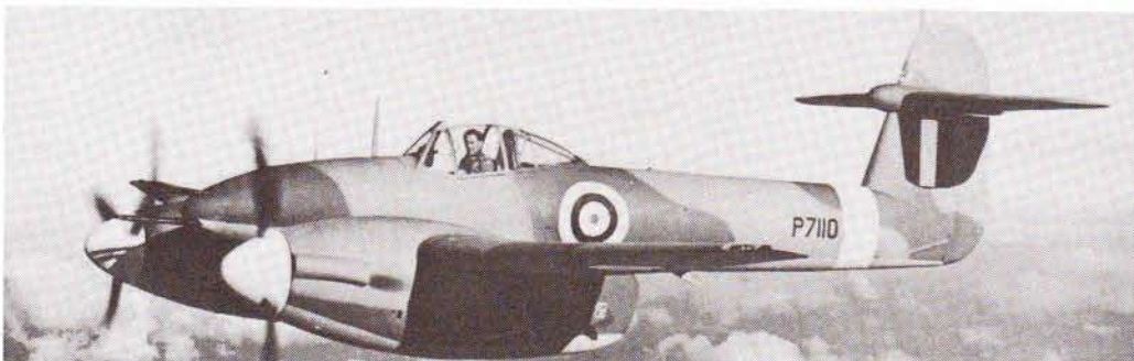
Only 12 Westland Whirlwinds were built after this P7110. Note the four-cannon armament and the "bullet" at the fin-stabilizer intersection that wasn't on the two prototypes.
