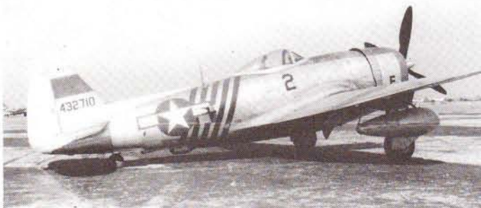
This P-47D-30 with a dorsal fin and 150-gallon drop tanks has the dark blue stripes of the First Air Commando Group, which was based in Southeast Asia in 1944-45.
