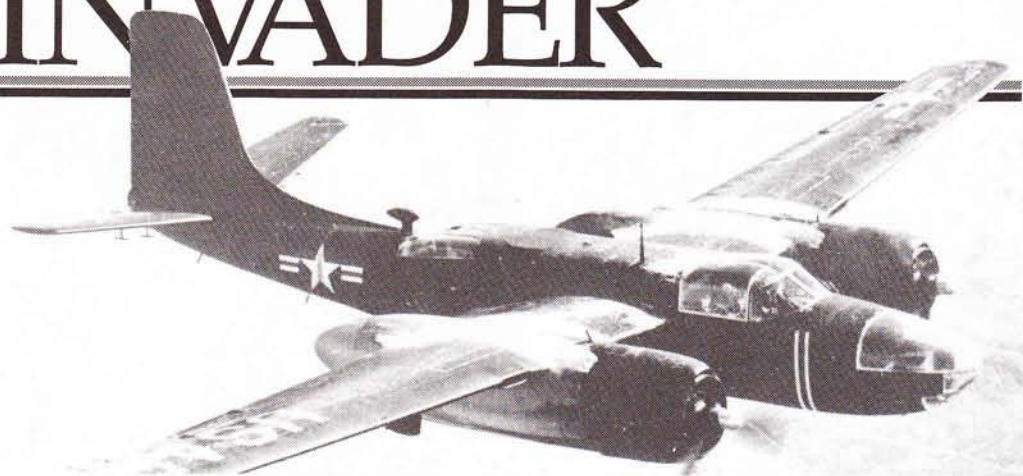
Close-up of a black-painted A-26C shows the molded Plexiglas bomber nose and the bulged pilots' canopy adopted after early A-26 combat experience.
