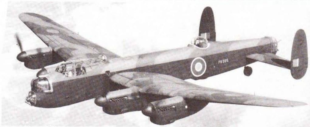
An Avro Lancaster I carrying standard British night-bomber camouflage. Note how far up the side of the fuselage the matte-black underside paint extends. Type B roundels are on top of the wing; Type C.1 roundels are on the fuselage. The fin flash is 24x36 inches.
