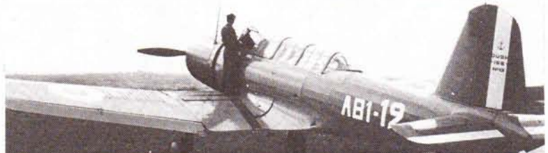
A Vought V-156F of the French Navy. Note the red, white and blue stripes on the elevators and the rudder, and the dive brakes on the wing (a feature not used on the U.S. Navy/Marine SB2Us).
