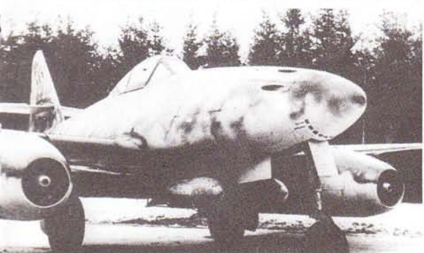
Me 262 nose details. At left, an Me 262A-2a with two 250kg (550-pound) bombs under the fuselage. At right, an Me 262A-1a fighter. Note the ports for the 30mm cannon in the upper nose.
