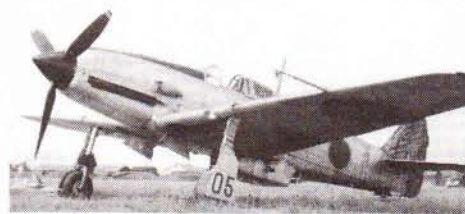
This ground view of a Ki 61-I shows the wide-track landing gear and basic natural-metal finish. Various camouflage patterns were often applied in the field.
