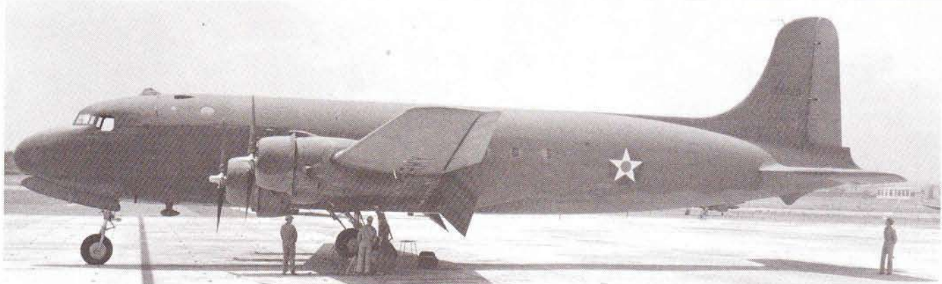
The third Douglas DC-4 was built as an airliner but was delivered to the U.S. Army in war paint as a C-54.
