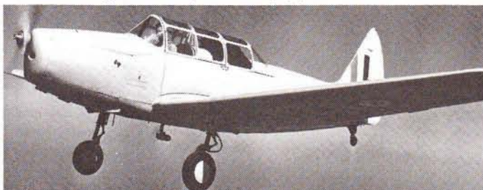
Above: The first Fairchild-built PT-26 was a winterized PT-19A with enclosed cockpits. This airplane carried Royal Air Force serial number FH651 and U.S. Army serial number 42-12499. The R.A.F. designation was Cornell I. Roundels and fin flash are correct for the 1940 to mid-1941 period.
