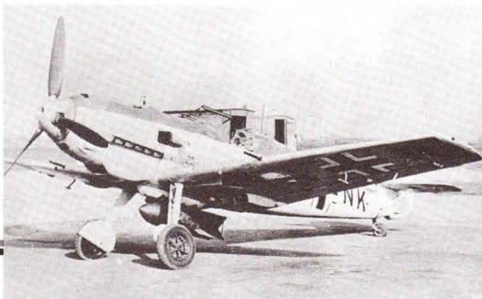
An Me 109E-4/B, in 1940 coloring, carrying a 550-pound bomb. Note the wide white borders on the fuselage and the underwing crosses, and the wing crosses now located farther from the wing tip.
