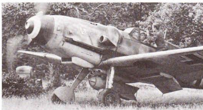
The Me 109G was outwardly similar to the F model, except for the bulges for larger nose-gun ammunition drums located ahead of the cockpit (which started with the G-3). Shown here is an ME 109G-10/R1.
