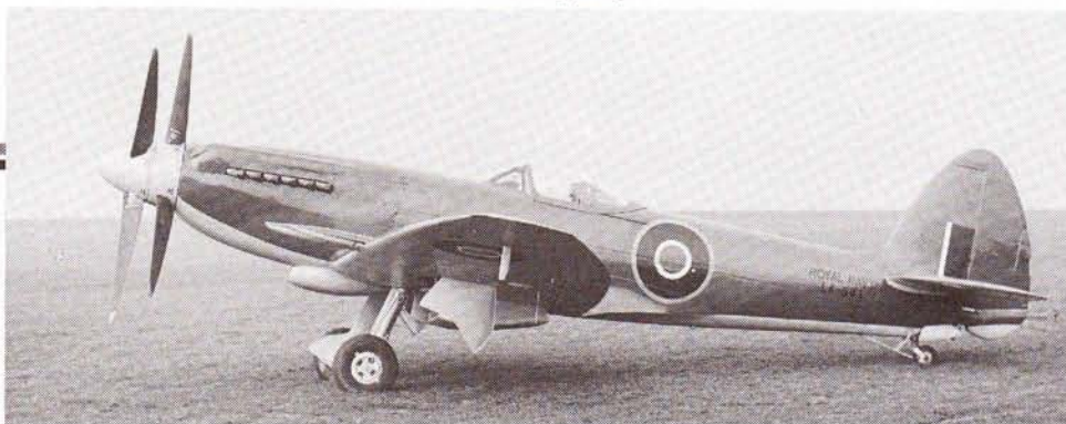
The final variant of the Spitfire line: the Seafire Mk 46 with contra-rotating propellers. Note the extension of the rudder carried by the stinger-type arrestor hook. The later Mk 47 was very similar, except for its greater fuel capacity and folding wings.
