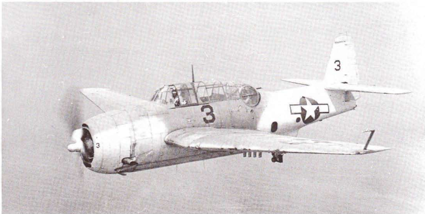
A TBM-3 with the white and gray camouflage adopted in June 1944 for anti-submarine patrol missions. Note the underwing posts for rockets and the camera outboard of the rocket mounts.
