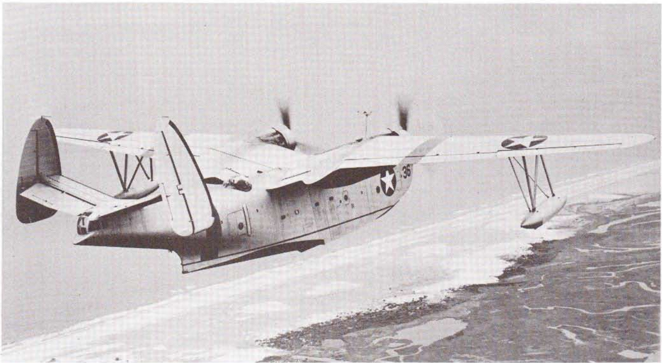
This PBM-3 with prewar silver coloring was photographed in late 1942 or early 1943. Note the unpowered tail machine-gun turret and flush panels for side gun stations. The red bands on the wings and hull (later changed to green) identify an instrument trainer.
