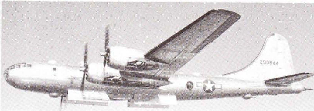
A Boeing B-29A-5-BN in flight with both sets of bomb-bay doors open. Note the four powered, remote-control gun turrets above and below the fuselage, and the 20mm cannon supplementing two .50-caliber machine guns in the tail turret.
