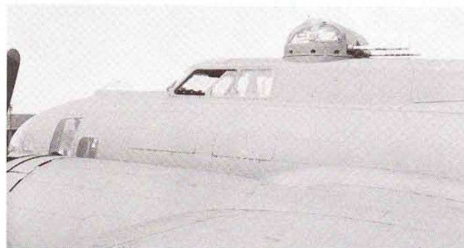
A top-powered gun turret and forward navigator's astrodome were added to the B-17E and retained through subsequent models.
