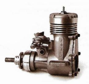
Double ball bearing, chrome brass cylinder liner, aluminum piston, makes this a durable, powerful motor. Schnuerle ported, and new EZ Single Needle carburetor. Comes with polished spinner nut.
