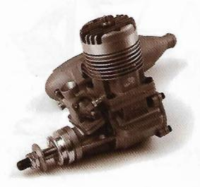
Double ball bearing, schnuerle ported, the Eagle 4 is offered with either a conventional ring type piston and cylinder, or with an ABC cylinder and piston. Cylinder casting can be turned to side or rear exhaust. Equipped with new EZ Single Needle carburetor.
