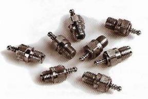
World famous with space age technology. Short reach fits most 15 size motors. Long reach fits most others. Standard plug is for control line use. Idle bar and Miracle plug for R/C use. Miracle plug also works extremely well in 4 cycle motors, and retains heat better than all other types. 2-volt plugs are mainly for lead acid battery use. All other plugs are 1.5 volts. Thread is 1/4-32.
