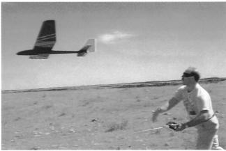
Fig. 6-6. This is the correct method for launching your sailplane. Firmly throw it straight ahead (or a little downward) to pick up enough speed to fly. Next fly straight out into the lift and begin performing Figure 8s.
