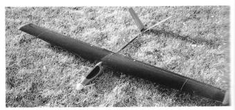
Fig. 11-9. The Impulse by Jarel Aircraft Designs. This is a highperformance electric sailplane suitable for beginners.
