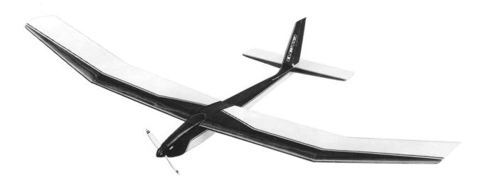
Fig. 11-1. The Electra. This model by Carl Goldberg Models is basically an electric-powered Gentle Lady. The deluxe kit comes complete with an electric motor and power harness.
