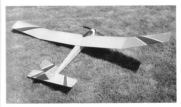
Fig. 7-1. This is the Goldberg Electra, which is basically an electric-powered Gentle Lady. It is stable and performs well in thermals.
