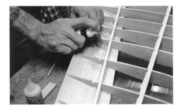
Fig. 12-7. The proper use of CA glues. First apply the thick CA glue to the wood surface. Next, position the part in its proper place. Then, spray the area with the accelerator and the glue will quickly cure.
