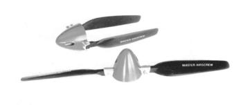
Fig. 8-14. These folding propellers are made by Master Airscrew. On the bottom propeller the blades extend while the motor is running. When the motor is turned off, the blades freely fold back (above), reducing the overall drag on the sailplane.
