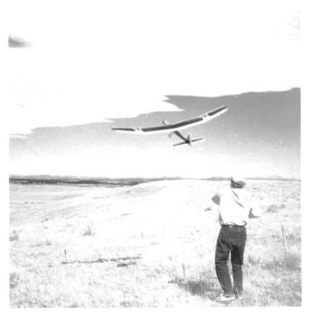
Fig. 6-8. You can use a short hi start at a slope. The tie down spot is just over the edge of the hill. This technique is useful when you are not sure if there is enough wind to keep your plane aloft.
