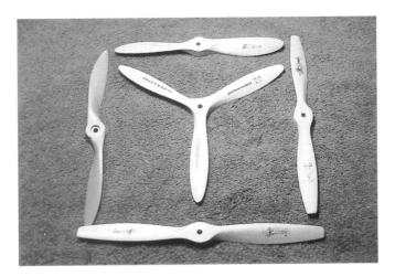
Fig. 8-13. Many rigid-fixed propellers are available to modelers. These include wood as well as nylon types that come in two-, three-, and four-blade versions.
