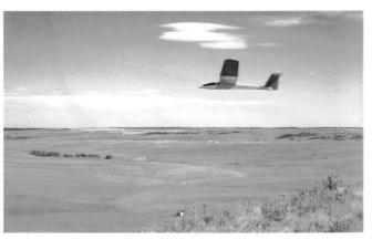
Fig. 6-11. If your approach is too high, as in these photos, fly straight ahead over the top of the slope into the lift. After climbing to 50 feet, make another attempt to land.
