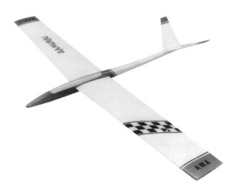
Fig. 6-21. Samurai. This sleek and highly aerobatic ship is as exciting as it looks. Its controls are novel and the wing panels are made to move independently for control.
