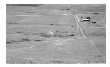
Fig. 6-14. This sailplane has descended below the top of the hill because the wind slowed down. It was successfully landed using the technique in fig. 6-13.
