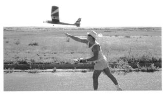
Fig. 13-2. The first few launches should be performed using a helper. With experience, you will be able to launch your plane by yourself. After the motor and radio checks out, start your motor, and then firmly throw your plane into the wind with the wings level.
