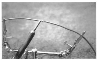
Fig. 8-10. Now take the two pre-tinned ends, overlap them, and heat them with the iron. The solder on the ends will melt and flow together. When it cools, a very strong shiny bond should result.
