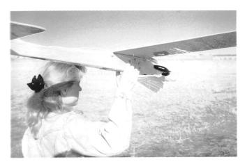
Fig. 13-5. Electric sailplanes can be easily launched using a histart. If one is already available such as at a soaring club, use this method to save battery power for extended flights.
