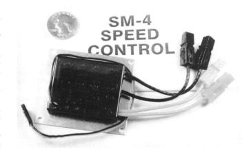
Fig. 9-14. This SM-4 Speed control by Jomar can be used with motors ranging from 05 to 40 in size. Full proportional throttle control is possible with this unit. Battery cell packs of seven to 21 can be used safely with this control.
