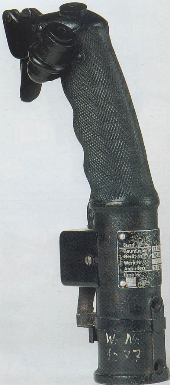
Port side view of Bauart made KG 13B control column.
