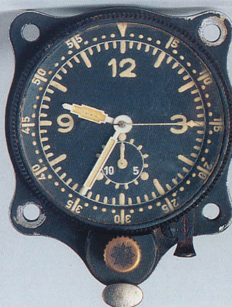
Chronometer fitted with stop watch button.
