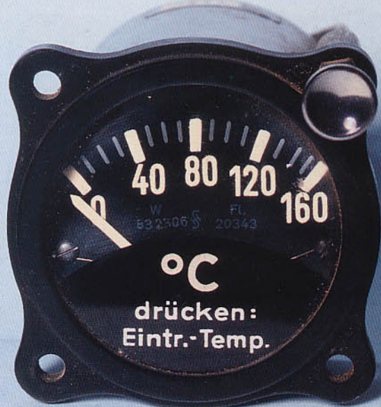
Supercharger outside air intake temperature, Siemens.
