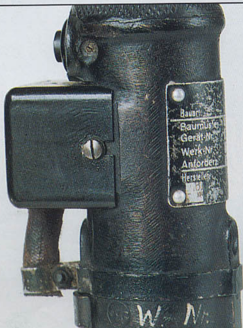
Close-up of KG 13B base showing electrical connection.
