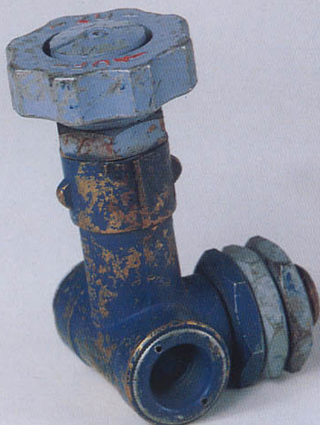
Oxygen flow remote control valve. Note color coding.
