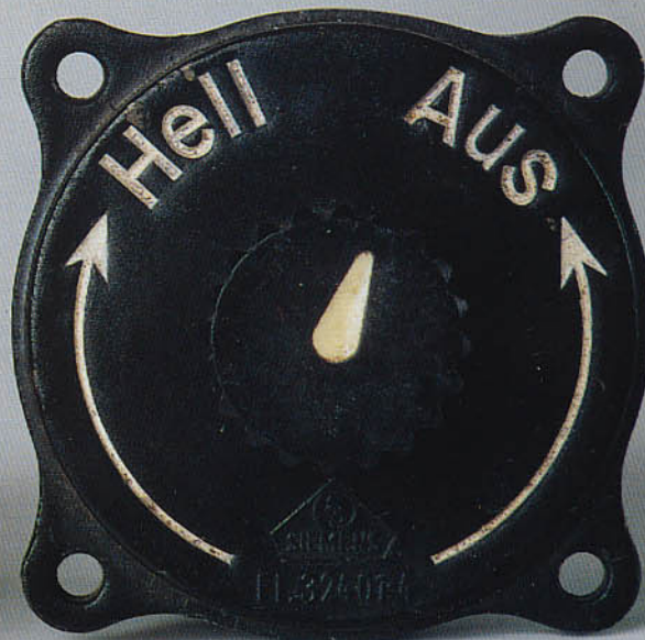
Dimmer control made by Siemens.
