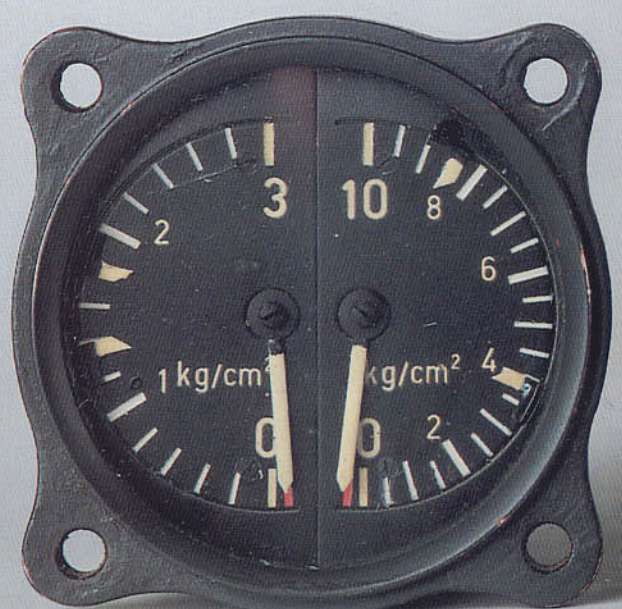
Dual fuel and oil pressure gauge.
