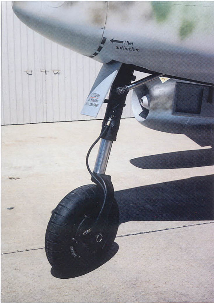
Left, lower left and bottom: Three views of the Me 262's undercarriage. Note that on this aircraft (NASM), the nosewheel compression leg lacks torque scissors.
