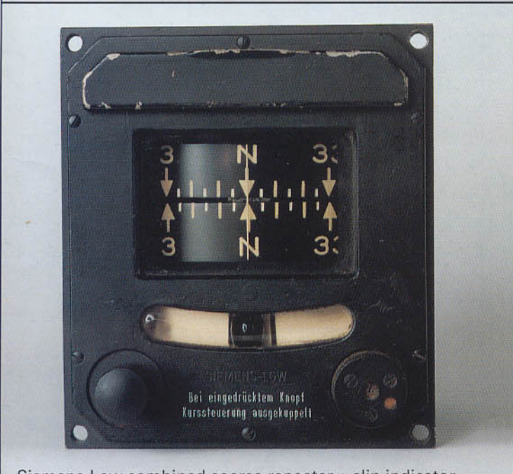
Siemens-Low combined coarse repeater + slip indicator.
