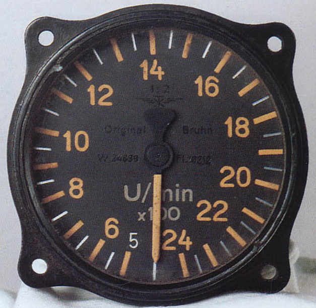
Tachometer calibrated to 2400 rpm marked Original Bruhn.
