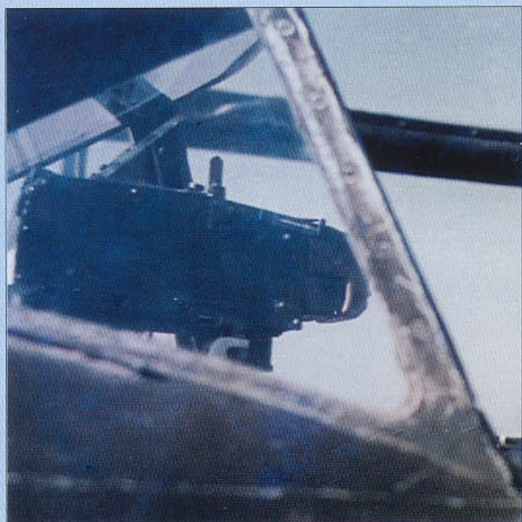
Above: The EZ 42/1-A1 gyrosopic gunsight (EZ - Einheitszielvorrichtung / Standard sighting device), manufactured by Askania, was introduced late in 1944 and intended for fighters such as the Ta 152, BV 155 and the Me 262 (shown above).
