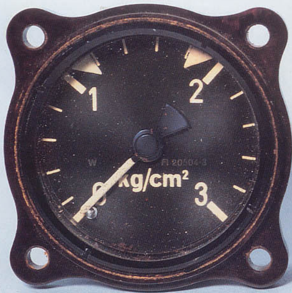
Methane/water boost pressure gauge.
