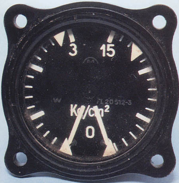
Dual fuel and oil pressure gauge.
