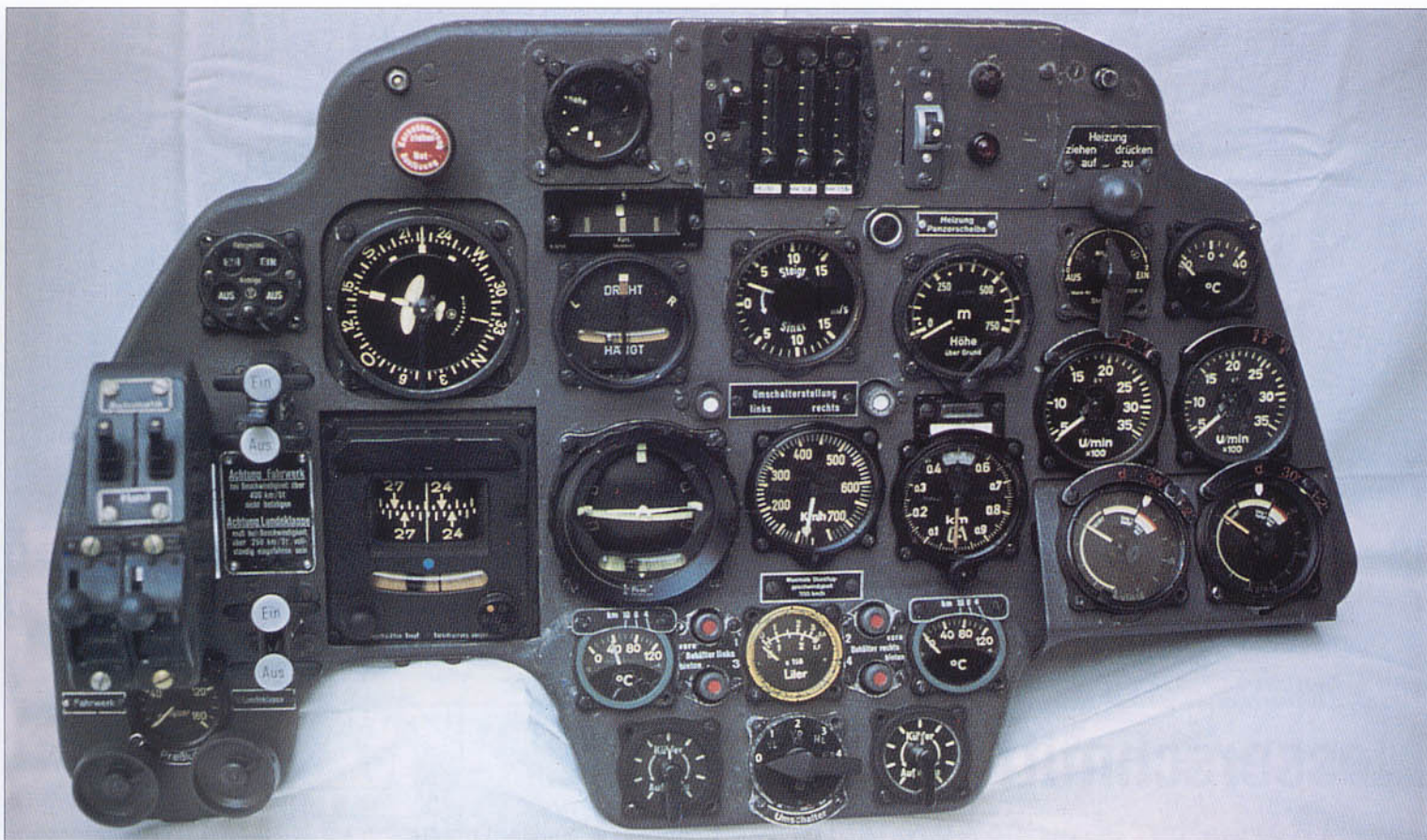
Above: The instrument panel shown above and the illustration below are typical of the ones used by the Bf 110 G-2 series. There were many variations within this basic format. The installation of new equipment to operational aircraft was a common occurrence in addition to aircraft returned from the front for reconditioning. The basic panel was available in metal or wood. The metal panel was fabricated from 3 mm sheet aluminum while the wooden version was made from 15 mm Beech veneer.
