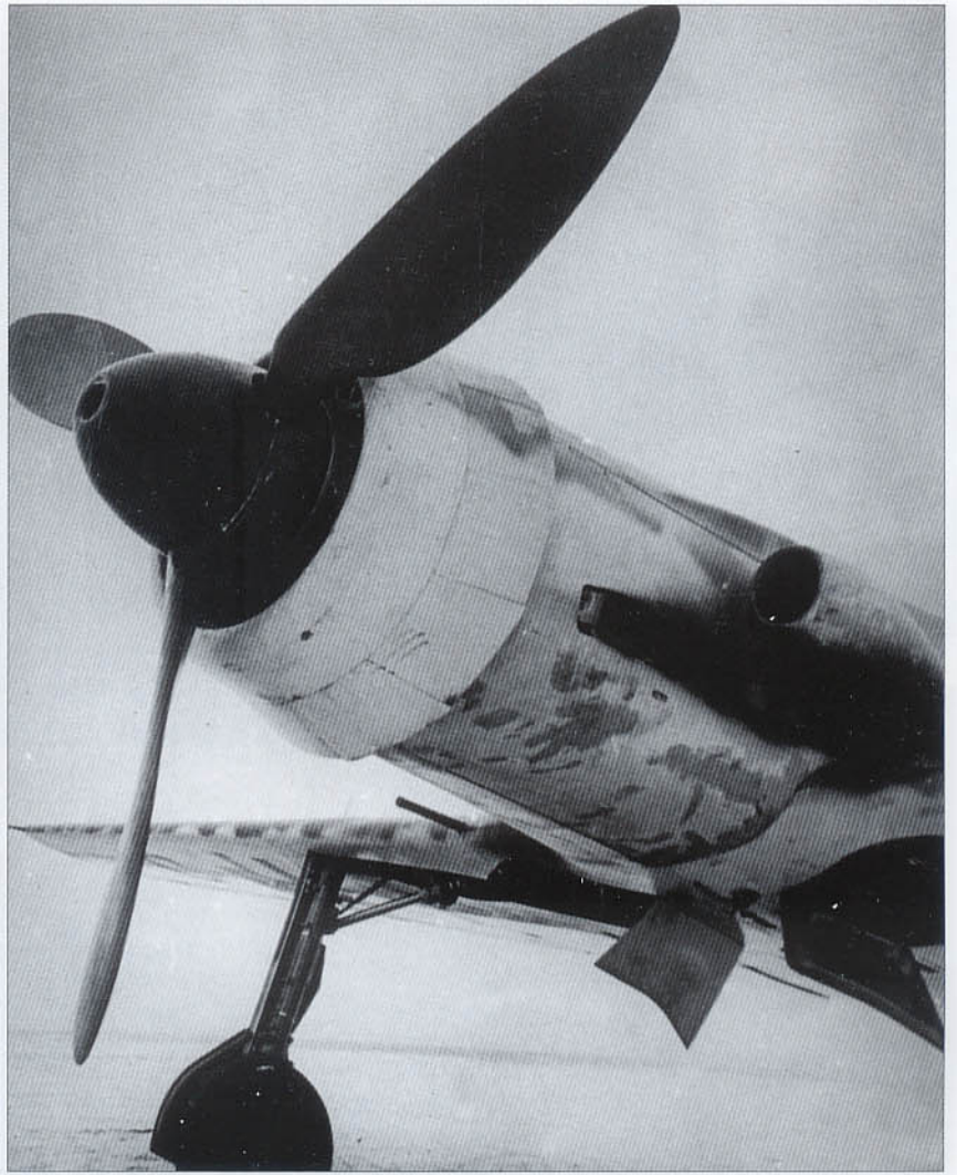
Above: A close-up of the top of the rear cowling of the Ta 152 V6 showing the installation of the twin 20 mm MG 151/20 cannons. Right: The 11 ft 9 inch (3,600 mm) diameter metal VDM variable pitch propeller of the Ta 152 V7 is well shown in this photograph. The spinner's opening is for the engine-mounted 30 mm MK 108 cannon. This prototype was powered by a DB 603 EM, although the DB 603 L was tested on the Ta 152 V6.
