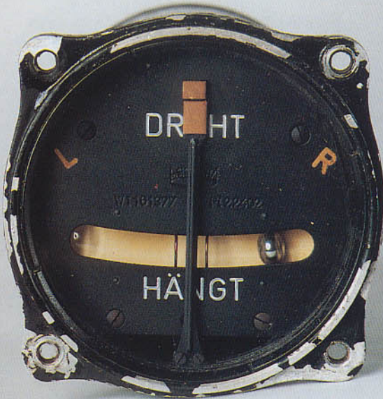
Turn and bank indicator made by Askania.
