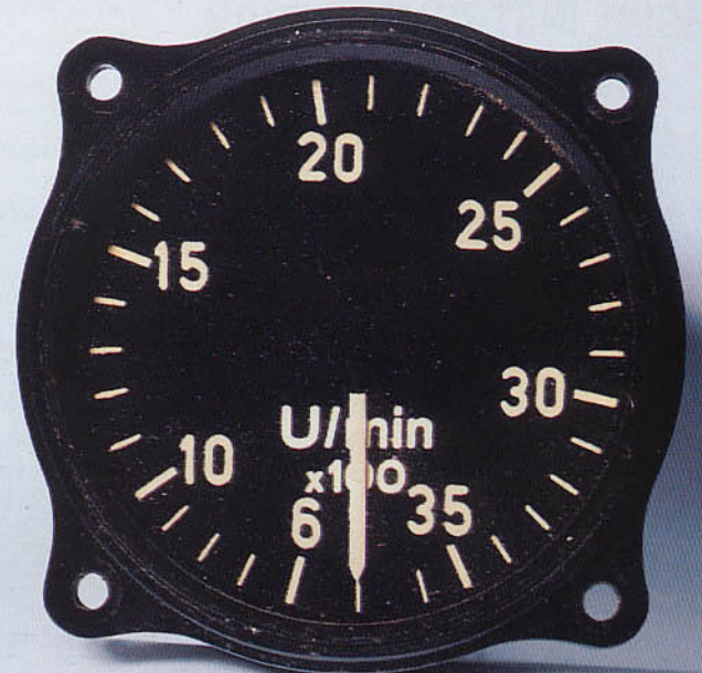
Tachometer calibrated to 3500 rpm.
