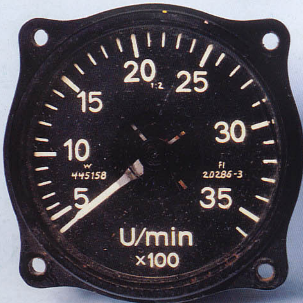
Tachometer calibrated to 3500 rpm.
