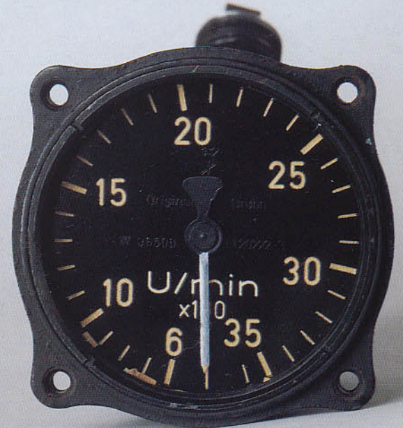
Original Bruhn tachometer calibrated to 3500 rpm.
