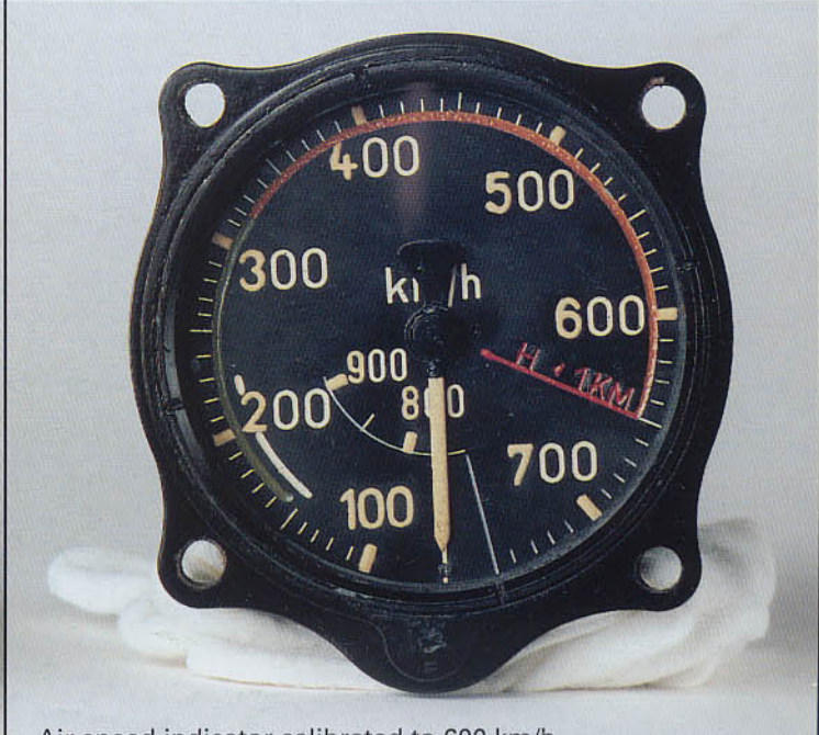
Air speed indicator calibrated to 600 km/h.
