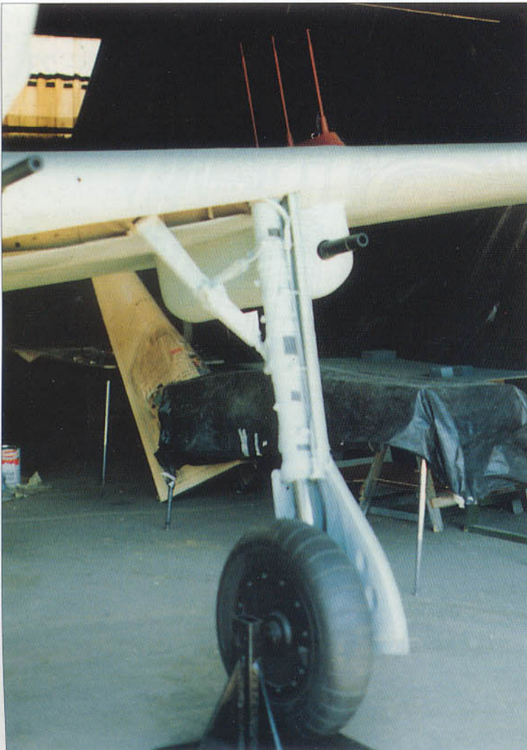
Below: A close-up of the port landing gear with the simulated gondola housing a replica of the MK 108 immediately behind it. The main wheels were size 700 x 175 with 300 mm diameter brakes. The brakes were hydraulically actuated by toe pressure on the rudder pedals. The wheels could be braked individually or together.
