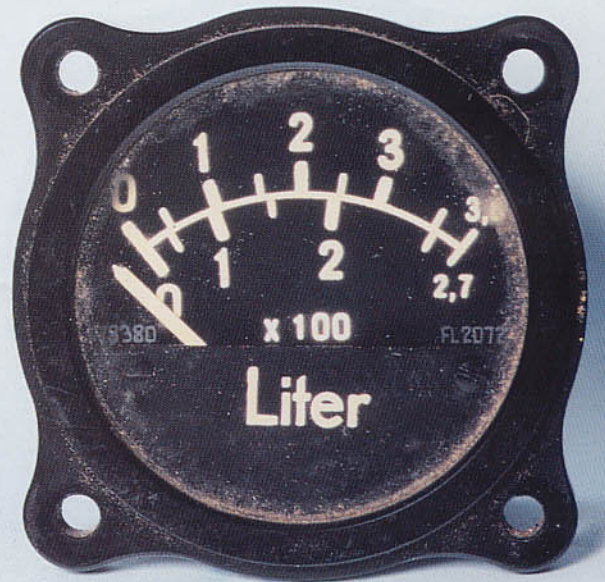
Dual fuel tank contents gauge.
