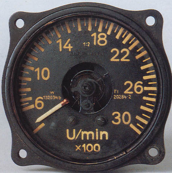
Tachometer calibrated to 3000 rpm made by Deuta-Morell.
