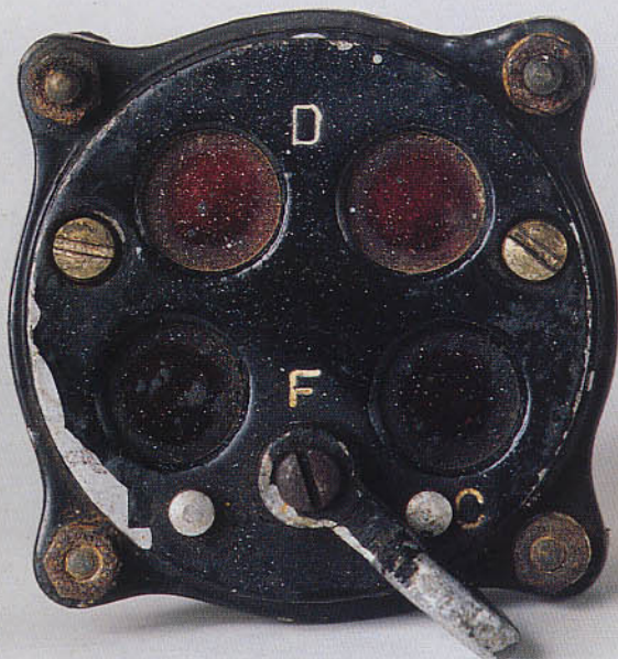
Undercarriage position indicator lights.
