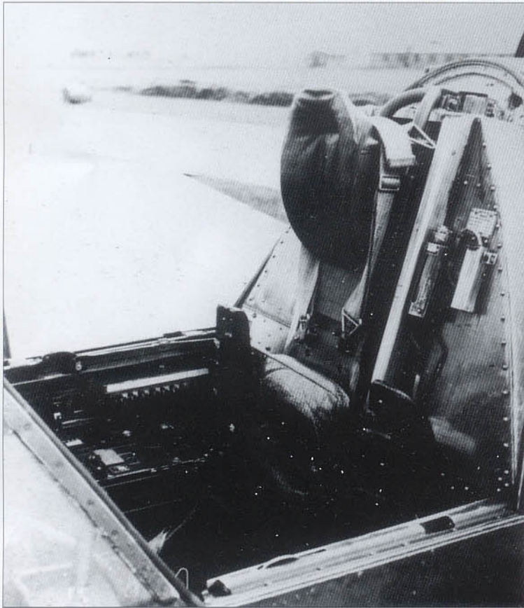
Above and left: Two views of the pilot's ejection seat. The top photograph shows the system installed within the Do 335 V1. If the pilot had to eject from the aircraft, he first drew his legs up and locked his heels onto the stirrups before being ejected.
