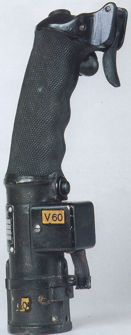
Starboard view of KG 13B showing microphone button.
