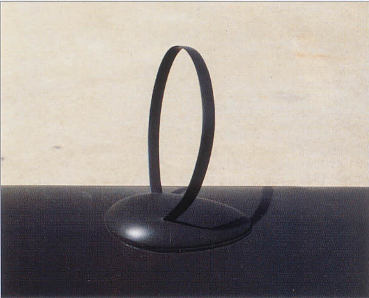
Below: Close-up of the fixed position homing direction finding antenna known as the Peilrahmen PR 16 which was mounted on the top of the rear fuselage.
