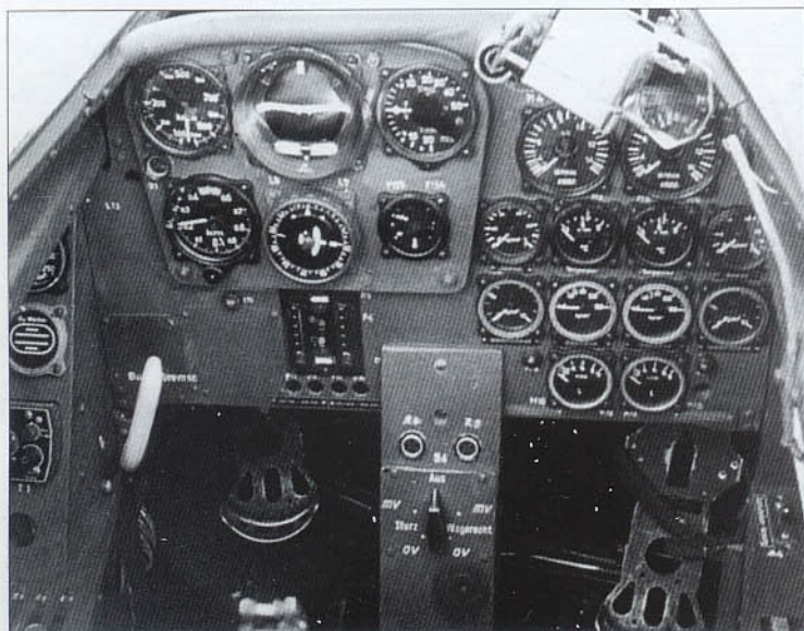
Above: Detail of the fusing panel for the external bomb load; the switch allows selection for a diving ( Sturz ) attack or a level ( Wagrecht ) attack. The arming indicator lights for each bomb are at the top of the panel. The arming panel for the nose-mounted cannon can be seen just to the left, below the blind flying panel.
