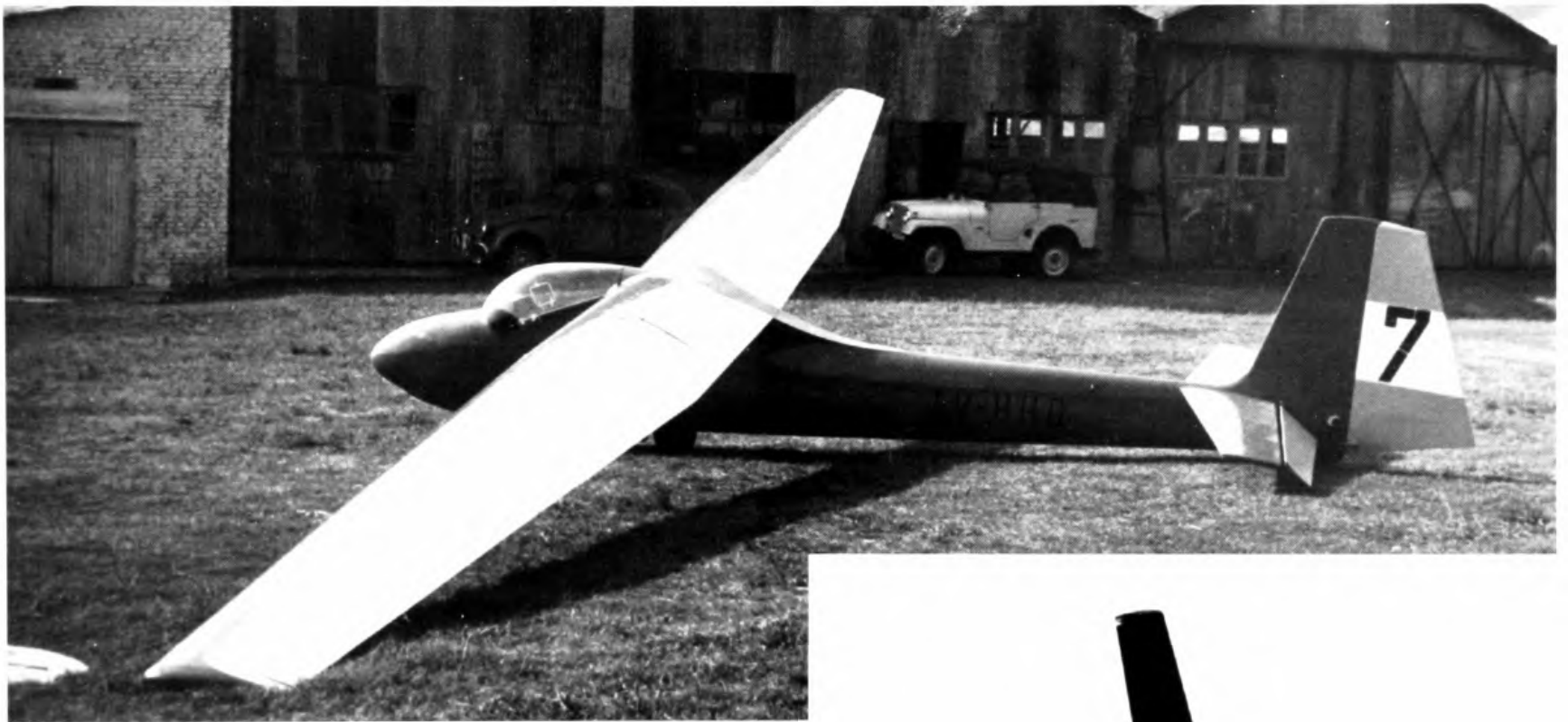
The Skylark 3F BGA 980, registered LV-HHO in Argentina, with bulbous canopy, aileron servo-tabs and a tailplane of reduced chord and greater span. ( F. Irving )
