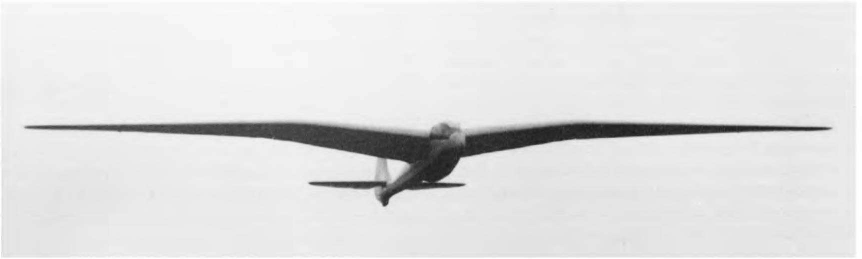
A characteristic view of the Petrel on approach to landing. The very thick wing root and pronounced taper, with the gull wing, give it a highly distinctive appearance. (M. Simons)
