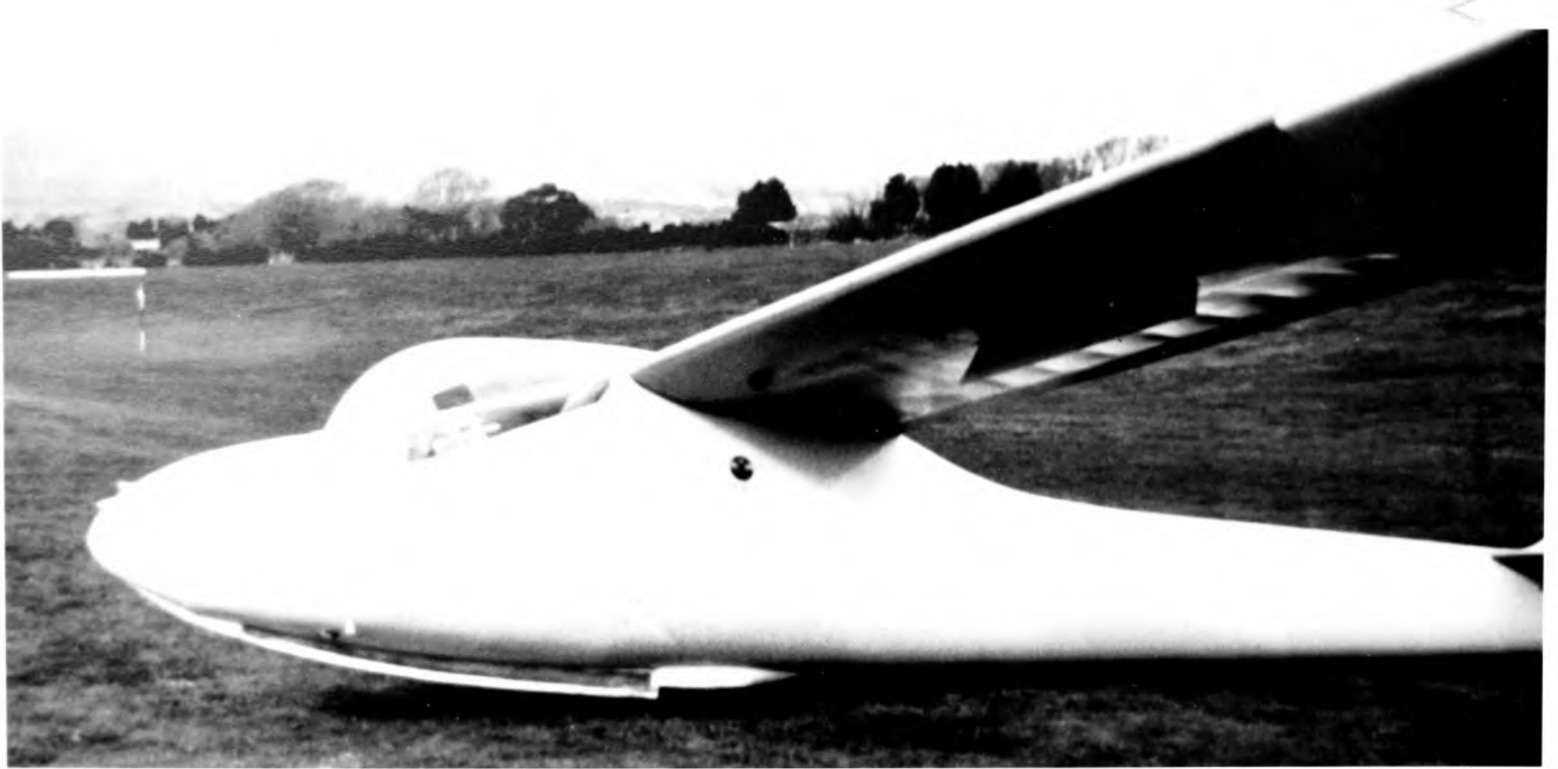
A Skylark 3F, showing the enlarged canopy and improved wheel fairing.
