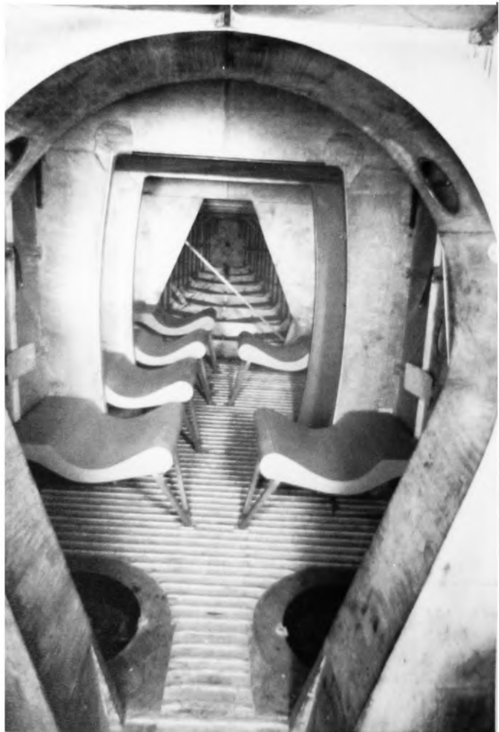
The rear cabin, with seats and a view down to the tail inside the fuselage. Chutes for supply dropping are visible in the floor. ( Slingsby collection )
