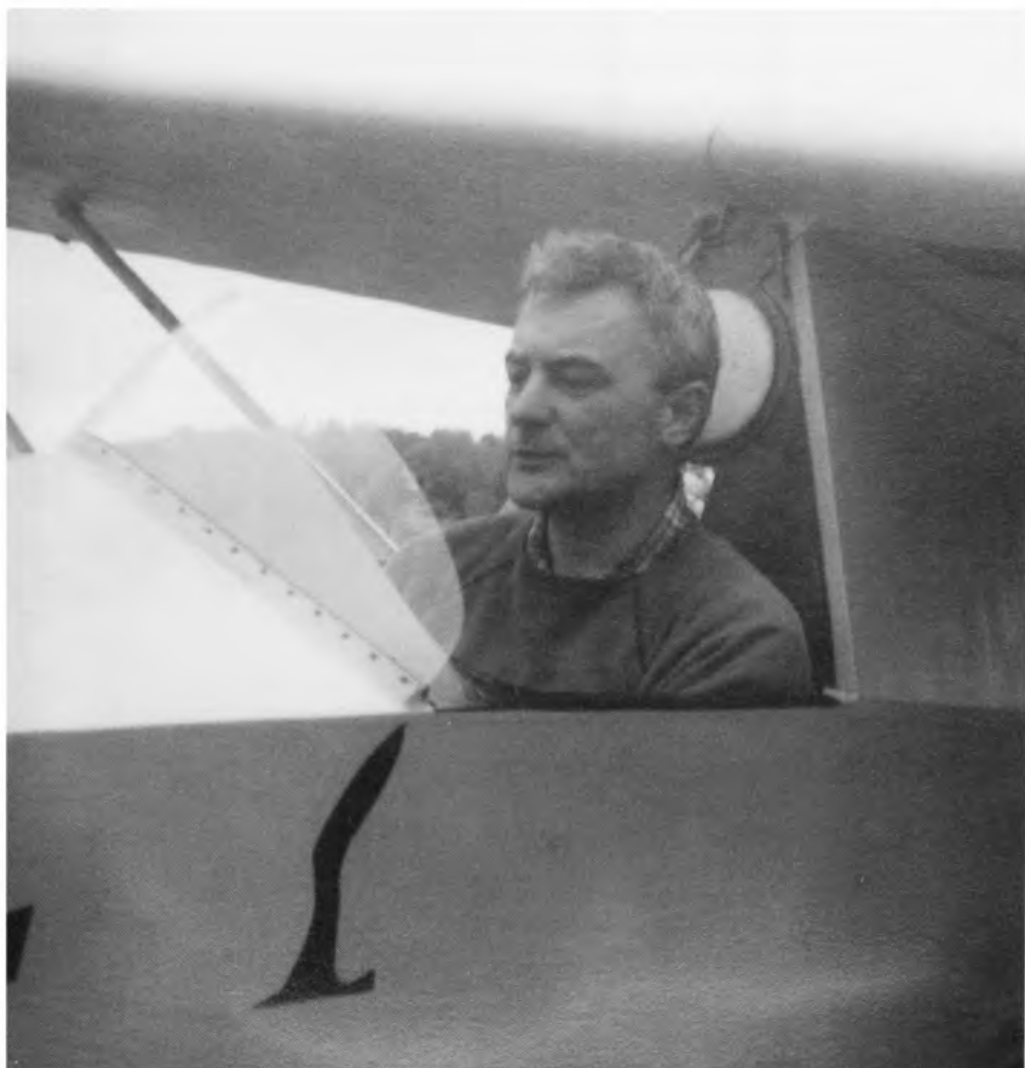
The cockpit of the UT-1, showing the handles of the wing mounting rods behind and above the pilot's head. A wind-screen was fitted. ( R. Smith )
