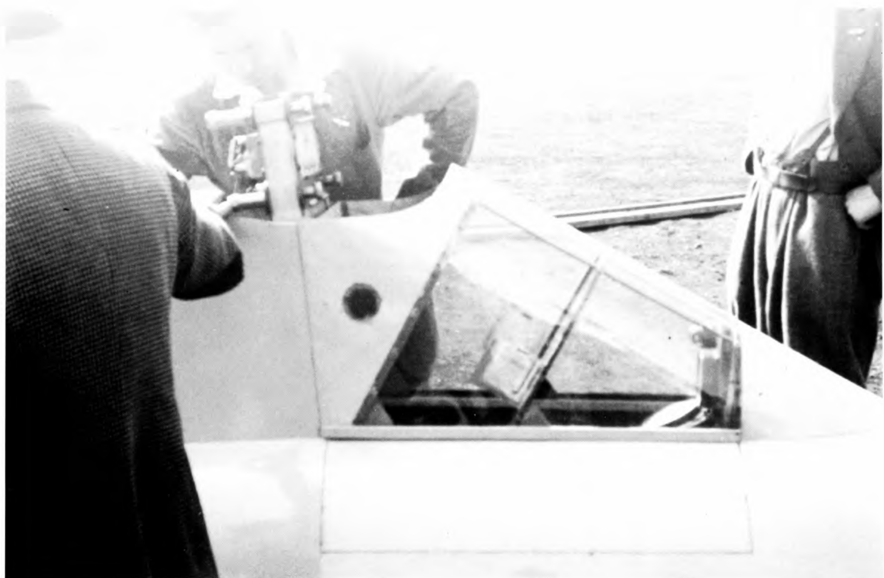
The cockpit canopy of Hjordis before modification. The main fittings on the fuselage frame are also visible. (Wills collection)
