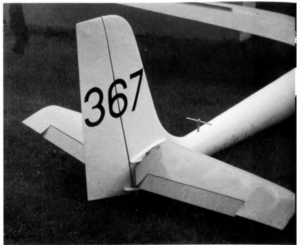
The tail unit of the Dart 15, showing the anti-balance tab on the all-moving tailplane. The wheel being ahead of the c.g. made lifting the tail of the empty aircraft for ground handling quite difficult. The T-shaped lifting handle was removed before flight. ( G. Bailey-Woods )
