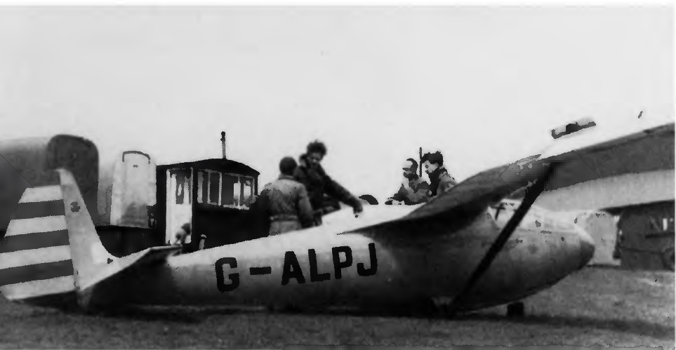
BGA 378, with wheel, at the Derbyshire and Lancashire Club site at Camphill in 1949, showing the club's blue and white stripes on the rudder and the registration letters. Otherwise the finish was clear dope and varnish. This Gull, with modified cockpit canopy, still flies regularly. ( M. Simons ).
