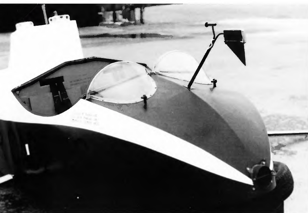
A close-up of the nose of Sedbergh WB924, showing the cylindrical ballast housing fitted to many ATC Sedberghs to allow solo flying without fuss. The pitot guard is removed before flight. (M. Simons)
