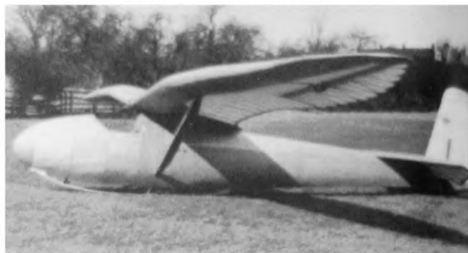
The prototype Kite with the angular Grunau Baby type of rudder. ( Wills collection )
