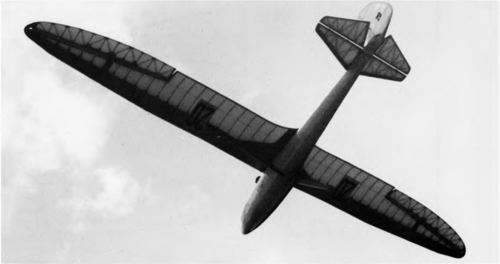
One of nine Kirby Kites flying in the 1938 BGA National Competitions at Dunstable. The pilots of this Midland Gliding Club example were F. J. Davies, R. F. James and B. T. Oliver. Note the absence of any seal for the elevator hinges. (C. Brown)
