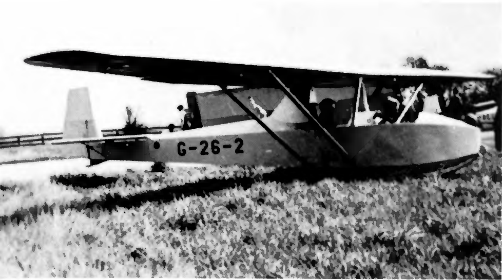
The original T-31 with the B conditions marking G-26-2. Note the absence of auxiliary struts. ( Slingsby collection. )
