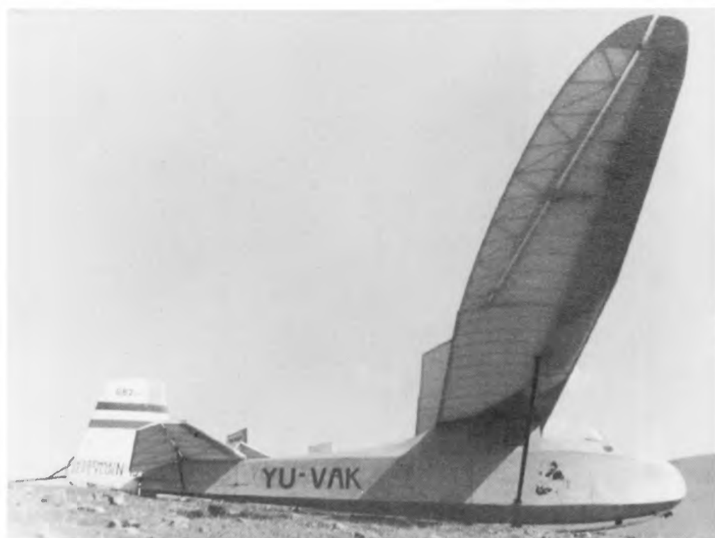
A Grunau Baby 2A in Yugoslavian colours. Note the revised form of elevator and cockpit canopy, but the absence of air brakes.
