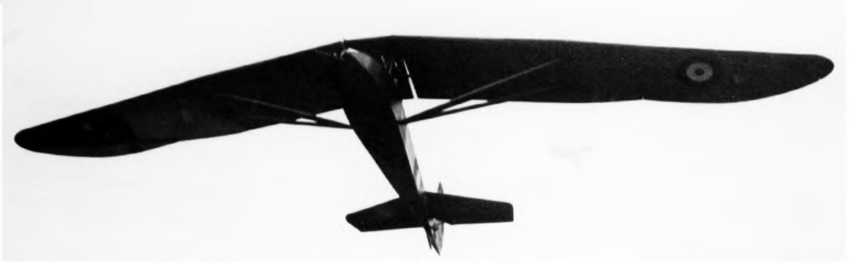
Falcon 3 in ATC paint scheme taking a winch launch somewhere in England. Note the apparent gap at the wing root was closed with transparent plastic. Signs of wing damage and repairs may be seen.
