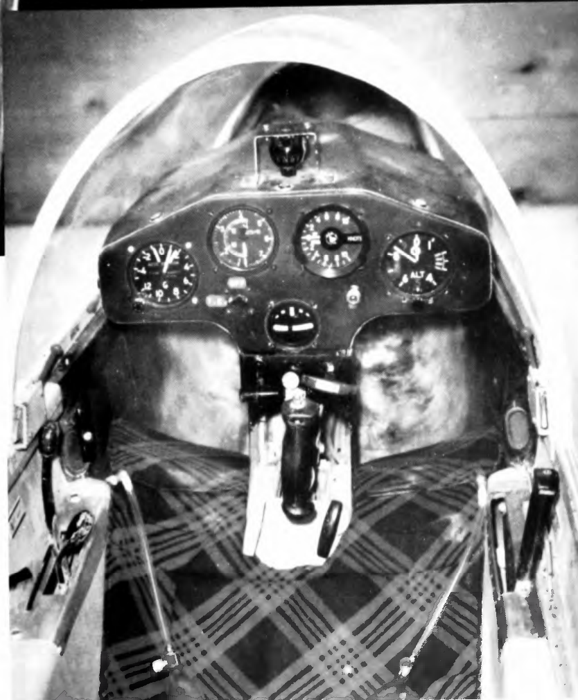
The instrument panel and cockpit of the T-59A, 17m Kestrel. On the left side of the cockpit are the flap and airbrake levers, the canopy latch, ventilator and drogue parachute deploy handle. On the right cockpit wall are the undercarriage retracting handle, seat back adjustment, canopy latch and ventilator. On the central console, left to right are the tow release below the landing flap handle, canopy demister and drogue jettison handle, with rudder pedal adjustment below. On the stick are the radio transmit button, elevator trimmer and wheel brake. On the seat, hand pumps for inflatable seat cushion. The water ballast tap is behind the pilot's head. (G. Bailey-Woods)
