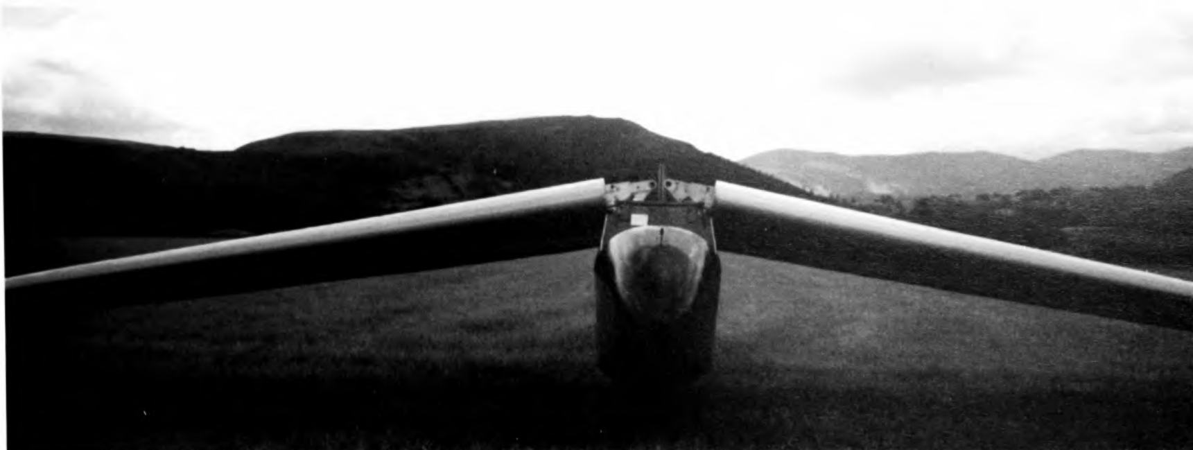
Rigging the Swallow. With both wings attached to the fuselage by two steel pins, the tips are raised together to allow the upper main spar connection to be made. (A. Edwards)
