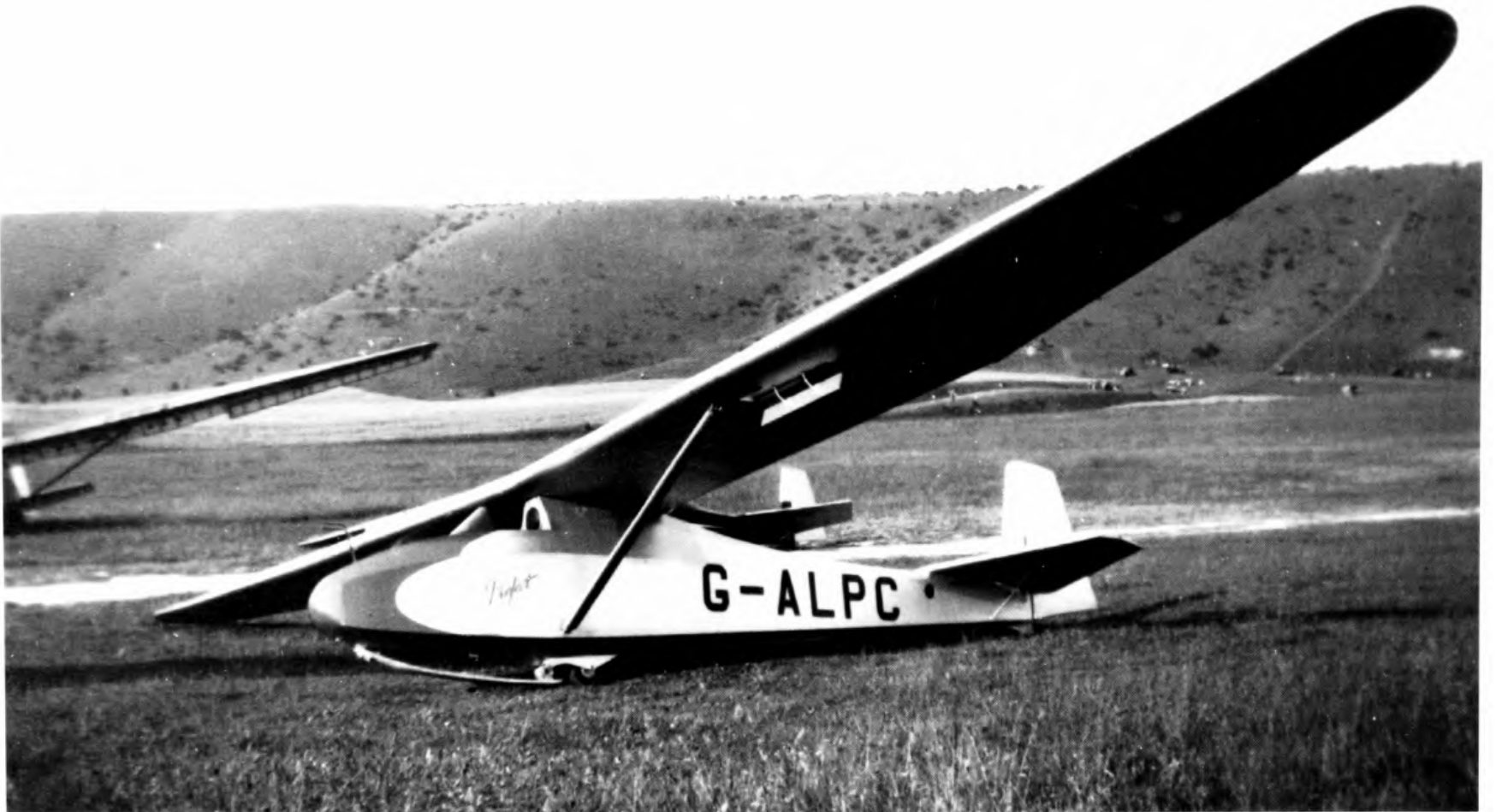
G-ALPC, the second Prefect built, is shown here at Dunstable in 1950. Note that the airbrakes were of the old DFS pattern. On later Prefects these were replaced by the vertical 'parallel-ruler' brakes of Schempp-Hirth type. In the left background is the wing of the two-seat Hawkridge Venture G-ALMF. ( Slingsby collection )
