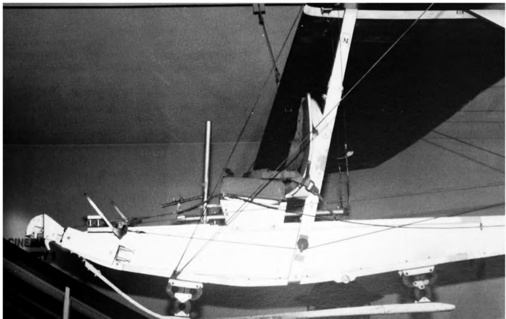
Grasshopper WZ791 on display at the RAF Museum, Hendon, in 1992. Although basically a very simple aircraft, rigging a primary glider correctly was not straightforward because the cables had to be correctly tensioned to ensure that the wings and tail unit were accurately aligned. To get this aircraft into position for display occupied the museum staff for 6 hours. ( M. Simons )
