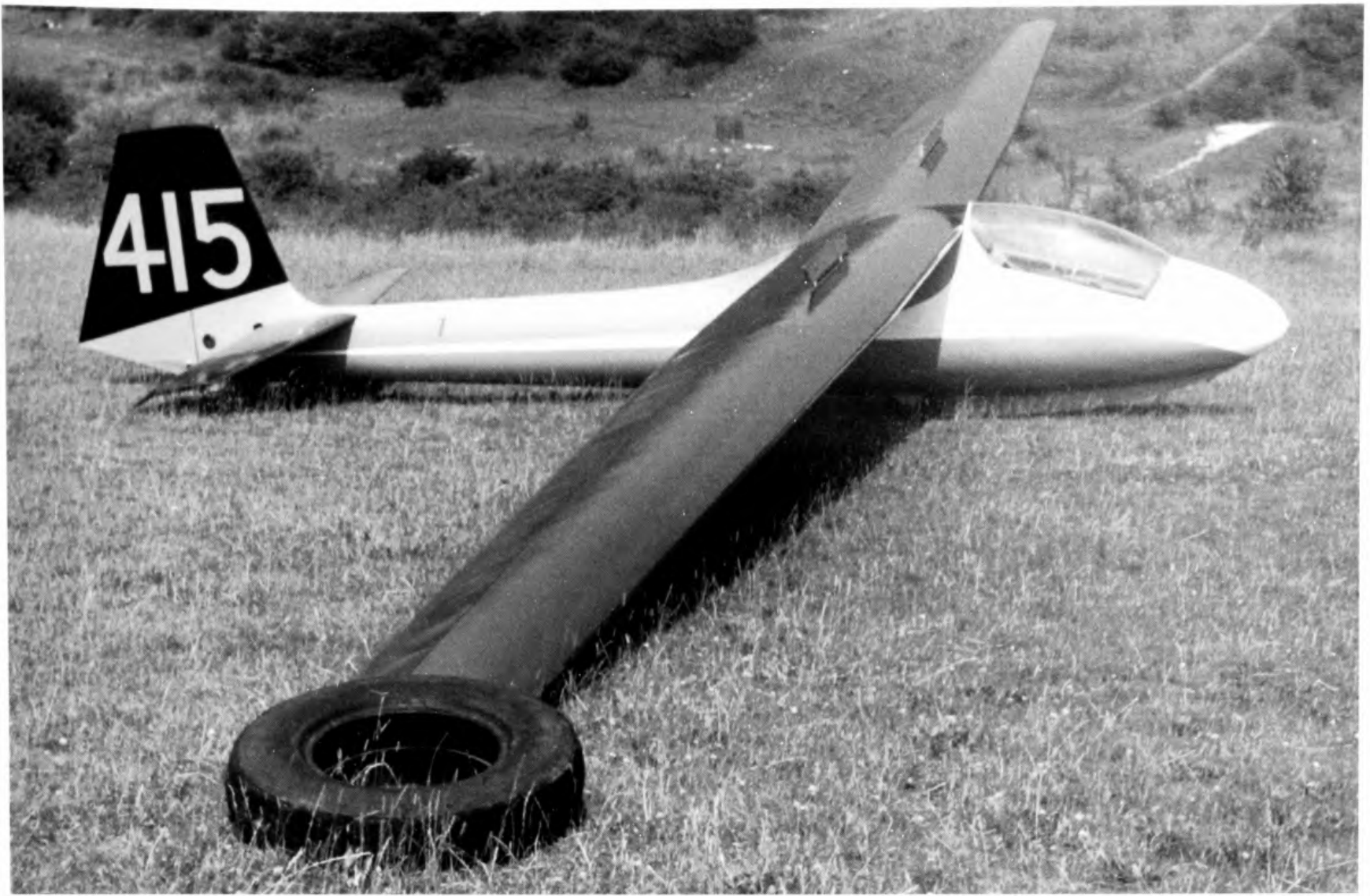
The Tull Brothers' Skylark 3, built from a kit and fitted with the Skylark 4 cockpit canopy, greatly improving the appearance and reducing drag. ( M. Simons )
