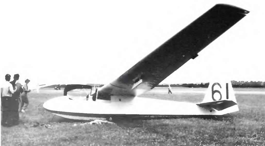
An Eagle 3 at Lasham. The airbrakes were now part of the outer wing, instead of being in the centre section. A fixed trim tab on the port aileron indicates that this particular aircraft had a 'one wing low' tendency, probably after repairs.
