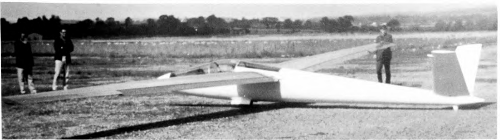
The prototype Slingsby HP-14, built from a kit supplied by Schreder. Here it has the original small V-tail. (G. Bailey-Woods)
