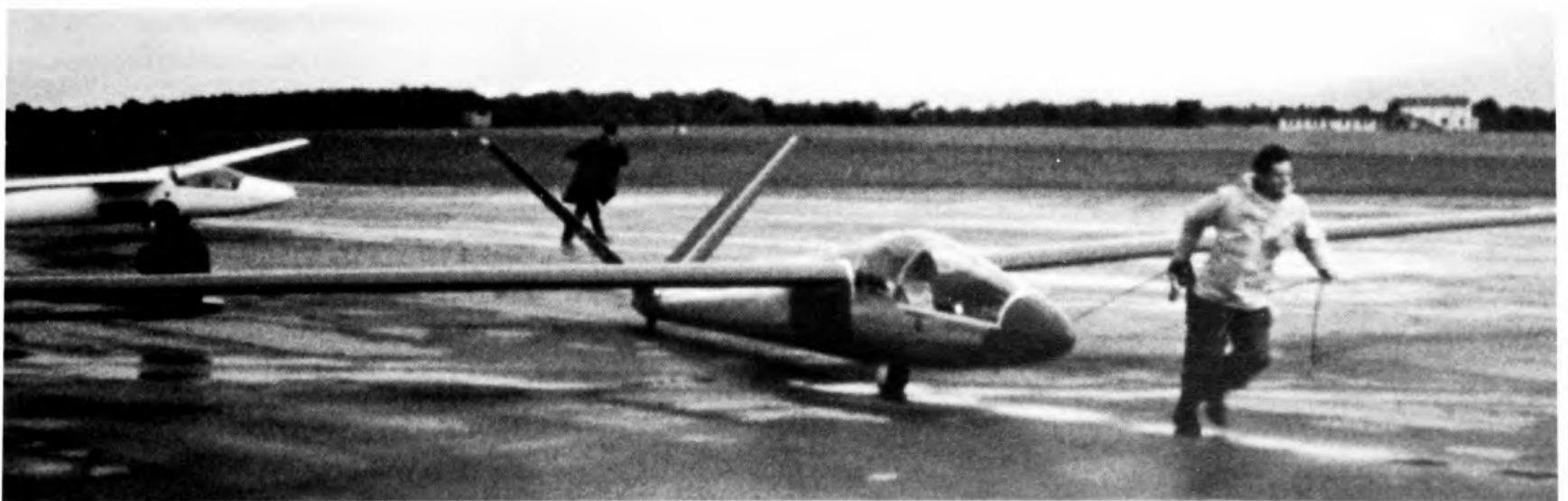
The Slingsby HP-14 at the British National Championships, being towed out to the take-off point at Lasham. The tail surfaces are greatly enlarged. (M. Simons)
