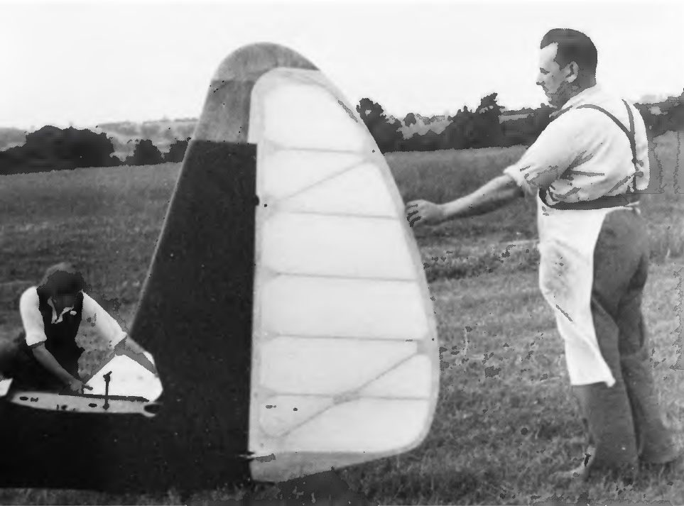
An early experiment with a much-enlarged rudder with aerodynamic balance. This was not adopted for production. ( Slingsby collection. )
