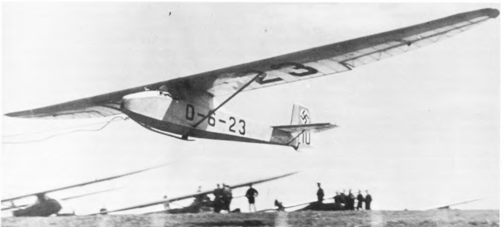
A Grunau Baby 2 bungee launched at the Wasserkuppe in the 1933 competitions. A windscreen has been fitted to this example and some instruments are carried, as indicated by the venturi and pitot tube on the front fuselage decking. Others of the type are visible on the ground. The markings were typical of the year in which Adolf Hitler came to power.
