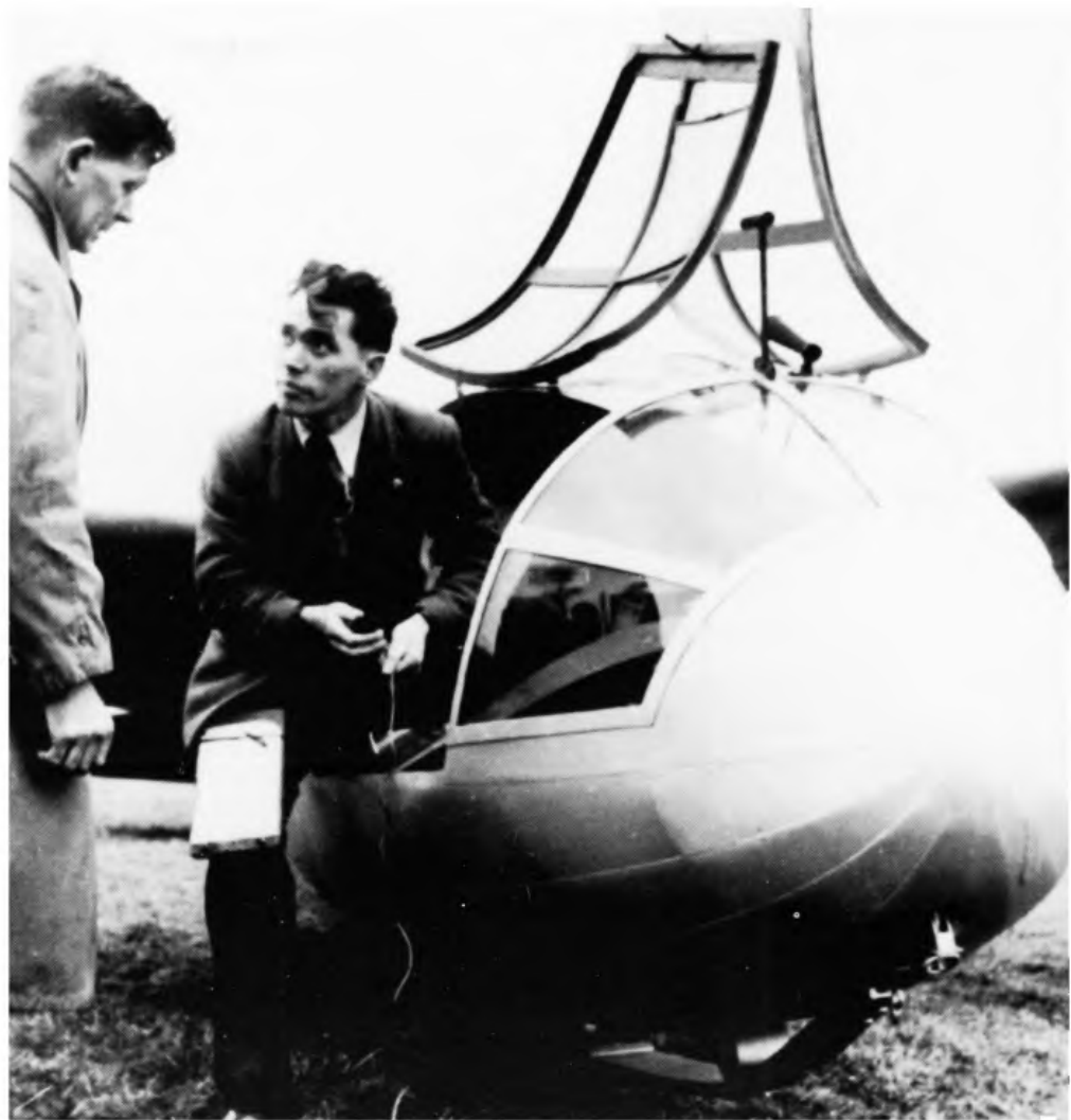
A photograph of unknown origin, but probably showing preparations for a test flight about 1952. The long tube may have been used to suspend a static bomb below the fuselage when in flight, to check the position error of the air speed indicator. Note the 'Ottfur' aero-tow release. Later photographs show this taped over, with the towline attached to the belly hook.
