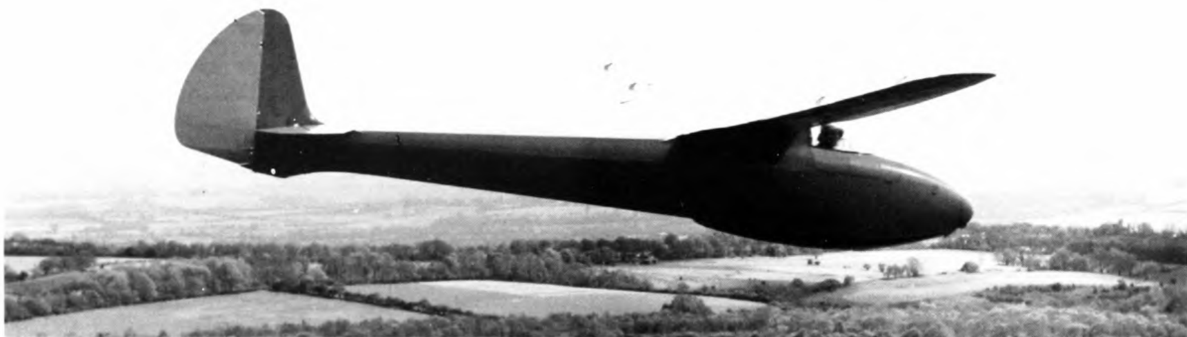
Philip Wills flying his Sky with the landing skid instead of the fixed wheel arrangement. Performance tests by the BGA Test Group 1 based at Lasham showed a gain of one point in
