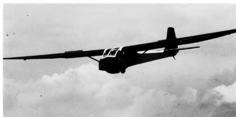
Only one T-46, often called the T-21C, was built. The wing remained similar to that of the T-21 but was mounted on the fuselage at shoulder level, with a tidy enclosed canopy. The tail unit was also redesigned, but the improvements were not considered sufficient to justify series production of the type. (I. Tunstall)
