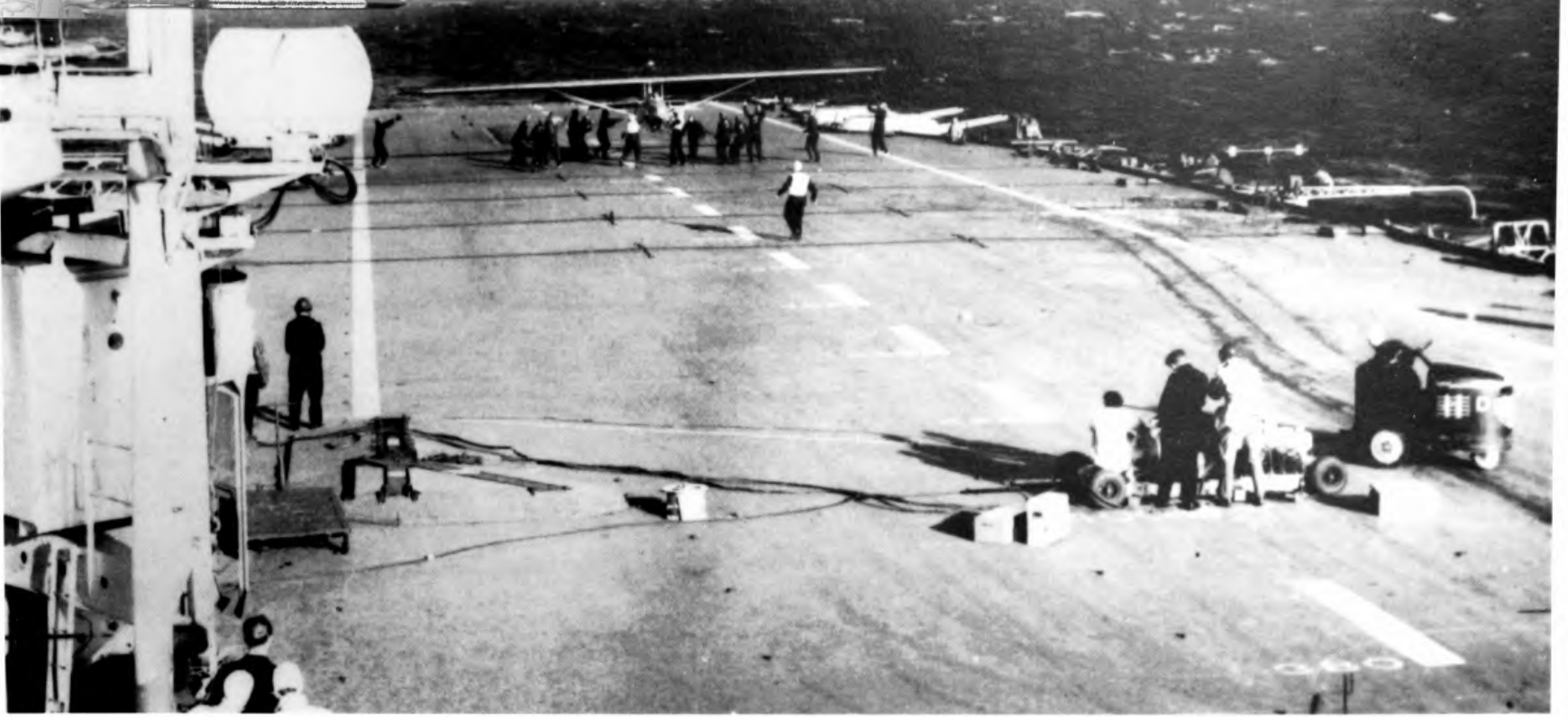
A view from the bridge. The T-20 is just airborne, restrained by the crew. The winch, and a small tractor, are seen in the right foreground. (Admiralty photo from J. S. Sproule)
