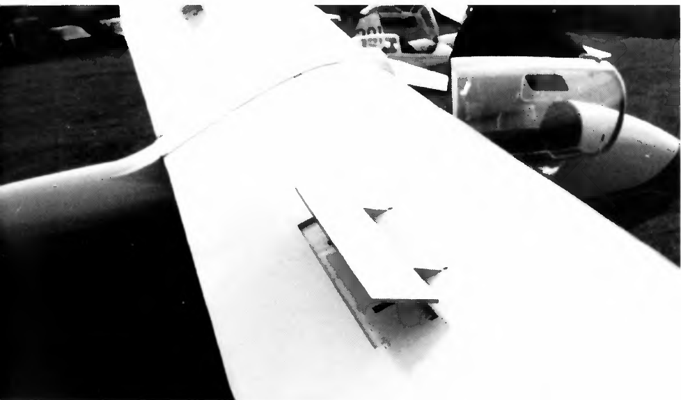
Airbrake detail of the Sky. When retracted, the brake paddle lies flush with the wing. (M. Simons)
