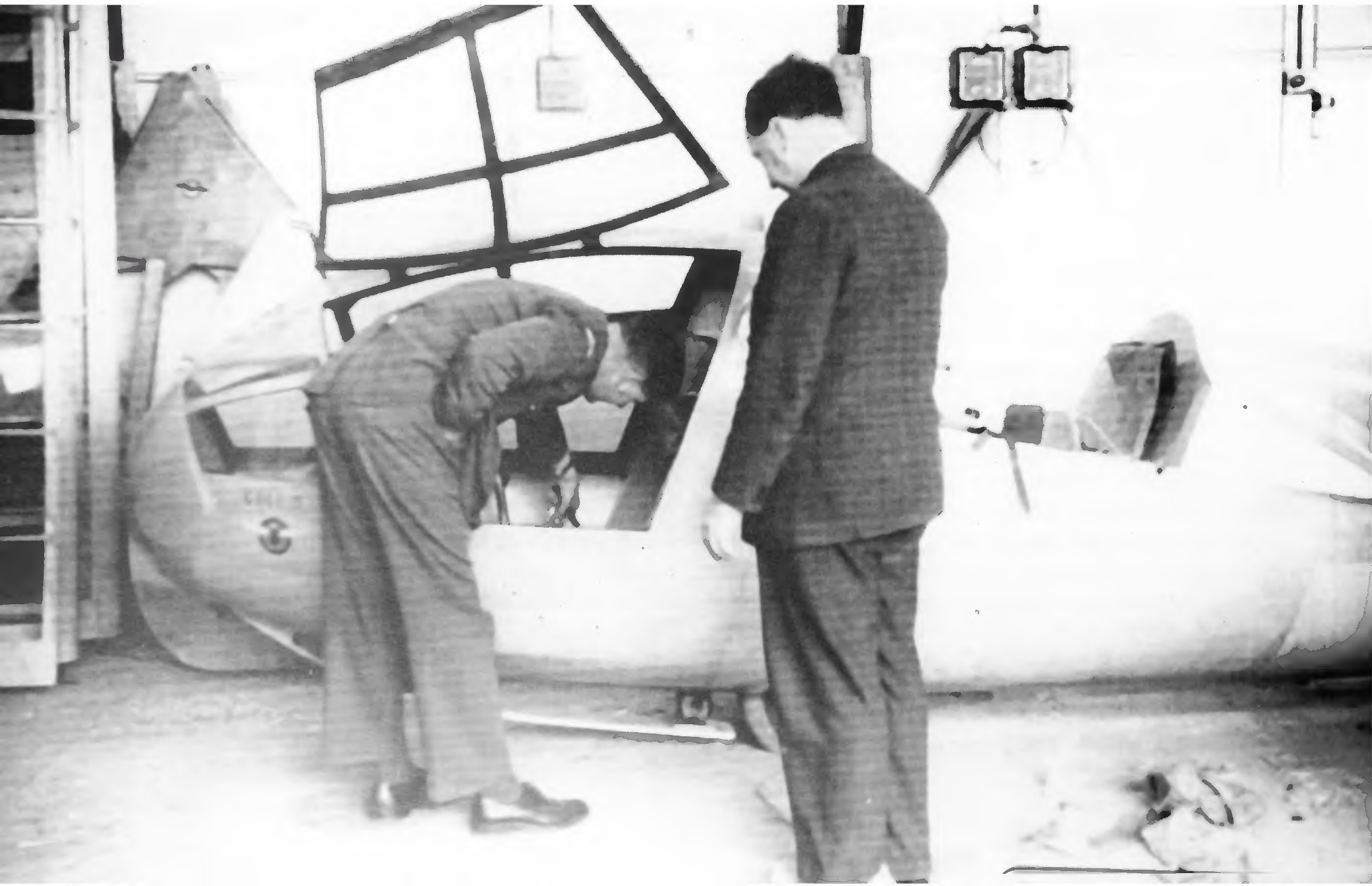
The Gull 2 nearing completion. Fred Slingsby (right) and an unknown assistant check the controls. Note the 'butterfly' type canopy. In the background are the A frame and wings of a Slingsby primary glider bearing the old golden eagle trade mark. ( Slingsby collection )
