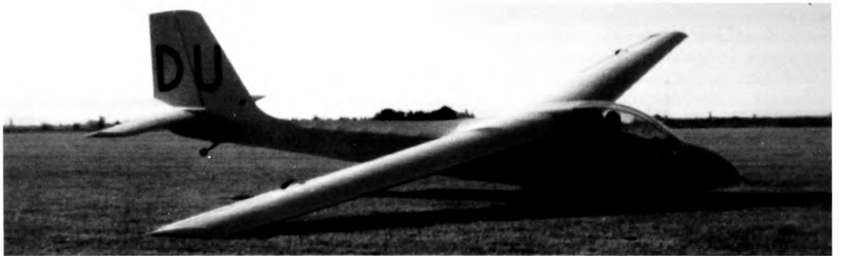
With two pilots on board, the Capstan rested on its wheel and front skid. On landing, once flying speed was lost the skid acted as a brake, but the wheel was also equipped with a brake, allowing very short landing run.
