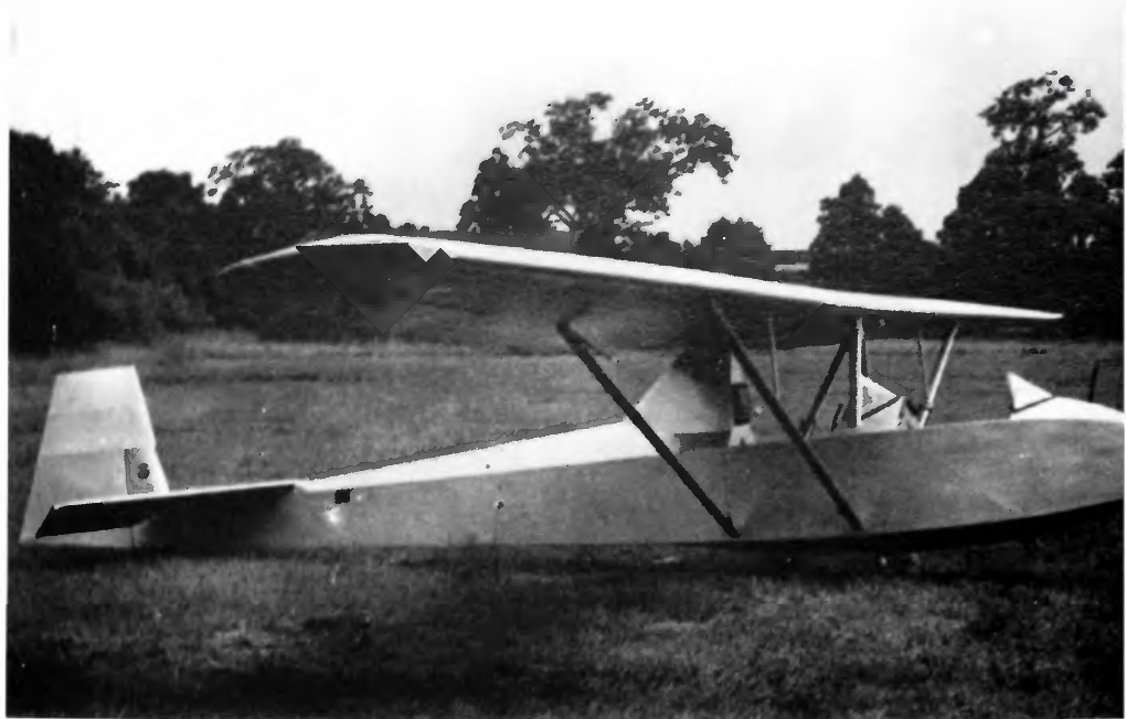
The prototype T-31B with the auxiliary bracing strut and spoilers. ( Slingsby collection. )
