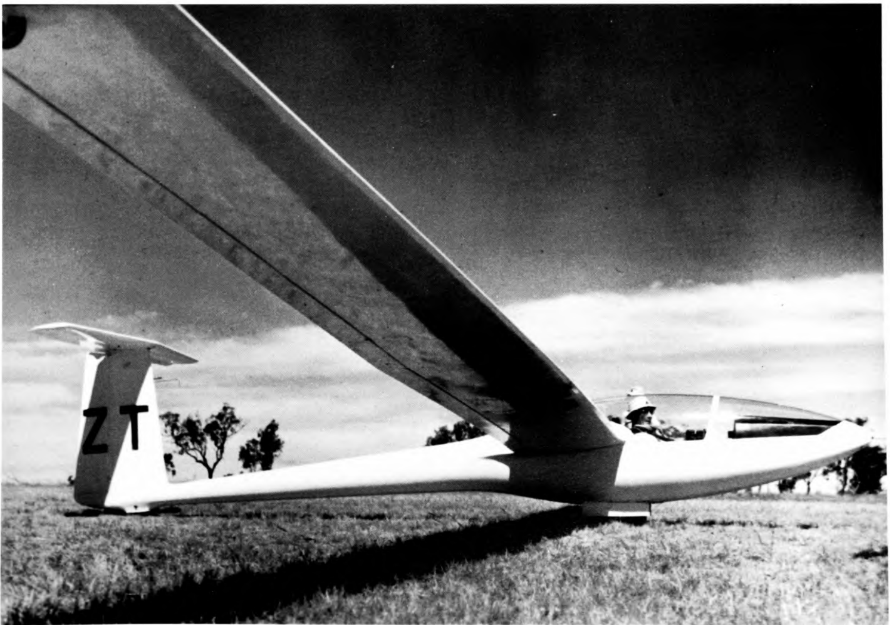
The Glasflügel 604, a 22m version of the Kestrel, flown by Bert Zegels at the 1974 World Championships at Waikerie. ( M. Simons )
