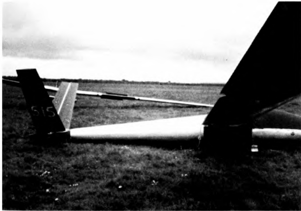
The enlarged tail unit of the HP-14 as flown by John Williamson in the National Championships. Incorrect rigging caused a spectacular ground loop on the first attempted take-off. (M. Simons)
