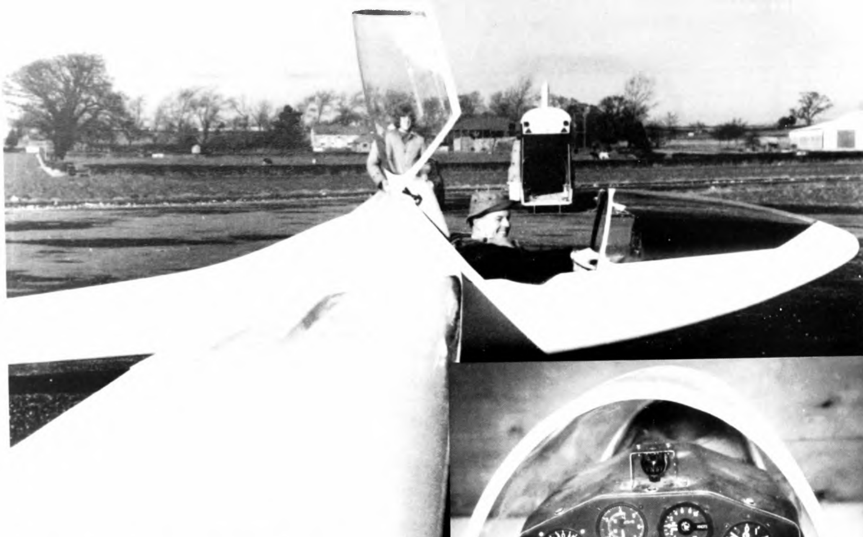
The first T-59A 17m Kestrel built by Slingsby prepares for take-off with Geoff Bailey-Woods as test pilot. The short canopy, with rear hinge, was introduced by Glasflügel but was changed to the older, long canopy on the Slingsby Kestrel 19. (G. Bailey-Woods)
