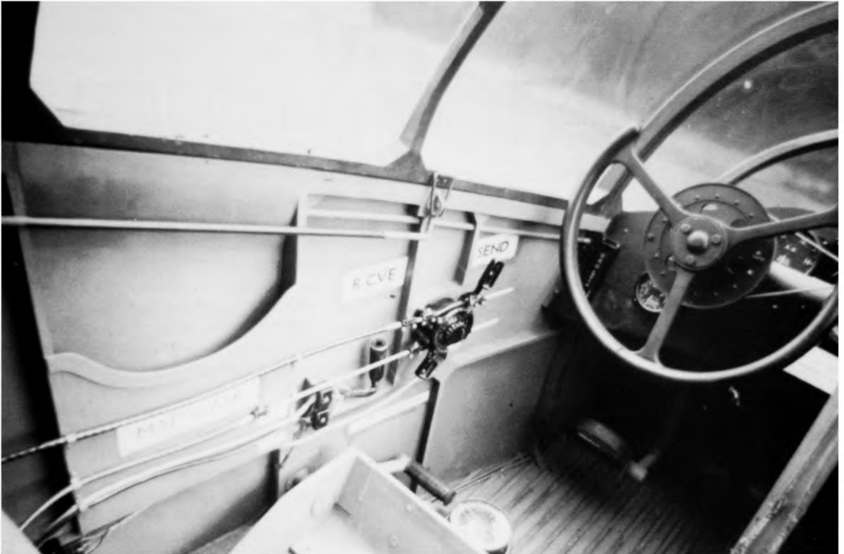
The cockpit, with wheel-type controls. The compass is mounted on the floor. ( Slingsby collection )
