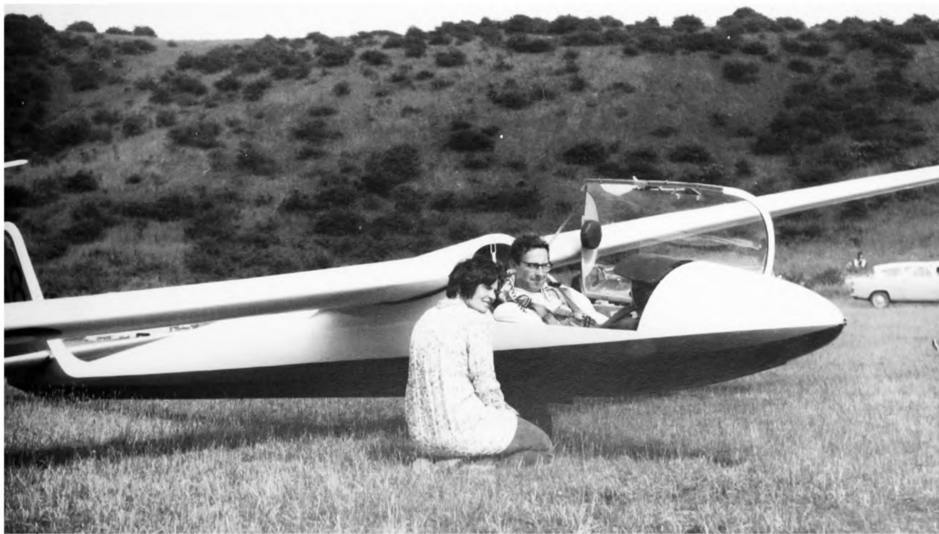
A Dart 17R with the author and wife, crew chief, preparing for aero-tow launch at Dunstable in 1967. Note the greatly improved ground clearance, allowing a lower angle of incidence. ( E. A. Hull )
