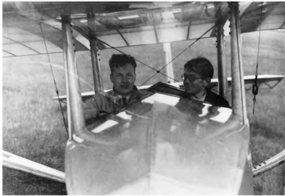
Murray (left) and Sproule in the Falcon 3 at Dunstable on the occasion of the 22hr two-seat duration record in 1938. Note the external aileron drive cables, transparent panels in the centre section, and crossed wire bracing behind the cockpit. (J. S. Sproule)
