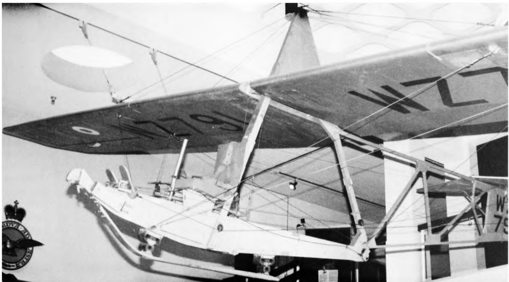
Grasshopper WZ791 on display at the RAF Museum, Hendon, in 1992. Although basically a very simple aircraft, rigging a primary glider correctly was not straightforward because the cables had to be correctly tensioned to ensure that the wings and tail unit were accurately aligned. To get this aircraft into position for display occupied the museum staff for 6 hours. ( M. Simons )
