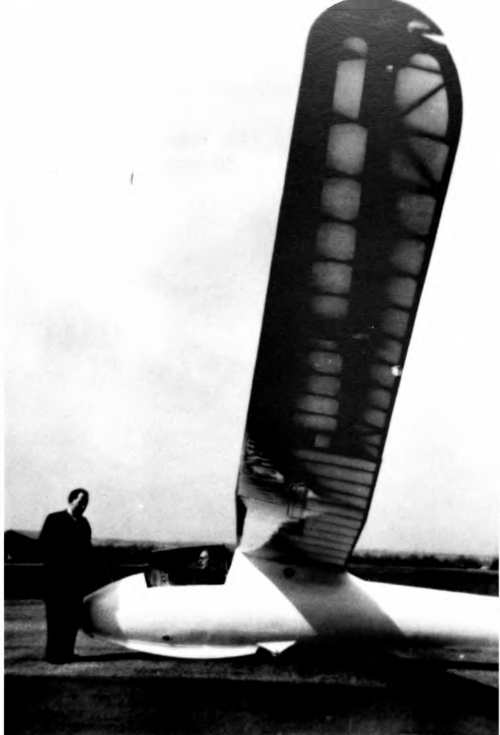
Wills, in the cockpit, and Slingsby, confer. The skids of the Gull 4s taken to Samedan were lengthened to fair in better with the wheel. The prototype, which was sold to the London Gliding Club, had a shorter skid. Also visible is the winch launching release. ( Wills collection )
