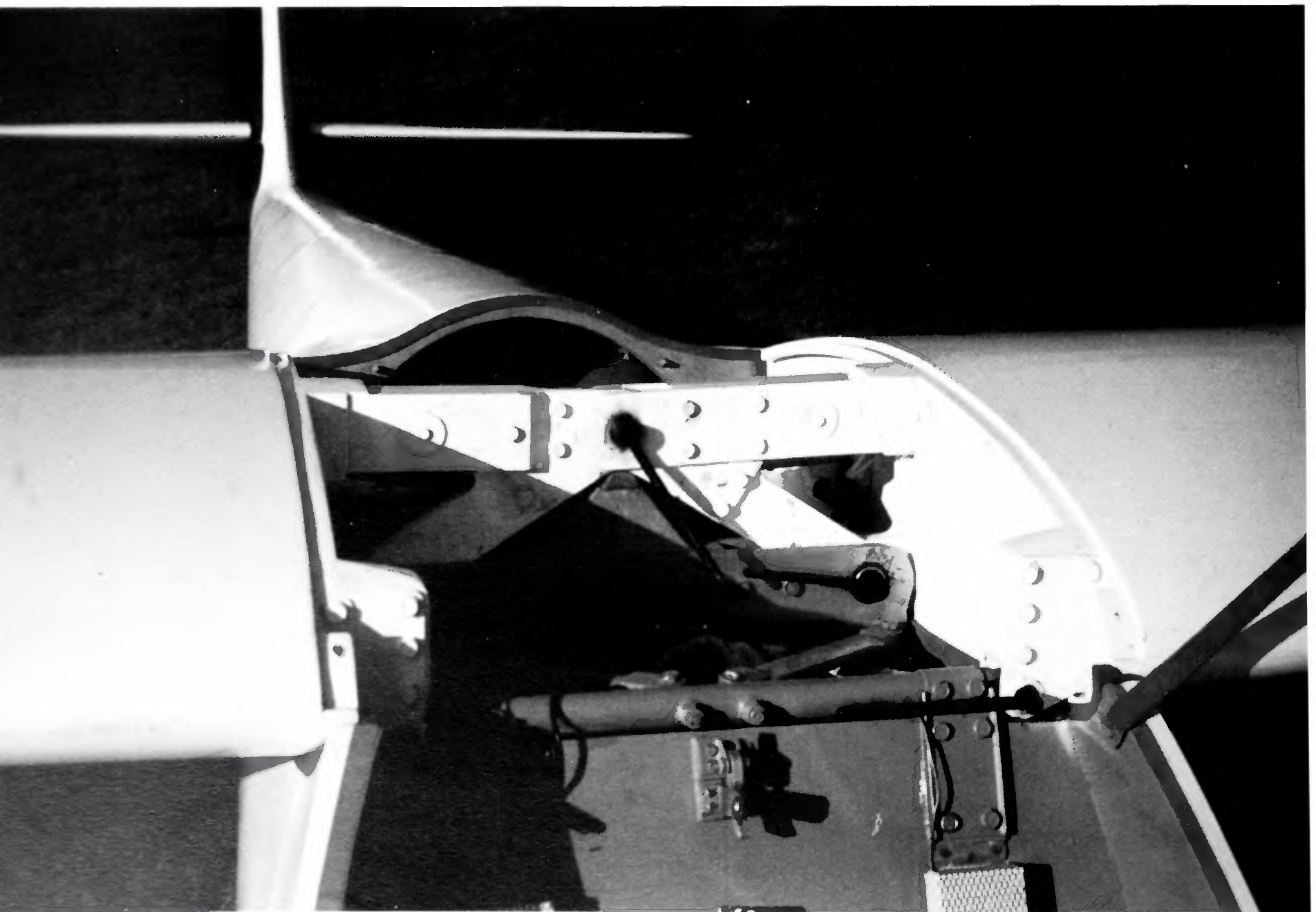
The wing rigging system of the Dart. Two steel pins, aligned on the same centre, attach each wing to the fuselage frames. A fifth pin then joins the upper flanges of the main spars. ( M. Simons )
