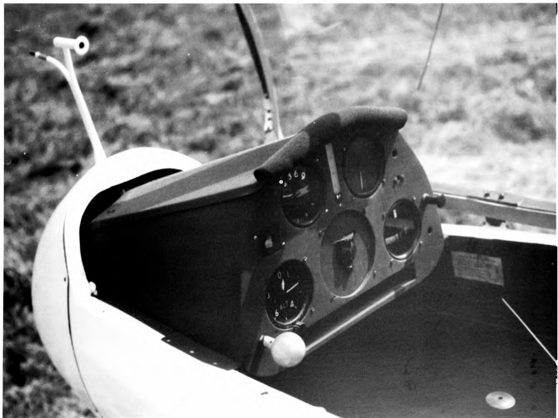
The instrument panel of BGA 418. The knob on the left is the tow release. ( M. Simons )
