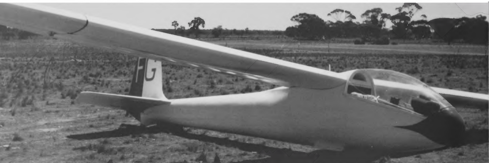
A much modified Skylark 4 in Australia. The cockpit canopy was altered to improve the contours, and a retractable wheel was fitted. ( M. Simons )
