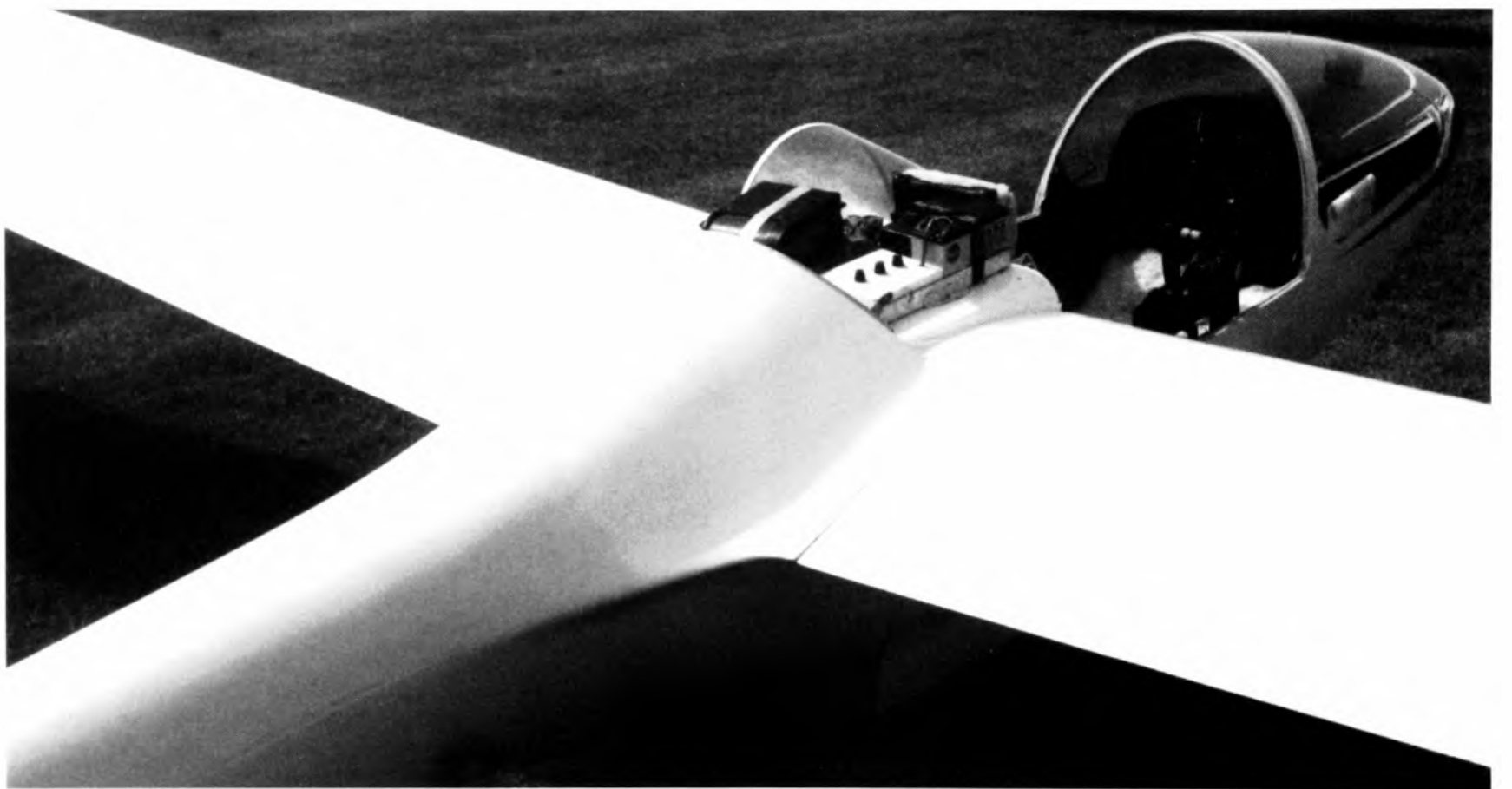
The Kestrel 19 showing the wing-root fairing developed to cure the low-speed flow problem. ( M. Simons )
