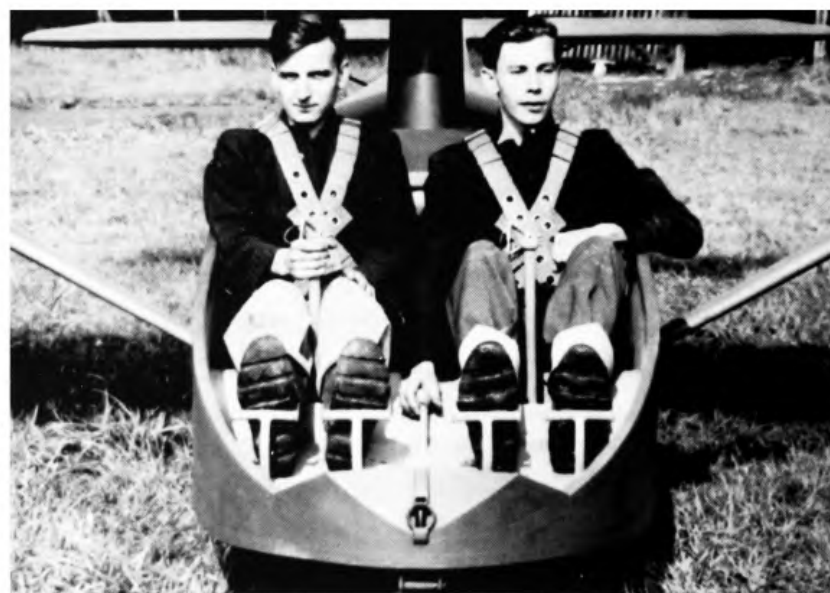
The original T-21P with its truly open cockpit. Other details of interest are the 'Sutton' harness made of canvas webbing, the instructor's hand on the tow release knob, and the aero-tow release visible in the extreme nose. The bracing wire sometimes fitted from the nose to the strut fitting is not present. (Slingsby collection)
