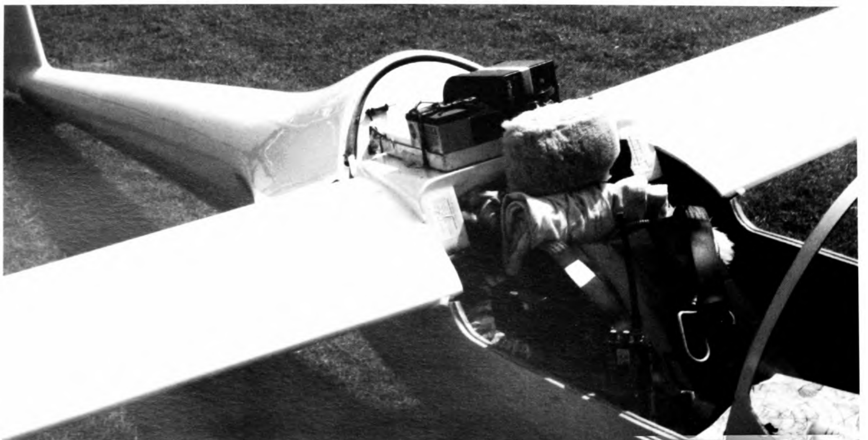
A Kestrel 19 showing the tray mounted over the wing roots to carry batteries and barograph. ( M. Simons )
