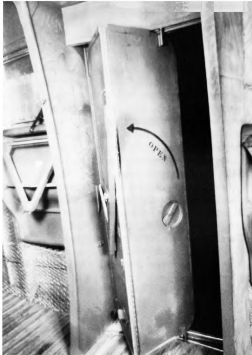
Folding doors for the paratroops to jump from. Note the seats folded away on either side. ( Slingsby collection )
