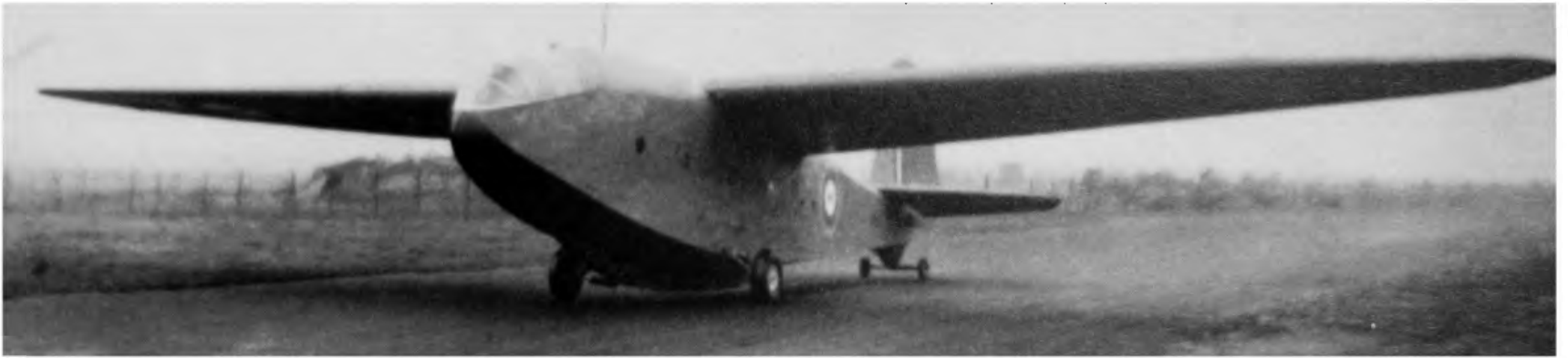
The Hengist prototype with rounded nose. The tail dolly was necessary to prevent the tail-skid overheating when dragged over the bitumen runway. ( Slingsby collection )
