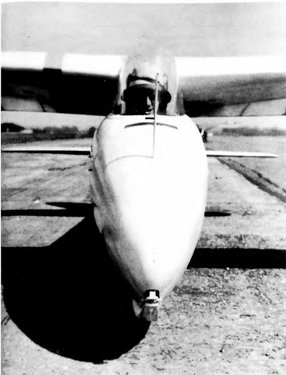
Philip Wills in the cockpit before going to the competitions in Switzerland. Note the thickening of the wing roots to allow a deeper spar, and the aero tow release just in front of the skid fitting. ( Wills collection )
