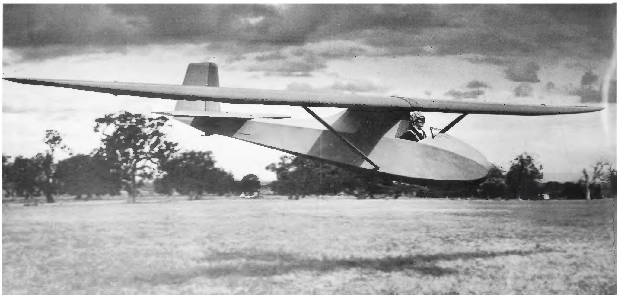
Typically, the Grunau Baby 2 was flown without any windscreen or cockpit canopy. This example is in Australia. (The Age, Melbourne)
