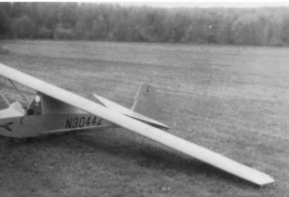
The UT-1, a Kadet built by Miller and Dawydoff in the USA. It was used for appraising the type as a trainer for military glider pilots. This aircraft, which still exists, has a straight-backed fuselage and tall rudder and no landing wheel, but the nose is of the later form. ( R. Smith )
