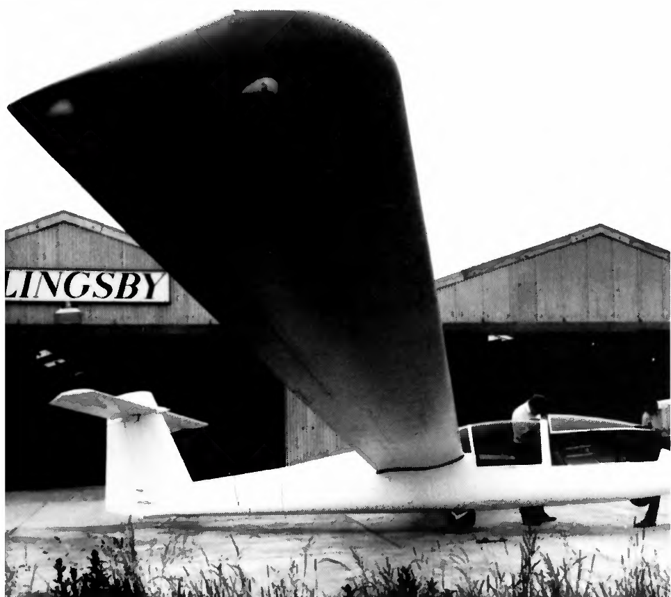
The interim T-53B/C demonstrator soon after completion of the alterations. The dorsal fin remains at this stage. Servotabs on the ailerons are just visible. (Vickers-Slingsby via G. Bailey-Woods)
