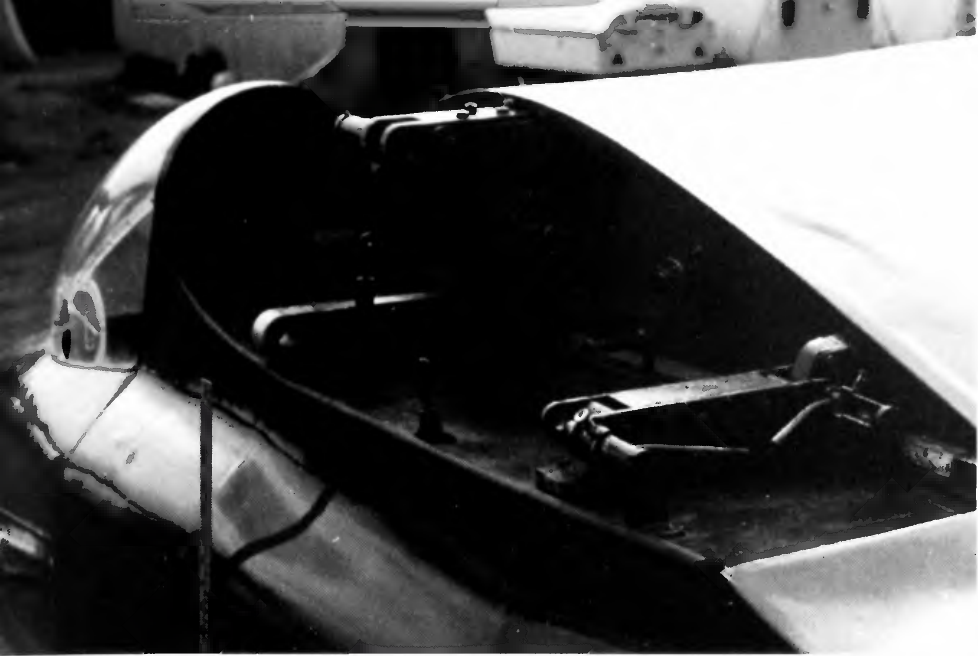
Rigging detail of the Sky. Two horizontal pins aligned on the same centre attach one wing to the fuselage. When the other wing is similarly attached the last pin is inserted to join the upper flanges of the main spars. Aileron and brake pushrods are linked with pip pins. (P. J. Teagle)
