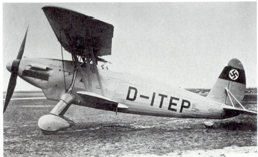
39: Port side view of the prototype Arado Ar 68e, D-ITEP, powered by the Jumo 210 engine. The later production Ar 68E briefly equipped the Luftwaffe's fighter squadrons in 1937, but was soon replaced by the superior Messerschmitt Bf 109. Subsequently the Ar 68E saw extensive service with the fighter-training schools (Bruce Robertson)
