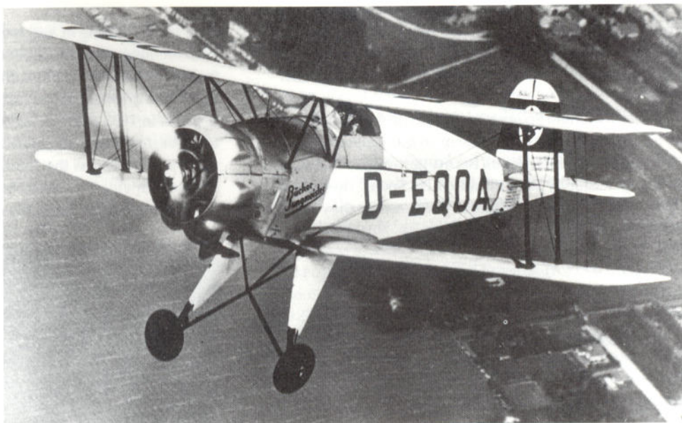
8: Bücker Bü 133C, D-EQOA, being flown by Rudolf Lochner, the 1937 German Aerobatic Champion during a demonstration over the Rangsdorf Lake in 1937. The aircraft is finished in the early standard factory finish of pearl white paint on all wood and fabric surfaces, with silver-finished metal panels and engine cowling (Bruce Robertson)
