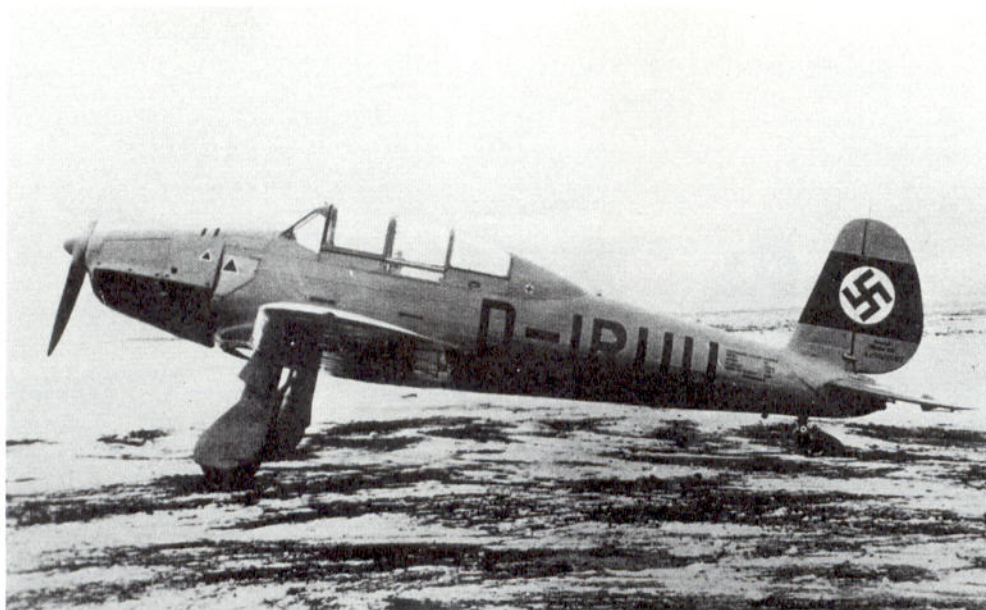
47: Side view of the first prototype Arado Ar 96, D-IRUU, after it had had the undercarriage, fin, rudder and cockpit canopies modified to early production standard (Bruce Robertson)
