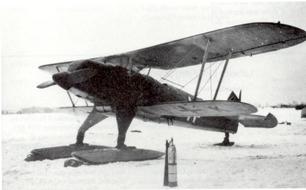
56: An highly unusual picture of an Heinkel He 51 fighter-trainer wearing enormous skis. The underwing code appears to be H?+IK, and the oversized swastika just visible on the fin suggests that the date may be winter 1939-40. The location is unknown (AMC)
