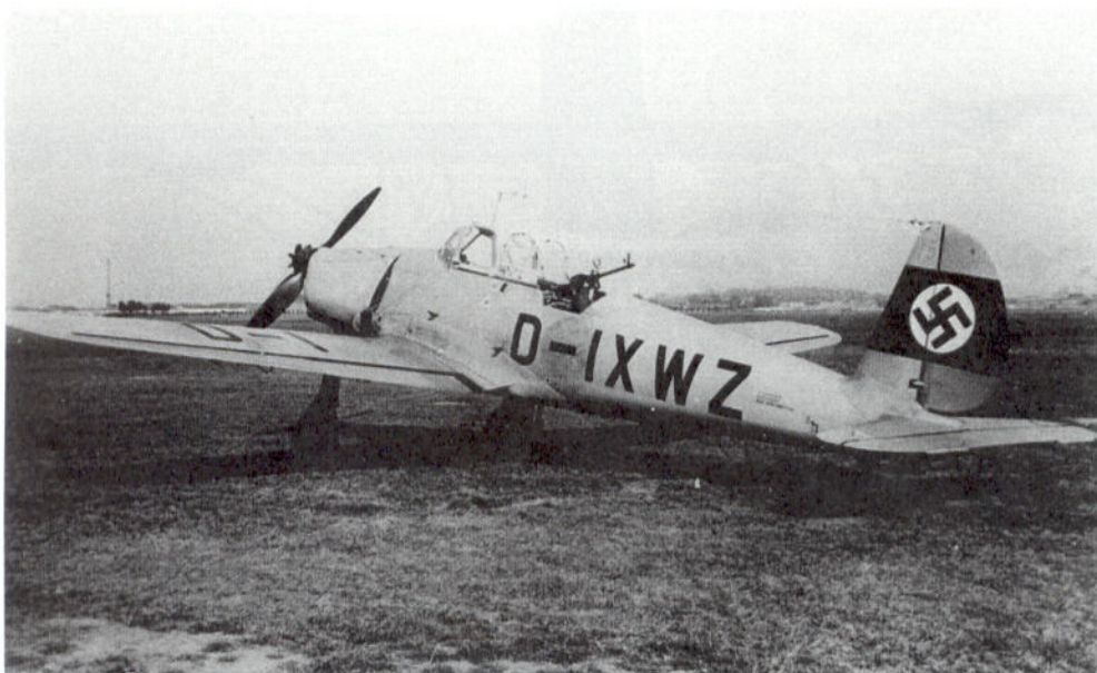
48: D-IXWZ was the Arado Ar 96 V9, fitted with a rear gunner's position in accordance with a Bulgarian requirement. This was the only aircraft so fitted (Bruce Robertson)
