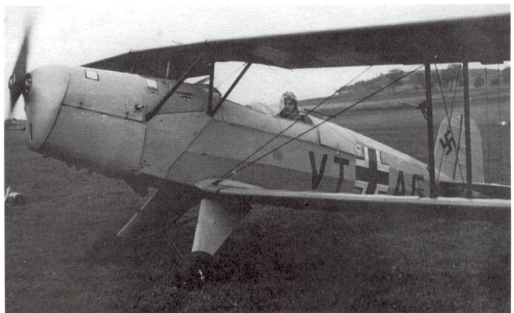
4: Unidentified Luftwaffe flight student running up the engine of RLM Grau 02 finished Bücker Bü 131, VT+AE or F, prior to a flight. Note the Bücker trademark between the cabane struts
