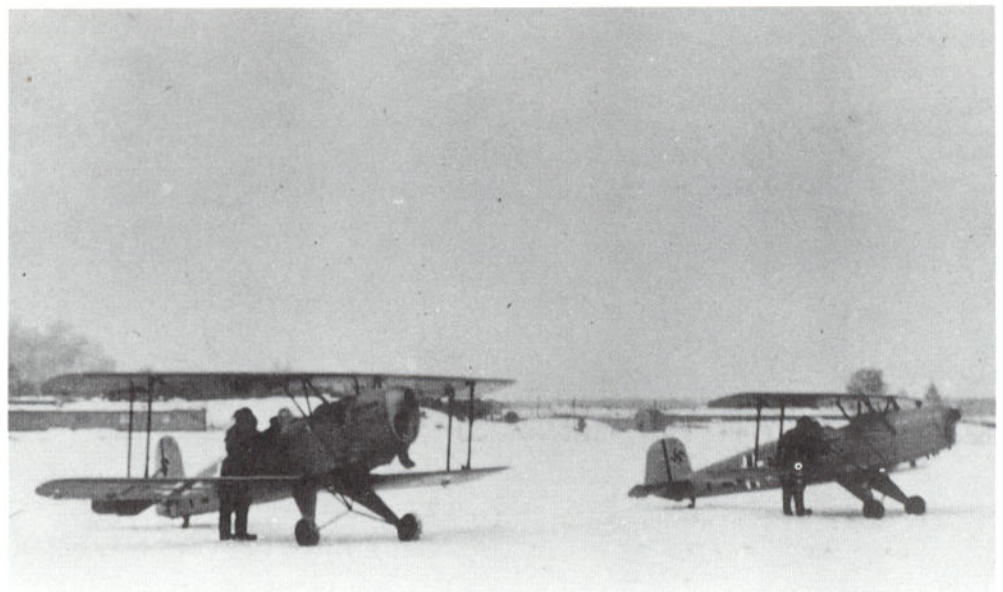
3: Brrrr! Training carried on whatever the weather. Two overall RLM 02 Grau Bücker Bü 131 trainers warming up their engines on a snow-covered Luftwaffe training base. Both aircraft appear to carry codes beginning PE+??. Location maybe in Czechoslovakia in winter 1939-40. Note that the machine on the left has the early style extended cranked engine exhaust
