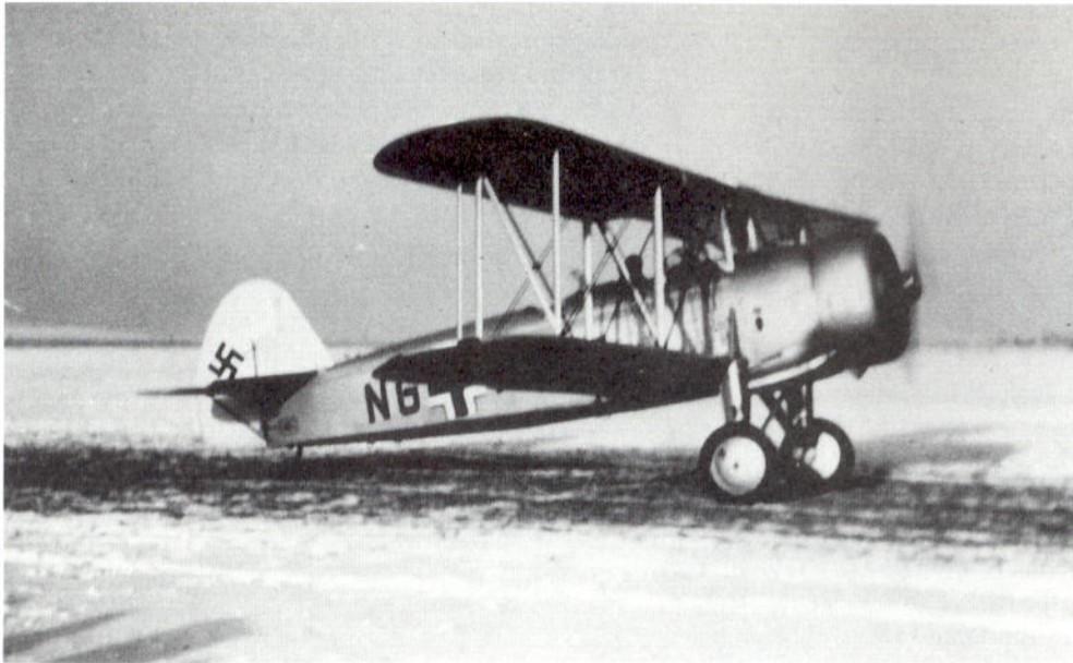
28: Following the occupation of Czechoslovakia, many Czech aircraft were used by the the Luftwaffe as trainers. Seen here on a snow-covered airfield is one of the rarest, a Praga E-241. This was a purpose-built trainer, powered by a Walter 'Pollux' radial engine. The prototype first flew in 1936 and 92 were in service with the Czech training schools at the time of the German occupation. Wearing an all-silver finish, NG+??, is in service with an unknown Luftwaffe training school, probably in winter 1939-40
