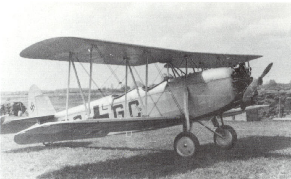
30: Very clear shot of an all-silver Letov (Praga) E-39, a Czech aircraft used extensively for training by the Luftwaffe. Coded ??+GC. The machine is believed to be in service with the Fliegerschule attached to Flieger Ausbildung Regiment 33 based at Elbing in early summer 1940 (AMC)
