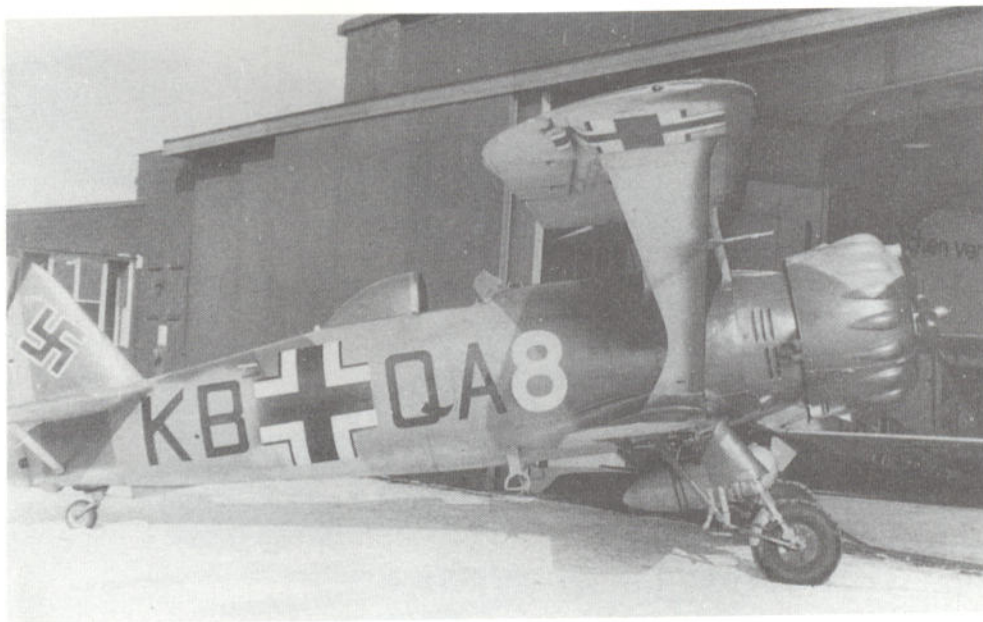
83: Henschel Hs 123, Werk Nummer 2732, KB+QA, white '8', in service with an unidentified Stuka Vorschule. As was common in the winter months, the wheel spats have been removed to avoid clogging with mud. The machine retains its original three tone upper surface camouflage (RLM 61/62/63). Note the feather edged finish to the dark green paint on the strut leading edge
