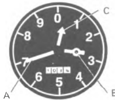
Fig 1.10 The altimeter. The altimeter indicates the glider’s height.
