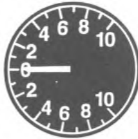
Fig 1.9 The variometer. The variometer indicates the glider’s rate of climb or descent.
