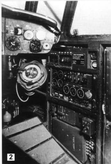
1. The quite narrow, 'single pilot' cockpit of the Do 217 was not untypical in German bombers, few of which boasted dual controls although the aircraft could however be flown by the observer in an emergency. The master compass is on the right below the instrument panel. (via Griehl). 2. On the right side of the Do 217E cockpit behind the compass in its angled housing was the main instrument panel with engine, temperature and pressure gauges clearly displayed. (Dornier via Griehl) 3. Potentially much more useful on the Do 217 from the combat point of view was to substitute the dive brakes with some extreme tail defence. Dornier devised a four-gun tail 'stinger' consisting of twin 81Z combinations which could be fitted in place of the long tail brake housing. 4. Having worked hard to comply with an official edict to incorporate an effective dive brake on the Do 217, Dornier developed two types. Neither proved ideal for such a heavy aircraft although this Perlon parachute brake could be used to kill speed in flight or during a fast landing.
