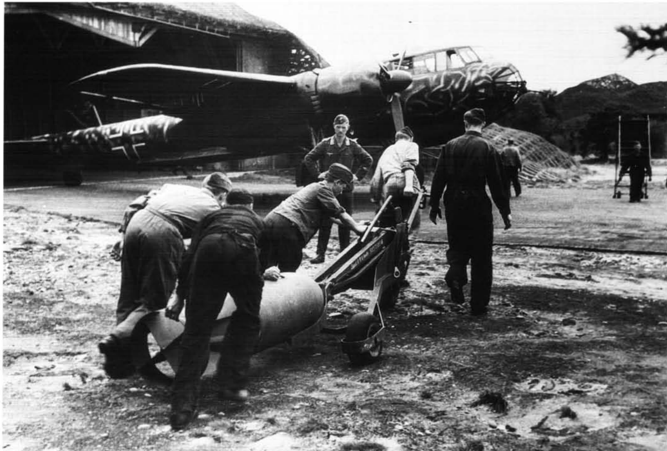
All hands to the bomb trolley as the groundcrew move an SC 500 bomb out to the hardstanding and a waiting Do 217E-4 of 5./KG 6 in a 'wave mirror' pattern camouflage scheme. The aircraft (3E+EN) is fitted with FuG 217 Neptun R early warning radar, as indicated by the set of four rod aerials under the starboard wing. (Bundesarchiv)
