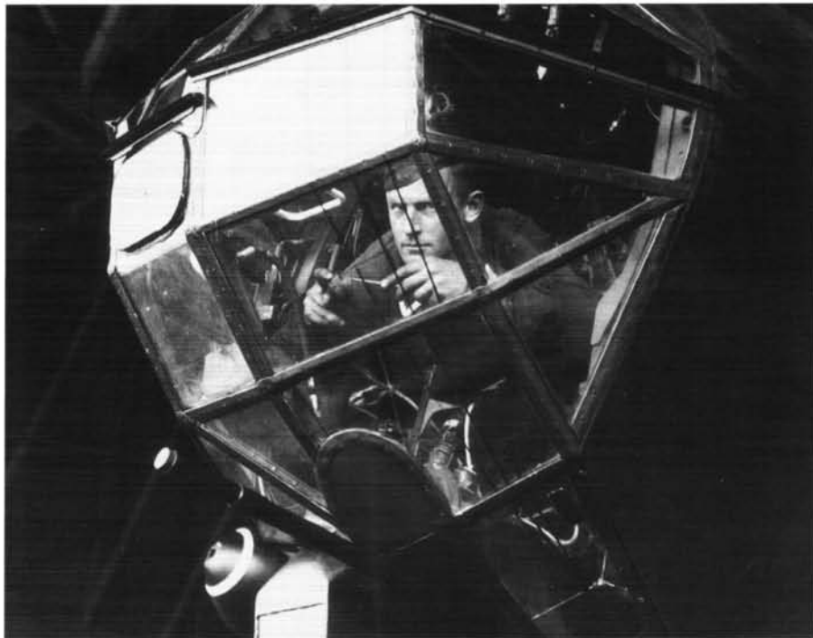
A Luftwaffe 'black man' working in the nose of a Do 217E-2/R5 sceptically eyes the camera poked his way. The optically flat perspex panels, including a blanked-off cannon port at top right, were designed to reduce distortion during the bombing run. The long barrel of the MK 101 cannon is to the right of the Lofte 7D sight. (Bundesarchiv)
