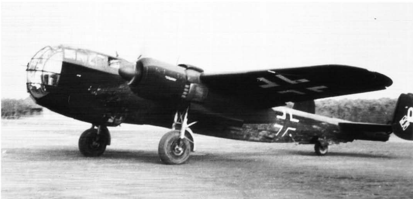
Above: The increased-span wing of the Do 217K-2 offset the weight of the Hs 293 and Fritz X remotely controlled bombs, the weapons that arguably gave the type its greatest claim to fame. W. Nr. 4572 has the RF2C remote sighting periscope in the cockpit roof. (Dornier) Below: Despite a universal use of mainwheel mudguards Dornier bombers had their rear fuselage paintwork regularly spattered by mud and dust kicked up by the tyres. To prevent equipment malfunction groundcrews cleaned delicate areas such as the FuG 10 radio aerial on the port side. Do 217K coded 'Q' of KG 2 is shown. (Bundesarchiv)
