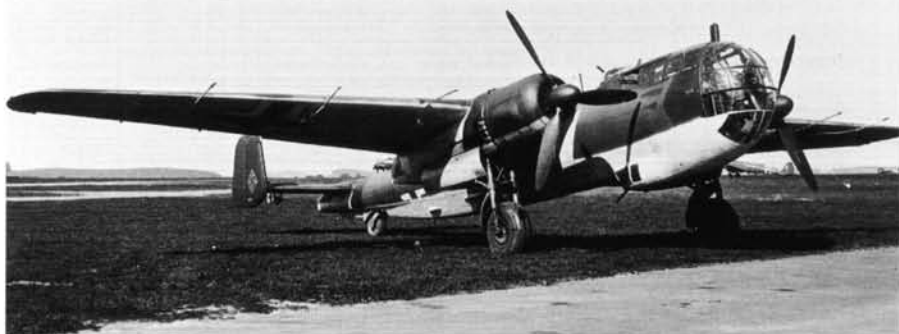
Above: The increased-span wing of the Do 217K-2 offset the weight of the Hs 293 and Fritz X remotely controlled bombs, the weapons that arguably gave the type its greatest claim to fame. W. Nr. 4572 has the RF2C remote sighting periscope in the cockpit roof. (Dornier) Below: Despite a universal use of mainwheel mudguards Dornier bombers had their rear fuselage paintwork regularly spattered by mud and dust kicked up by the tyres. To prevent equipment malfunction groundcrews cleaned delicate areas such as the FuG 10 radio aerial on the port side. Do 217K coded 'Q' of KG 2 is shown. (Bundesarchiv)
