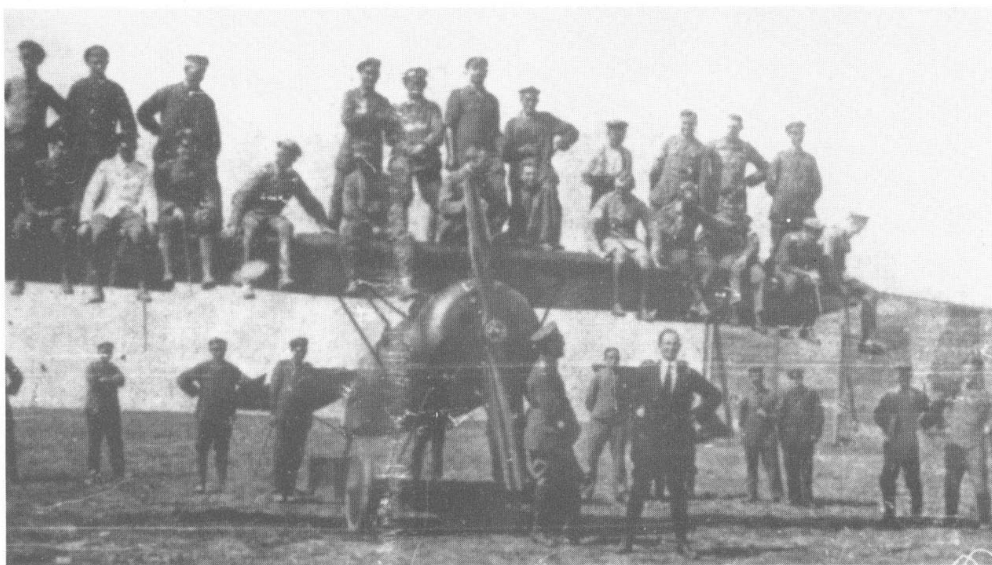
(Right) Anthony Fokker standing defiantly in front of an E.V on Jasta 19's aerodrome while twenty-four of the unit's personnel are used to demonstrate the wing's strength. This photo was taken on 23 August 1918 when Fokker attended the crash commission's report on E.V wing failures. Cross and Cockade International
