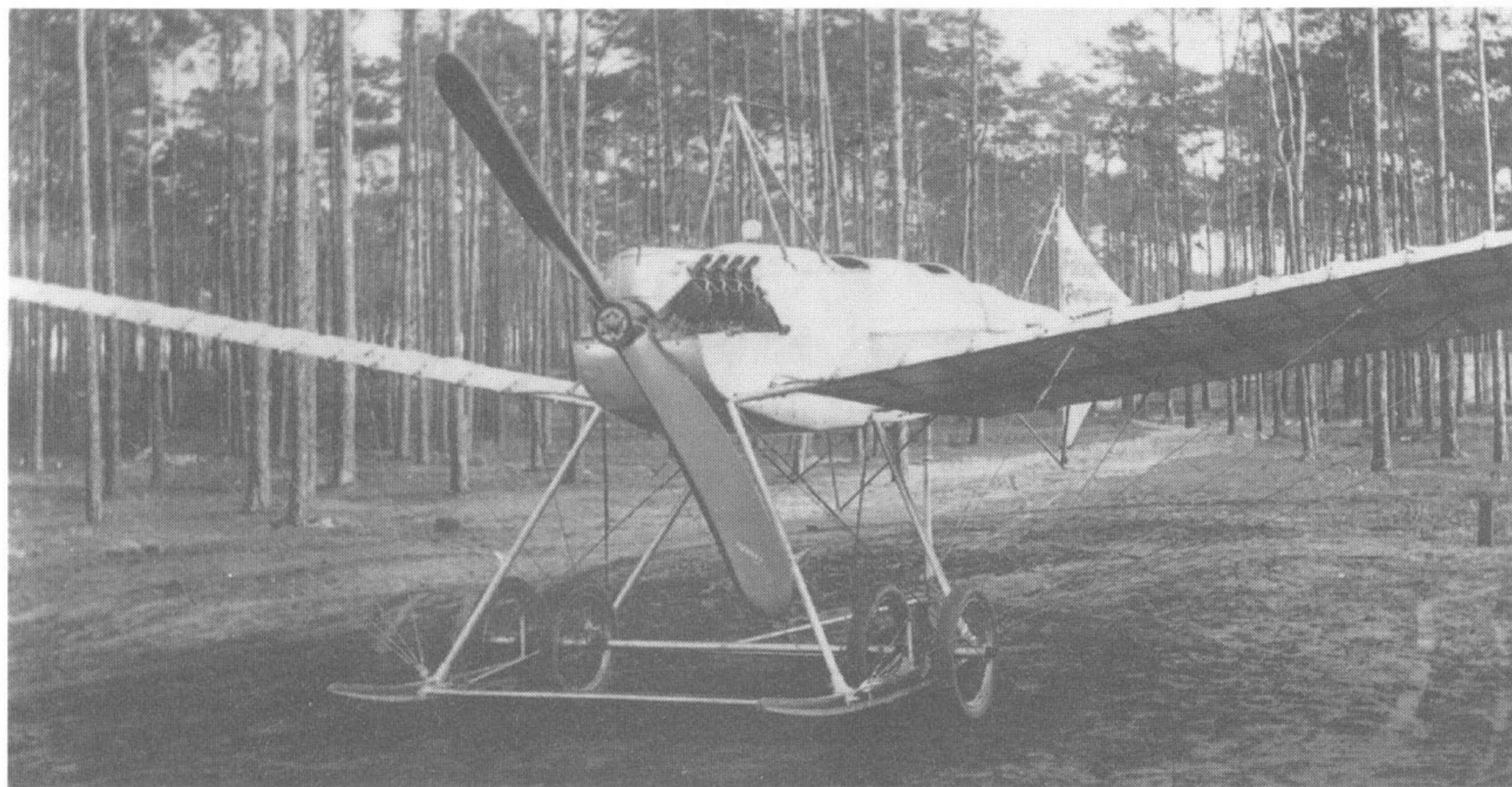
The third variant of the Spinne III in 1911, fitted with a 70hp Renault engine. Frank Cheeseman
