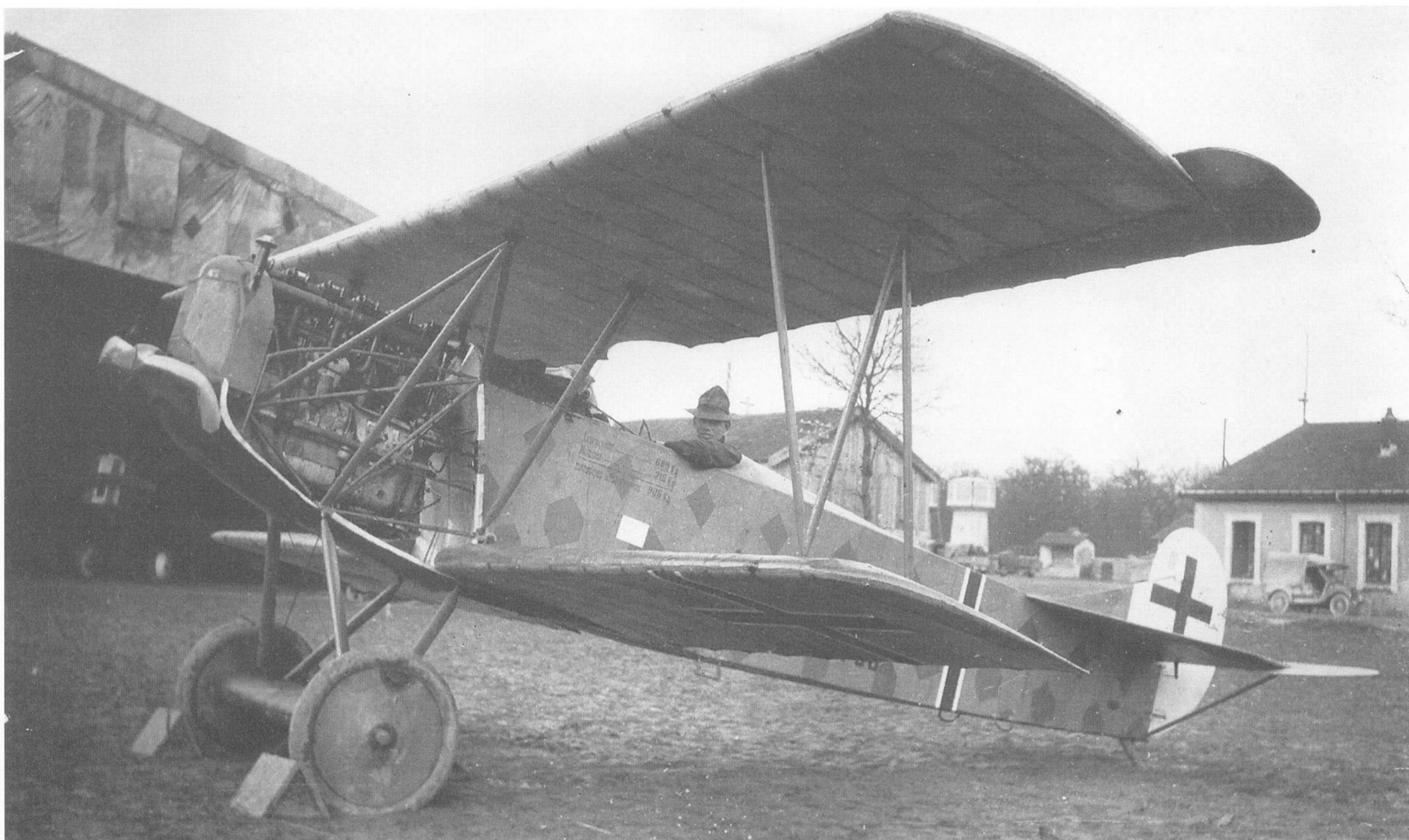
(Below) 185hp BMW IIIa-engined Fokker D.VIIF 7788/18 received by the Americans in Koblenz on 2 January 1919. Greg Van Wyngarden
