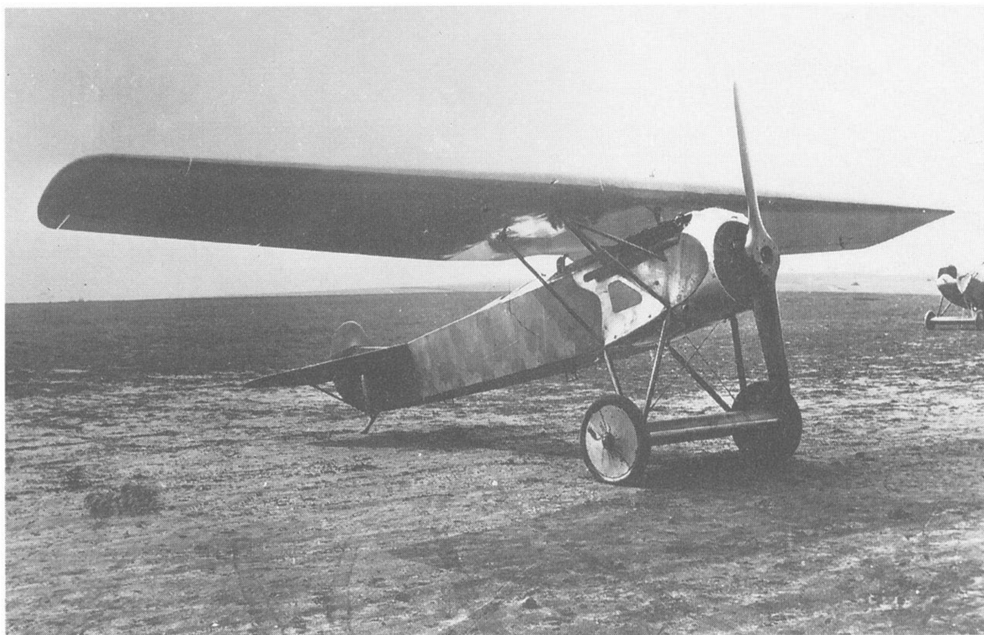
Fokker V.27 fitted with a 195hp Benz Bz.IIIb water-cooled engine. Cross and Cockade International
