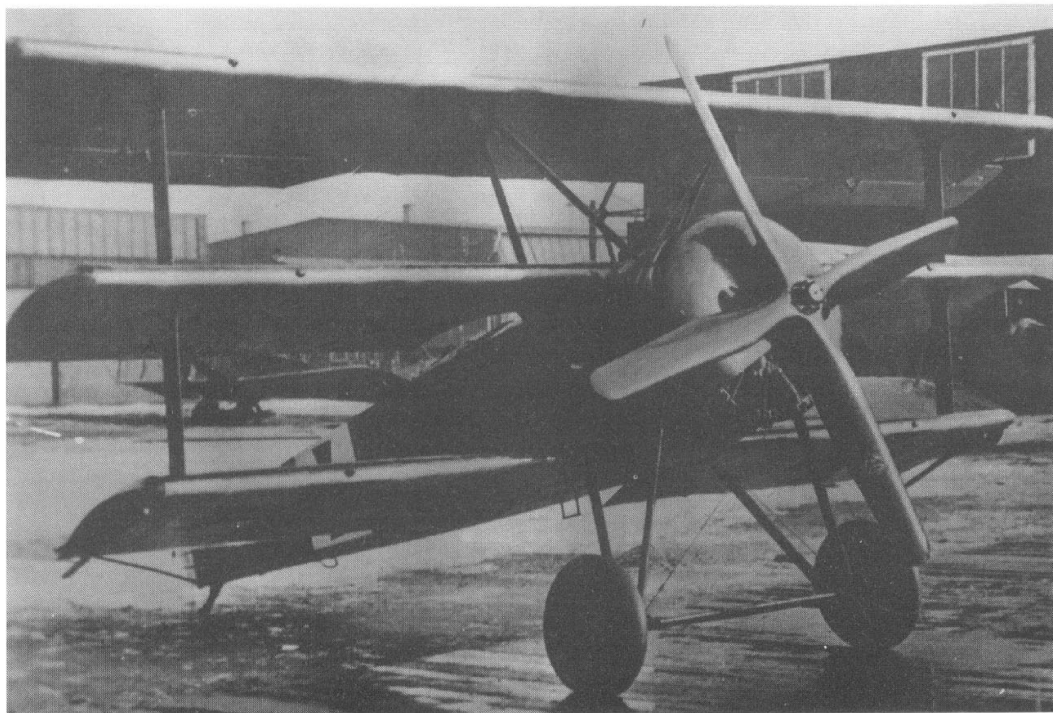
The complete V.7 with its large four-bladed propeller and 'tall' undercarriage.
