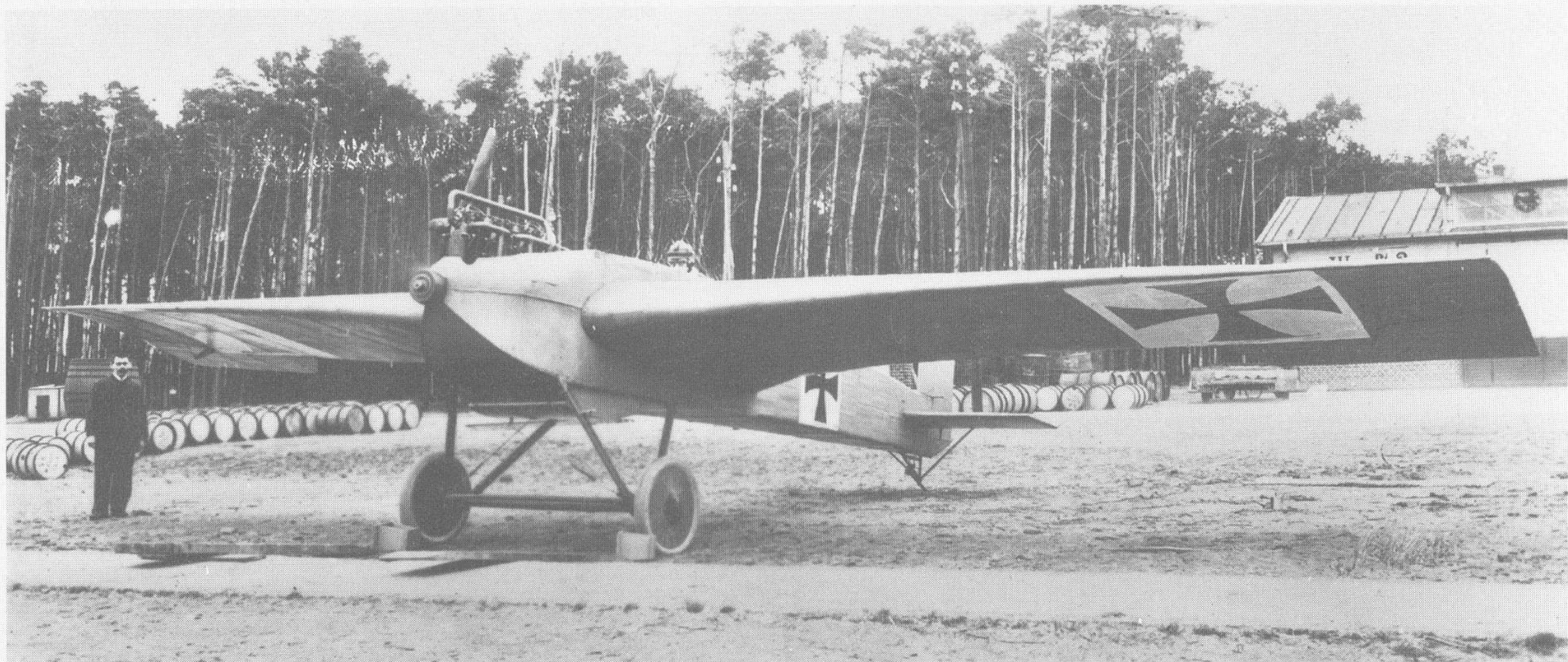
(Above) The original all-steel Junkers J.1 monoplane of 1915. Cross and Cockade International
