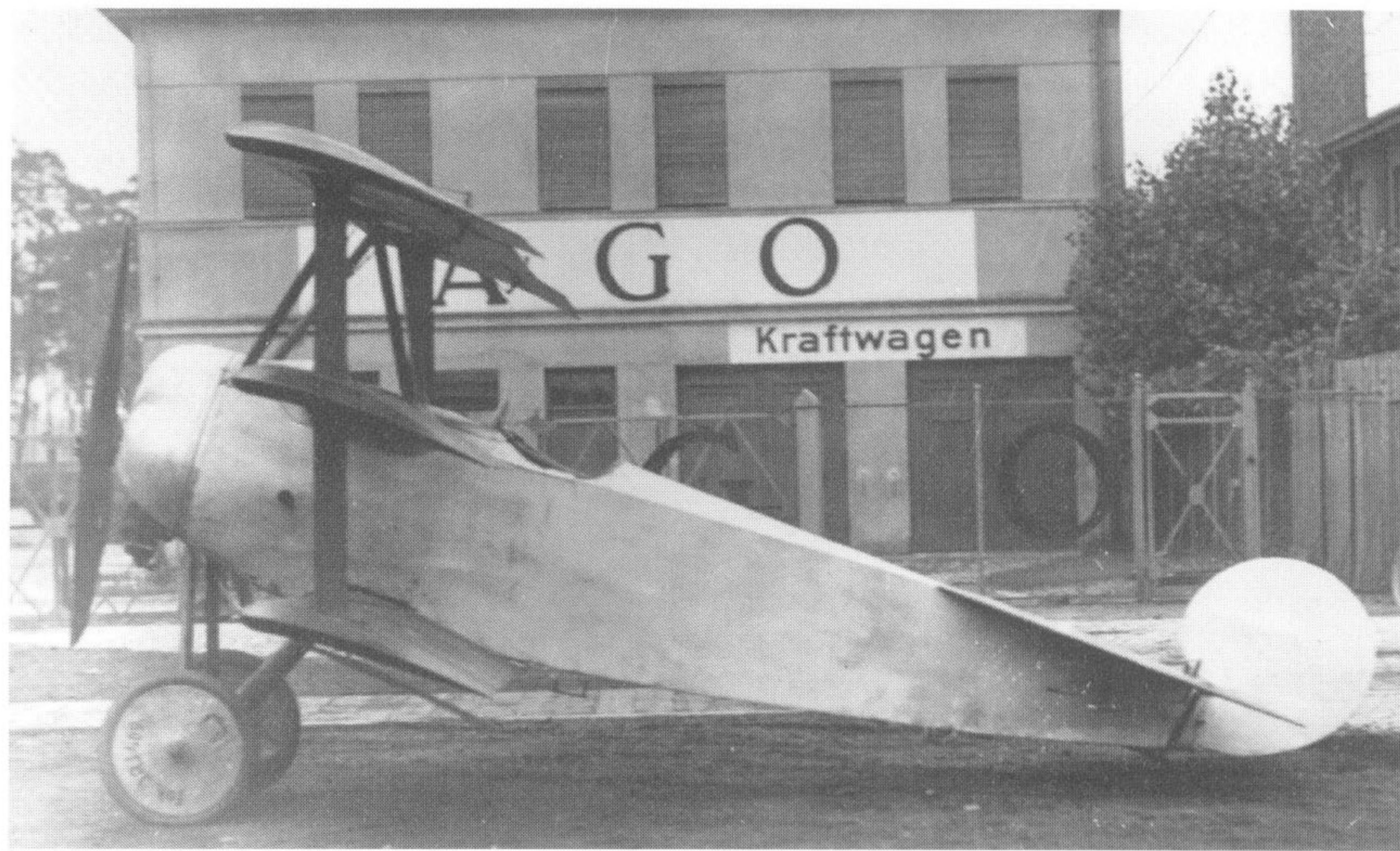
Fokker Dr.I 469/17 (factory number 2095) fitted with an Oberursal UR.II engine at the Fighter Competition. Peter Grosz
