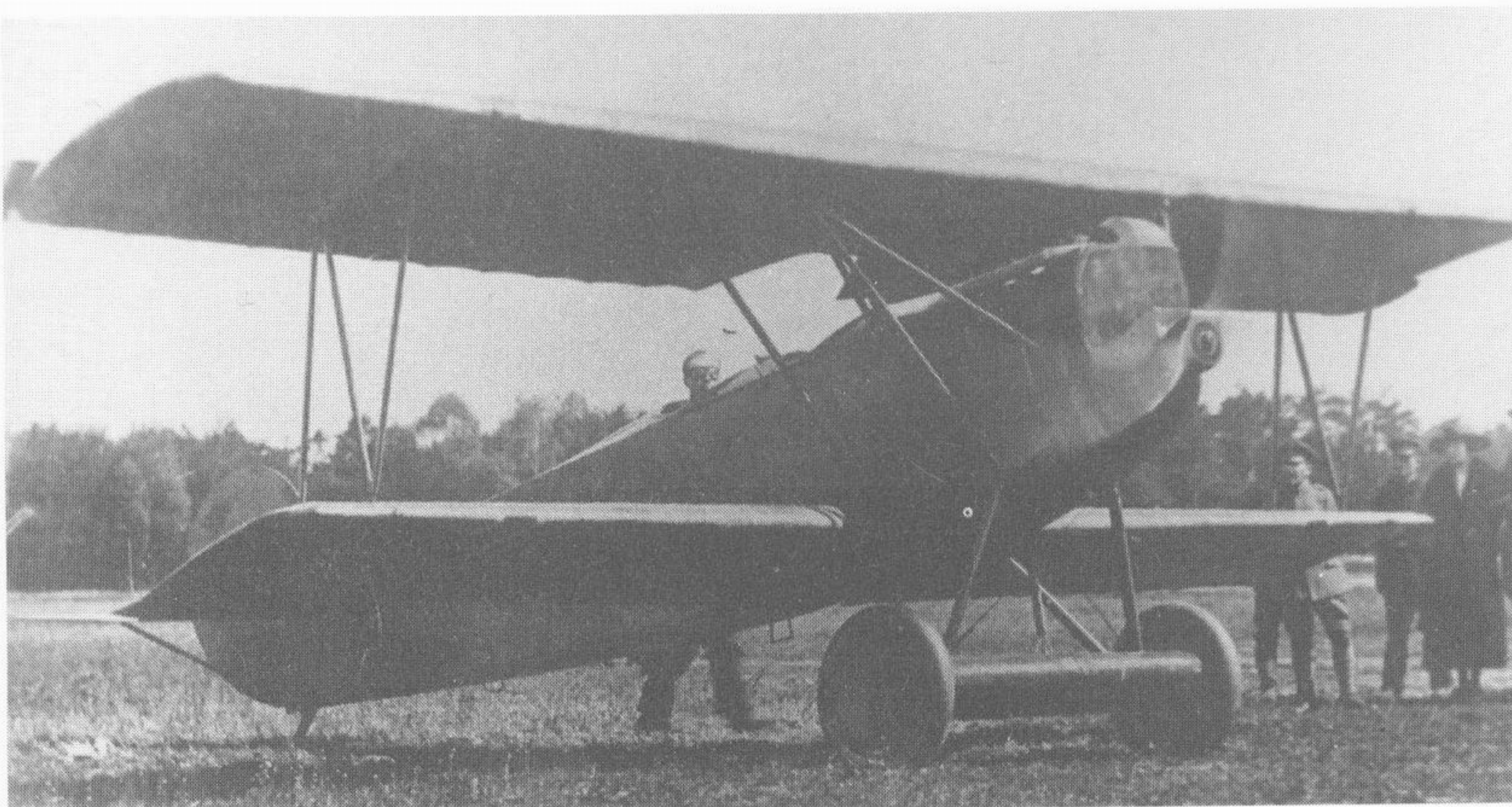
V.35, a two-seat version of the D.VII with a fuel tank in its undercarriage sub-wing. The pilot in this instance is Ernst Udet. Cross and Cockade International
