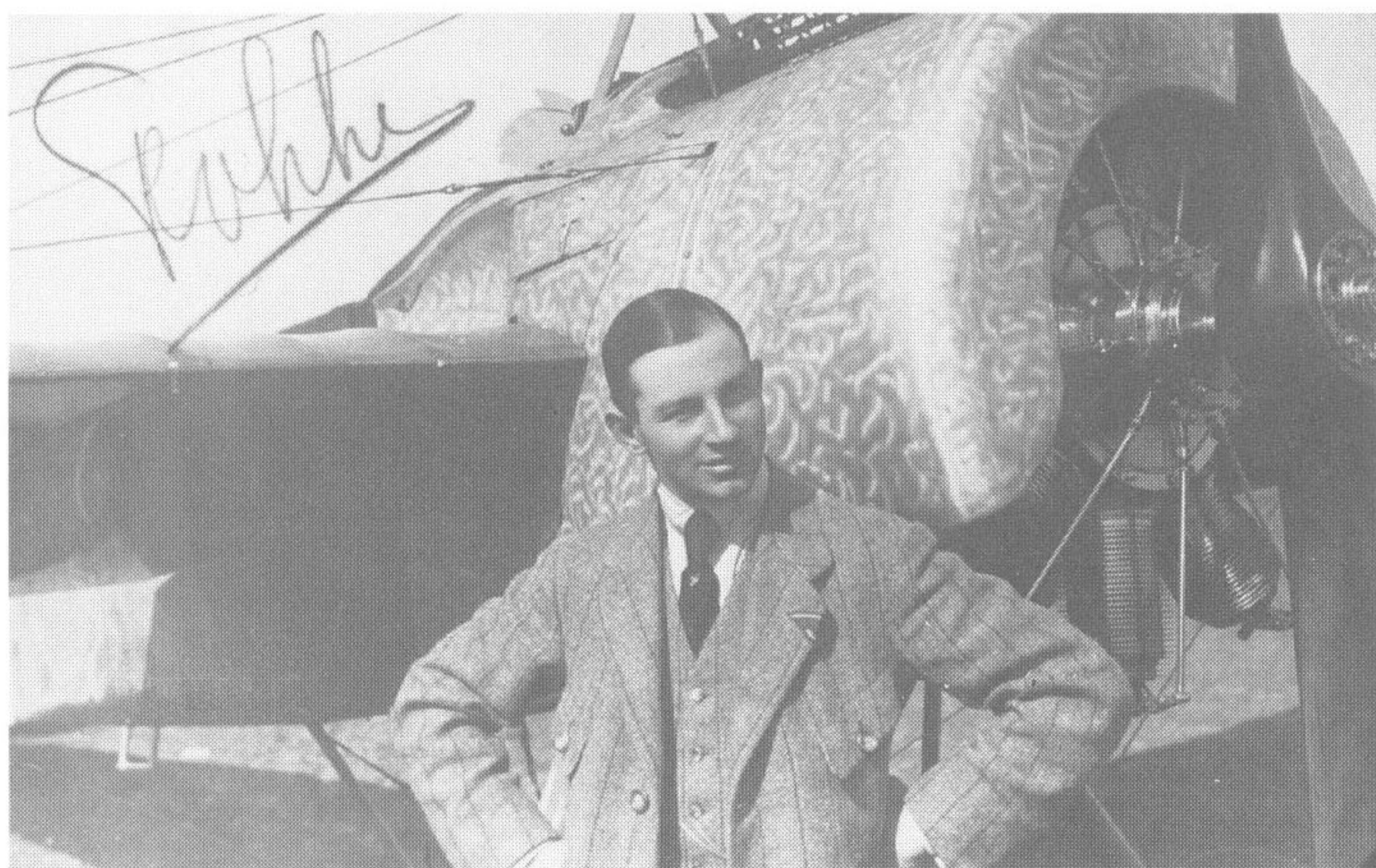
Anthony Fokker poses in front of the machine-turned cowling of an E.III. Frank Cheeseman
