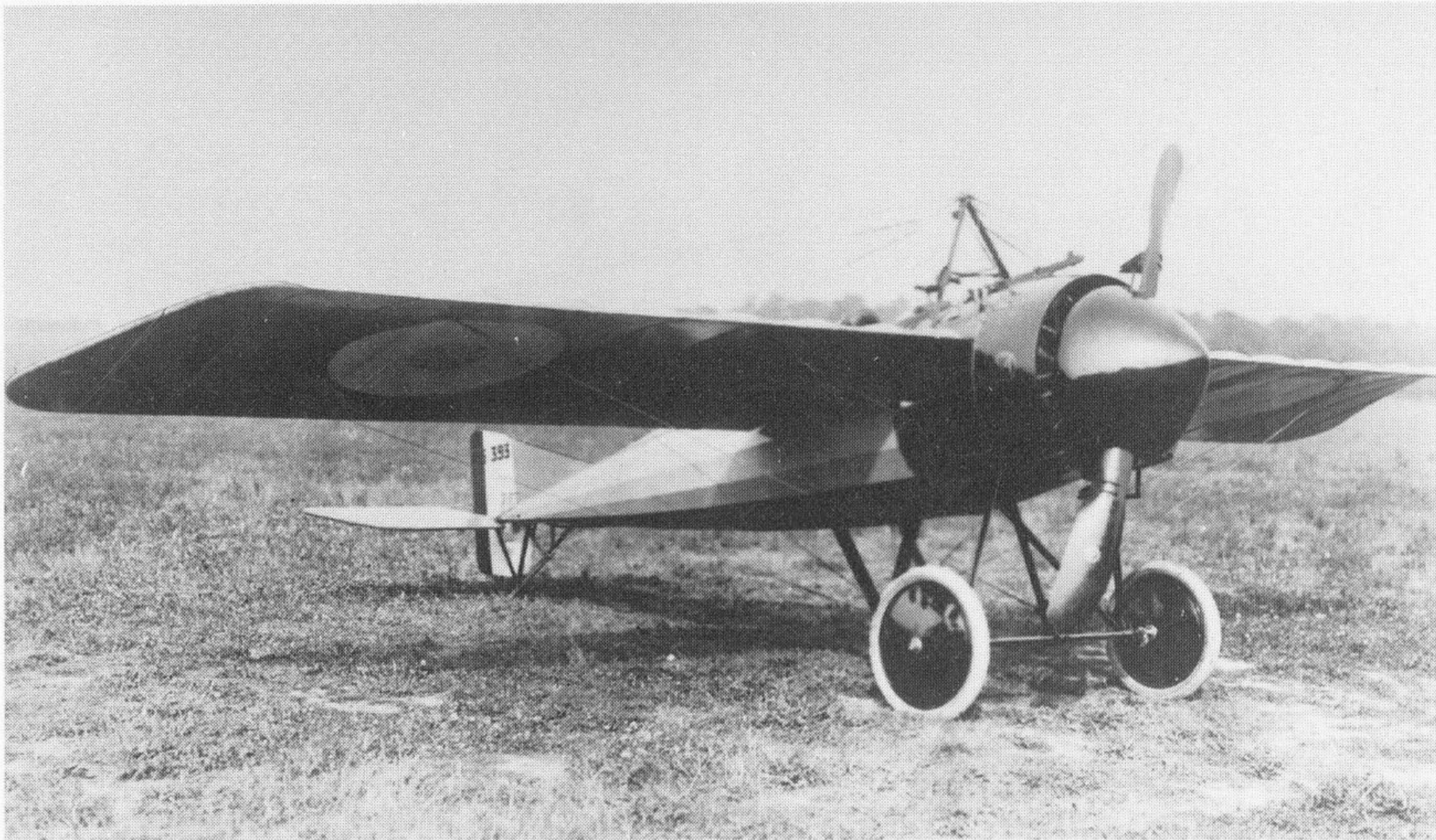
A French Morane-Saulnier Type N fitted with steel wedges to protect its propeller from bullets.
