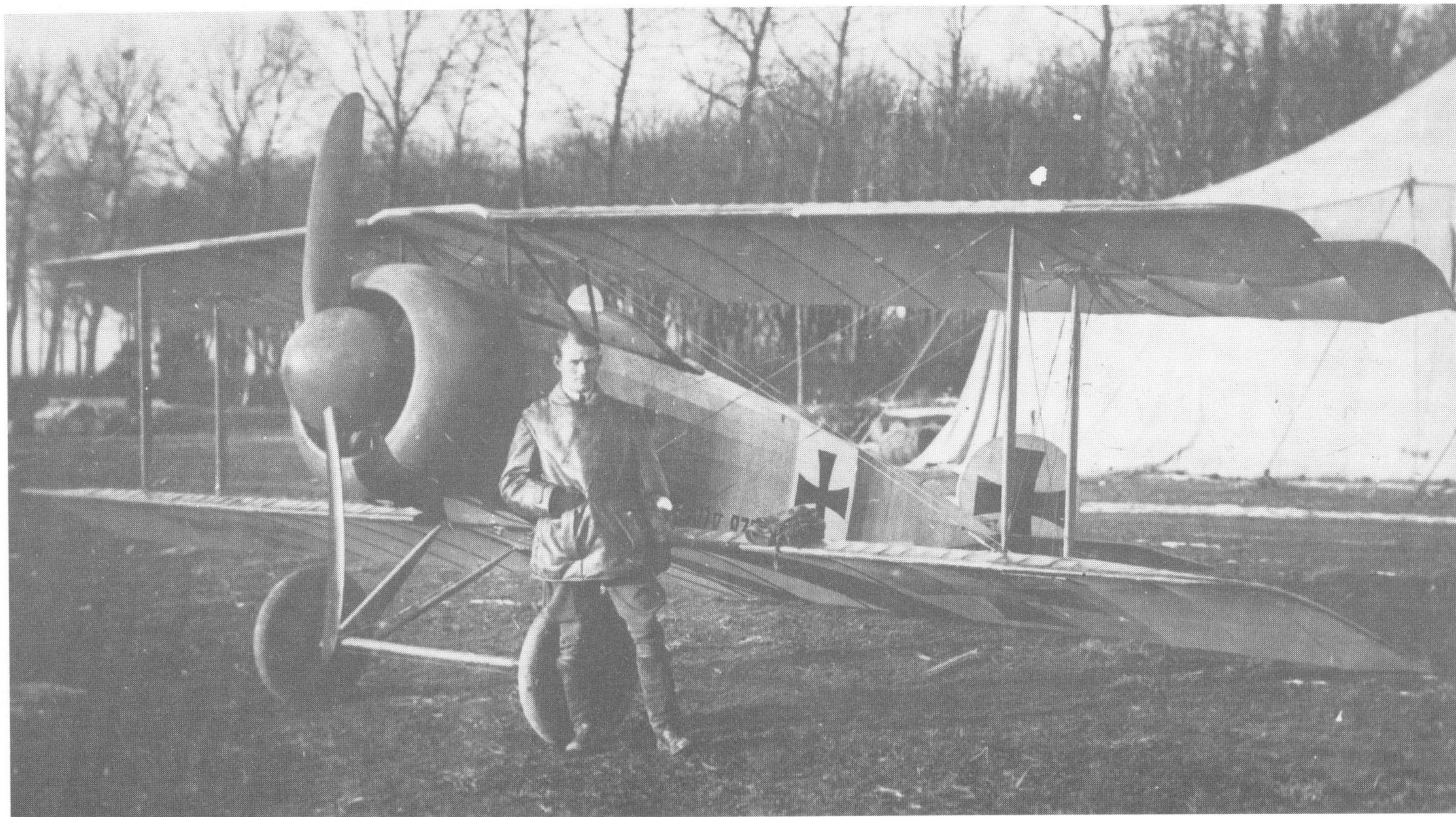
Fokker D.V of the 2700/16 series. This is a training aircraft and was probably used at either an Armees Flug Park or with a Jasta to familiarize pilots with rotary engines prior to their equipment with Dr.I triplanes. Greg Van Wyngarden
