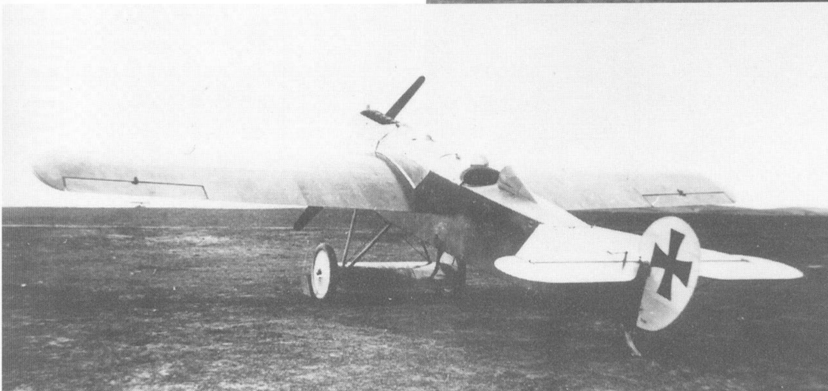
(Top) Fokker V.23 fitted with a 160hp Mercedes D.IIIa water-cooled engine. Cross and Cockade International
