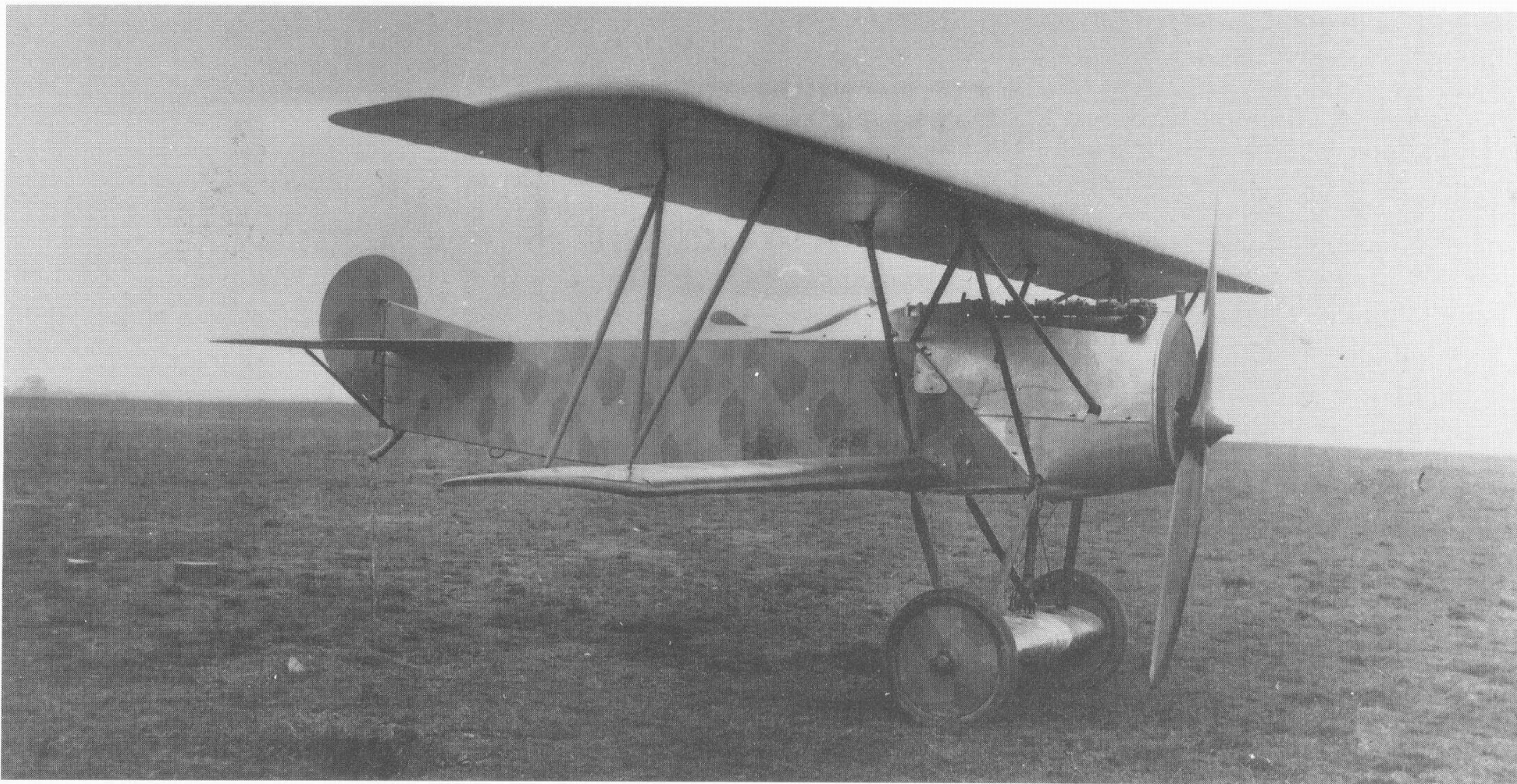
Fokker V.36 with a fuel tank on its undercarriage sub-wing. Harry Woodman
