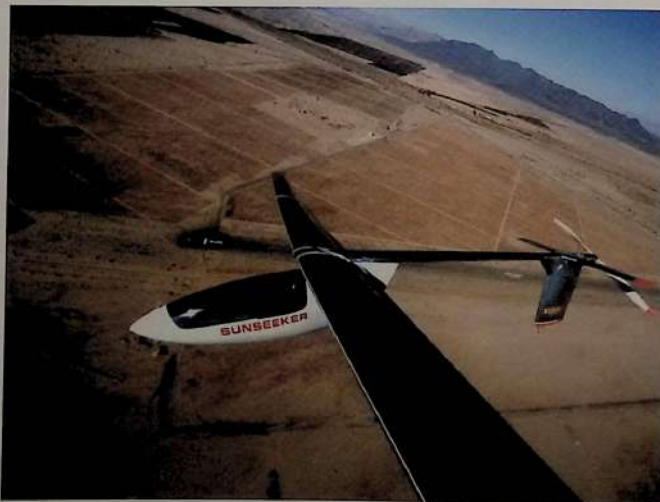
The Sunseeker wing and tailplane totally covered with photo-voltaic solar cells
