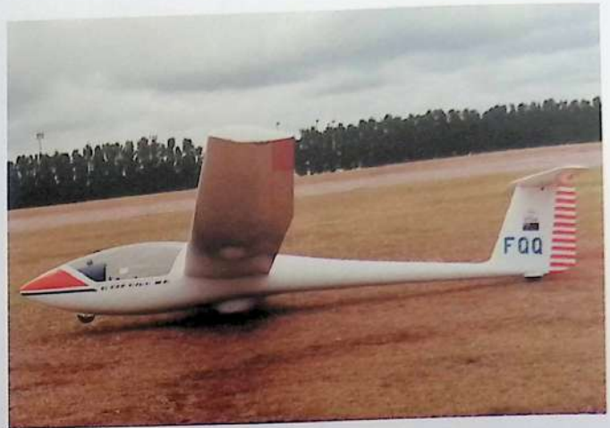
Above: The later Astir Club III B with new fuselage and cockpit, which some pilots found uncomfortable
