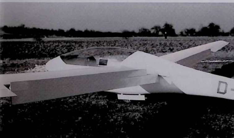
Middle: Mosquito showing the combined flap airbrakes
