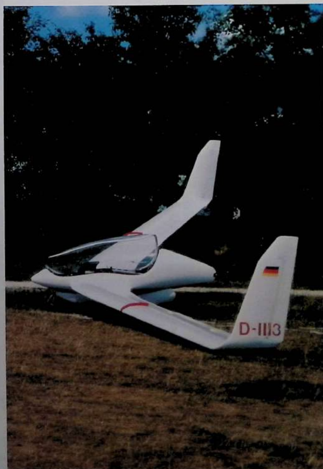
An unusual attempt to advance sailplane design: tailless SB 13 "Arcus" (Photo Jochen Ewald)
