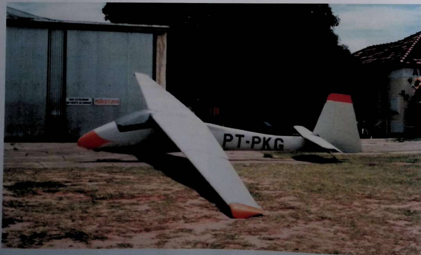
The KW - 1 B2 Quero Quero, later called the IPE - 01 became a useful club sailplane
