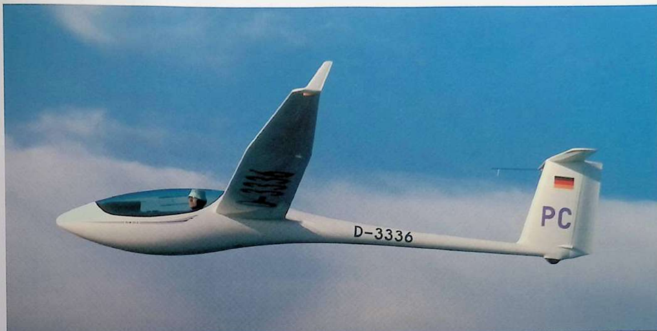
Waibel's design of 1980 for the Standard Class, the ASW 24. Special attention was given to the cockpit strength and pilot protection in bad landings. (Photos Manfred Münch)
