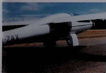
Above: The nose cone moves forward to free the propeller. The drive shaft from the engine buried in the fuselage, passes between the seats. The pilots here are Harry Schneider and Noel Roediger, at Gawler, S Australia.
