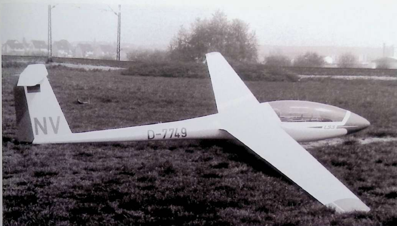
With a more orthodox arrangement of flaps and ailerons, the LS 3A was considerably lighter than the earlier version. The vertical tail area was also increased.
