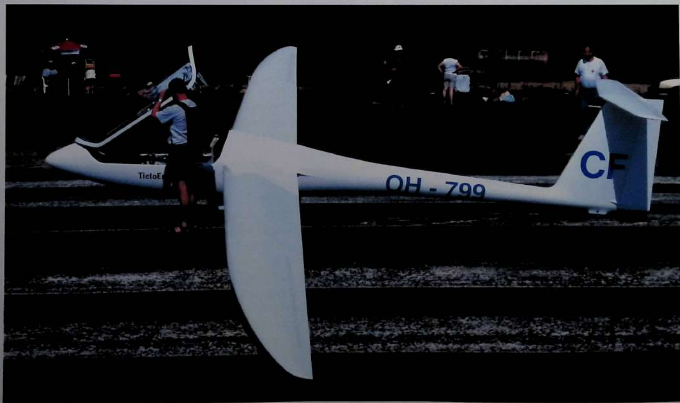
The SZD 55, Poland's very successful Standard Class challenger for the SH Discus. Note the curved taper of the wing. (Photo Jochen Ewald)
