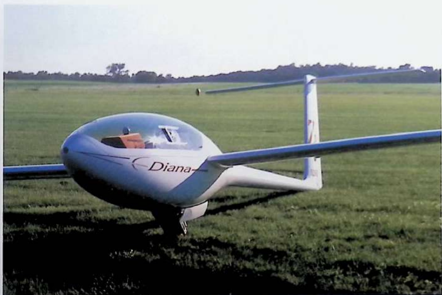
The SZD 56 'Diana' showing the unusually thin wing and narrow tail boom. It was claimed that this was technologically the most advanced sailplane in the world.
