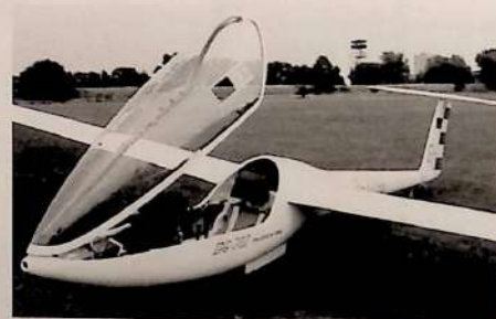
The DG-202 17 metre span with carbon fibre spar
