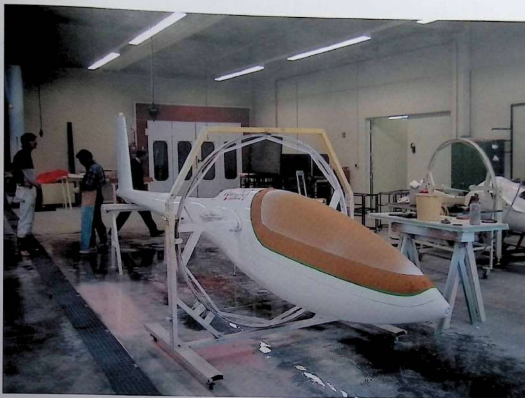
After moulding there is still a lot of work to do. Finishing the surfaces and fitting canopies requires hours of sanding by hand.
