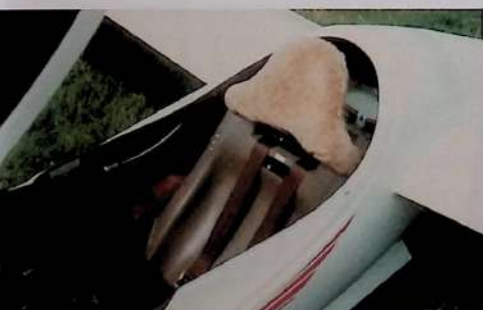
Waibel's design of 1980 for the Standard Class, the ASW 24. Special attention was given to the cockpit strength and pilot protection in bad landings. (Photos Manfred Münch)
