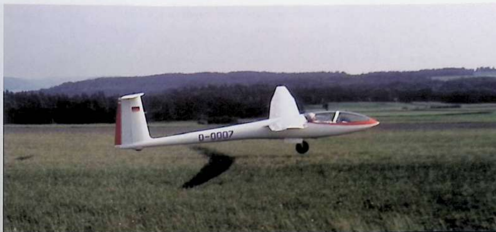
Supreme in the air, winning numerous national and world records, launching the ASW 12 was straightforward but if the brake parachute did not work, landing was a serious problem. (Photo Adolph Wilsch)
