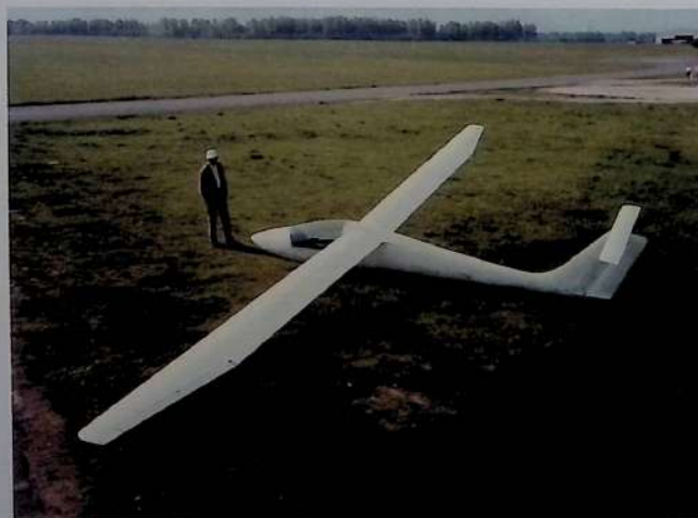
The Morelli M 300 was designed to demonstrate the effective use of alloy extrusions
