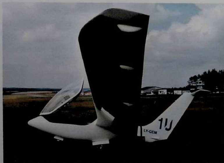
Genesis on the ground showing its special wing - fuselage arrangement (Photo Jochen Ewald)
