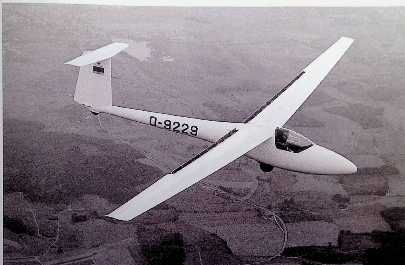
H 205 Club Libelle showing the airbrakes deployed
