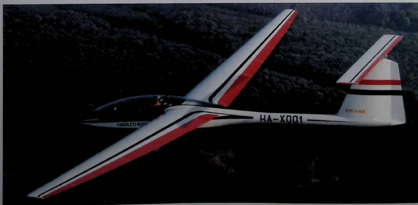
KM 400 in flight 1983. Mihaly Kesselyak's unusual sailplane design had no movable elevator, only a fixed tailplane. Longitudinal control was achieved by setting the flaps. (Photo Dr. László Széll, provided by Gábor Fekets)
