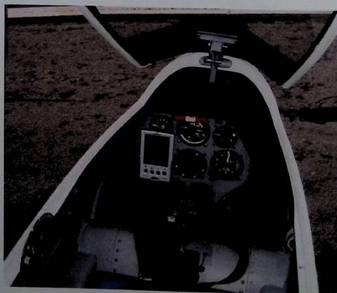
HP - 18 cockpit with instrument panel and canopy hinged in front
