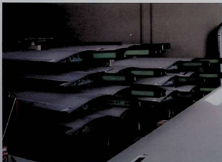
Stored wings awaiting rough edges to be cleaned up, before assembling with fuselages
