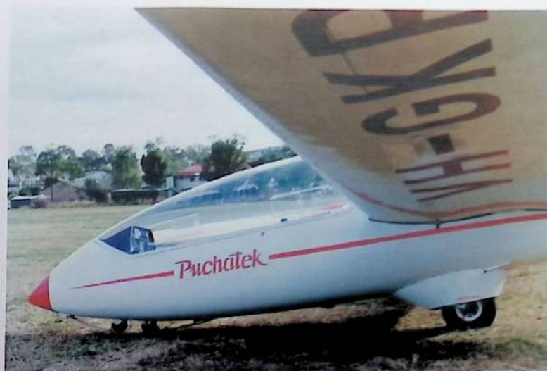
The Puchatek rests on the nose skid even when empty
