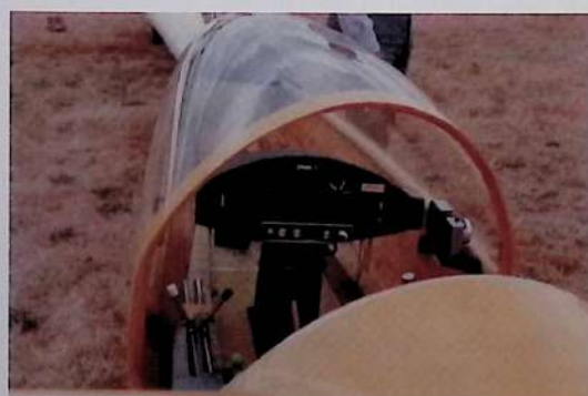
Above: Gary Sunderland's Moba 2 showing the sliding nose cone partly open
