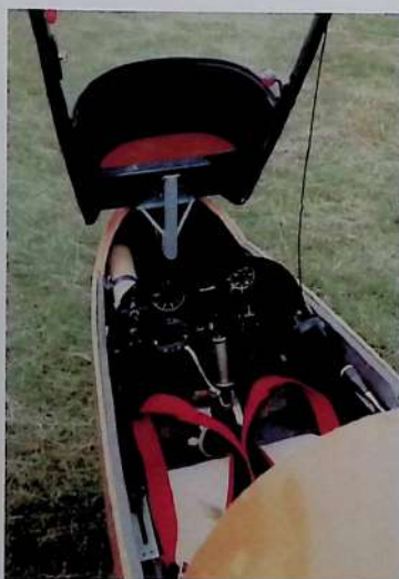
Right Above: Elfe S 4 during assembly. The photograph shows the wing spar joint but the main pins are not yet in place and the 'hotelier' coupling for the control is not yet connected.
