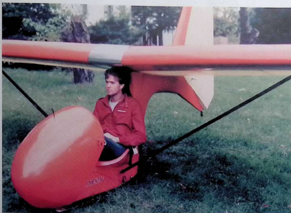
The Monarch E. Note the tow release at the side of the nacelle, and the control cable running round the pulley and into the wing
