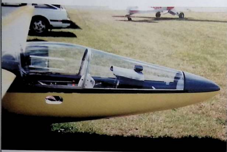
HP - 14 cockpit. The front part of the canopy was a simple curved piece of Plexiglas. The rear section was moulded and supplied with the kit.
