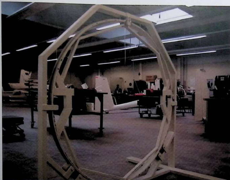
Large rotating frames help with turning fuselages over.
