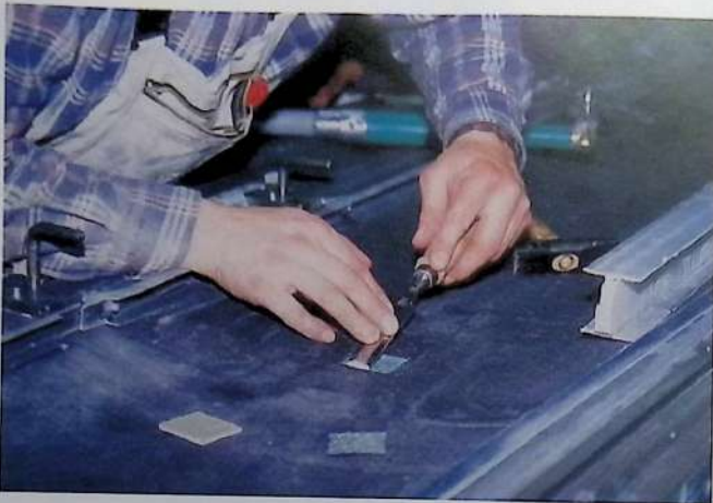
Before upper and lower skins are joined, control rods, ballast tanks, etc. have to be built in
