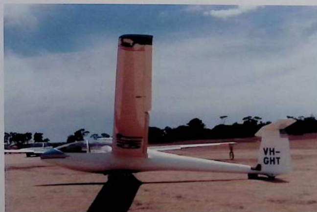
H 206 Hornet Standard Class sailplane with the same wing as the Club Libelle but an improved fuselage with retracting wheel
