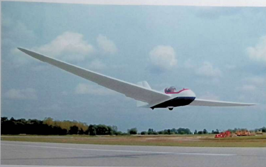
Pioneer 2D, with the span extended to 15 metres
