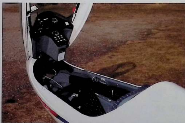
Above: The Instrument panel is raised with the canopy for easy access.
