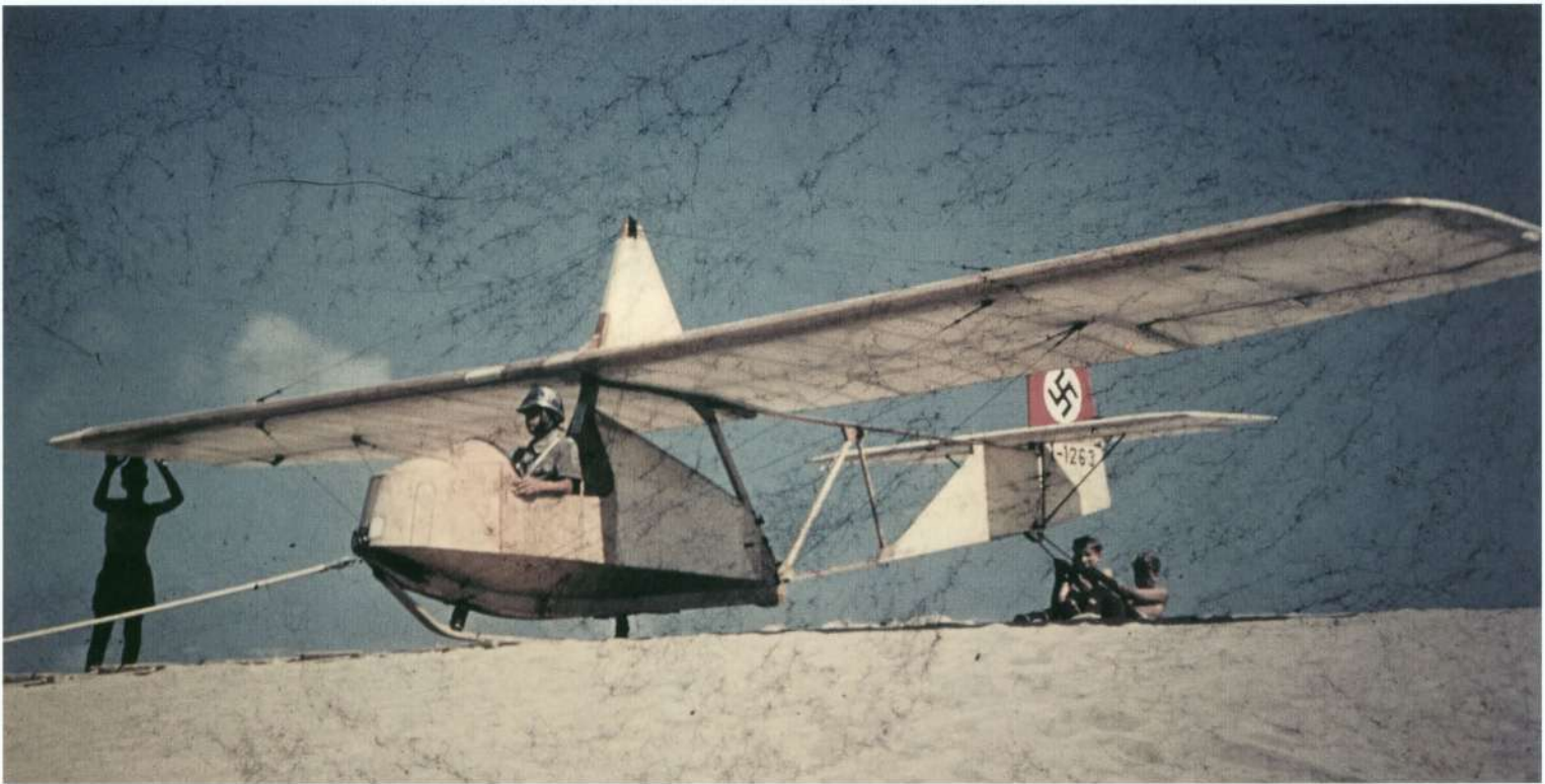
Above: A light nacelle was fitted to the S.G. 38 for the more advanced students. Note the crash helmet: standard wear for the NSFK.
