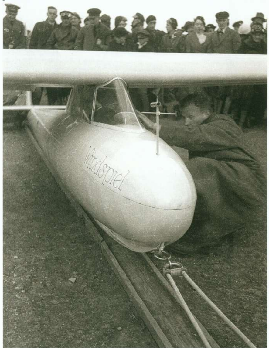
Windspiel ready for launching. The horizontal bar on the mast gave the pilot a guide to the trim attitude
