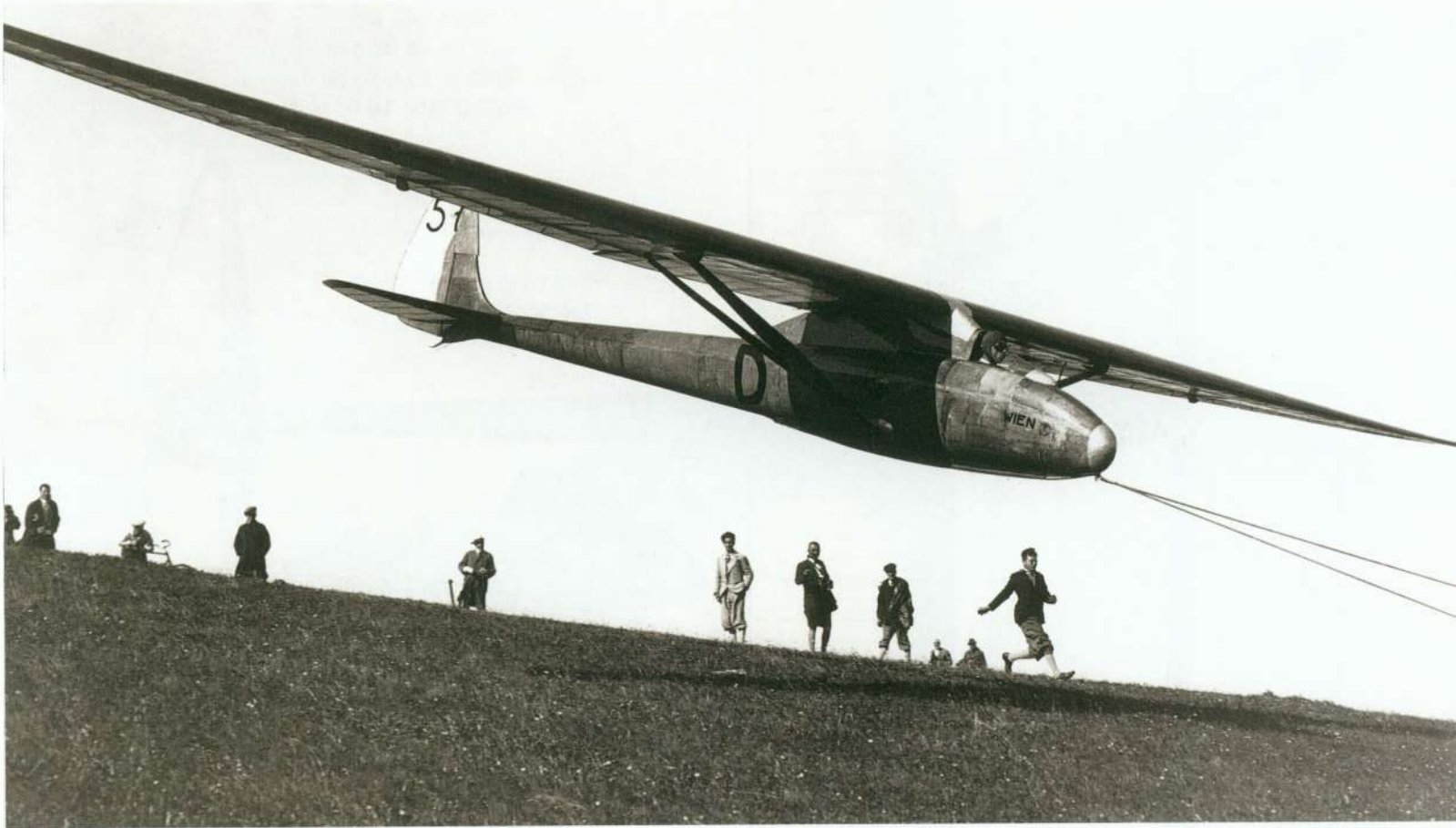
Above: Bungge launch of the Wien at the Wasserkuppe.
