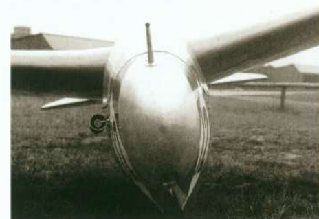
Above and right: The Duha 2, OK - Mario, designed and flown at the Internationals by J Chlup, was a much changed version of the Duha 1. It was a fifteen metre sailplane with a wing of pronounced 'gull' form, and a contoured transparent canopy. Chlup did not make a score. It has not been possible to make an accurate drawing of this type.
