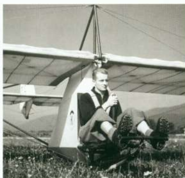
Above: The original English primary glider, the 'Dagling' marketed by the R.F. Dagnall company. The tail was carried on steel tubes.
