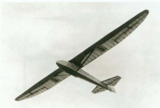
Above: Plans for the GB 2 were sold and numerous examples were built all over the world. Slingsby built fifteen under licence, one which is shown here. Note the broad ailerons.
