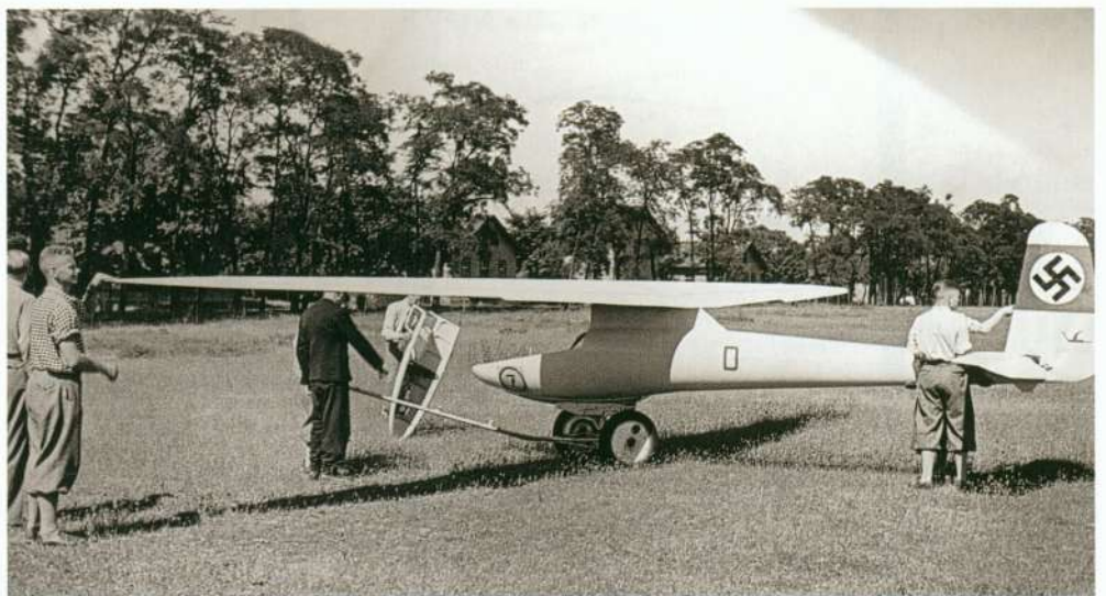
Right: The divided ailerons identify this as the D - 28B. Note the removable cockpit cover and the wheeled dolly for ground handling.
