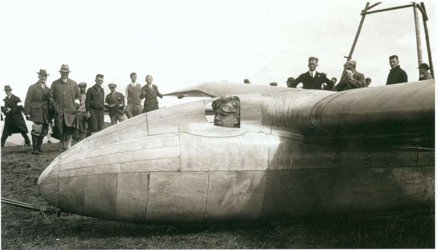
Above: To save a little drag, the pilot was fully enclosed with only small portholes to see through. Behind the Fafnir among the crowd is Peter Riedel, with arms akimbo, dark jacket and tie.
