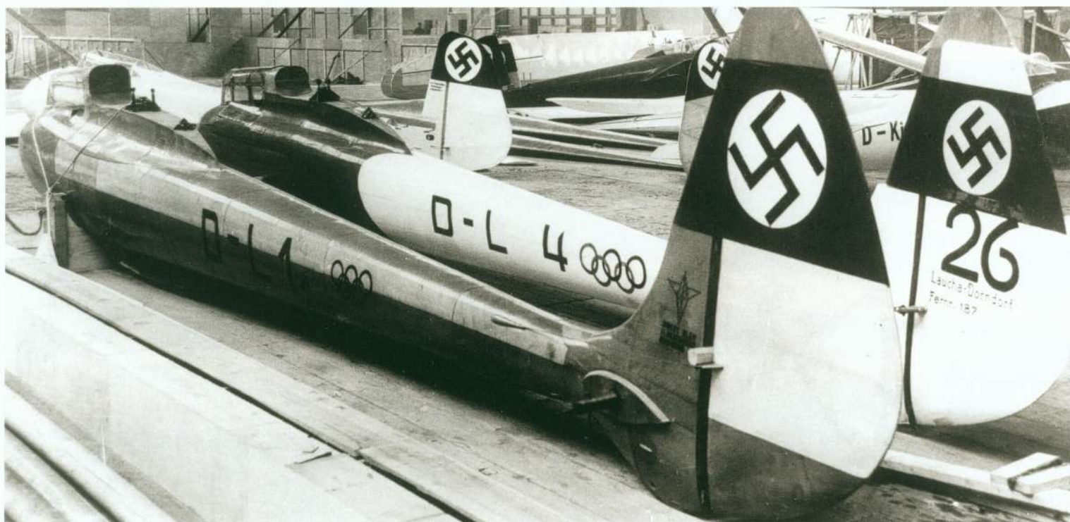
Below: March, 1936. At an aviation and water sport exhibition in Berlin, Condors carrying the Olympic rings were displayed. Note the high rudder horns and cables passing above the all-moving tailplane.
