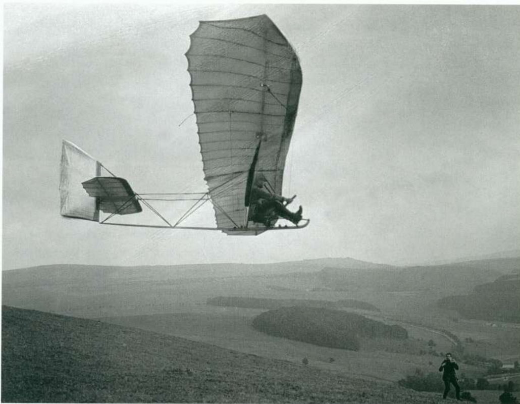
Left and right: The Harth Messerschmitt S - 10 in flight. Control in pitch was achieved by pivoting the mainplane on its transverse axis, a method of control which Messerschmitt used on several later sailplanes, and which was tried also by the Darmstadt students for their Geheimrat.
