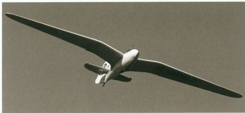
Above: An early Habicht built by Schweyer. Note the small vertical tail surfaces.
