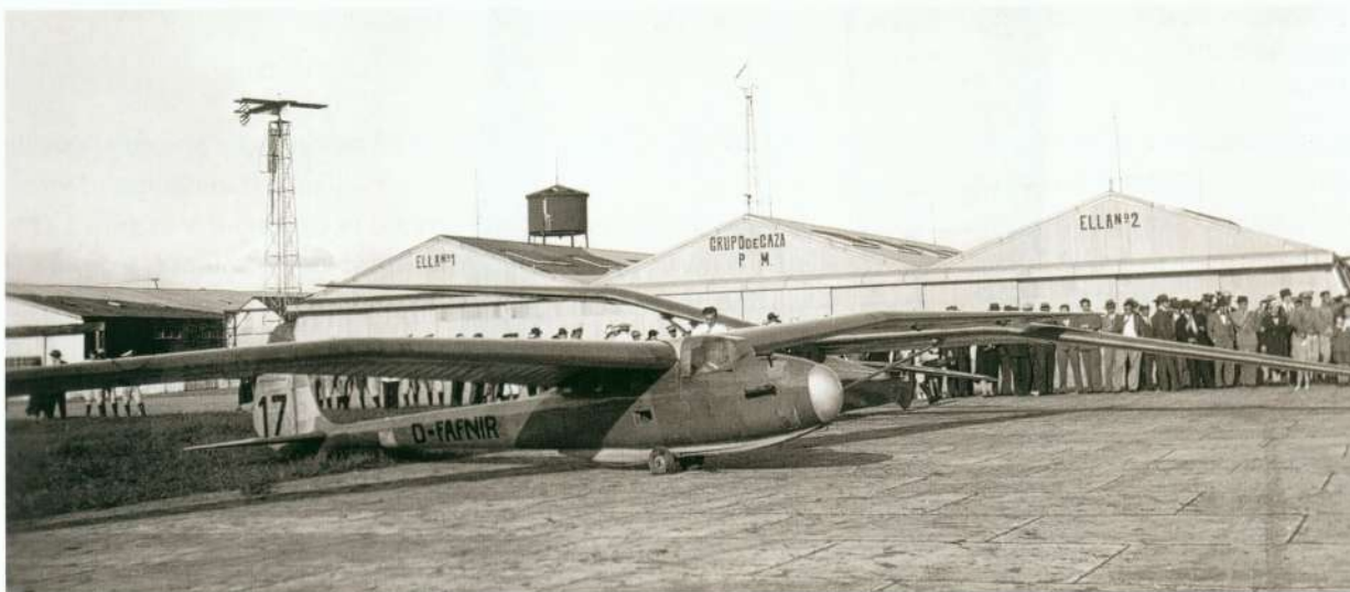
Above: To save a little drag, the pilot was fully enclosed with only small portholes to see through. Behind the Fafnir among the crowd is Peter Riedel, with arms akimbo, dark jacket and tie.
