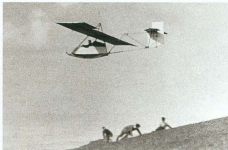
The original 'Djävlar anamma' or 'Hols der Teufel' designed by Lippisch. This was the basis of the Grunau 9 primary glider. Later versions by Schleicher and Jacobs also named Hols der Teufel, were really quite different.
