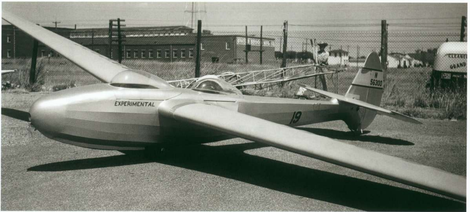
Above and left: The Laister Kauffman LK - 10, called the TG - 4 by the US military, was often modified, post war, to the so called 'flat top' configuration.
