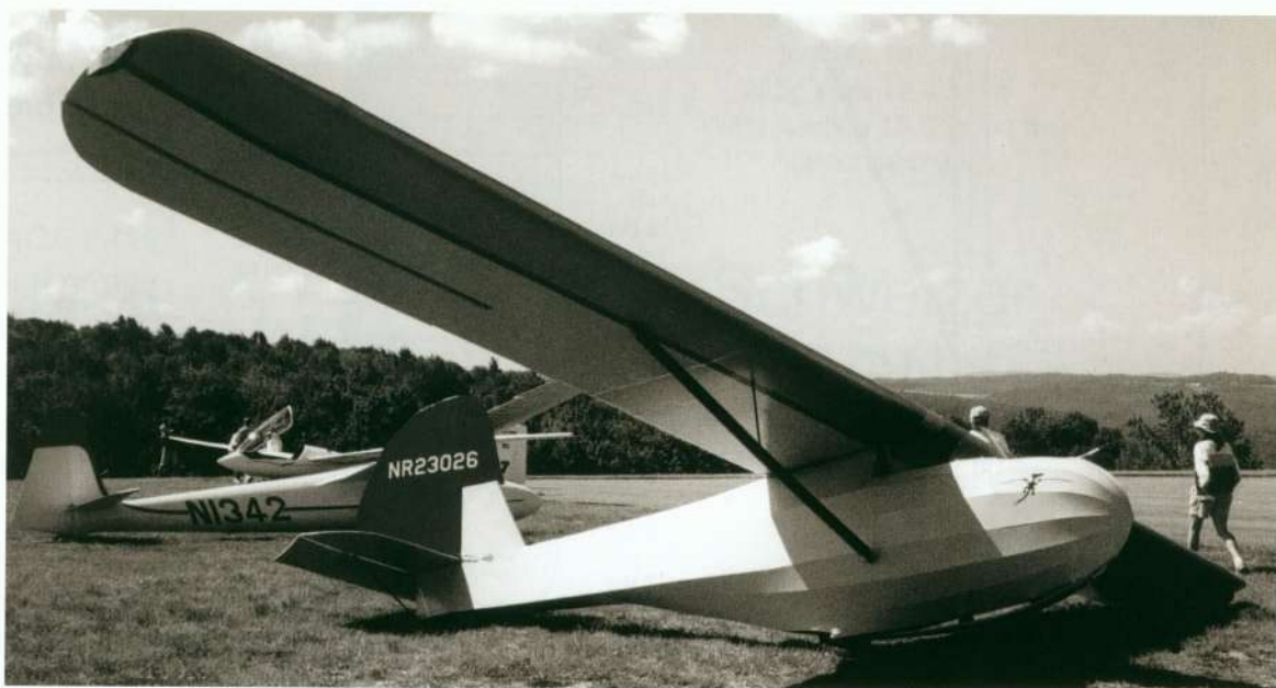
Right: The Schweizer SGU 1 - 7 had a metal wing and steel tube framed fuselage and tail, fabric covered.
