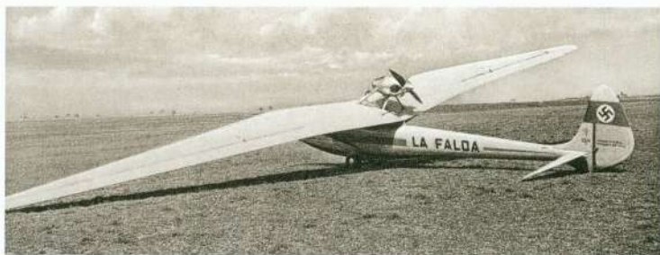
La Falda was flown as a 'pure' sailplane. The intention was to use the motor to bring it home after an outlanding.
