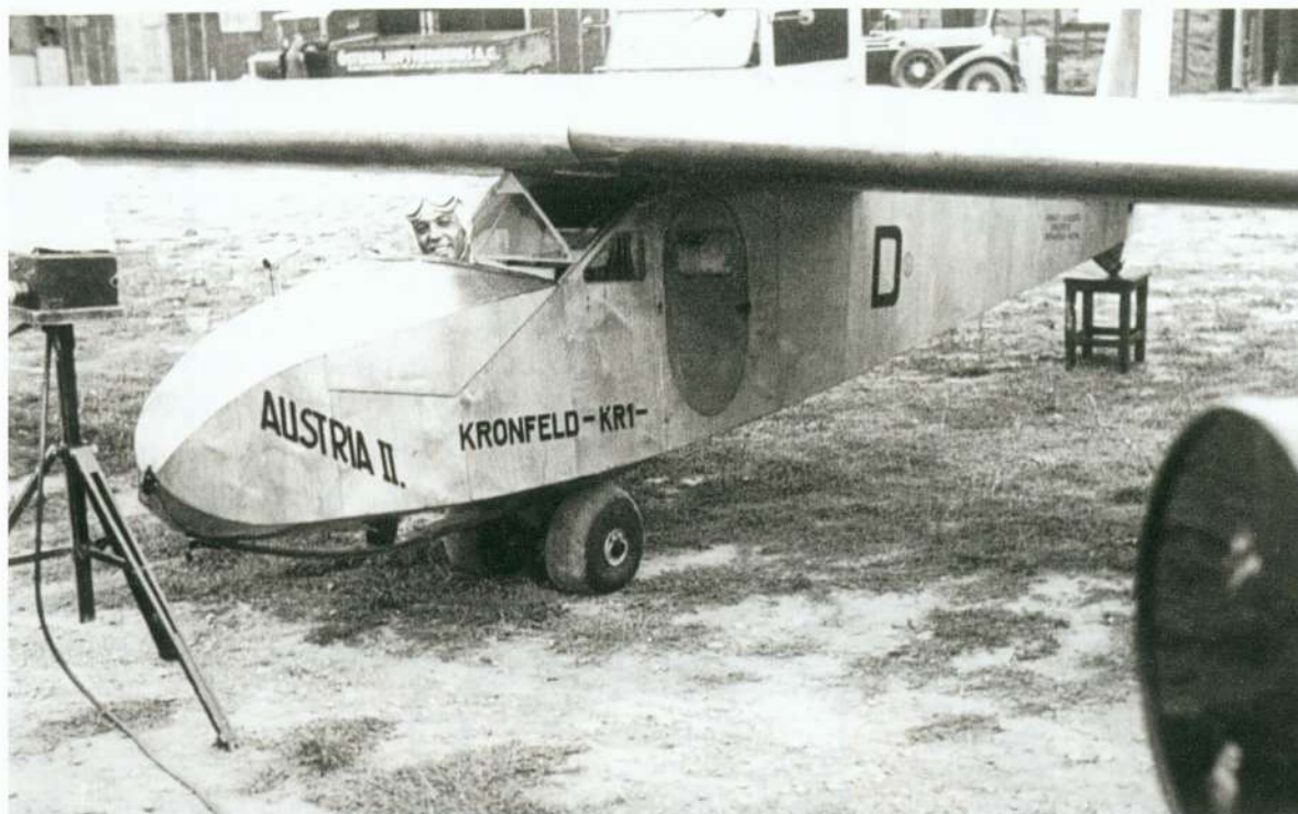
Kronfeld's Austria II. Cabin with door under the wing.
