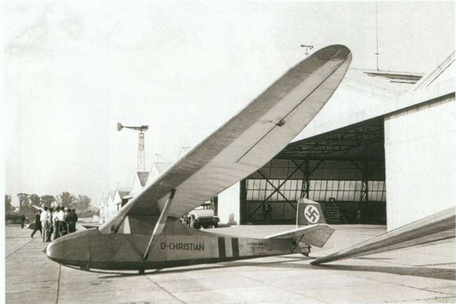
Above: Plans for the GB 2 were sold and numerous examples were built all over the world. Slingsby built fifteen under licence, one which is shown here. Note the broad ailerons.
