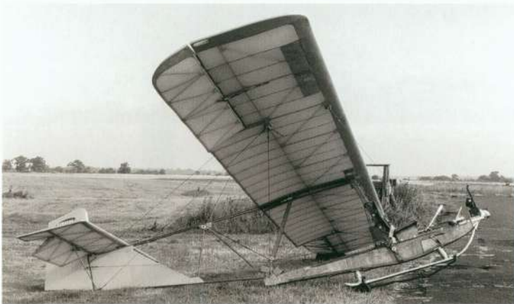
Above: A light nacelle was fitted to the S.G. 38 for the more advanced students. Note the crash helmet: standard wear for the NSFK.
