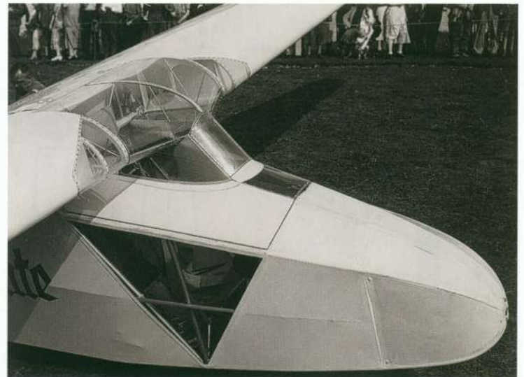
Above: Cockpit canopy and transparencies of the Atalante.
