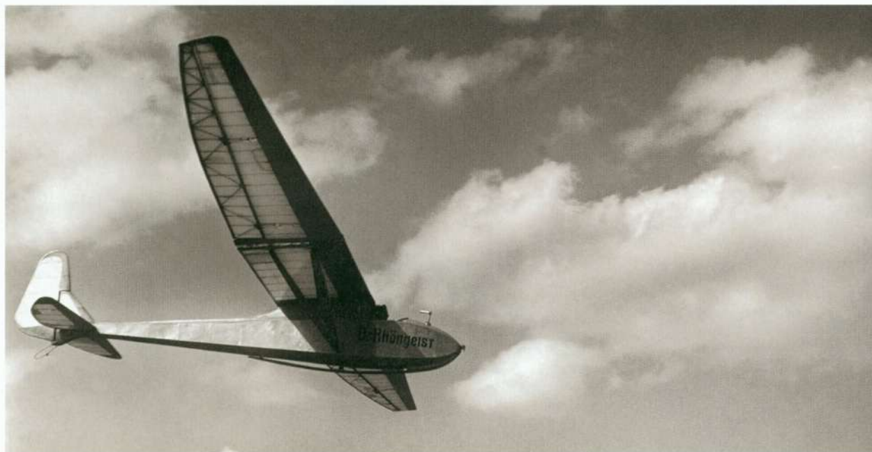
Many gliding clubs in Germany used the Professor type. The photo shows the original Rhöngeist fitted with the modified ailerons of the Professor 2. But the tail is still unchanged.
