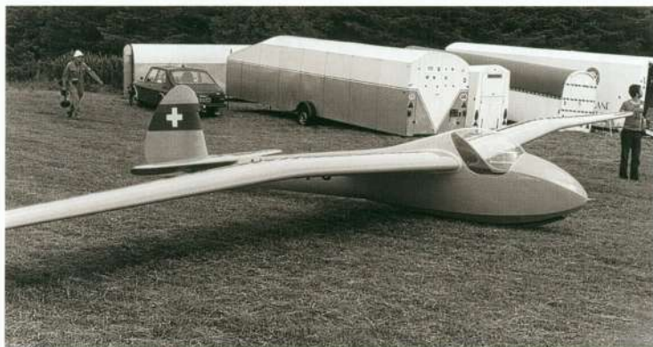
Right below: The Moswey 2A had the wing span extended to 15.5 metres.
