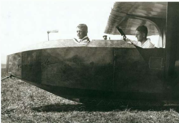
Above: The Darmstadt Margarete of 1923. Second pilot well back below the wing. Left: The Margarete flown solo at the Wasserkuppe.
