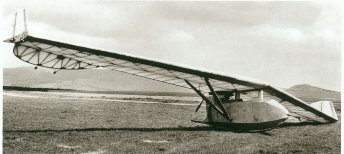
Right: The Storch V was fitted with a motor and flew well, encouraging Lippisch to continue with further work on tailless and delta aircraft.
