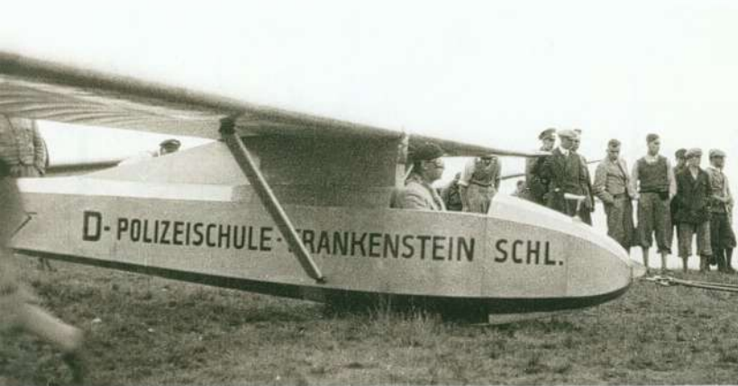
Above: The Grunau Baby 1 had a straight backed fuselage and tall rudder.
