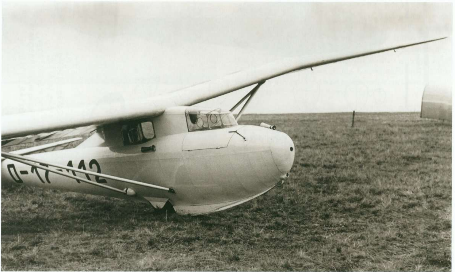
Above: The Mg 9a, with wheel and inverted V struts. Austrian markings after the Anschluss.
