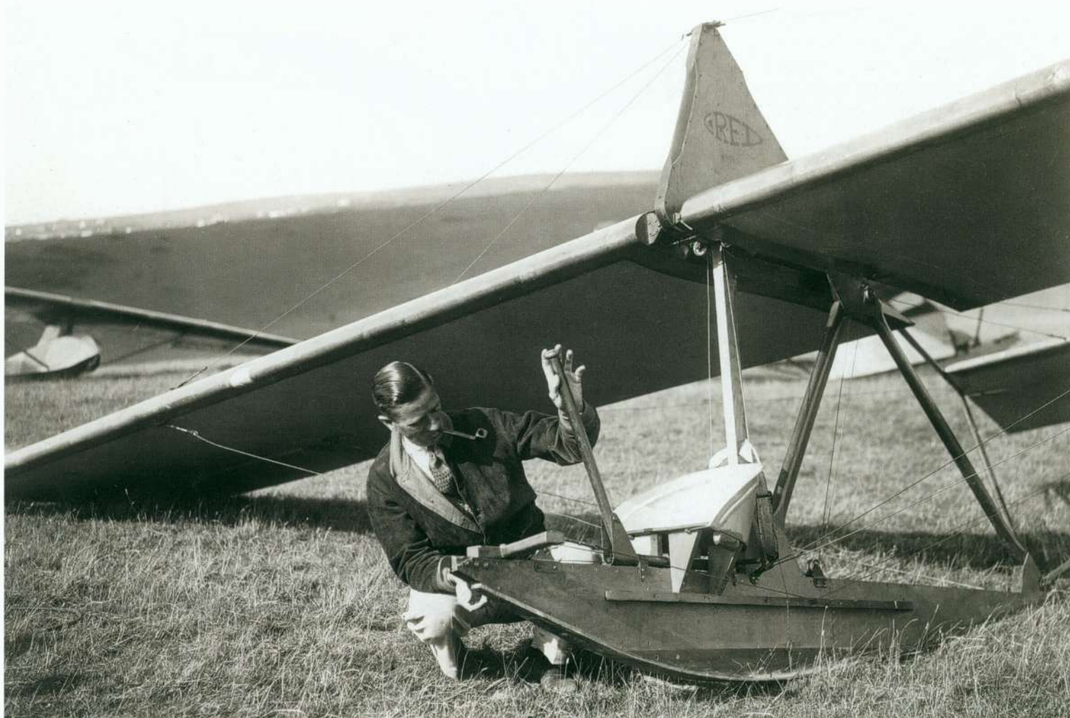
Above: The original English primary glider, the 'Dagling' marketed by the R.F. Dagnall company. The tail was carried on steel tubes.
