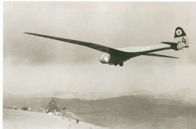
Above: The cockpit canopy originally (1934) was not fully faired to the fuselage.
