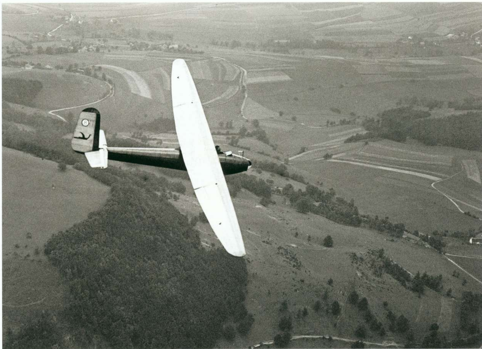
Above and left below: The D - 17, Darmstadt 1, showing the structure of the wing and ailerons, large vertical, all-moving rudder carrying the Darmstadt school's emblem. It made its contest debut at the Wasserkuppe in 1927 after the destruction of the Konsul.
