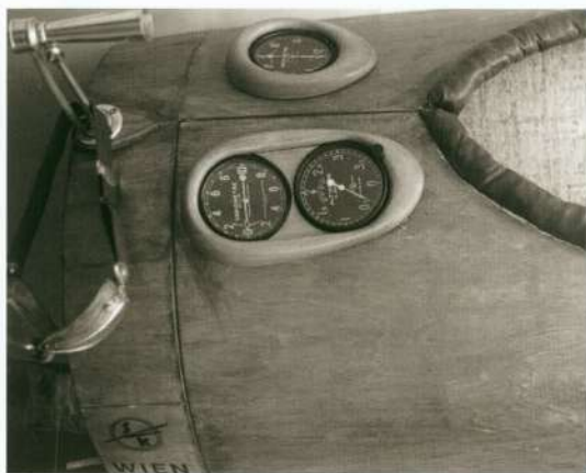
Left: The Wien instruments mounted on the fuselage decking. A replica by Klaus Heyn
