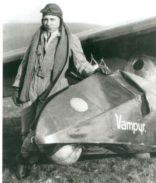
The Vampyr, showing the pneumatic, tricycle undercarriage and the leather cockpit cover which was fastened over the pilot's shoulders, leaving only his head exposed. The pilot here is Hentzen.
