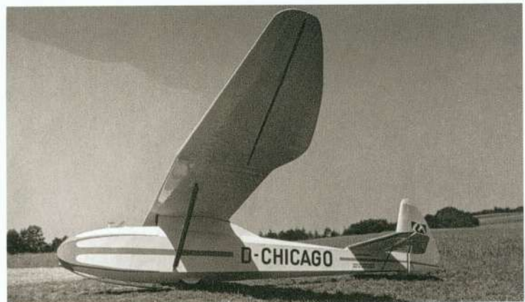
The Göppingen 1 Wolf was a rival to the Grunau Baby but was different enough to prevent confusion. The example shown here had the original broad ailerons.
