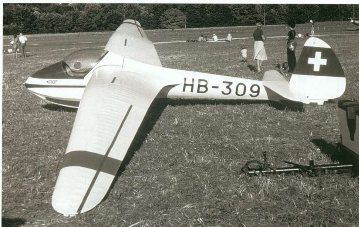
Right below: The Moswey 2A had the wing span extended to 15.5 metres.
