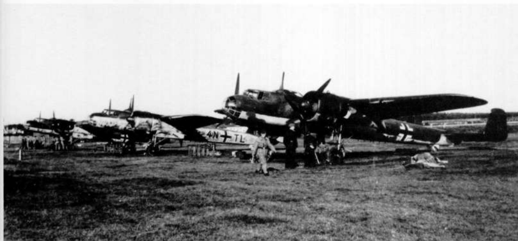
An undated early war photograph of Dornier Do 17 P 4N+TL of the 3.(F)/22 seen parked between two Do 17 Ps of the 3.(F)/11. While the aircraft in the foreground, 6M+TL is finished in the darker combination of 70/71 over 65, as is the third aircraft in line, the lighter colours evident on 4N+TL suggest that it remains in the segmented upper scheme in the 60 series of colours.
