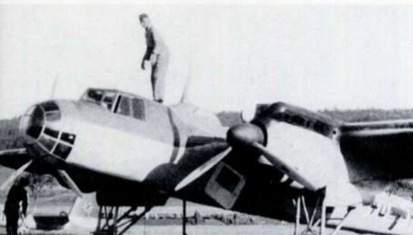
Seen here at its home base at Kassel-Rothwesten in 1938, Dornier Do 17 F-1 coded 40+F11 of the 1.(F)/22 finished in the newly introduced, three-colour segmented camouflage of 61/62/63 over 65 under surfaces.
