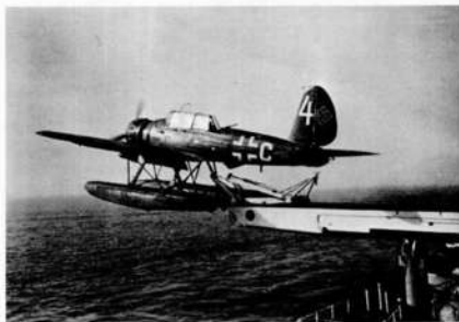
Arado Ar 196 A-3 coded K3+CO seen at the moment of launch from an on-board catapult. Although the aircraft is from Seenotstaffel 6 (Air-Sea Rescue Squadron 6), the photograph is included in this publication as it gives a clear view of the catapult dolly on which the aircraft was mounted for launching.
