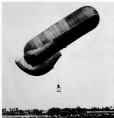
A Parseval-Siegsfeld Drachen (Kite) balloon and its observer ascend above an area of the Belgian countryside in the summer of 1915. Based on the original balloon designed by Major von Parseval and Hptm. von Siegsfeld in 1896, aside from their First World War German use, these later versions also saw service with the Belgian Army; copies of the design also found their way into British, French and Russian service during the same period.
