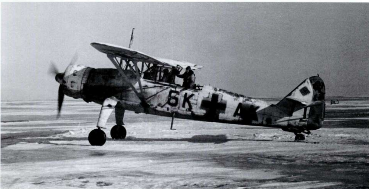
An Hs 126, coded 6K+AK of the 2.(H)/23 taken in the Kalinin area during the early winter of 1941. Note the towing attachment mounted aft of the tail wheel.
