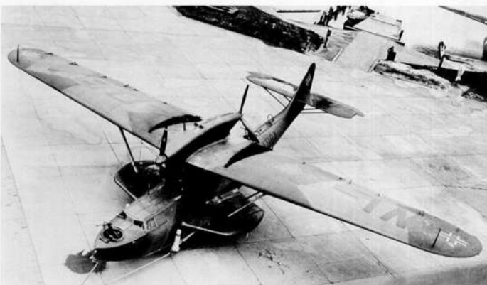
Dornier Do 18 G VI, W.Nr. 841 on the slipway at the E-Stelle Travemünde. Finished in the specified maritime upper splinter scheme of the greens 72 and 73 it carries full national markings as well as the short-lived Wehrmacht Luft code WL - ADBA applied in black across the top of the wing and to both fuselage sides. Clearly visible in the top view is the heavy 'V'-shaped exhaust staining from the wing-mounted exhausts of the forward Junkers Jumo diesel engine.
