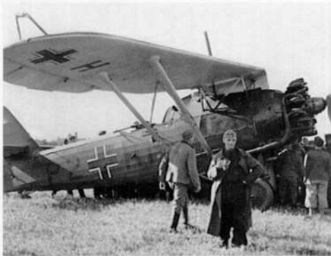
Finished in the standard scheme of the greens 70/71 over blue 65 under surfaces with early style Balkenkreuze and the swastika applied across the rudder/fin hinge line, Heinkel He 46, P2-HM of the 4.(H)/21 was photographed at Gross-Lassewitz on 1 September 1939.
