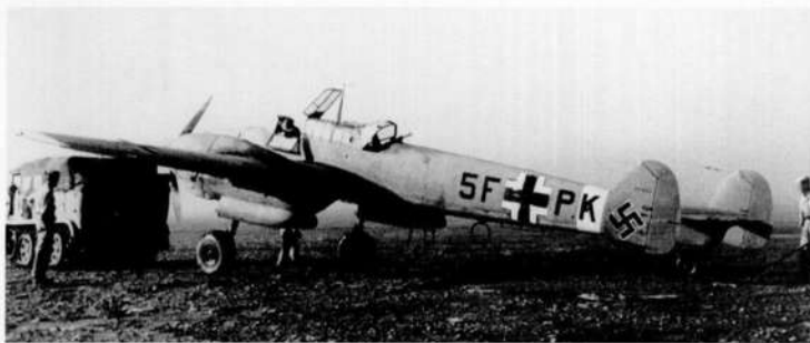
In this photograph, believed to have been taken in the Benina area circa December 1941, Messerschmitt Bf 110 E-3/Trop 5F+PK, W.Nr. 4427 of the 2.(H)/14 wears an overall upper finish of the newly introduced colour of sand yellow 79 over blue 78 or 65 under surfaces. Around the rear fuselage is the white identity band commonly worn by Luftwaffe aircraft during the early stages of the North African campaign.
