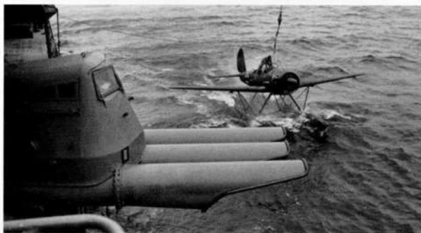
Arado Ar 196 A-3, T3+HL taxis alongside a slowly moving 'Prinz Eugen' as the observer connects the lifting strop in preparation for hoisting the aircraft inboard. To the left of the photograph and trained to port, is one of the four triple torpedo batteries carried by the ship. Although she never sank a single enemy vessel, she is remembered as a 'lucky' ship and although heavily damaged on several occasions, was the only heavy surface unit of the Kriegsmarine to survive the Second World War intact. One of her Arados is currently in storage at the Paul E. Garber Facility in Silver Hill, Maryland, USA.
