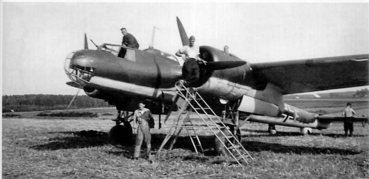
Undergoing maintenance to its port BMW 132N engine, Dornier Do 17 P-1 of the 4.(H)/31 sits in the sun at its base believed to be at Stadtkyll, Germany in the summer of 1940.
