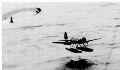
An Arado Ar 196 A-2 comes in to touch down close to the leeward side of its parent ship.
