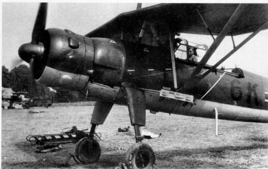
The pilot of Henschel Hs 126 A, L2+L37 of the 7./LG 2 holds his aircraft on a slow, steady course while the observer hangs precariously over the side to operate his hand-held HK camera. The blemishes visible in the photograph on the upper wing surface surrounding the L2 and 37 are believed to be the residue remaining after temporary 'war games' markings were removed.
