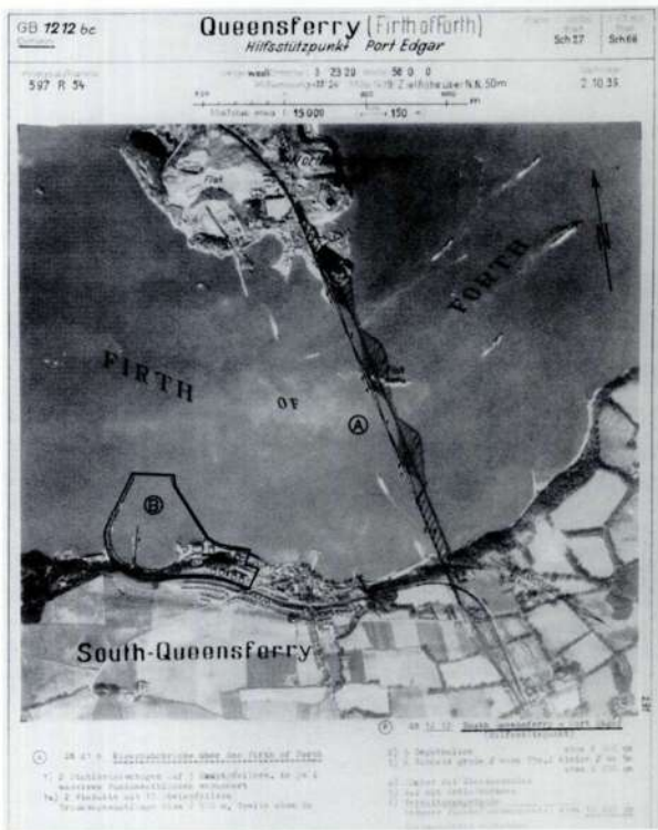
Believed to have been taken by an aircraft of the AufklGr.ObdL prior to 2 October 1939, this aerial reconnaissance photograph from a Luftwaffe target folder covers the Midlothian district of South Queensferry/Port Arthur, target number GB 12 12. Identified on the photograph, item A is the well-known Firth of Forth cantilever railway bridge, the construction of which is clearly shown by the shadows cast on the waters of the Firth, while the North Queensferry anti-aircraft locations are simply noted by the word 'Flak'. Item B identifies coastal defence positions, unidentified depots, storage tanks, a quay and an oil-pier (oil-pier). In the mid lower right of the photograph is an arrow showing the flight line to Edinburgh, 13 km (8.07 miles) to the south-west.
