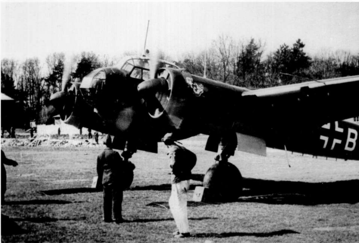
4U+BH of the 1.(F)/123 undergoes an engine run-up at an un-named location in Northern France in November 1940. Either a Ju 88 A-1(F) or A-5(F) variant, it has undergone a partial conversion from its original bomber configuration with the removal of the underwing dive brakes, the mounting brackets for which can be seen beneath the wing leading edge. In keeping with a practice that began when the Staffel flew Dornier Do 17 Ps, the Staffel emblem of a caricature of a Luftwaffe airman holding a telescope has been applied to the outboard engine cowling panel of each engine.
