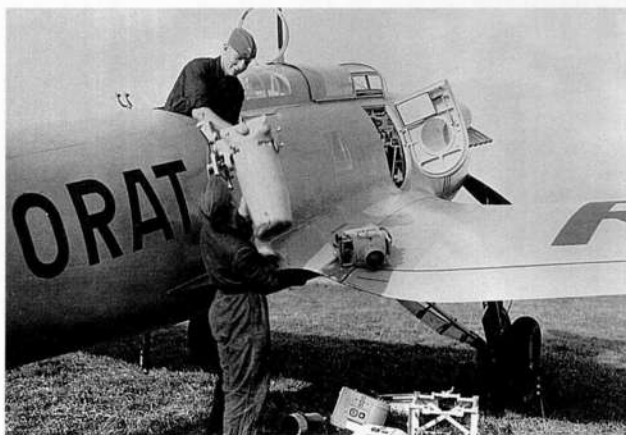
Mechanics removing an Rb 50/18 camera from D-ORAT , a civilian registered Heinkel He 70 believed to have been in pre-war service with Aufklärungsgruppe 11 in East Prussia. The camera sitting on the wing is a Zeiss HK 19 Handkammer while on the grass beneath the wing is a camera mounting frame, film magazines and a second unidentified camera.
