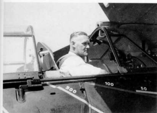
This close-up view of the cockpit area of an unidentified Henschel Hs 126 A-1 clearly shows the Revi gun sight for the fixed, forward-firing 7.9 mm MG 17 machine gun, canopy slide rails and latch and the four sighting reference lines painted on each fuselage side for the observer's use in photographic work with a hand-held camera.
