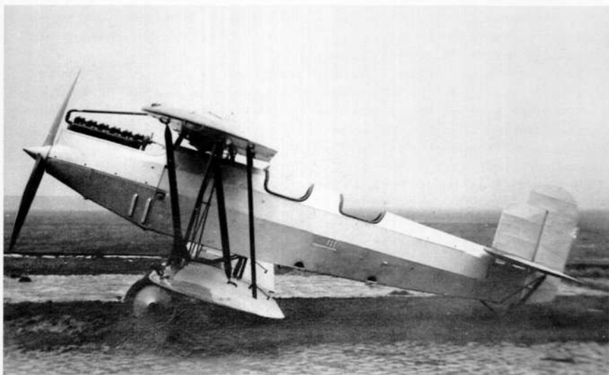
Three views of a BMW Iva powered Albatros L-75 trainer of the type used by the various Reklamestaffeln during the early 1930s.
