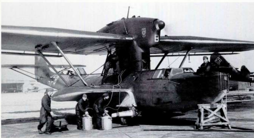
Dornier Do 18 D-1 of the 2./KüFlGr. 906 undergoing servicing of the fuel system for its Junkers Jumo 205C diesel engines. Coded 8L + BK and finished in the standard maritime scheme of 72/73/65, the aircraft letter 'B' is yellow and is repeated on the front of the wing pylon while on the side of the cowling can be seen the Staffel emblem.
