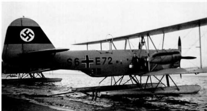
With its overall 63 finish broken only by its national markings and code letters, Heinkel He 59 S6+E72 of the FFS (See) 3 is seen here moored stern first to a slipway at Stettin circa 1937.
