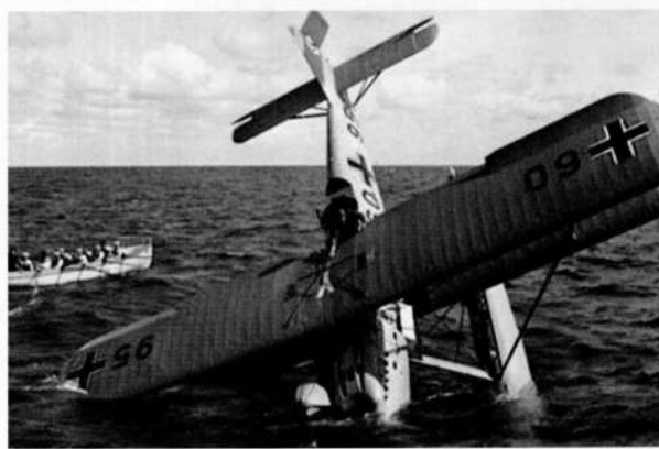
In similar fashion, Heinkel He 60 60+Y95 ended up nosed over into the sea. Neither the cause nor the resulting fate of this aircraft is known, although note the broken starboard float, perhaps due to a heavy landing. In both cases, the addition of a thin black border to the outer edges of the white borders for the arms of the Balkenkreuz suggests that both incidents occurred after mid-1936.
