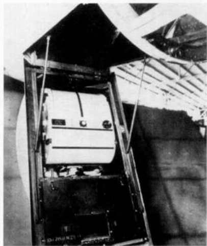
A Dornier factory photograph showing the opened blister housing for the Rb 50/30 camera installation in a Dornier Do 215 B, the installation of which must have provided for the easiest accessibility of all fixed on-board reconnaissance cameras in Luftwaffe aircraft.
