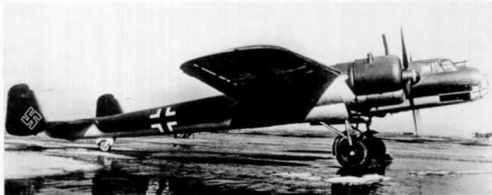
A factory photograph of Dornier Do 17 P W.Nr. 4013 finished in the prescribed 70/71/65 pattern for the type. The light coloured band around the spinner is thought to have been yellow.
