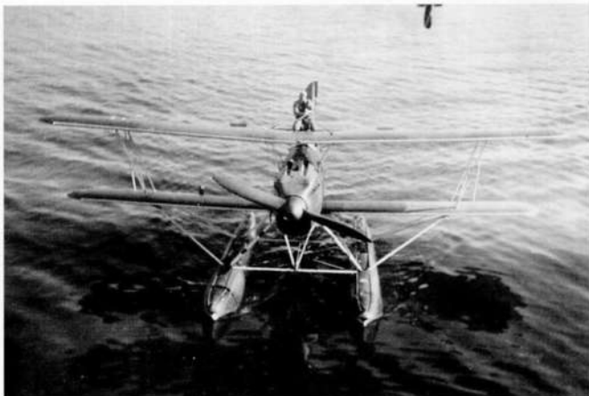
A Heinkel He 60c coasts towards its parent ship while the observer stands by at the rear of the wing in preparation for securing the lifting strap to the ship's crane to hoist the aircraft inboard.
