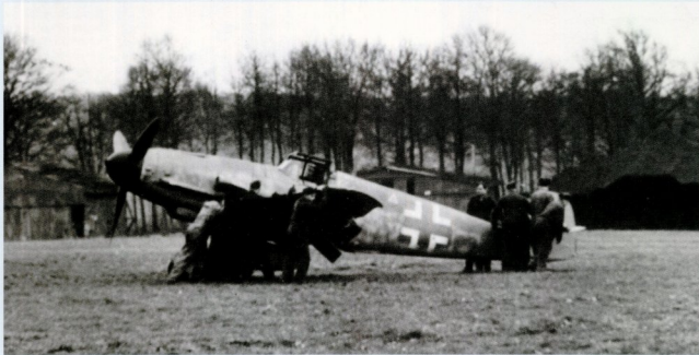
Staffel personnel of the 5.(F)/123 manhandle a Messerschmitt Bf 109 G-4/R3 of the 5.(F)/123 over what appears to be a soggy section of the airfield at St. Pol early in 1943. Just visible on the lower fuselage is the ventral camera window and fairing.
