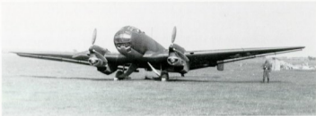
Two views of what is believed to be Junkers Ju 86 P of the 2.(F)/ObdL, T5-RK, which carried out high-altitude flights over the British Isles from its base at Oranienburg near Berlin during 1940; in the second view, an unidentified member of the Staffel is seen holding the circular crew hatch for the pressurised crew cabin.
