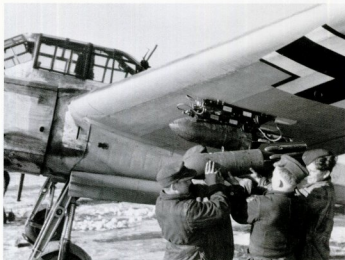
As with other reconnaissance units as the war in the East progressed, the 2.(H)/31 were often called upon to conduct anti-partisan operations both in the Balkans and the Eastern Front. In this view, armourers are seen loading SC 50 bombs to the ETC 50/VIII bomb-carriers beneath the port wing of one of the aircraft of the Staffeln in preparation for such a mission on the Eastern Front in 1943.
