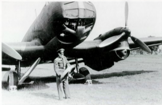
Two views of what is believed to be Junkers Ju 86 P of the 2.(F)/ObdL, T5-RK, which carried out high-altitude flights over the British Isles from its base at Oranienburg near Berlin during 1940; in the second view, an unidentified member of the Staffel is seen holding the circular crew hatch for the pressurised crew cabin.
