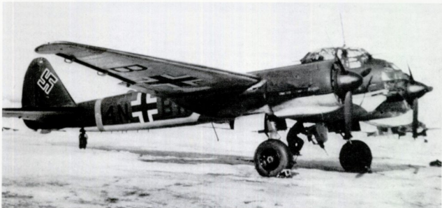
An early Junkers Ju 88 D-1, 4N+BK of the 2.(F)/22 at an airstrip in the area of Poltava in the early winter of 1942. Finished in a standard 70/71/65 camouflage, the lower surfaces of the wing tips are painted in the theatre colour of yellow while the theatre band around the rear fuselage is much narrower than was usually seen on Ju 88s.
