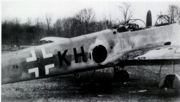
This Messerschmitt Me 410, 7A+KH, of the 1.(F)/121 was found in this stripped and derelict state at Rheims, France, by advancing Allied troops in the summer of 1944. Finished in 74/74 upper surface colours with a mottle of these colours along the fuselage sides, the open centre of the Balkenkreuz and area behind the code letters has been repainted in a darker green or grey, possibly the result of over-painting the markings of a previous unit.
