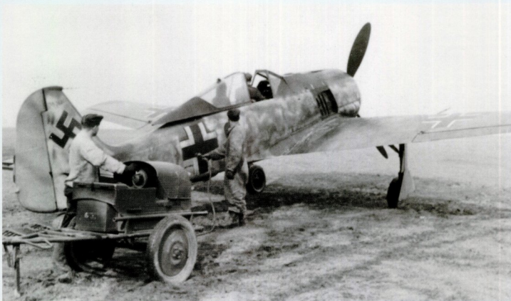
Another photograph of Focke-Wulf Fw 190 A-3/U4, 'Red 9' at St. Pol in March 1943, taken this time from 'Red 10'. The photograph below shows the ground crew with an engine start trolley.
