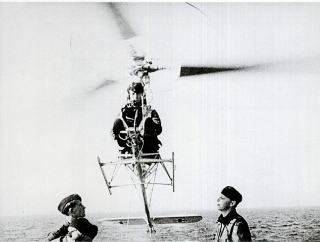
A view of the controls of a Focke-Achgelis Fa 330 as it sits ready for use abaft the conning tower of a type IX U-boat.
