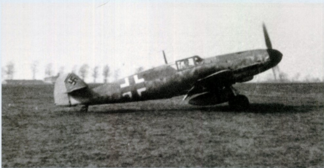
An unidentified Messerschmitt Bf 109 G-4/R3 of the 5.(F)/123 taxis past the camera at the St. Pol airfield in the spring of 1943. Finished in the standard day fighter camouflage of 74/75/76 with a dense mottling of 74/75 along the fuselage sides, the spinner is painted either in black or 70, and while the rudder appears to be yellow, it is impossible to determine whether this required colour has been applied to the lower cowlings.
