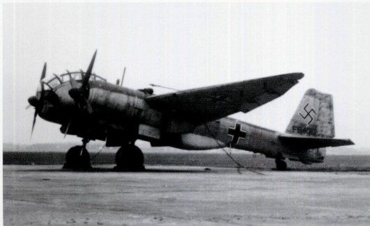
Taken after its capture and transfer to the United States, this view of Junkers Ju 388 L-1, W.Nr. 560049 in spurious markings applied by the Americans, clearly shows the bulged ventral pannier to carry a pair of Rb 50/30 or 75/30 cameras or, for the night role, a pair of NRb 40/25s or 50/25s. Although issued to the Luftwaffe in small numbers, it never became fully operational in its intended role. This particular aircraft is currently in storage at the National Air and Space Museum in the USA in a dismantled state.
