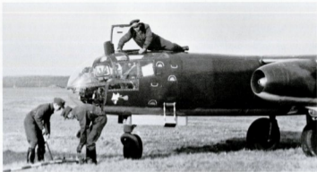
Ground crew prepare to attach the towing bar to the nose gear leg of Werner Muffey's Arado Ar 234B(j), T9+KH. Clearly visible on the lower forward fuselage is the jet-propelled sparrow motif. It is believed that this aircraft was the only one of Kommando so decorated.
