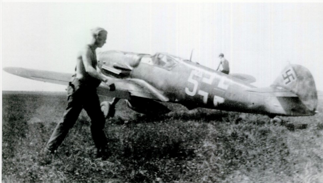
A Messerschmitt Bf 109 G-6 or G-8, 5F+ "Yellow 5" of NAGr. 14 seen at St. Malo during the summer of 1944. In common with their Allied opponents, pilots of single-engined Luftwaffe fighters frequently had a member of the ground crew sit on a wing to guide the pilot while taxiing his machine.
