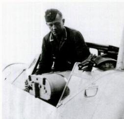
Bildstelle equipment personnel of the 5.(F)/123 are pictured in the process of installing a fresh film magazine on to the fuselage-mounted Rb 75/30 of Messerschmitt Bf 109 G-4/R3, 'Red 12', at St. Pol, France in mid-1943.
