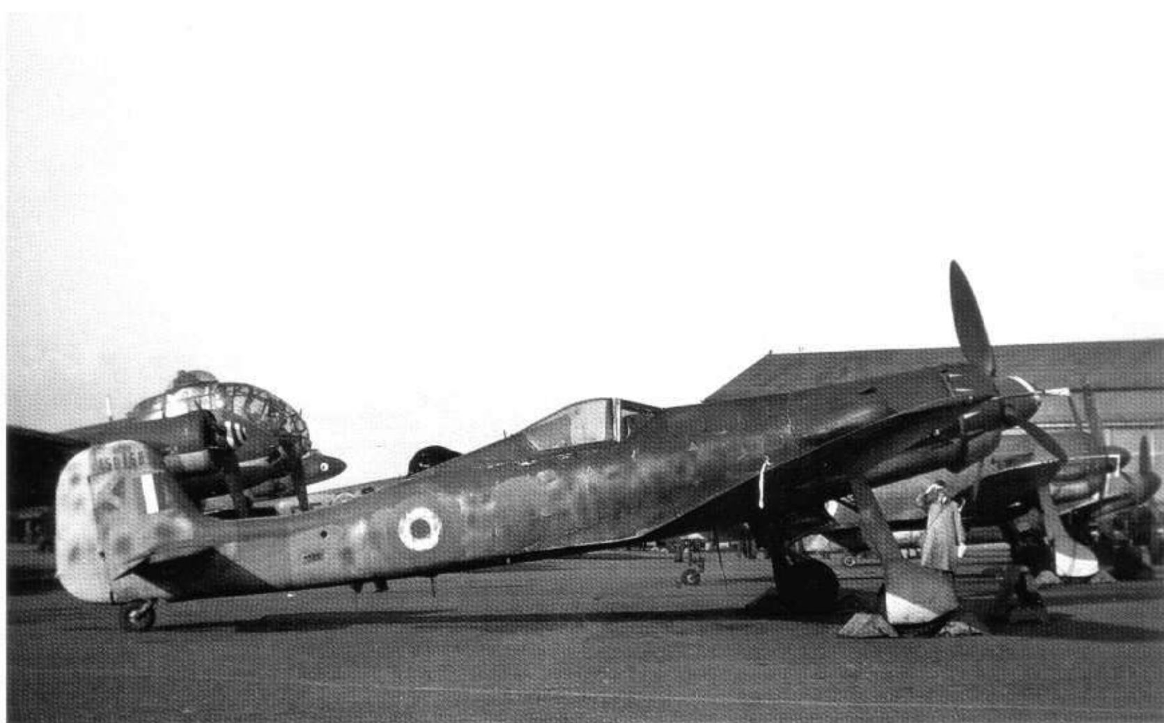
350: Once flown by Ofw Willi Reschke of Stab./JG 301 as 'Green 9', this Ta 152H-1, WNr 150168, was captured intact and sent to Farnborough. Apart from the overpainted German markings, the aircraft remains in its original camouflage finish: 81/82/76. It appears that despite instructions to leave the undersides of fighters unpainted, the Ta 152H received a solid coat of 76 on its underside. The low tonal contrast between the two dark greens is obvious. Propeller blades are 70. When originally captured there was a Reich Defence Band in red and yellow around the rear fuselage
