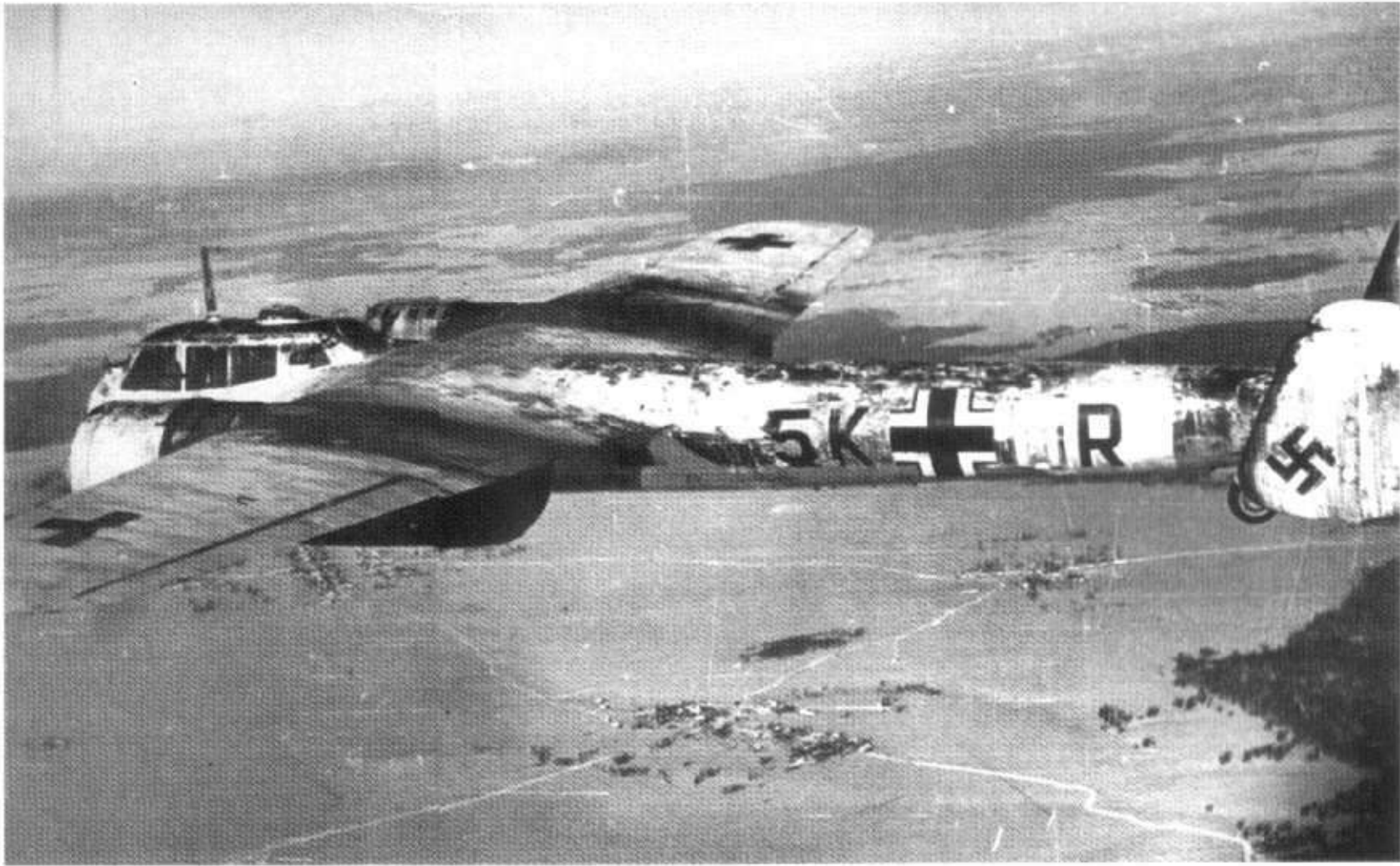
198: In the case of this Dornier-Do 17Z of 7./KG 3, 5K+HR, it is apparent that the temporary snow camouflage has been applied as per instructions, by brush. Wear and weather, however, are already washing it off, adding to the camouflage effect
