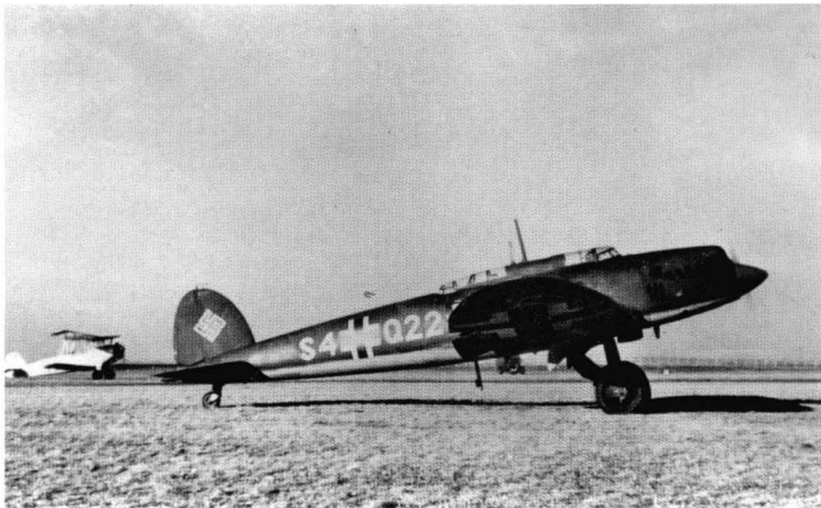
289: This Heinkel He 70, possibly WNr 1774, of FFS E A/B Quackenbruck, wears the early style of training codes found in the immediate pre-war years but in white, not black. The black-painted underside to the wing carries an enormous Balkenkreuz and the code, S4+Q22, in white again. The glossier finish of the 7160 lacquers used for the national insignia is clearly visible
