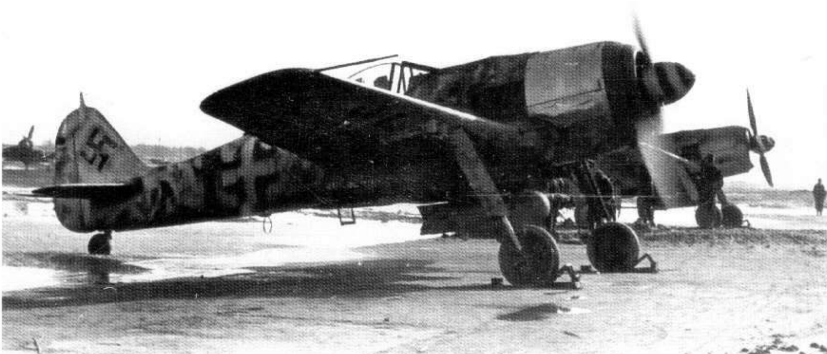
203: A pair of Fw 190F-8/R1 fighter-bombers of SG 2 in Hungary in early 1945. The winter camouflage on the nearest aircraft has been hastily applied in stripes and is heavily weathered. Armed with an AB250 bomb container, the machine shows signs of the shortages which were beginning to afflict the Luftwaffe at this stage of the war; the underside appears to have been left unpainted, as does the engine cowling which has several dents in the bulge over the air intake. The cowl ring may be yellow. Note the maximum simplified Balkenkreuz
