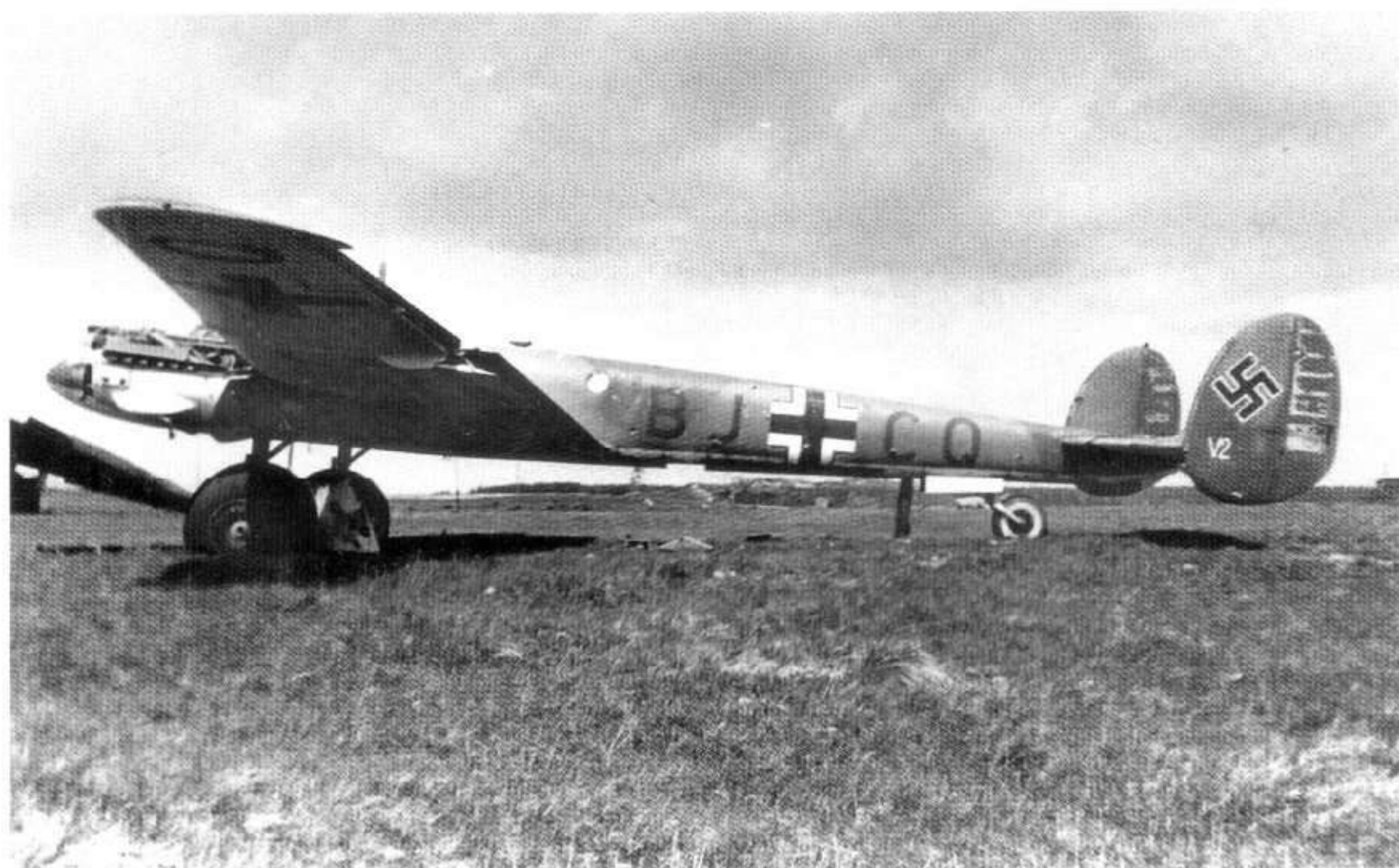
136: The wreck of the Messerschmitt Me 261 V2, BJ+CQ, abandoned at Lechfeld in 1945. The aircraft had been there for some time as the 70/71 camouflage had washed out revealing the primer (compare with the description of Flieglackette 20 on page 222). Both Balkenkreuz and swastika have a thin black border
