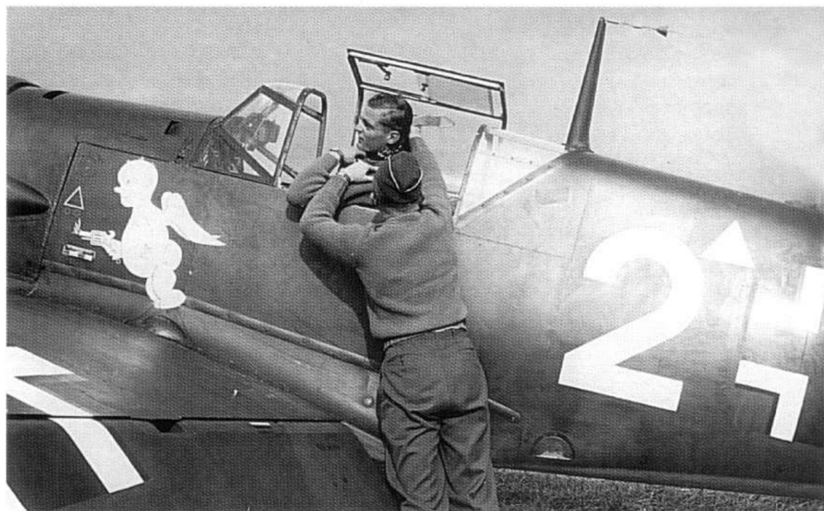
69: Pictured in late 1939, at first glance this Bf 109E appears to be an overall dark green but the subtle difference between RLM 70/71 can be seen on the wing root and flap. The aircraft carries standard insignia for the period, except for the personal emblem of a gun-toting angel and grossly oversized wing Balkenkreuze. These were not uncommon on several types of aircraft at this time, probably on account of a mis-interpretation of the official instructions and the hope that such markings would prevent mistakes by their own flak and aircraft (see page 152)
