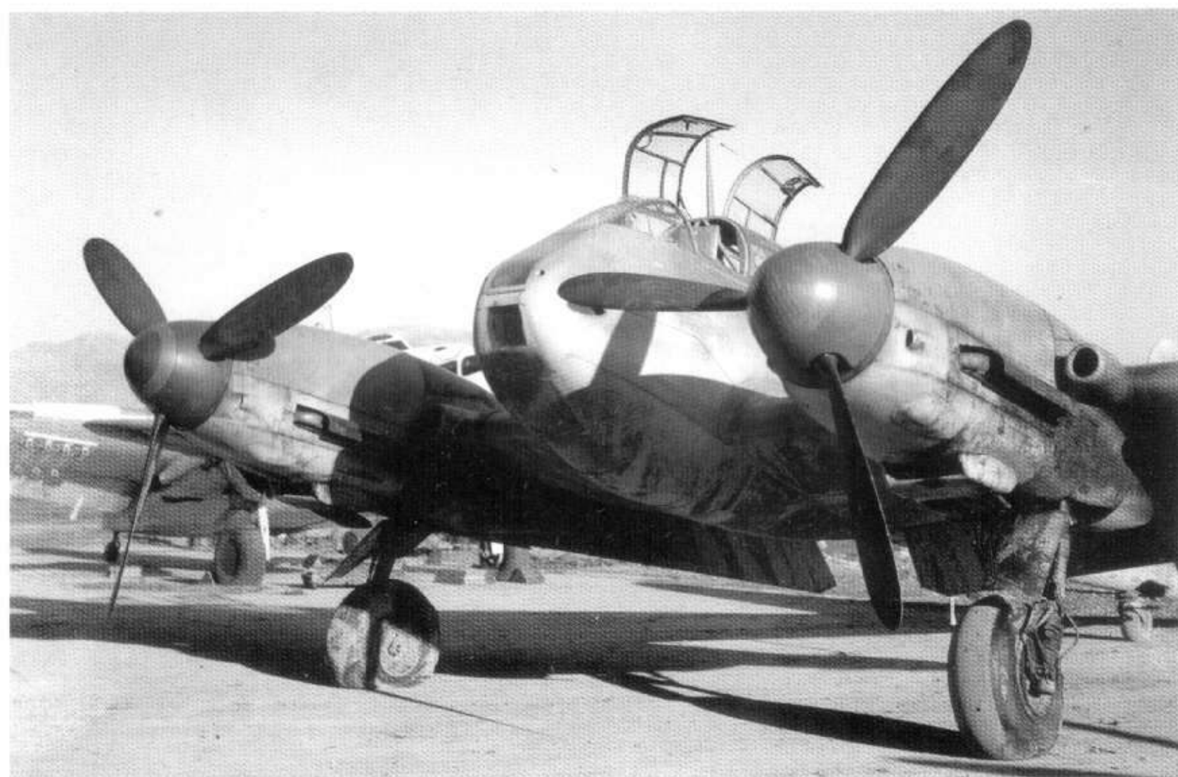
94: Messerschmitt Me 410A-3, F6+OK, WNr 10259, of 2.(F)/122, seen shortly after it was captured in Sicily in November 1943. It is finished in the standard camouflage of RLM 74/75/76 with a ring on each spinner painted in red 23, the staffel colour
