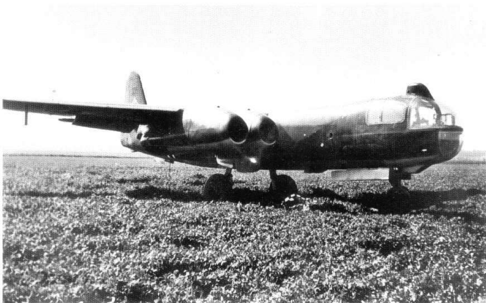
349: The sixth production Ar 234C-3, WNr 250006. The official camouflage drawing for the Ar 234C dating from 19 June 1944 calls for it to be finished in 70/71/65. By the time the aircraft were finally finished, however, the two greens had officially been superseded by 81 and 82. Considering the high gloss finish, it is impossible to say from this photo which colours were used
