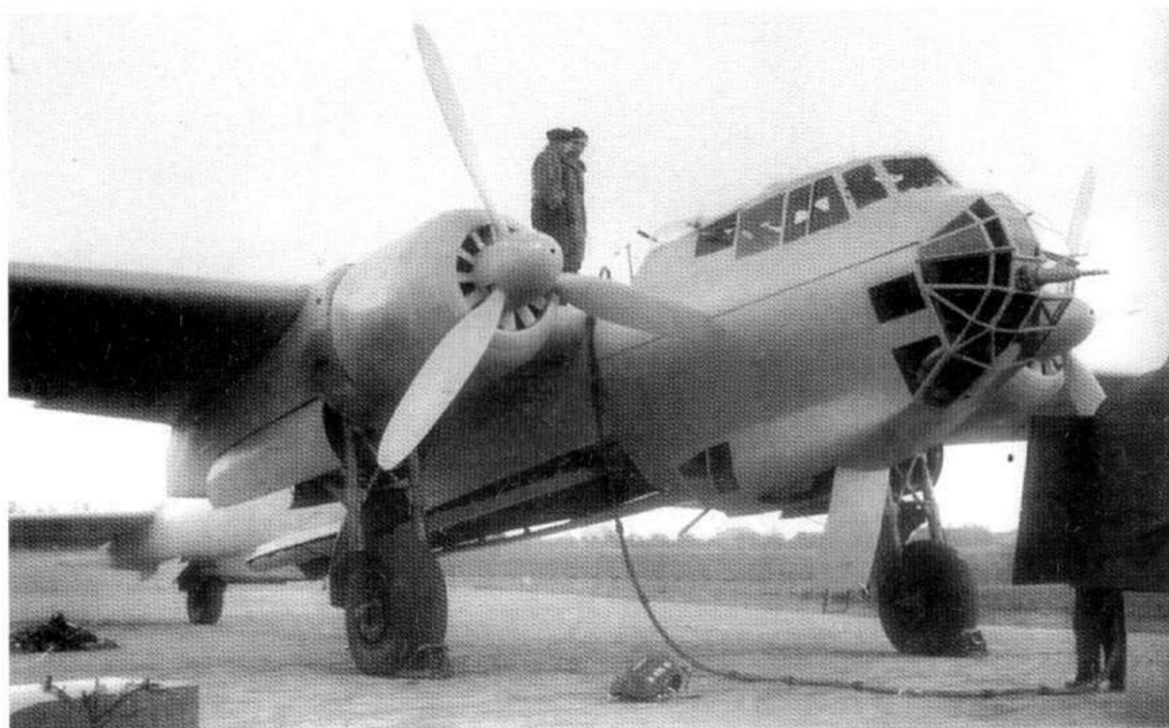
101: This Dornier 217E-3 is apparently finished overall in RLM 65 (1941 version), including the engine cooling fans, with no markings visible. A few aircraft were actually delivered to KG 2 and KG 40 for service in this colour scheme, which was not inappropriate for use over the ocean. Note how the bomb bay doors fold
