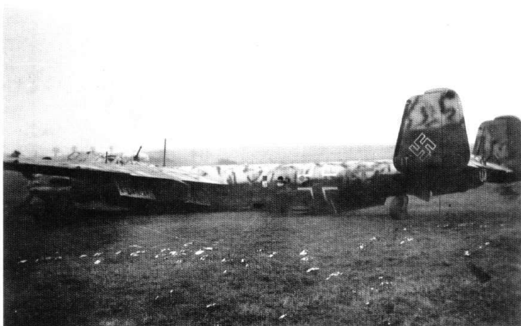
223: A Dornier Do 217M which crashed near Toul in France in late 1943-early 1944. The aircraft wears the last two letters of a just discernible code, 'AT' in 77 or, more likely, 23 Rot. Barely visible on the fin is a yellow werk nummer, 3046(?). Undersides are entirely 22 while the upper surface and upper halves of the rudders are 76 with a meandering black line sprayed over the top. National insignia are just the white portions. The camouflage style suggests that this could be a machine of KG 2 during their involvement in 'Operation Steinbock', the 'Little Blitz' against Britain
