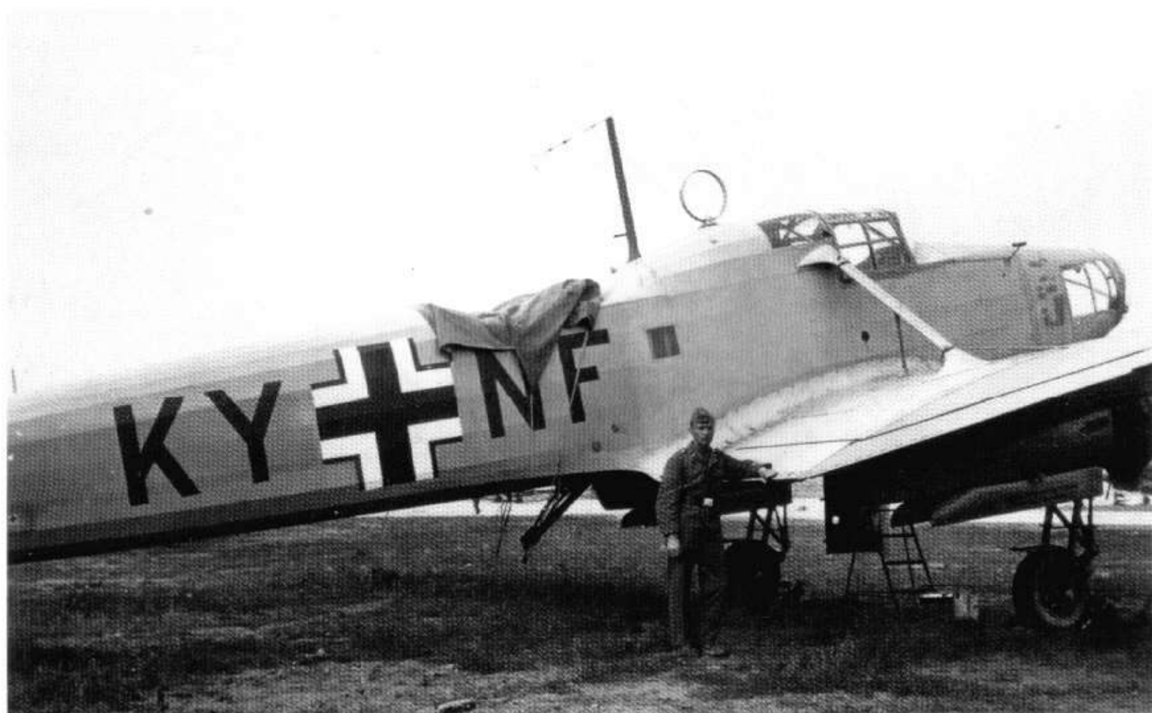
290: A Focke-Wulf Fw 58, KY+NF, belonging to KFS Thorn in late 1940. Finished in overall RLM Grau 02, it wears a Balkenkreuz in the 'early-war' style, applied to the full height of the fuselage as required. The marks just behind the nose glazing are primer paint after small repairs (AMC)
