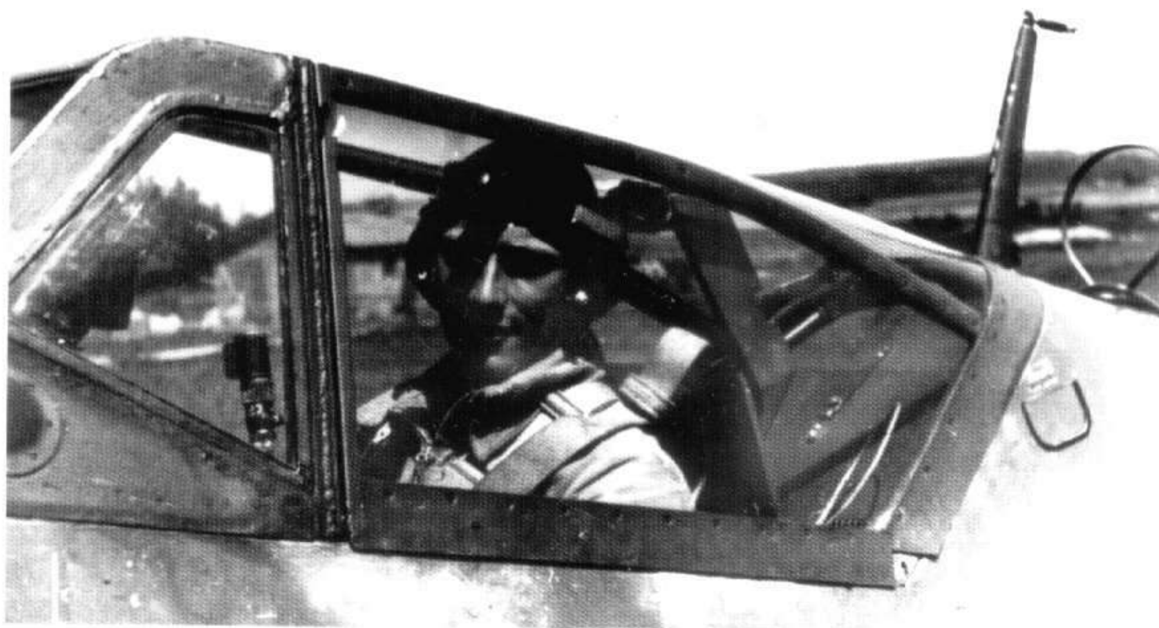
321: The Erla type hood on this late-production Bf 109 reveals the crude welding around the windshield framing and the generally heavy construction. The rear head armour is obvious as is the extensive use of 66 as an interior finishing colour. It is obvious that the average Bf 109 pilot did not enjoy the same level of visibility as that of a P-47D or P-51D. Camouflage is 74/75/76, while the antenna mast is 70
