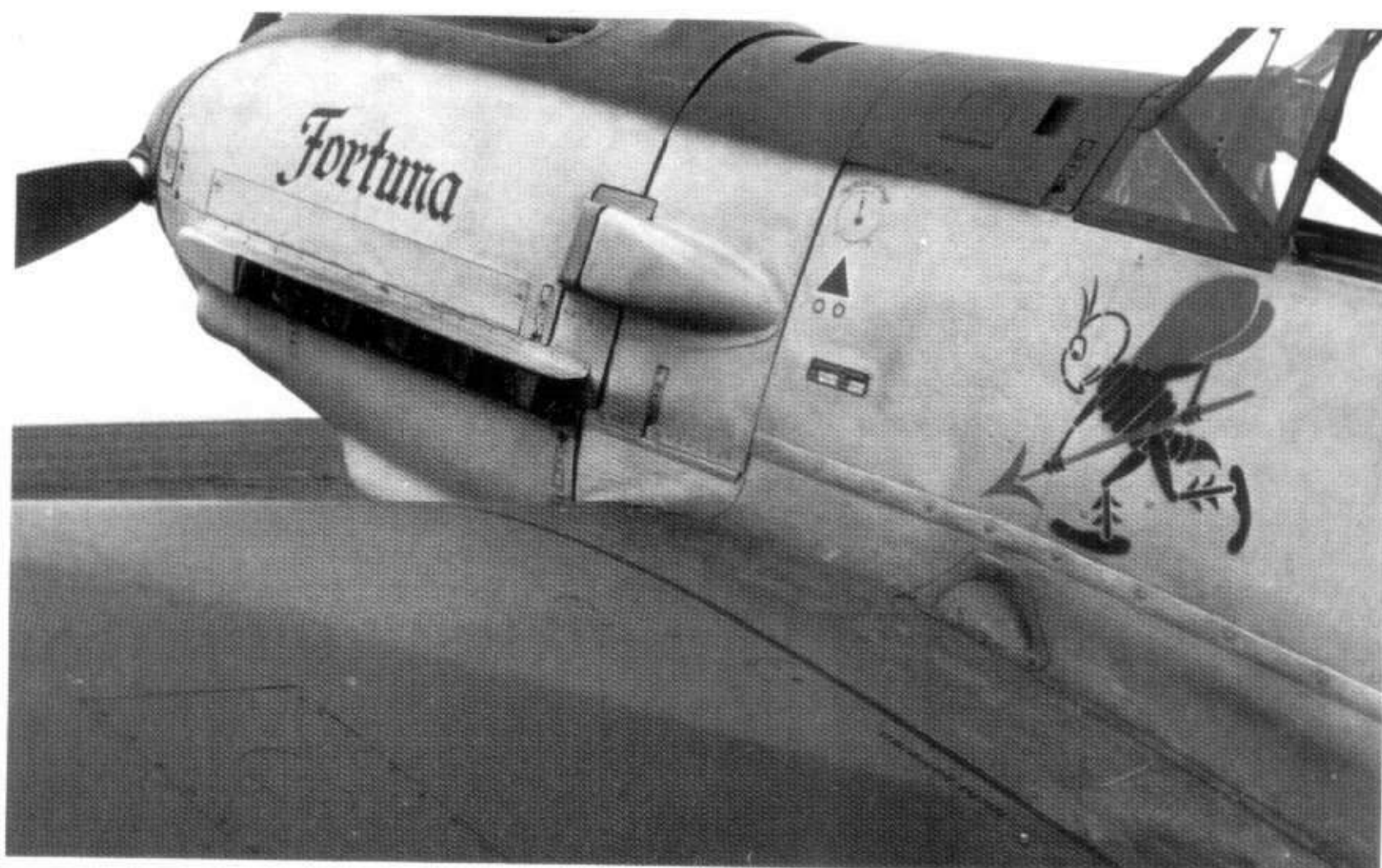
75: This Bf 109E-4 of III./JG 3 is pictured in France in 1940. The aircraft is finished in RLM 70/71/65, the latter being of the later 1941 shade. The intended matt finish to the paint is clearly visible and it is apparent that all maintenance stencilling is still in place. Note the Gruppen 'Stechwespe' emblem is painted in Schwarz 21, with wings and spear in Hellgrün 25
