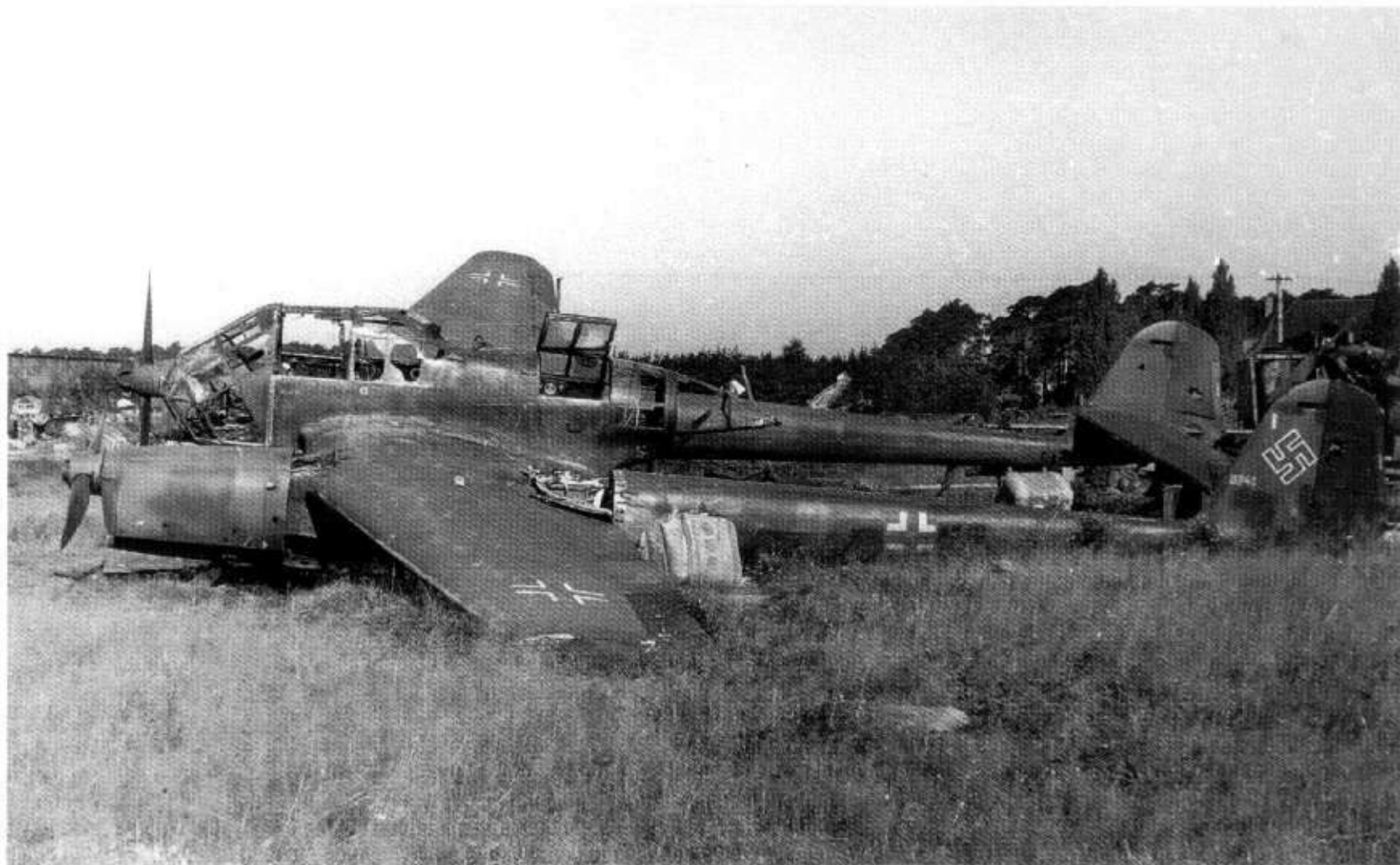
302: Found abandoned at Berlin-Gatow in summer 1945, this Focke-Wulf Fw 189A, WNr 0241, (French-built?) is in standard 70/71 camouflage which has been overpainted in a darker tone where the unit codes, theatre bands and a unit emblem had been. All national insignia are of the correct white maximum simplified type
