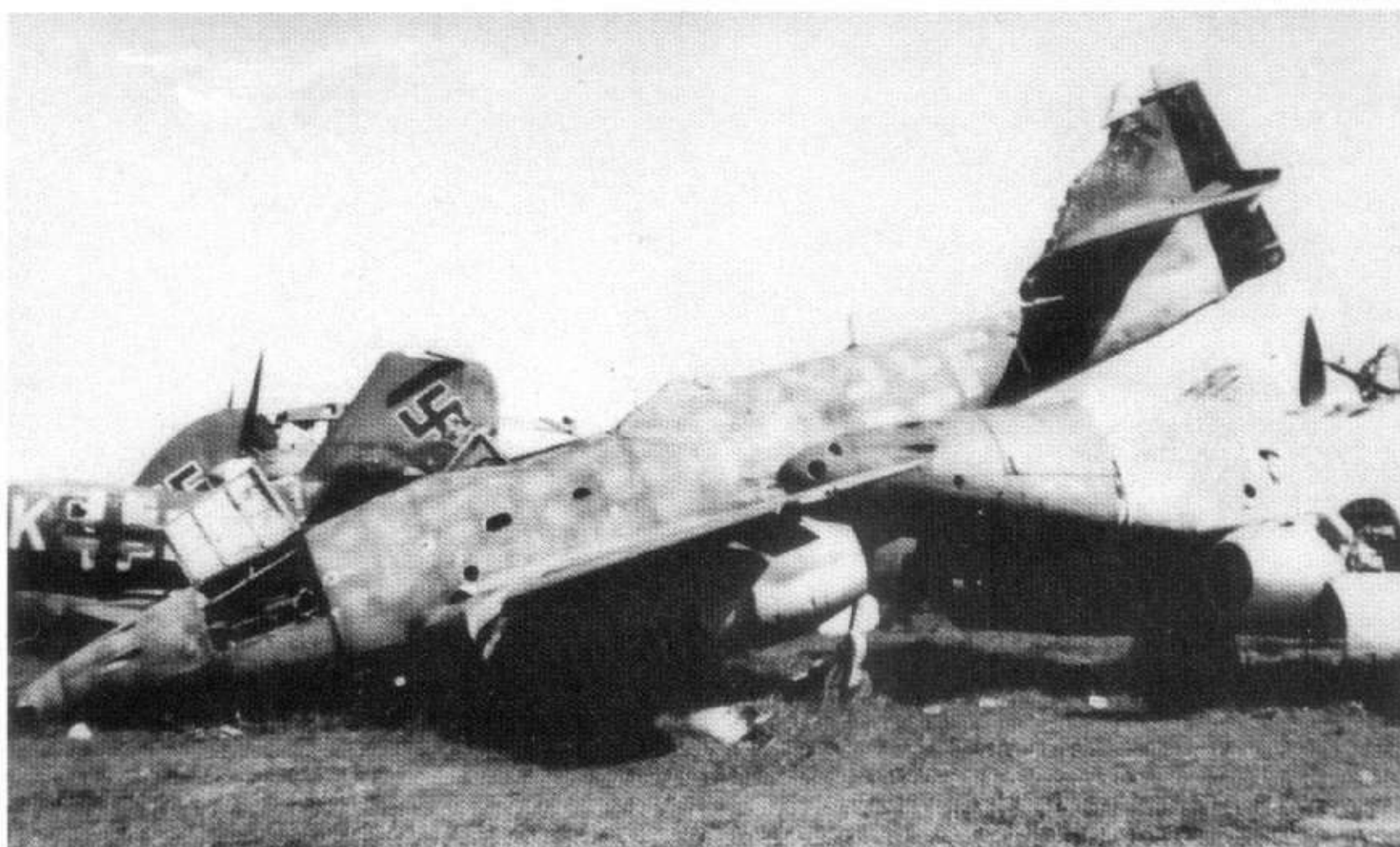
332: Wrecked Me 262A-2a, WNr 111685, once of I./KG 51, whose barely discernible code, '9K+FH' can just be made out. It is apparently finished in a thinly-applied coat of RLM 82, the rudder carrying a solid coat of this colour. Overall on the fuselage are regular light blotches, possibly of 76, but more likely metal, primer and filler on joint lines showing through a very thin coat of weathered paint. Tip of the nose and fin are white, the staffel colour, to match the white 'F'. The werknummer is some 200mm high, while the Balkenkreuz should be black against the light background
