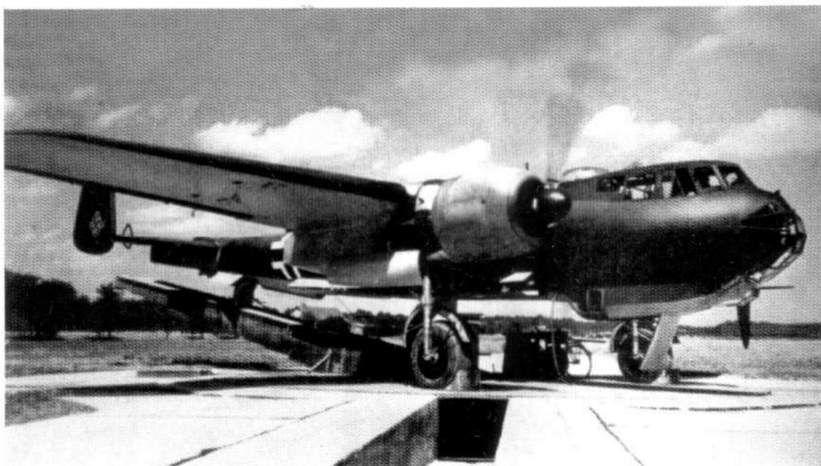
100: A Dornier Do 217E on the compass-swinging platform at Frierichshafen-Löwental prior to delivery to the Luftwaffe. The machine was supposed to be finished in RLM 72/73/65 but appears to be overall 72 on the uppersides. The starboard engine cowlings is still in primer finish. While the fuselage cross and swastika are in place, there are no underwing markings showing. These may yet have to be applied or may have been censored from the picture
