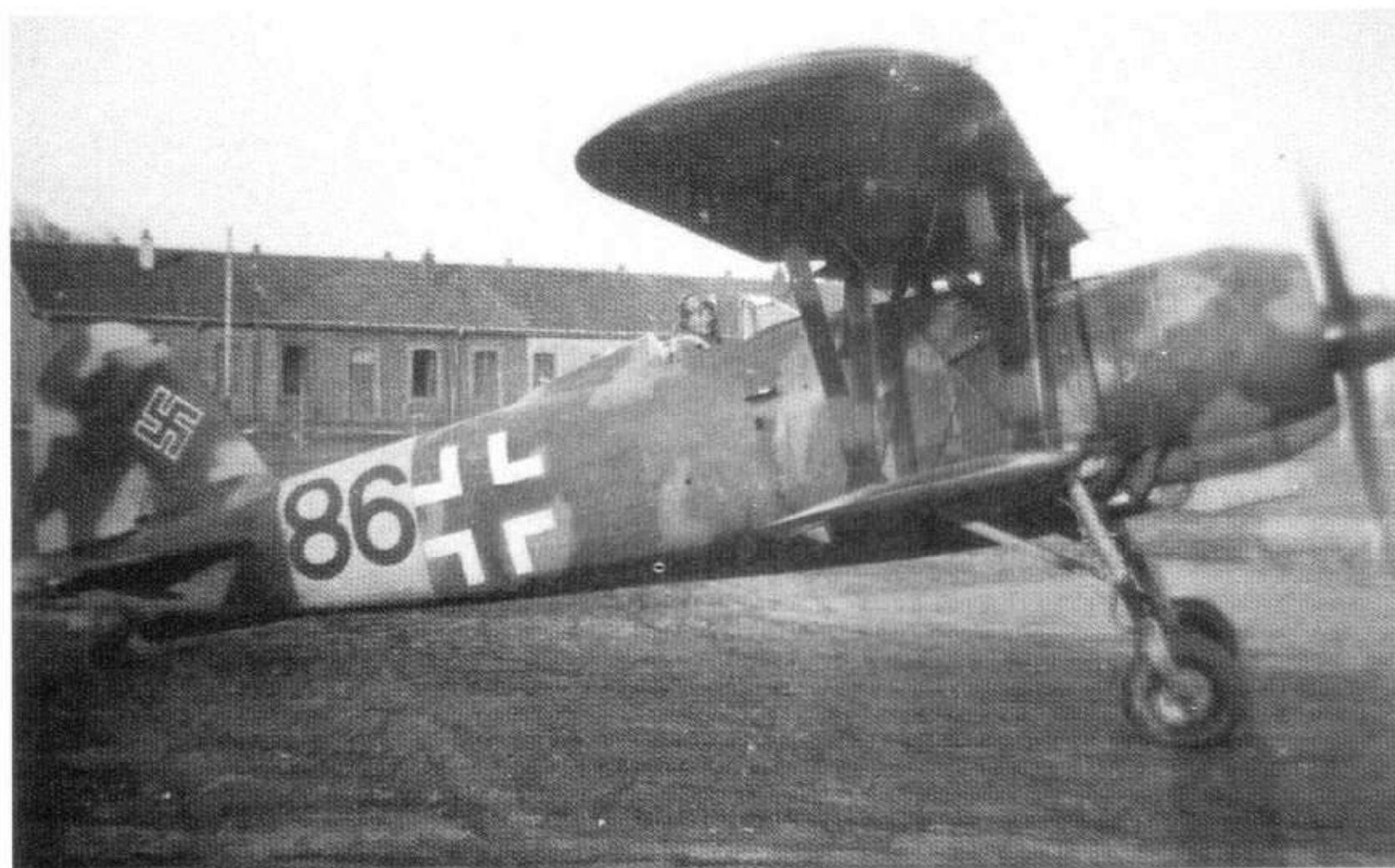
130: As the war progressed many unusual aircraft were press-ganged into Luftwaffe service, among them this Fiat CR 42 used for training. Camouflage on 'Black 86' is RLM 71 with 02 blotches and an 04 Gelb band. The national markings are of the late-war maximum simplified type. Note that the wheel fairings have been removed to simplify maintenance
