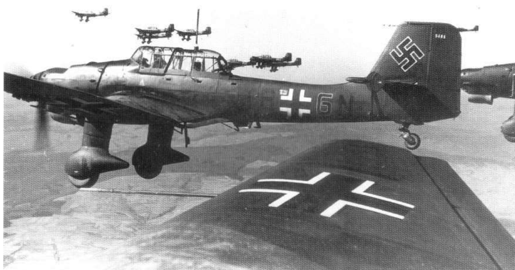
70: Junkers Ju 87B-2s of 5./St.G.2; T6+GN, WNr. 5486, in the foreground, somewhere near Bonn in winter 1939-40. All wear standard 70/71/65 with all visible swastikas and Balkenkreuze with thin black borders. The letter 'G' had a thin white border and unusual proportions when compared with the official style shown on page 151
