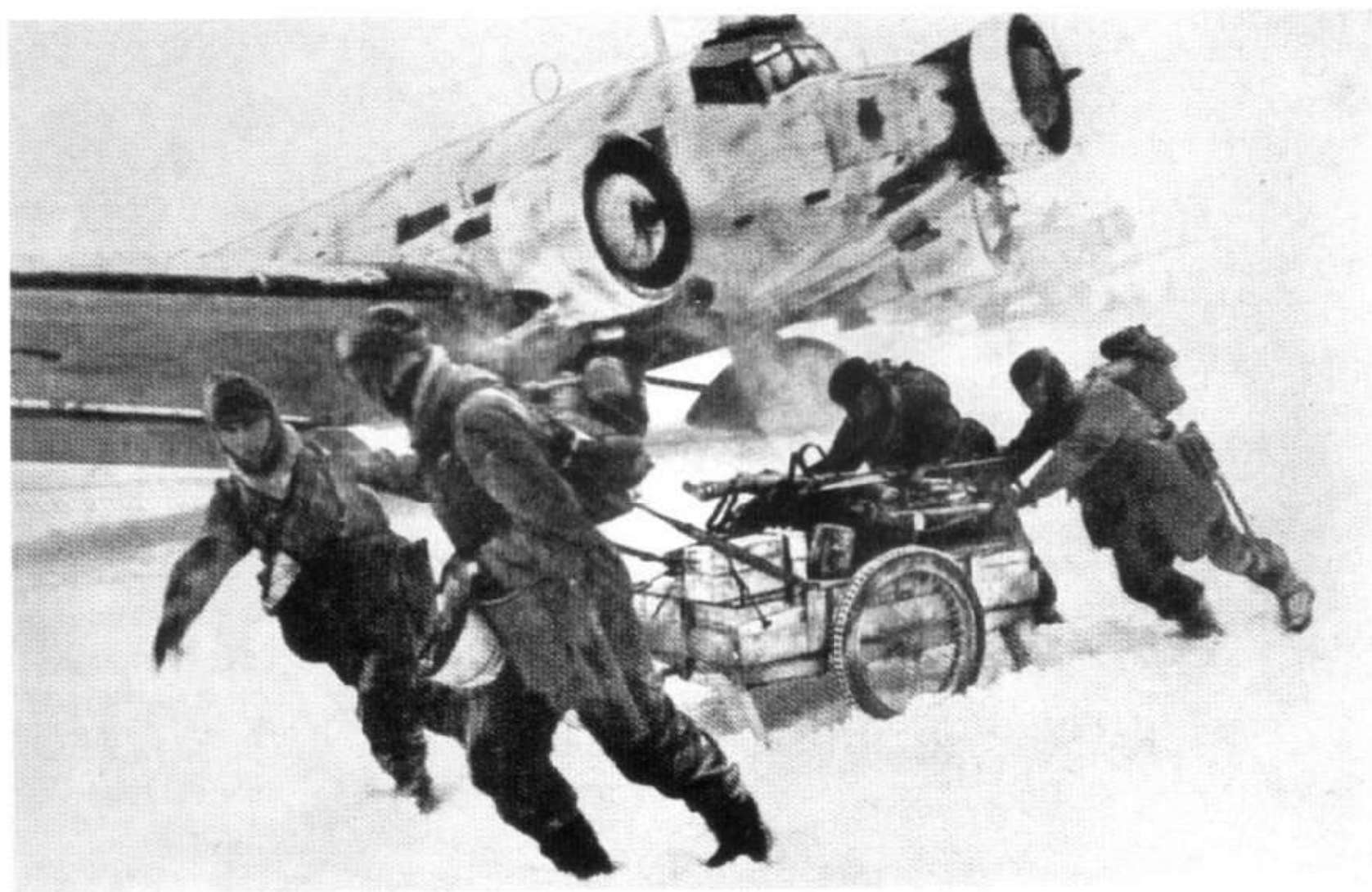
196: Ground troops unloading a Junkers Ju 52/3m, probably from BFS 2, whose pig emblem can be just made out forward of the cockpit, in a typical Eastern Front winter setting. The aircraft wears a thinly applied coat of temporary white paint, either Ikarin A2515.21 or 7126.21. The paint is already wearing away from the leading edges of the wings. As the losses mounted in the east, many experienced crews and instructors from the flying schools were pressed into running aerial supply missions
