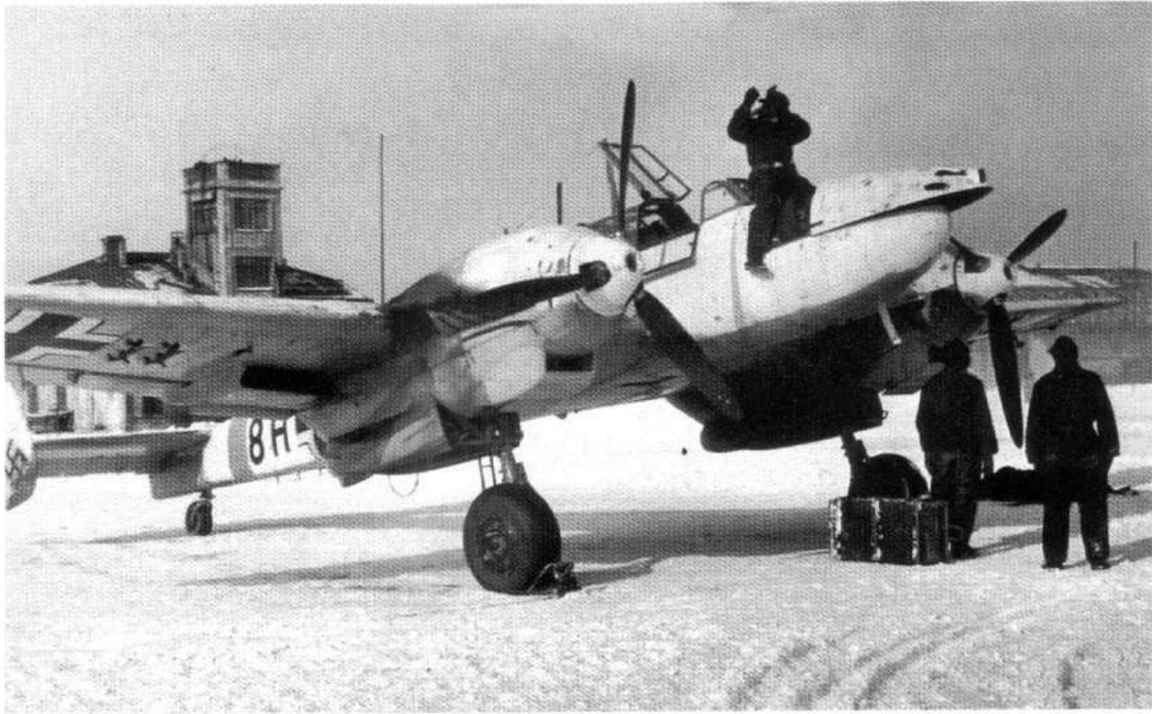
200: Pictured in the winter of 1942-43, this Messerschmitt Bf 110E-3 of Aufkl.Gr(F)/33 (possibly 3. Staffel) has been recently finished in temporary white snow camouflage, applied by brush. Yellow undersides to the engine cowlings have also been recently applied, note the contrast between the underside RLM 65 (or 76)
