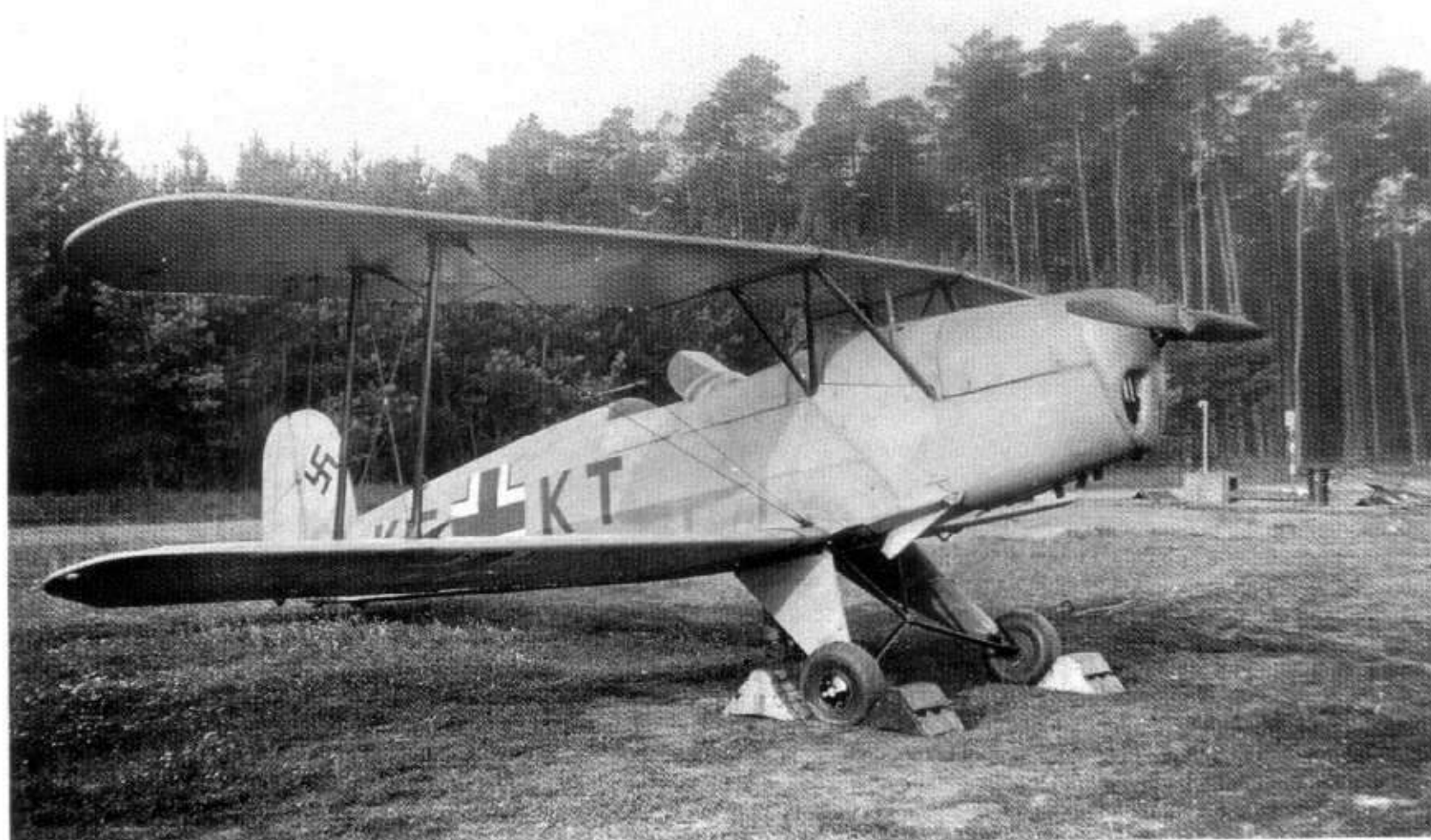
112: Wearing an overall RLM 02 Grau finish, this Bücker Bü 131, KE+KT, of LKS 2 at Berlin Gatow in 1941, is a typical trainer of the early war years. The angle of the light makes the fuselage markings appear unusually pale (AMC)
