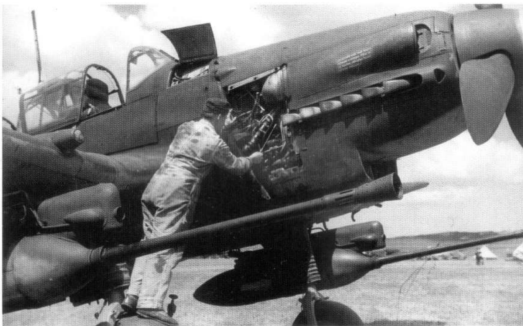
106: A fitter attending to the engine of a Junkers Ju 87G-1 tank-hunter. Although the official scheme was for the classic RLM 70/71/65, the aircraft shows signs of re-painting around the stencilling on the air intake which may indicate that it is now one overall colour. A spinner ring in yellow(?) the staffel colour, can be just made out. The completely matt finish is worthy of note
