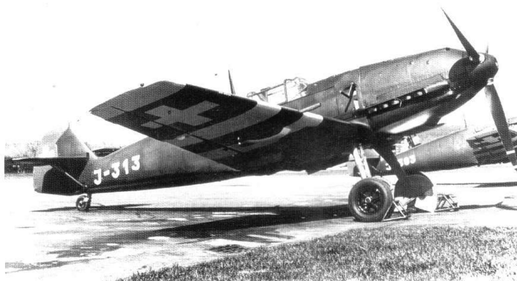
263: 'J-313', WNr 2161, was one of the earliest Bf 109E-3s to be delivered to the Swiss Flugwaffe (on 20 June 1939) and was finished in standard 70/71/65, as were all the Bf 109Ds and Es delivered to Switzerland. As seen here in post-war style markings with the red and white wing bands, the original finish has been overpainted an overall green. The later Bf 109Gs sold to Switzerland were all finished in entirely standard 74/75/76 in accordance with the OS Liste
