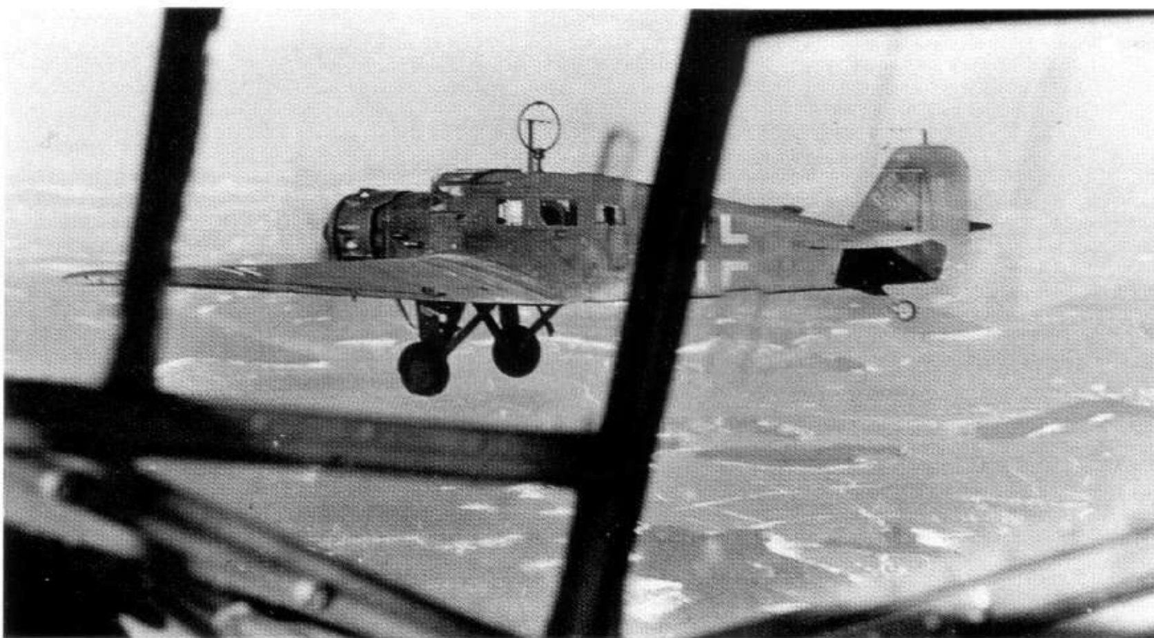
303 Left: A well-worn Junkers W34. No colour demarcation is visible, therefore it is very likely that the aircraft was finished only in 71/65. Swastika and Balkenkreuz are the 'late' style noted on page 155, in white against the dark camouflage
