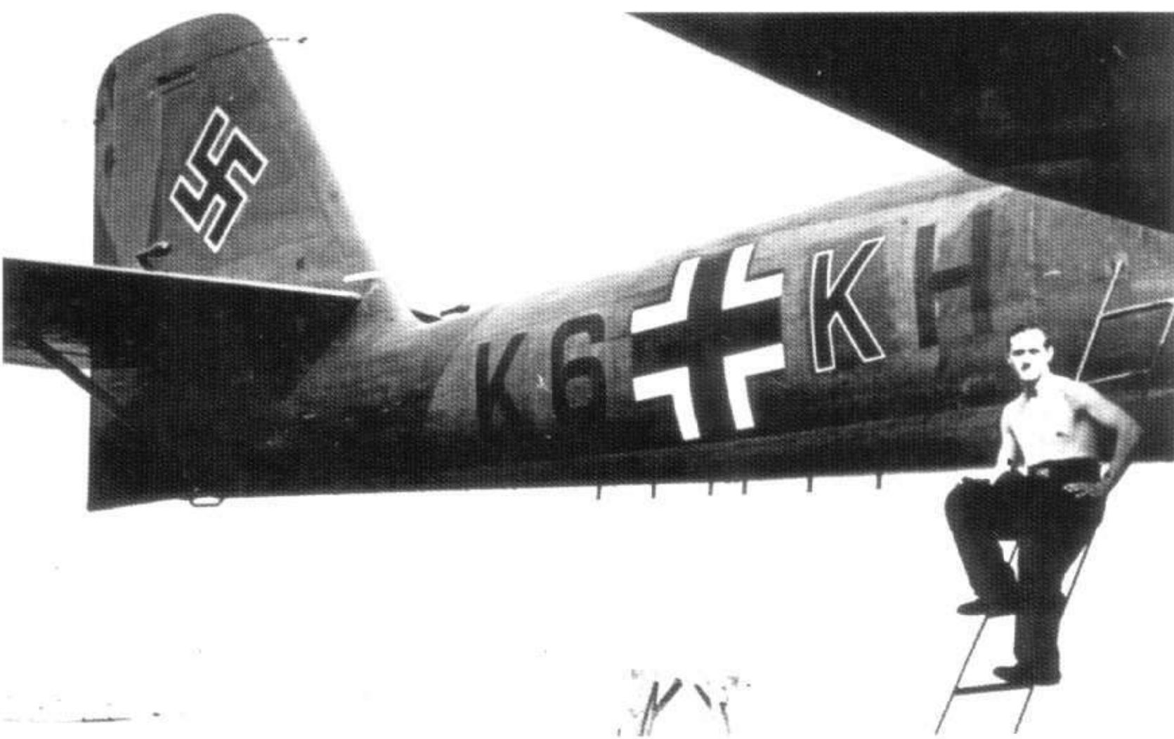
177: The fuselage of an Heinkel He 115, T6+KH, WNr 2503(?), of 1./Kü.Fl. Gr 406 based in Norway, showing the early style swastika and Balkenkreuz with the thin black border. All letters were painted in black, the letter 'K' with a white border has apparently been recently painted over an earlier letter. The well worn camouflage is 72/73/65
