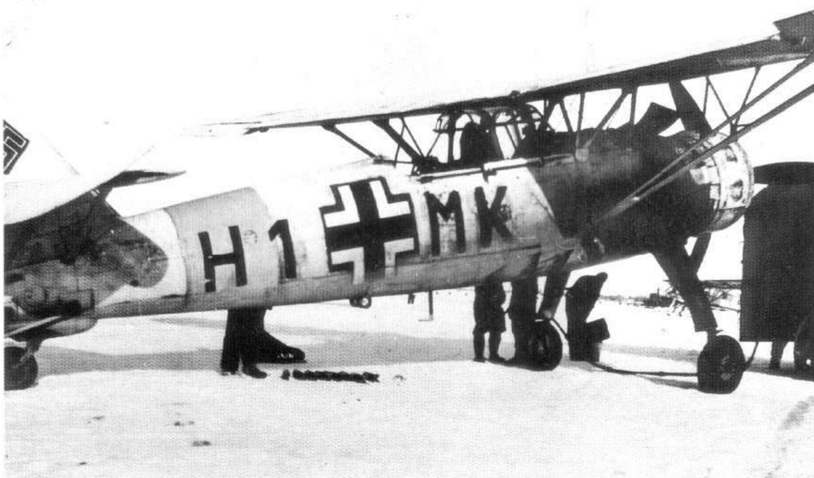
208: This Henschel Hs 126B-1 of Aufkl.Gr(H)/12, 'H1+MK', has had the temporary winter camouflage roughly applied by brush with all national and unit markings left clear. As usual, the finish is rapidly wearing away where it is exposed to the dirt thrown up by the landing gear and the ground crew clambering over it. The yellow fuselage band is rather wider than required by regulations and the unit code is oddly spaced
