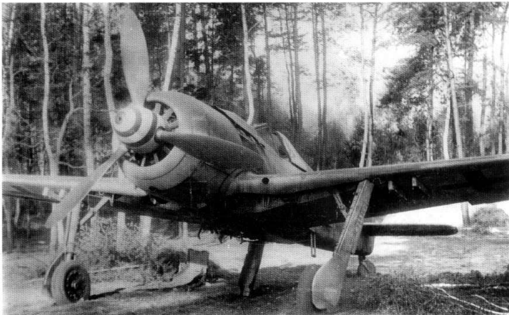
117: Left abandoned at Pardubice in Czechoslovakia, this Fw 190F-8/R1 was once in use with SG 77. Fitted with ETC 71 bomb racks, the very dull finish suggests that the underside is in a grey-green variant of RLM 76, while the upper-sides are believed to be in RLM 81/82. The spinner is apparently finished in non-standard black with a very wide white spiral
