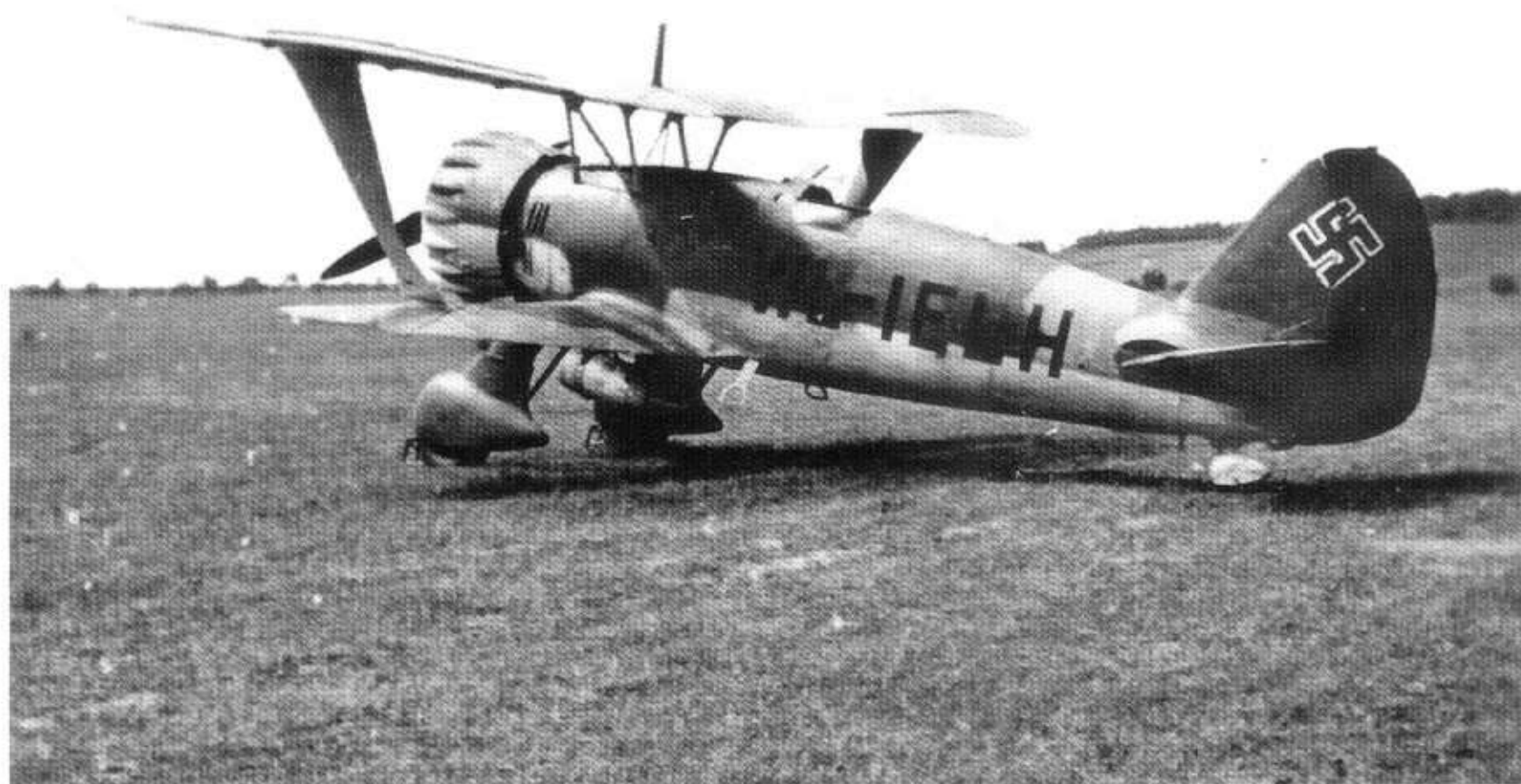
285: With effect from 1 January 1939, all Luftwaffe aircraft which were not in front line service but were on the strength of training schools and the like (see page 150) were to carry a civilian registration with a 'WL' (WehrmachtLuft) prefix. These remained in use until about March 1940. This Hs 123A is obviously in use with a training school as it is coded WL-IELH. Camouflage is the 61/62/63/65 scheme. Note the swastika has been modified in accordance with the instructions issued in January 1939 (see page 150) by having the red band over-sprayed
