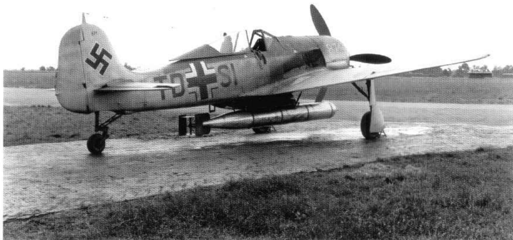
193: Bearing the Stammkennzeichen 'TD+SI', this is WNr 871, the first of two Focke-Wulf Fw 190A-5/U14 torpedo-bomber prototypes. Differing from the standard model mostly in terms of undercarriage strengthening, an extended tailwheel and a larger fin, it appears to be finished in the standard RLM 74/75/76 fighter colours. Markings are entirely standard for the mid-war period
