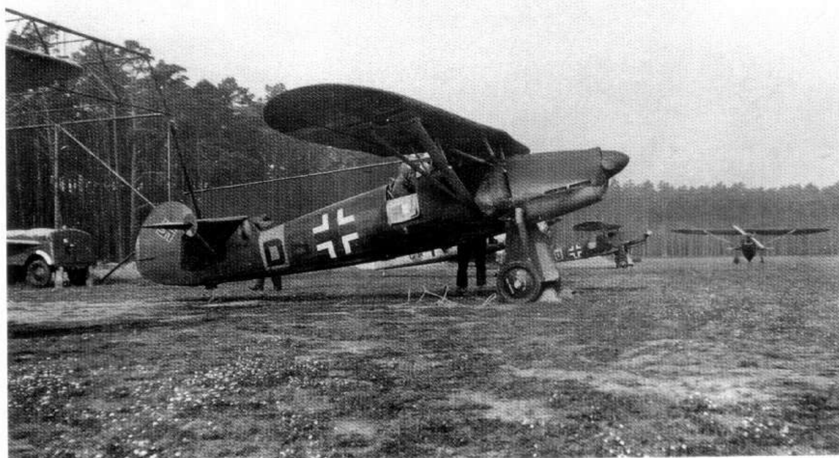
113: A Focke Wulf Fw 56 of LKS 2 at Reinsdorf in 1942-1943 in a 70/65 camouflage. This is a good example of an aircraft camouflaged by the unit following the issue of an order on 21 January 1942 calling for such finishes to reduce their vulnerability to roving RAF fighters. Coded DB+??, it has a yellow fuselage band and lower wing tips. Behind is an overall grey example, CA+??, and further back another green finished aircraft, DB+??. Balkenkreuz and swastika are of the mid-war style (see page 155)
