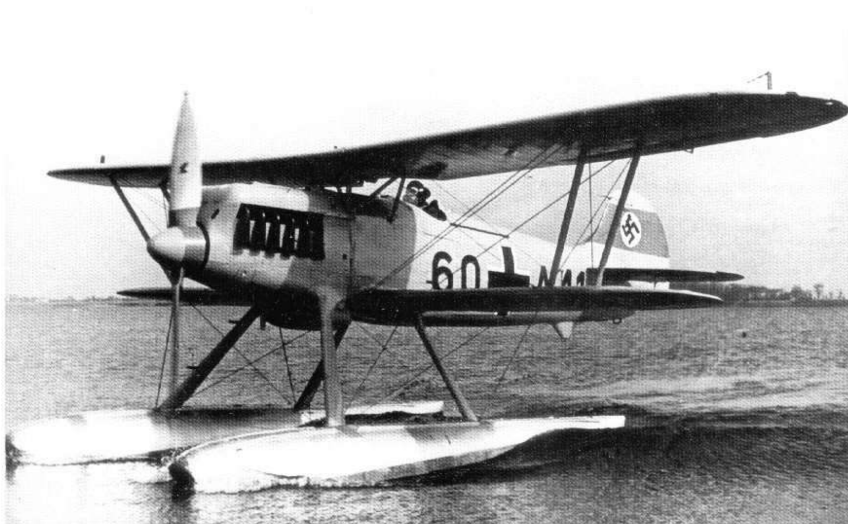
165: A photo of the very rare Heinkel He 51B-2 with floats. The aircraft was painted in the pre-war light grey L40/52, while the floats received a final coat of Silber 01 for maximum protection. All markings date from the 1936 period, the '60+A11' code indicating that the machine, 'A', is in service with 1/Küstenjagdgruppe 136, based at Kiel-Holtenau in late 1936. Note the manufacturer's trade mark on the propeller blade
