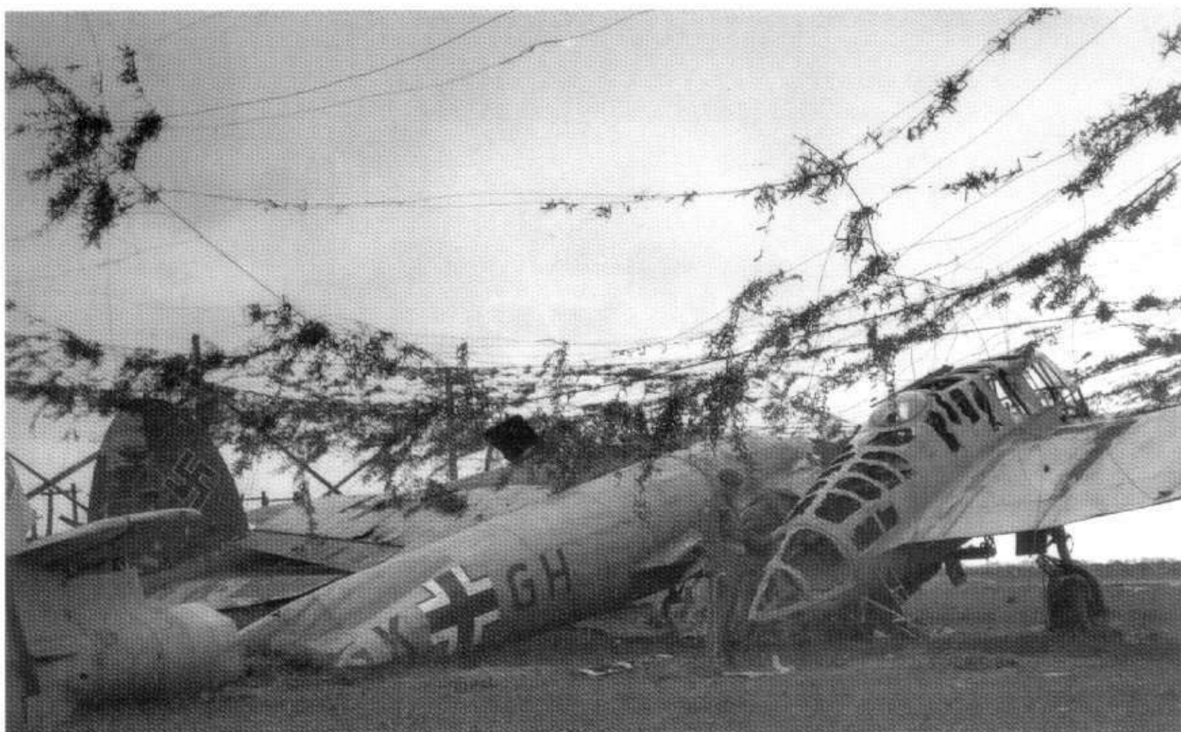
125: This Blohm and Voss Bv 141B is something of a mystery as only five of this type were supposed to have been produced but as far as is known, none bore the code GK+GH. Painted RLM 02 overall, the aircraft wore the mid-war type of national insignia when it was found abandoned at the Blohm and Voss works at Wenzendorf in May 1945. The simple camouflage could indicate that it was either left over from a training school or was being refurbished for operational use
