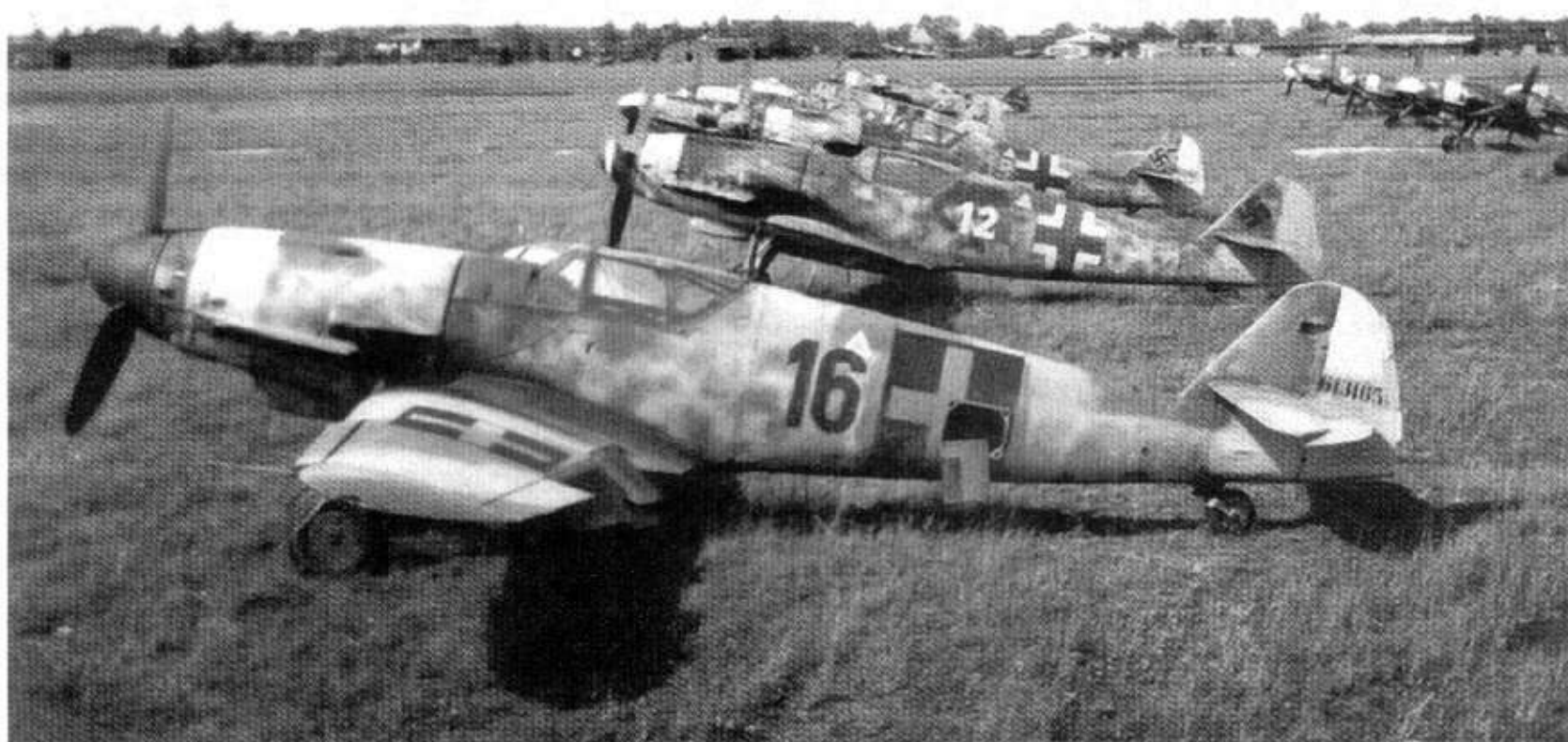
118: Abandoned aircraft at Munich-Riem in May 1945. Nearest is a Wiener-Neustadt built Bf 109G-10, WNr 613165, 'Black 16', in Hungarian markings. Probably finished in RLM 75/83/76, the spinner and a ring around the cowling are in RLM 70. Immediately to the rear is another yellow ring. The Hungarian national insignia follow the requirements for simplification like those of the Luftwaffe. Further back, ex-Luftwaffe owned 'White 12' and red or green '19', WNr 613195, show further variations in national insignia. Both have yellow cowling bands
