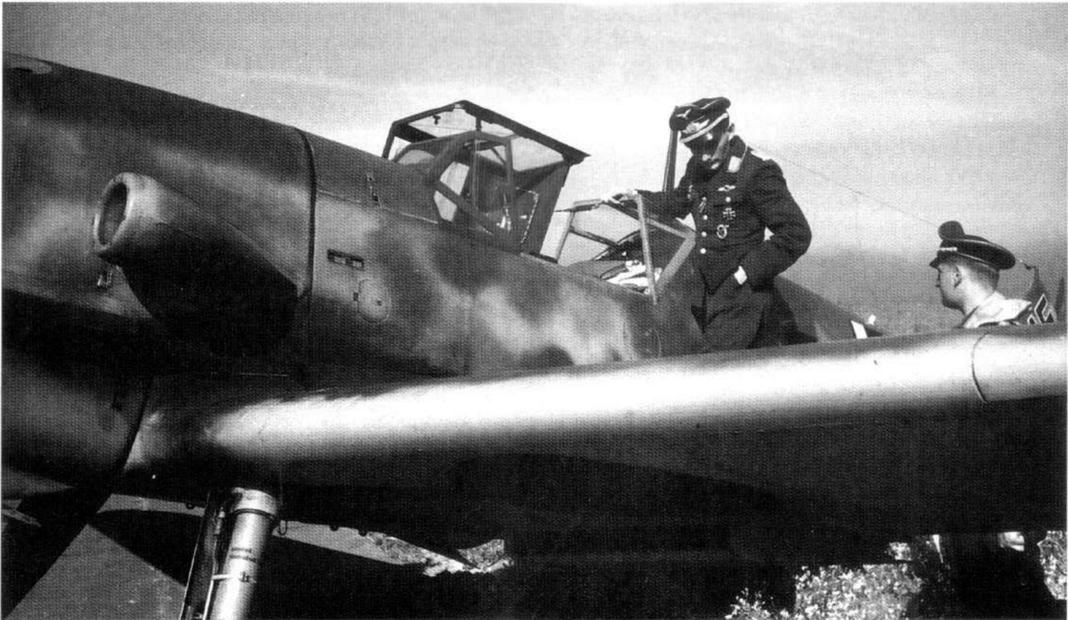
355 Below: The matt finish to the 74/75/76 camouflage on this Bf 109F-4 reconnaissance aircraft of I.(F)/122, F6+WL, is as it should be according to the regulations. The pattern is as the OS List except that the underside 76 has been brought up over the wing leading edge. Note the RLM Grau 02 of the undercarriage leg and the 66 to the cockpit interior and head armour
