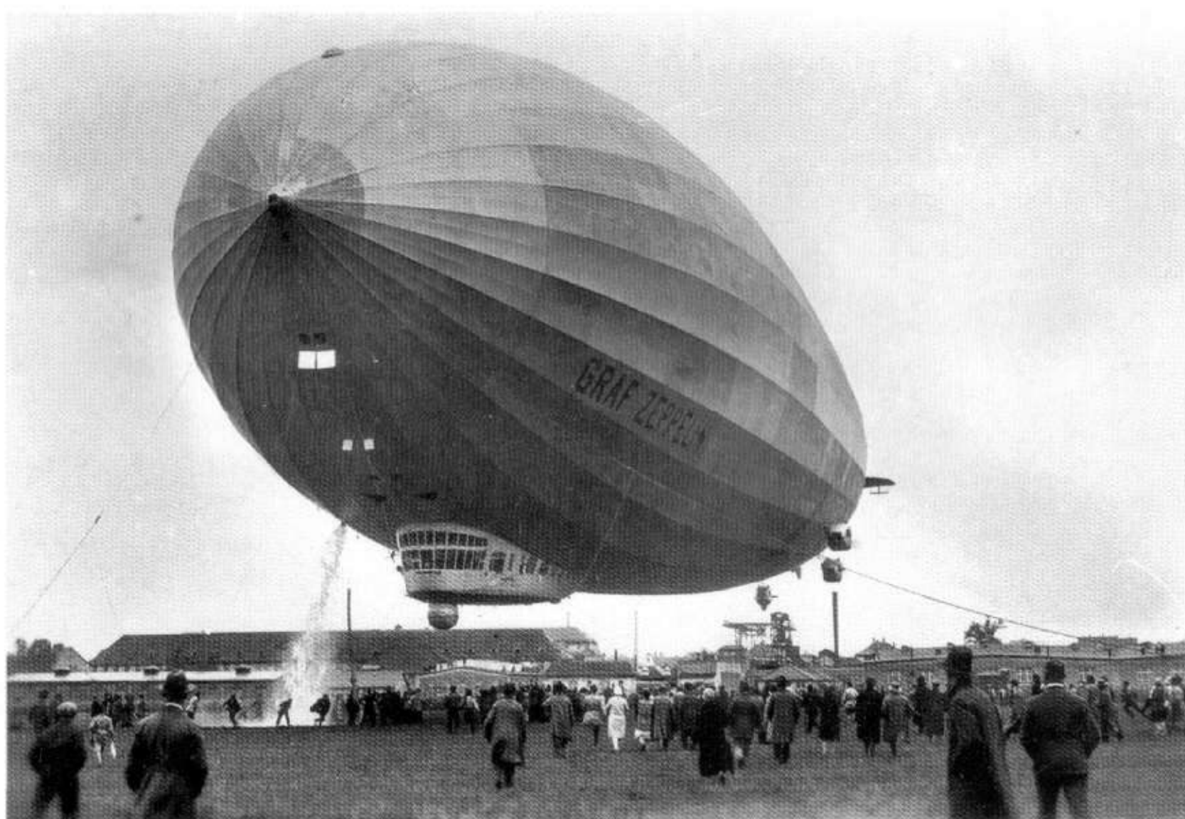
33: LZ127, Graf Zeppelin, discharging water ballast over some unfortunate members of the crowd watching as the vessel is manoeuvred to its mooring mast. The dull finish to the envelope reveals how dull and weathered the protective coating quickly became, as related on page 34
