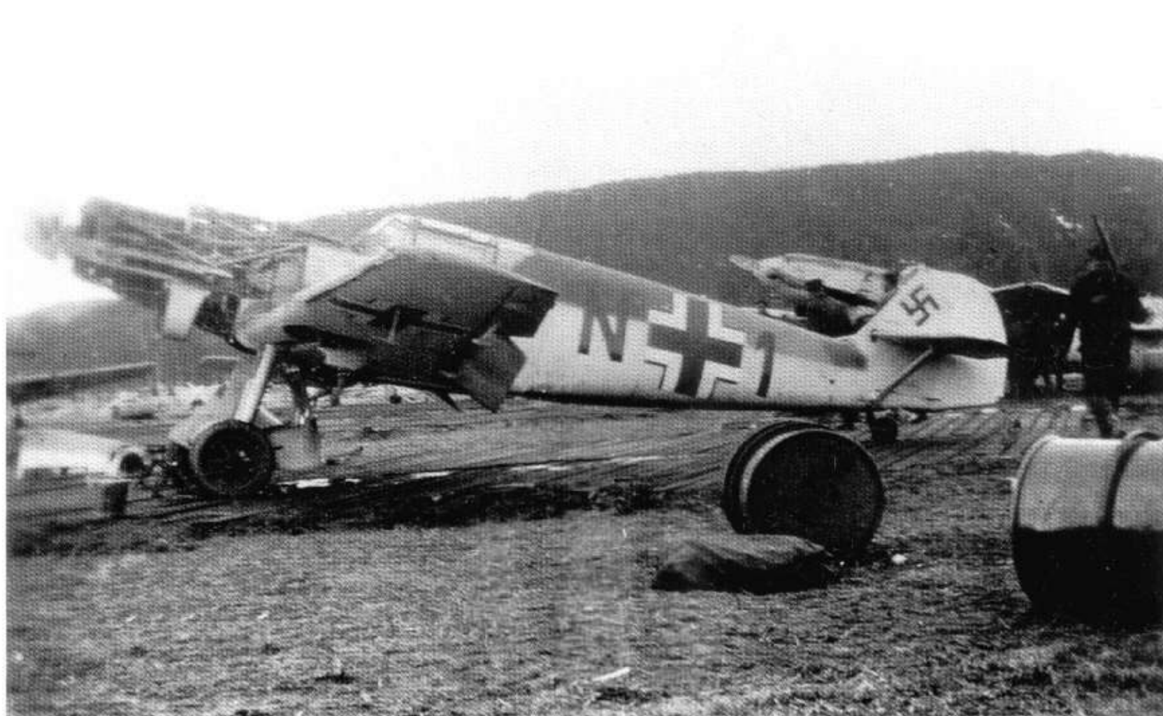
229: A Bf 109D, N+1, of 11(N)./JG 2 pictured at Vaernes in Norway sometime between May and late August, 1940. At this time 'twilight' fighter units were just being formed as additional staffeln to fighter gruppen. These aircraft were identified by the letter 'N'—'night'. This is probably the Staffelkapitän's machine, finished in 71/02/65. Balkenkreuz and swastika are of the 'early war' style with thin black borders, the number and letter are red
