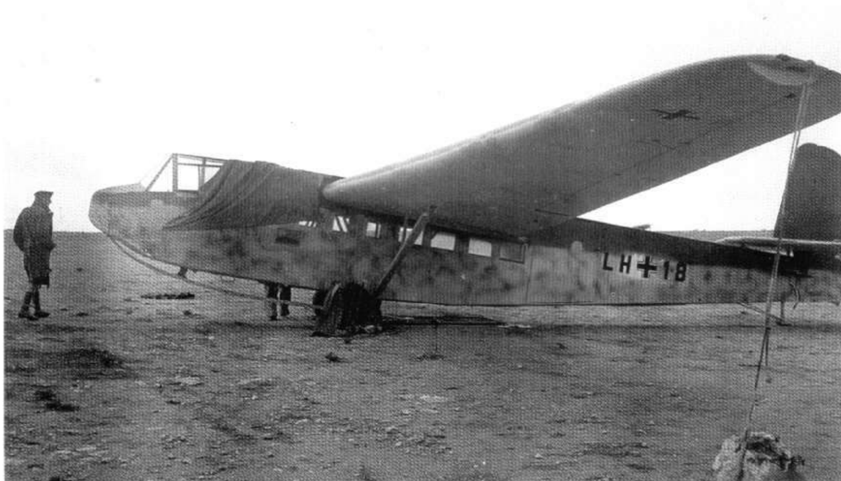
254: This DFS 230 from LLG I or II was also abandoned in the Wesern Desert. Finished in the same colours, probably 70/71/65, as others of the type, it also carries unit and national identity markings. The very small size of the markings was probably chosen to both enhance the confusion caused by glider landings among enemy positions and also to assist the camouflage
