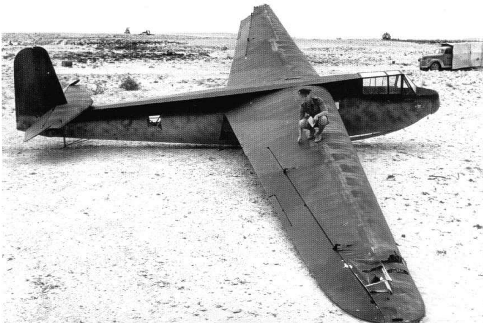
253: A starboard side view of the same DFS 230 seen in photo 252 shows it to be finished in at least two, and possibly three, colours on the uppersurfaces. Most likely 70/71, the very matt finish is noteworthy, as is the total absence of any national or unit markings
