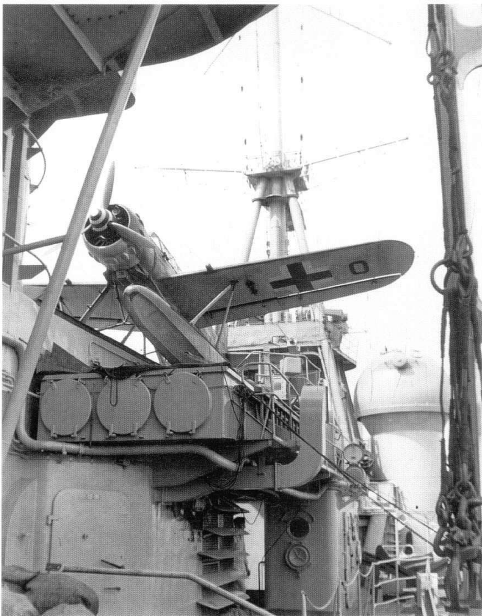
194: An unusual view of Arado Ar 196, T3-OM, of BFGr. 196 aboard the catapult of the Kriegsmarine heavy cruiser Prinz Eugen at her surrender in Copenhagen at the end of the war. Markings and camouflage of the Ar 196 remained much the same throughout the conflict. The major difference here is the white spiral on the spinner, which was required on all Luftwaffe operational aircraft as a recognition marking from 20 July 1944
