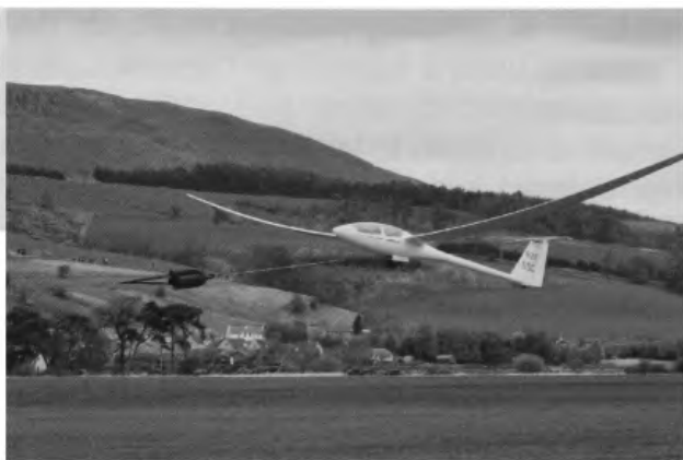
The SGU ASH-25 being winch-launched. Note the lift-generated curvature of the 25 metre wing-span..
