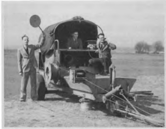
The "Wild Winch" - Ex balloon winch converted for glider launching with Lt Stevenson with the signalling bat, David Hendry "driving" the winch and Maurice Berry listening to the launch instructions.
