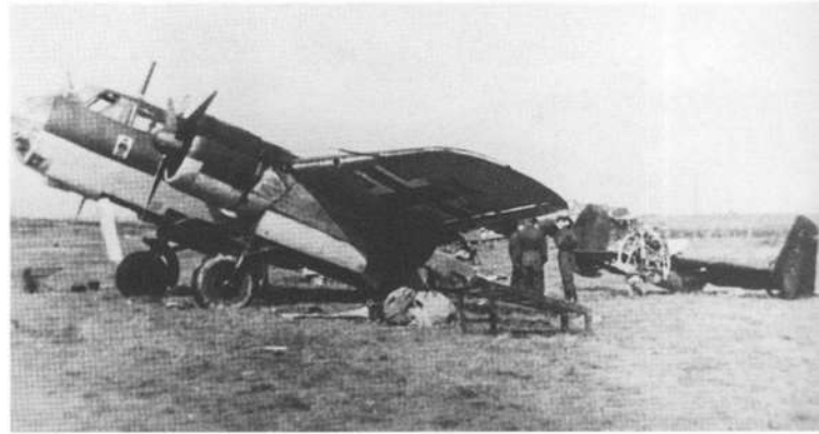
Dornier Do 17 Z-2, W.Nr. 1169, coded 5M+K of Wekusta 26 at Smolensk, Russia on 16 September 1941. The rear fuselage was broken off either when the aircraft landed (had suffered damage from enemy fire during a mission) or by an enemy bombing attack on the airfield. The Dornier was painted in a standard 70-71-65 camouflage scheme and had the Wekusta owl emblem under the cockpit.
