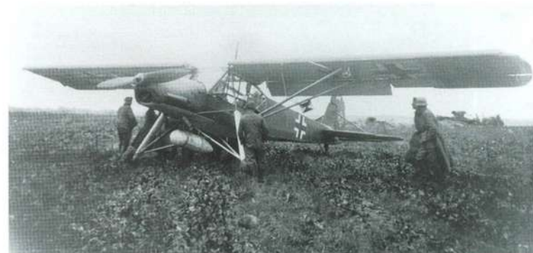
This Fieseler Fi 156 C-3 'Storch', W.Nr. 5837, coded NB+YN, belonged to the Flugber./Fliegerkorps VIII and was the personal transport of Gen.von Richthofen. It had a 70-71 splinter upper surface scheme with 65 Light Blue undersides, yellow underwing tips and a command pennant on the tail.
