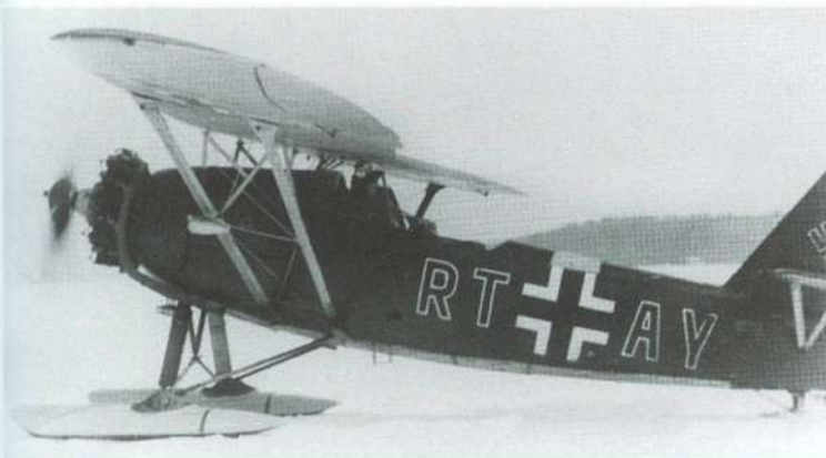
There was a stark contrast between this dark-coloured Heinkel He 46 C, coded RT+AY and the surrounding snow. The aircraft was assigned to the Flugber.RLM and had a splinter 70 Black Green and 71 Dark Green uppersurface and 65 Light Blue under surfaces. It had a yellow fuselage band and code letters outlined in the same colour – notice it also had skis in place of the normal tyres.
