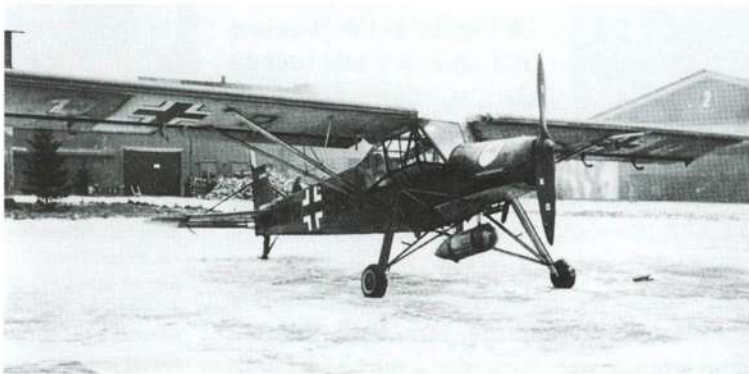
This 'Storch' was assigned the Verbandskennzeichen 1R+SH and belonged to the Kurierkette AOK Lappland in Finland from 1941 to 1944. The Fi 156 C-1, W.Nr. 4248, had a very weathered and worn upper surface camouflage so it is impossible to determine if it was a 70-71 splinter pattern although that is most likely. The under surfaces were 65 Light Blue and it had yellow underwing tips but no fuselage band.
