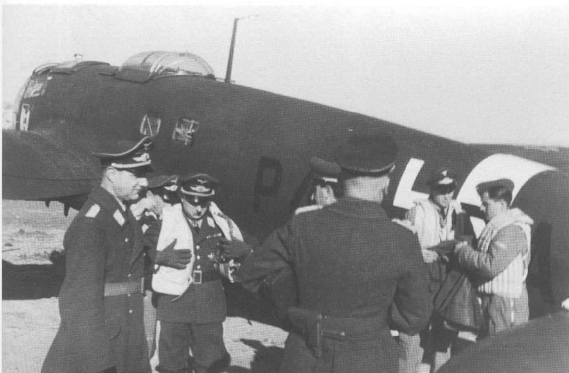
This Heinkel He 111 H-4 coded P4+BA was assigned to the Korps Führungskette/X.Fliegerkorps. It was painted in a standard RLM 70-71 splinter upper surface camouflage scheme with 65 Light Blue undersides. It also had a white fuselage band and an emblem just below the cockpit. The date and location are unknown.
