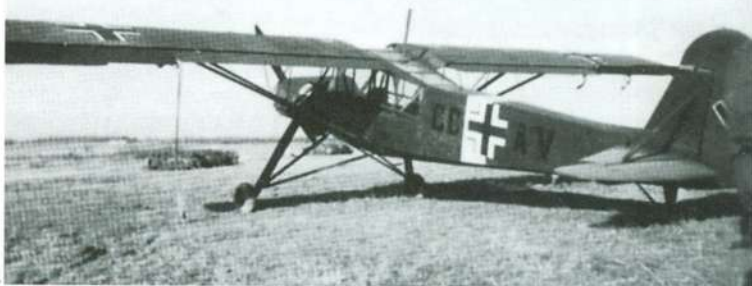
Parked in Russia in October 1941 when the photograph was taken, this Fi 156 C-1 (notice the flat rear upper cockpit glazing), with the code CC+AV, was assigned to Verbindungsstaffel 68. It had a standard factory RLM 70 Black Green and 71 Dark green splinter upper surface along with 65 Light Blue undersides, and a yellow fuselage band in a rather unusual position for a 'Storch'.
