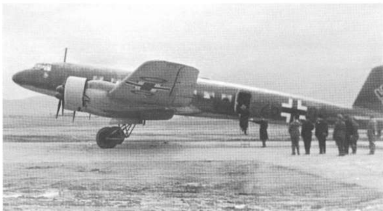
This photograph shows Hitler's personal transport at Salon, France in July 1942. The Focke-Wulf Fw 200 A-09, W.Nr. 3099, coded 26+00 was painted in a standard RLM 70 Black-Green and 71 Dark Green splinter camouflage scheme with 65 Light Blue undersides and belonged to the Fliegerstaffel des Führers. The engine cowlings appear to be painted yellow.
