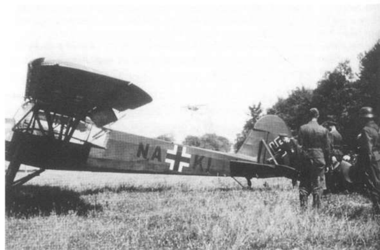
The Fliegerstaffel des Führers also had at least one 'Storch' assigned to it as demonstrated by this photograph showing Fi 156 C-2, W.Nr. 4414, coded NA+KI. The aircraft was painted in a standard factory 70-71 splinter upper-surface with 65 Light Blue undersides.
