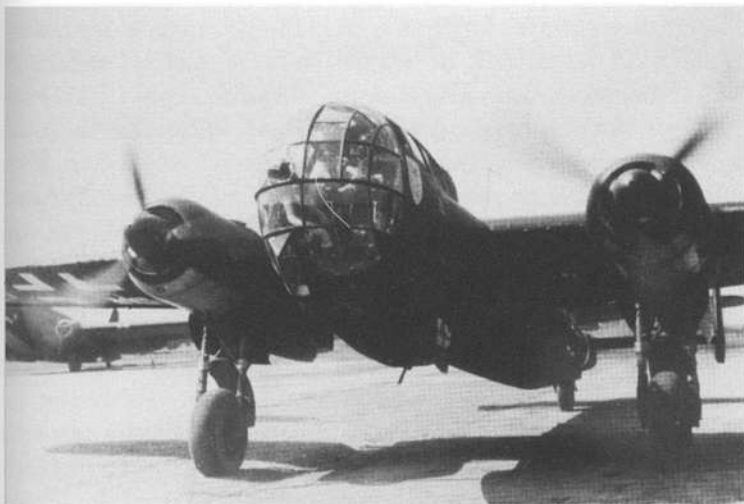
Left: This Dornier Do 217 K-1, W.Nr. 4429, coded F5+FH was part of the Verb.Staffel/Luftflotte 2. It was photographed in Italy during 1943 and was painted in a standard 70-71 splinter upper surface camouflage scheme with mostly black undersurfaces (under sides of the engine cowlings were still 65 Light Blue). This aircraft as well as others in the Staffel were often used by Generalfeldmarschall Albert Kesselring on his trips.
