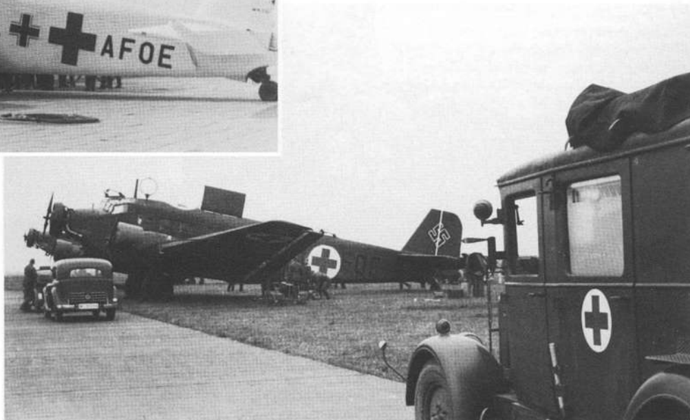
Junkers Ju 52/3m, W.Nr. 1349, coded WL+AF0E from an unknown early Sanitätsflugbereitschaft in Poland during September 1939. It was painted white overall with black engine cowlings and wing exhaust shields. Notice that it still had the normal national insignia in addition to the red crosses in all six positions (fuselage sides and upper and lower wings). It was probably from the predecessor of one of the units that later became Sanitätsflugbereitschaft 7 or 11.
