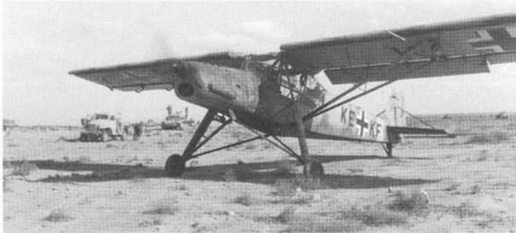
This 'Storch' had a rough splotchy application of Sand Yellow (probably Italian) paint over its European 70-71 factory splinter scheme. The fuselage band is much darker than the white of the Balkenkreuz and could possibly have been yellow with the aircraft being previously on the Eastern Front. The Fi 156 C-2 coded KE+KF, was photographed in North Africa in September 1941.
