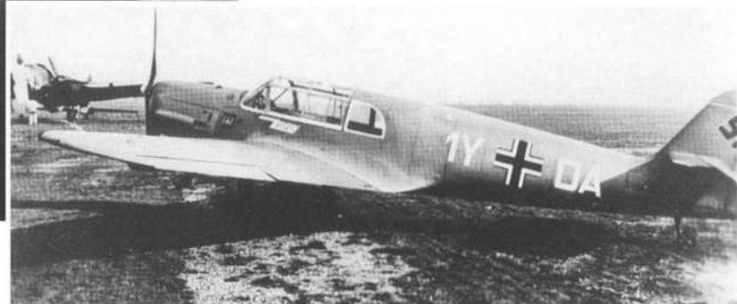
Below: This Messerschmitt Bf 108 coded 1Y+DA, belonged to the Flugber./Luftflotte 4 in August 1939 when the photograph was taken. It appears to be painted in a RLM 02 Grey-Green overall scheme and had white codes with the 1Y+DA also painted on the wing upper surfaces.
