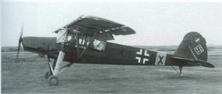
This Fi 156 C-3 'Storch', coded CE+GX, belonged to the Flugber./Luftflotte 1 and was photographed in Russia in late March 1942. It had a typical factory 70-71 splinter pattern along with a yellow fuselage band and underwing tips, plus a command pennant on the rudder.
