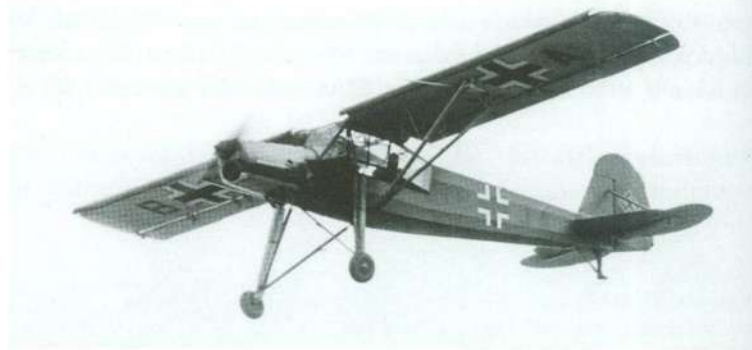
A 'Storch' of Verbindungsstaffel 68 flies low overhead in May of 1941 just before the start of Barbarossa. The Fi 156, BB+JA, had a dark green finish and it is difficult to determine if it was a standard factory 70-71 splinter camouflage or just a single colour. It did have 65 light blue undersides and all black codes.
