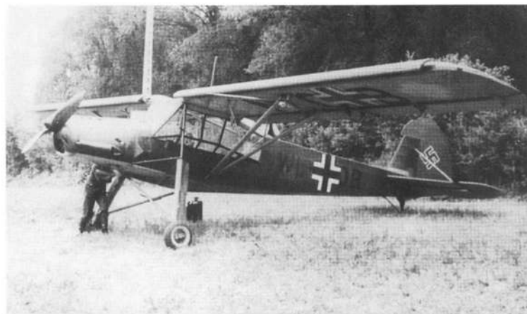
ABOVE: This Fieseler Fi 156 C-1 coded WL-INOB, of the Flugber./Ob.d.L. was parked in a field in France during 1940. The 'Storch' had a typical factory 70-71 splinter scheme with all black codes.
