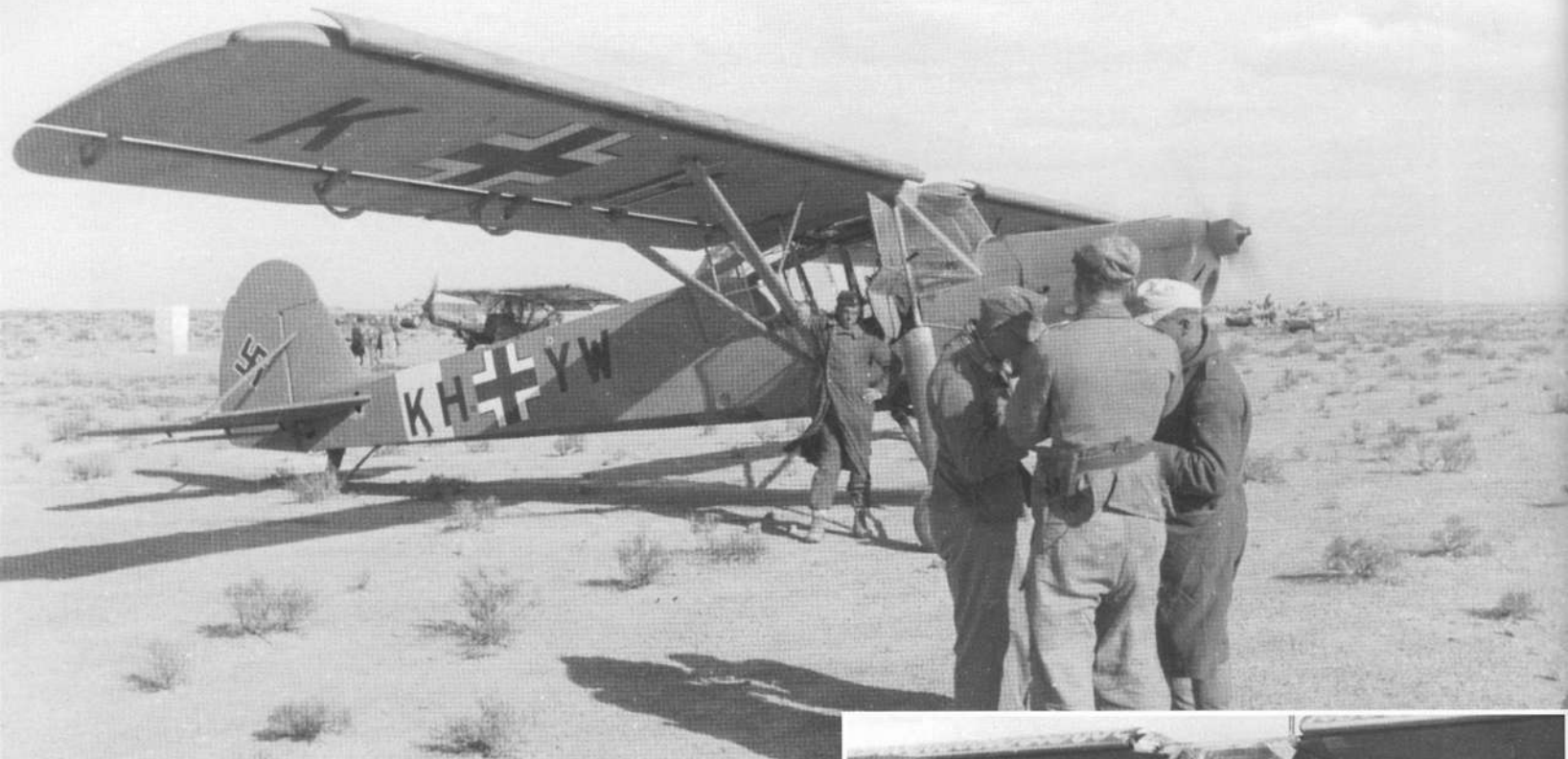
Above: The pilot of this Fi 156 C-3/trop, W.Nr. 5163, coded KH+YW, belonging to Wüstennotstaffel 1, confers with others about his upcoming mission. Taken in Libya in the fall of 1942, the photograph shows well the RLM 79 Sand Brown and 78 Light Blue desert scheme along with the Mediterranean white fuselage band and underwing tips.
