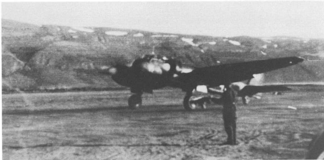
Above: This Heinkel He 111 H, coded 1B+RH was also photographed in the far north on Mezhdusharskiy Island off the tip of Novaya Zemlya, Russia on 20 July 1942. It was painted in a black-green and dark green splinter upper surface with light blue undersides and had a narrow yellow fuselage band. The propeller spinners were painted white.
