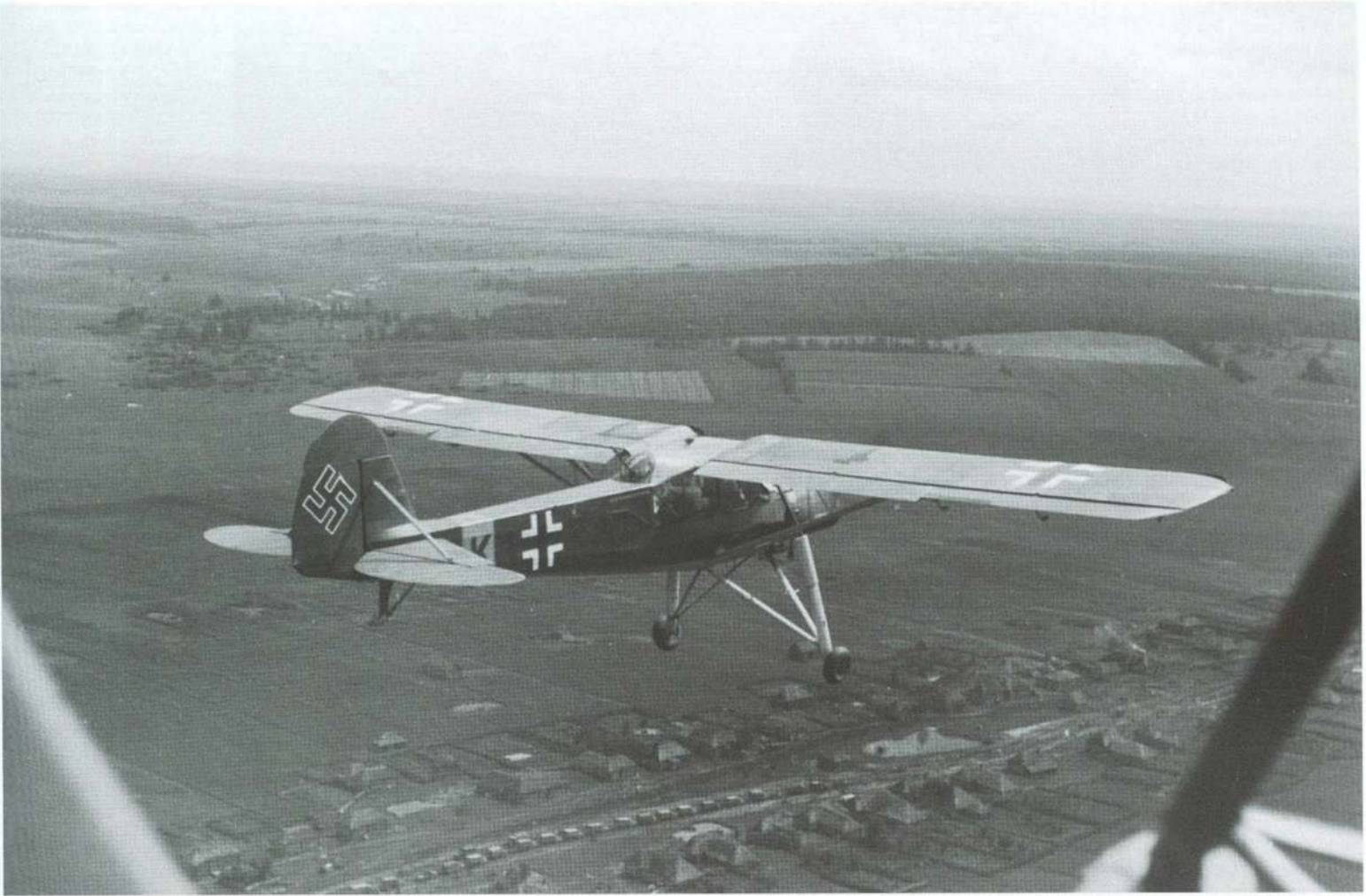
This Fieseler Fi 156 C-3 'Storch' coded K1+RA was assigned to the Korps Führungskette/V.Fliegerkorps and later to the Stab/Luftflotte 6. It is shown flying over Russia during the late summer or early autumn of 1941 and was painted in a standard RLM 70-71 upper surface splinter camouflage scheme with 65 Light Blue under surfaces along with a yellow fuselage band.
