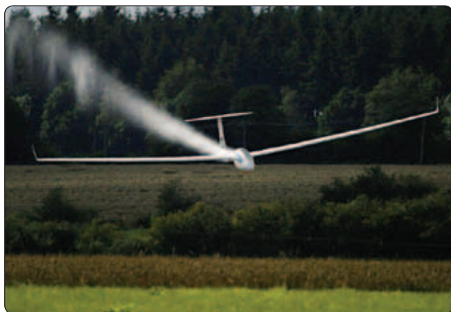
Figure 2-4. Sailplane dropping water ballast before landing.
