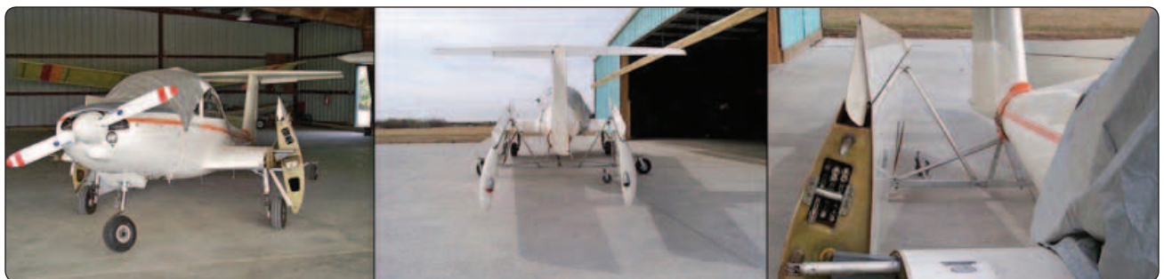
Figure 6-2. The wings of the glider can be folded in order to conveniently store the glider.
