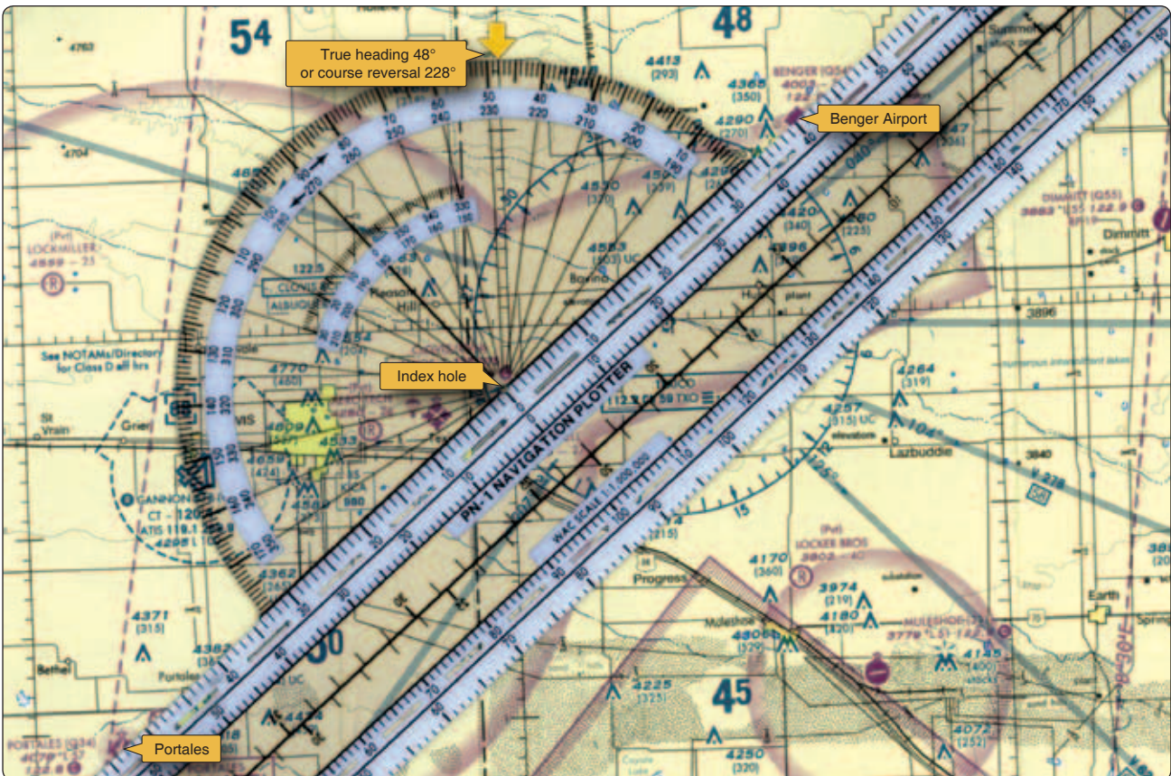
Figure 11-6. Using the outer and inner scales of the navigation plotter.
