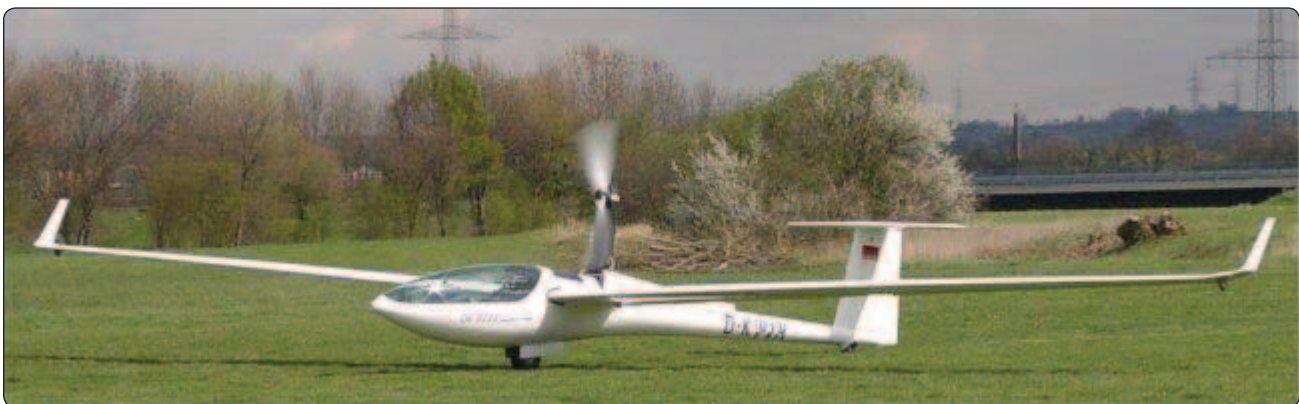
Figure 2-16. A DG-808B 18-meter high-performance glider in self-launch.
