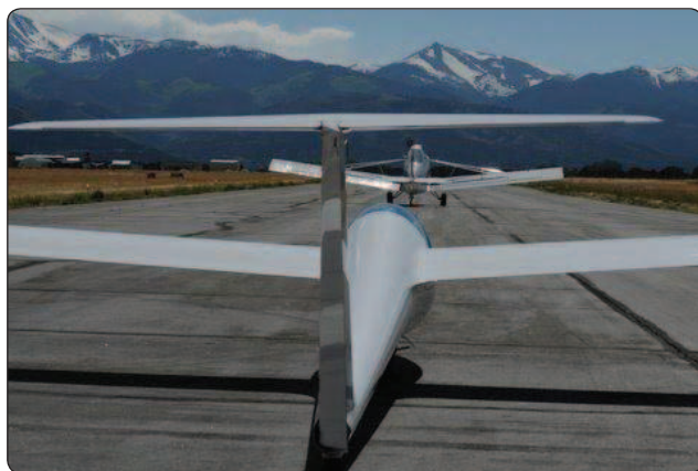
Figure 12-11. The takeoff is done by smoothly and quickly advancing the throttle in one motion so that the glider does not overrun the tow line.
