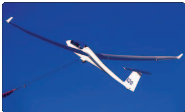
Figure 2-2. Schmepp-Hirth Ventus-2 glider with factory winglets installed.
