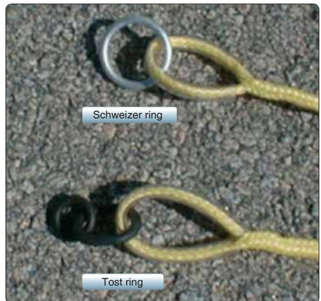
Figure 8-10. Examples of Schweizer and Tost tow rings.
