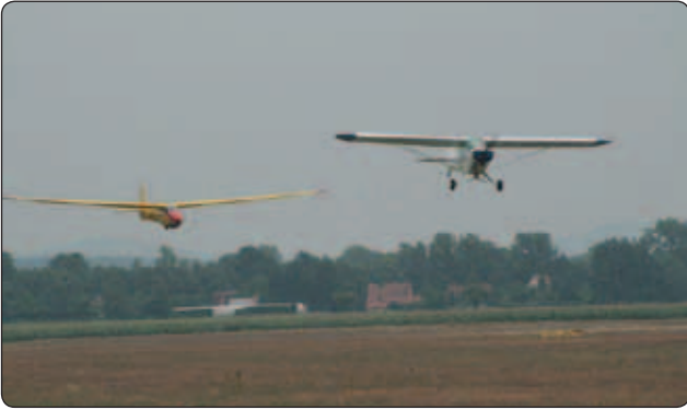
Figure 12-1. Gliders use tow planes to launch and obtain altitude.
