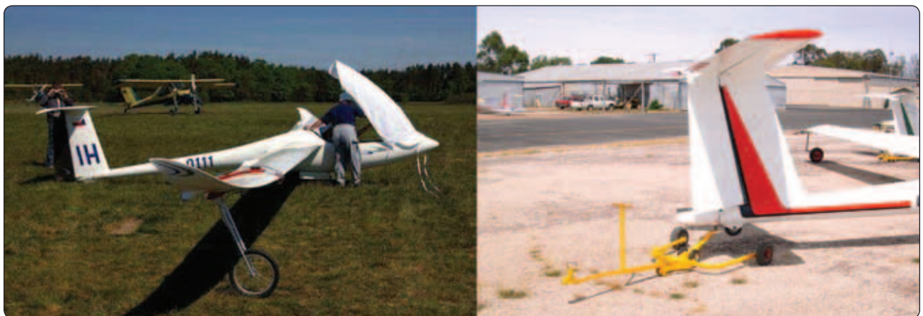
Figure 6-7. A wing dolly (left) ready for attachment and a tail dolly (right) being used for glider transport.
