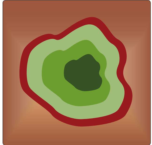
Figure 9-9. Cross-section through a thermal. Darker green is stronger lift; red is sink.
