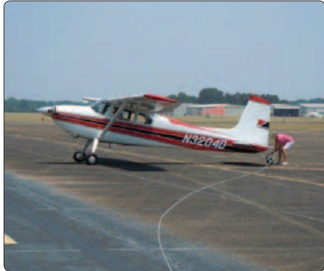
Figure 12-6. It is both the tow pilot and glider pilots responsibility to check the condition of the tow rope before flight.
