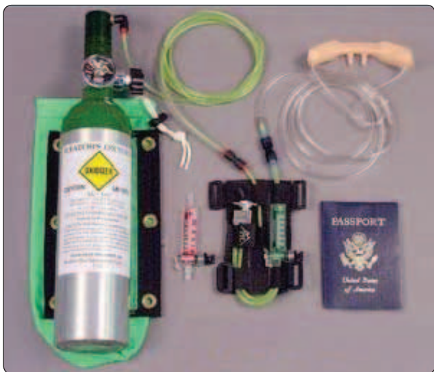
Figure 13-9. Continuous-flow oxygen system.
