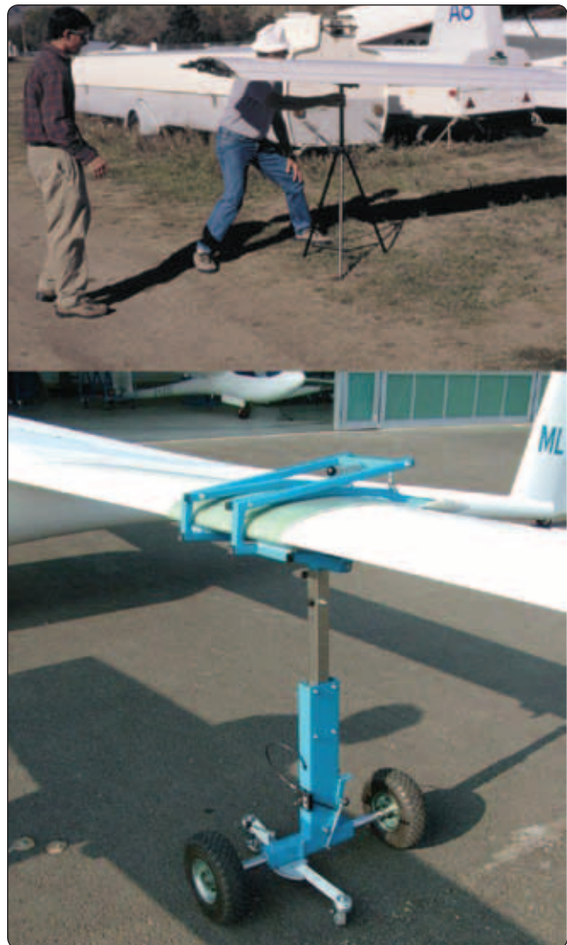
Figure 6-1. Wing stands and wing dollies are used as support when assembling the glider.
