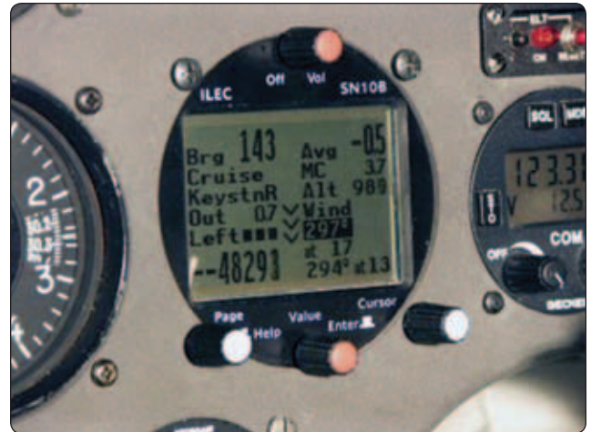
Figure 4-29. High end flight computer system.
