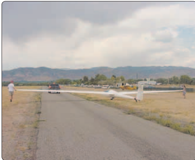
Figure 6-6. Positioning the glider for the tow vehicle.
