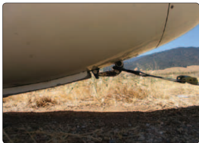
Figure 6-11. Schweizer-type tow hook.
