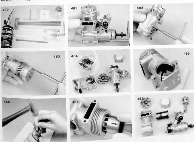
K&B's model 4011, which we are overhauling, and their model 6550 61 cubic inch engine have unique crankcase units. Most ball bearing engines have a press fit between the bearing assemblies and the crankcase while the shaft slips smoothly but easily into the bearings. K&B press fits the bearings in the crankcase, but also provides a heavy press fit between the bearings and shaft. That requires a different disassembly method than given in Chapter Fourteen and we'll show it now.
