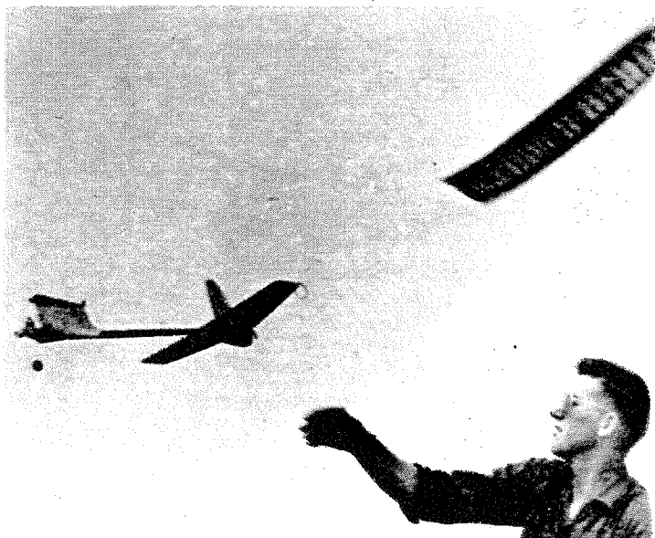
She went thataway—the wing, we mean. "Thataway" being backwards! This sad episode was staged by Robert A. Jones of Norfolk, Va. Rubber band which was holding wing at launch time is blurred streak
