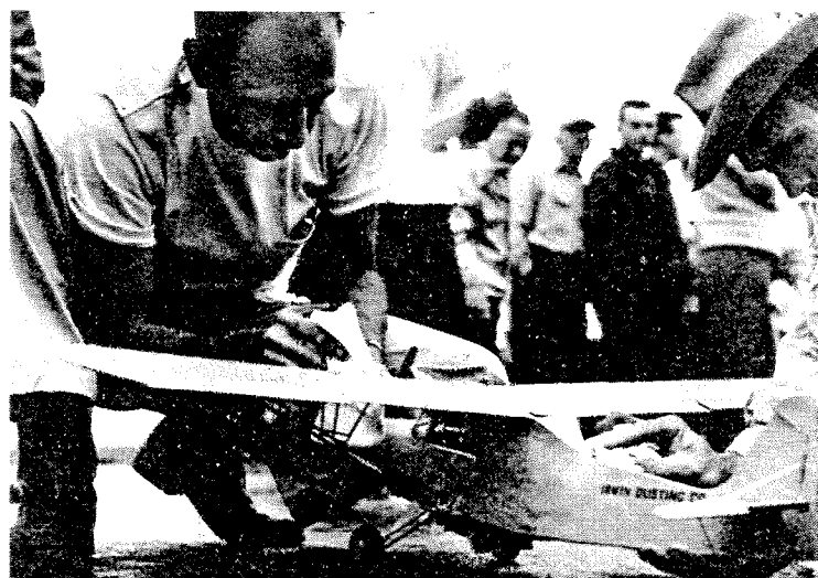
Two-time flying scale champ Thomas Dean of Corpus Christi (lt.) dries off his Aeronca "duster" model. Power was Cameron .19. Everything works on model including prop on duster bin, tiny seat belts, shock absorbers.
