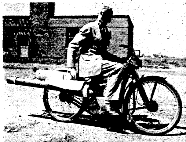
Adventurous Bill Tenney, the master-mind of Dyna-Jet, with his jet-powered motorcycle. Units are Aeromarine D5-1's—Dyna-Jets in cluster formation.
