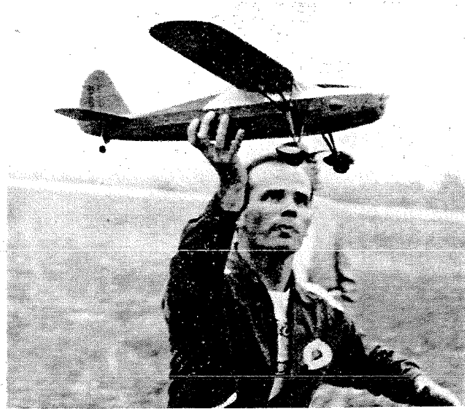
Half-A flying scale champ Edward Stoll of Detroit testing his Fairchild 24, a modified Berkeley design. Ed's 290.22 points were more than 100 ahead of next contender. Wasp .049; event was flown ROG in drizzle.
