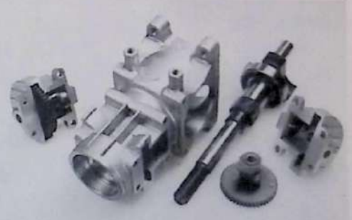
Saito engines use front camshafts, driven directly from the crankshaft main journal by spur gears. In the flat-twin Saito models, such as the FA-90T shown here, a separate camshaft is used for each cylinder.
