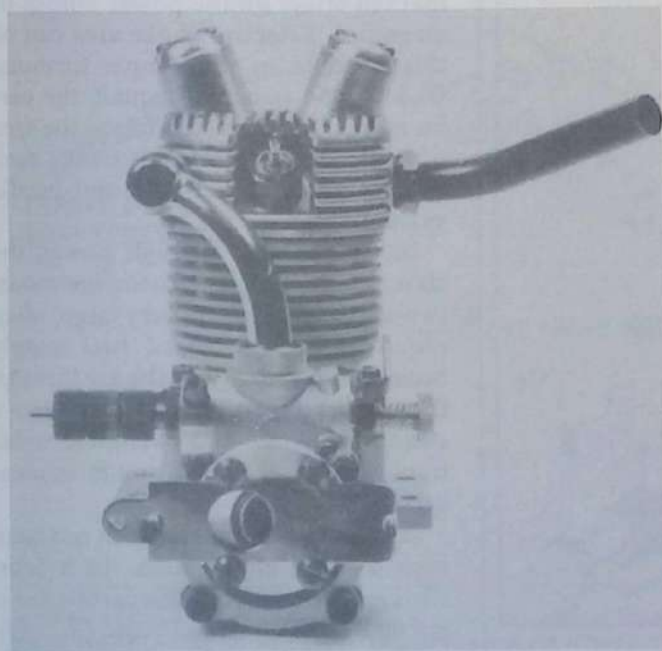
Rear view of the Saito FA-45 showing its two-needle carburetor. The slide type choke control is not self-reopening.
