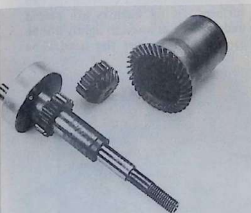
Dylla engines were uniquely different in that the complete cylinder sleeve and head rotated, driven from the crankshaft by spur gears and bevel gears.
