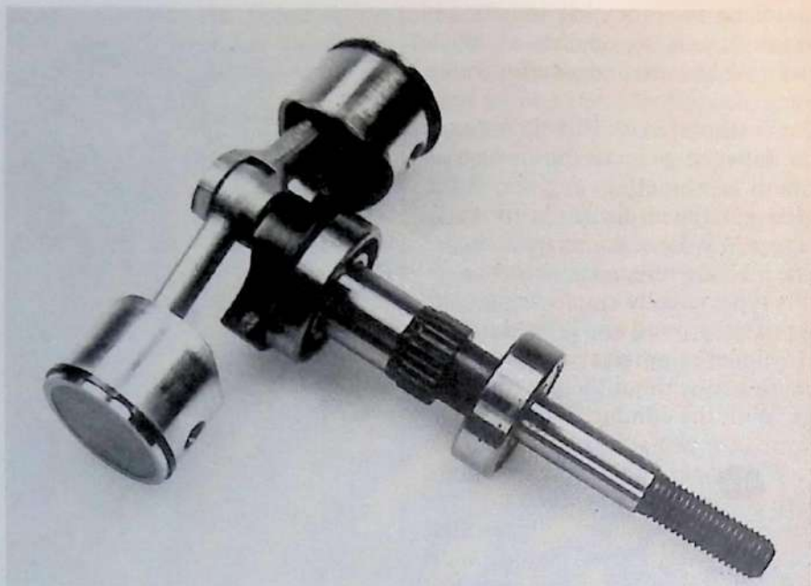
A common method of fitting two connecting-rods to a single crankpin is with a fork and blade type bearing arrangement as shown here.
