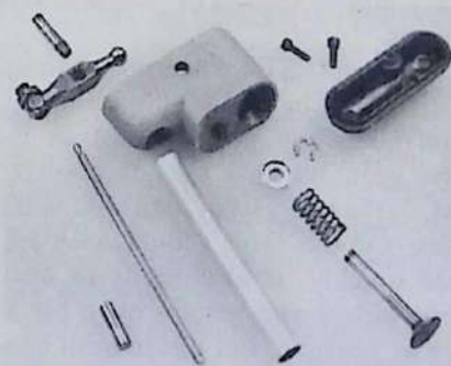
Technopower 'Big-Bore 5' radial engine valve train for just one of its ten valves. Rocker-box is of investment cast aluminum, while cover is of glass-reinforced nylon.
