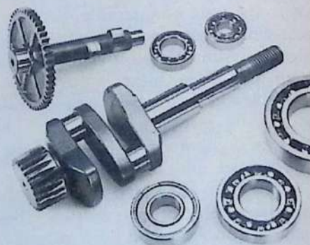
The O.S. FT-120 Gemini horizontally-opposed twin provides this good example of a two-throw crankshaft. It is carried in three ball journal bearings accurately aligned in a one-piece crankcase casting. Spur gear driven camshaft is supported in two ball bearings.
