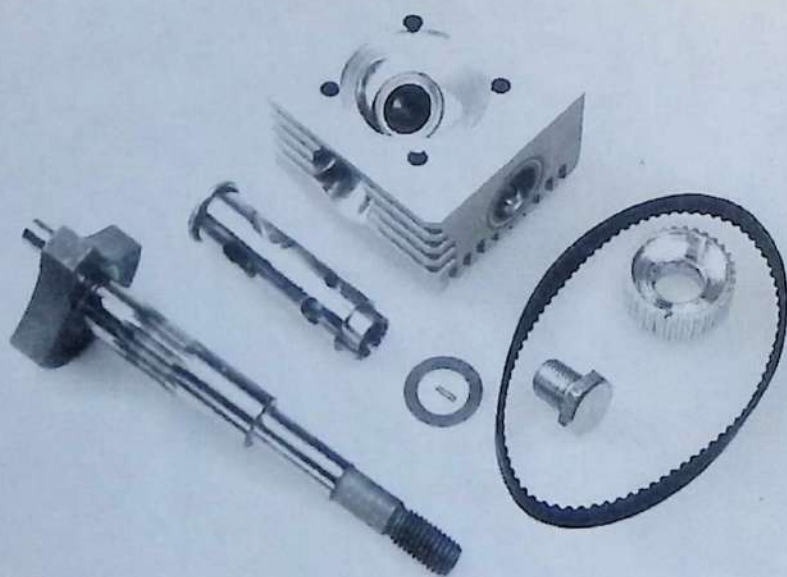
Simplest four-stroke engines of all are the Webra T4-40, T4-60 and T4-80. Horizontal axis valve is driven directly from crankshaft journal by toothed belt.
