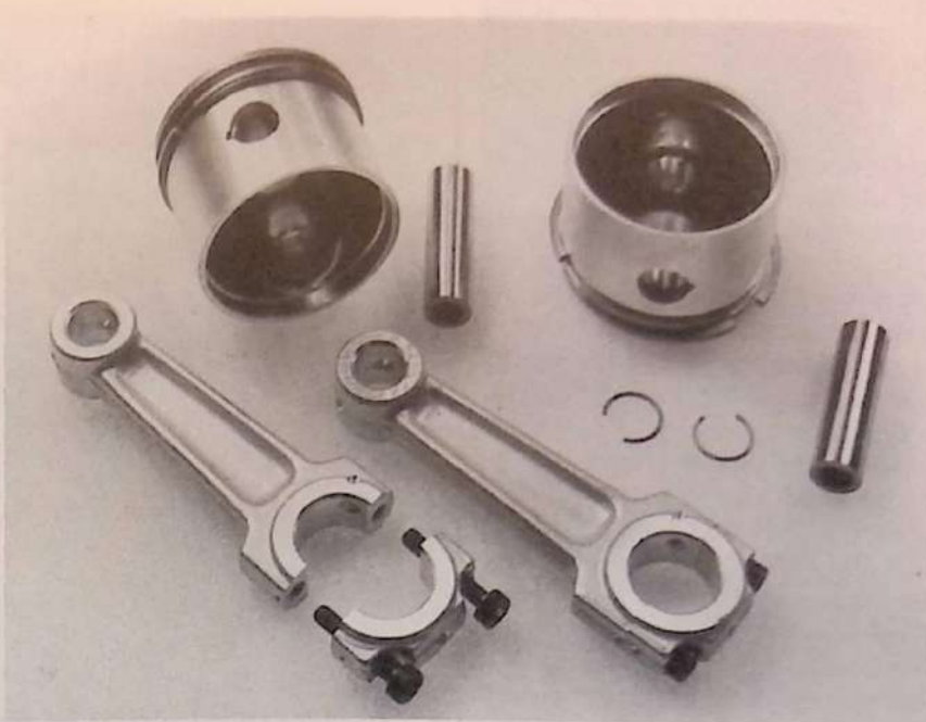
Kavan FK-50 pistons are made by German Mahle Company and follow full-size practice in having an elliptical skirt section, plus an oil scraper ring. Sturdy forged conrods have I-beam section shanks.
