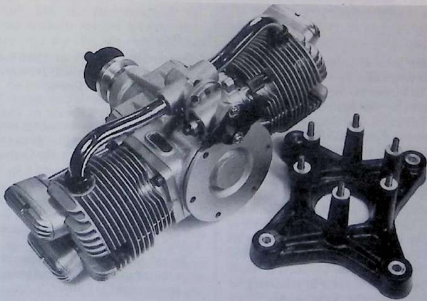
Good heavyweight cast-aluminum radial mount for the big 2.75 cu in. Saito FA-270T twin.
