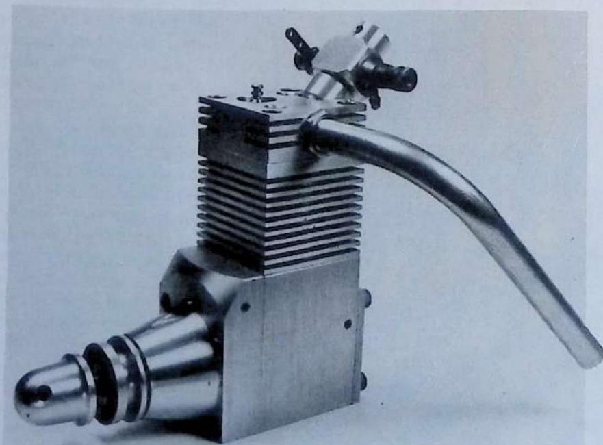
The Dylla 10cc (0.60 cu in.) rotary-valve engine. Dylla engines were made in Austria in small numbers during the late nineteen-seventies.
