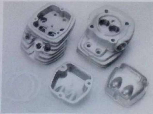
Left: Admirable examples of pressure die-casting seen in the original O.S. FT-120 Gemini cylinder heads and rocker-box components. Simple discoid combustion chamber design, but with fairly large valves and well located glowplug.
