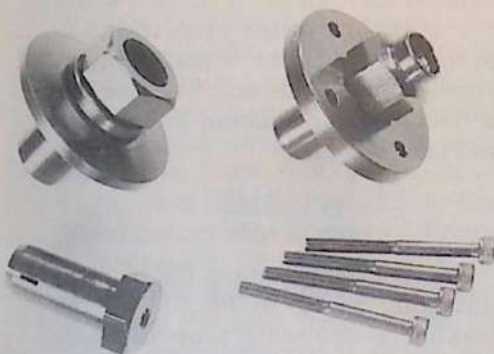
O.S. safety locknut type prop fastening (left) as supplied with O.S. Gemini, Sirius and Pegasus engines. With a through-bolt type fastening (right) it is essential to use props with adequately proportioned hubs and to keep screws and propnut tight at all times.
