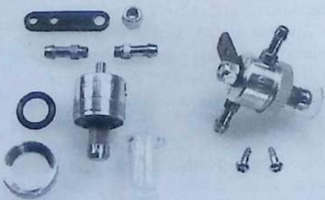
An alternative type of fuel filter from Saito. It has a detachable transparent sediment bowl.
