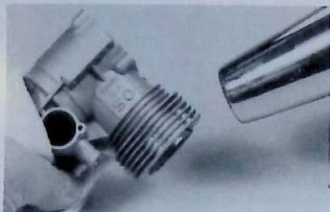
If the cylinder liner is too tight to slide out of, or into, case, apply heat to expand aluminum casting.
