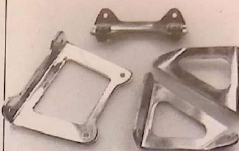
Firewall mounting brackets for Kavan FK-50 are of aluminum alloy plate and incorporate resilient three-point attachment to engine using rubber bushes.
