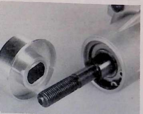
Three typical examples of prop driver attachment. Top: split taper collet (O.S. FS-60). Center: Woodruff key (O.S. FS-61). Bottom: prop driver bore shaped to fit flats on crankshaft (Enya R120-4C).
