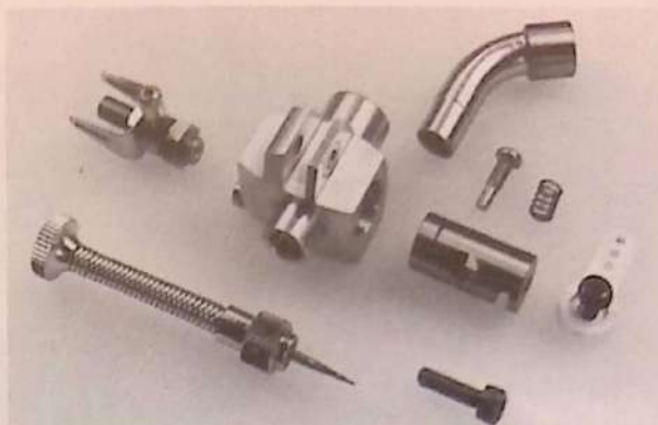
Enya "G-Series" carburetors have non-adjustable mixture control (i.e. no secondary needle) via a tapered fuel metering slot in the surface of the throttle barrel. Fine tuning of the idle mixture is then achieved with an airbleed screw.
