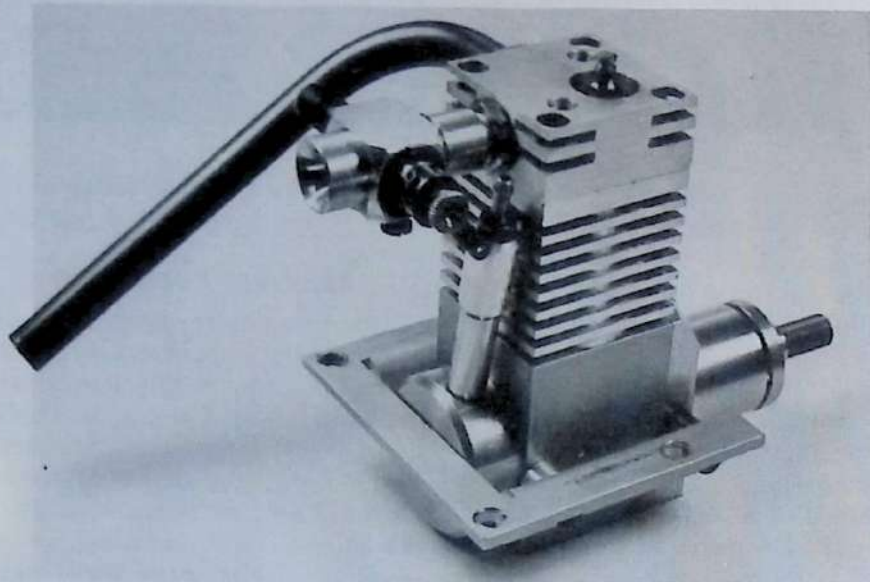
The Dylla 9cc (0.55 cu in.) rotary-valve four-stroke, one of several engines of this make which featured a rotating cylinder sleeve.
