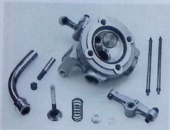
Right: Several O.S. four-stroke cylinder heads use shallow "bath-tub" shaped combustion chambers. This example, showing also valve and rocker parts, is from the FS-90.
