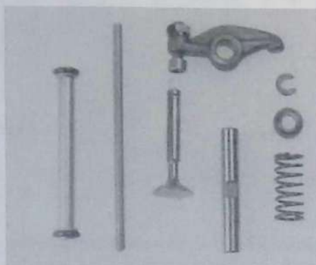
Typical pushrod-overhead-valve components (O.S. FS-40). Left to right and top to bottom: pushrod cover, pushrod, rocker-arm with clearance adjuster, valve, rocker-shaft, valve-spring with cap and retainers.
