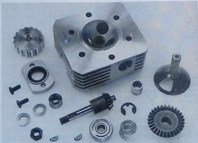
Cylinder-head and valve parts of the original Webra T4. Conical Aspin-type valve is at right. Other parts include bevel gears, bearings and toothed pulley for belt drive from crankshaft.
