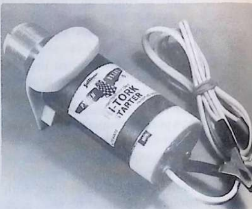
Sullivan "Hi-Tork" 12-volt electric starter will start most engines of up to 1.2 cu in. displacement. To avoid stalling starter with a big engine, prop should be rotated backwards 1½ turns from compression before applying starter.
