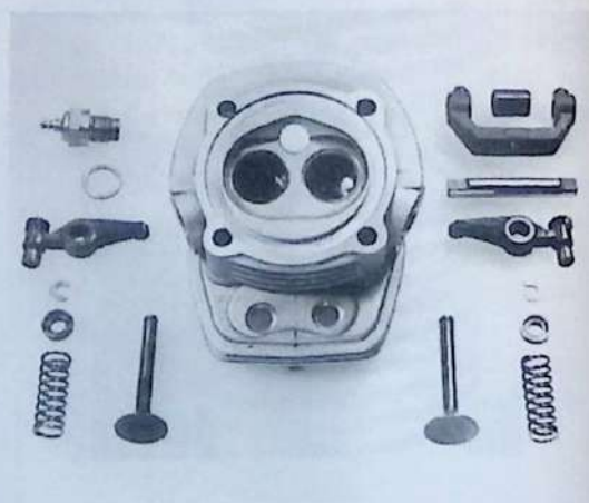
Left: Saito engines feature part-spherical combustion chambers with inclined valves, as in this head from the earliest Saito four-stroke, the FA-30 Mk.I.
