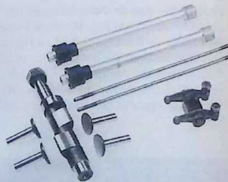
Kavan Twin camshaft with four mushroom type cam followers (i.e. for both cylinders), plus pushrod covers and rocker assembly from one cylinder. (Exhaust lobe on camshaft is for driving oil pump.)
