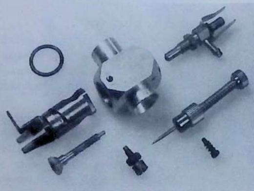
Left: Parts of the Webra TN carburetor. Note the cam slot in the throttle barrel which causes the barrel to move inwards as it rotates towards the closed position.
