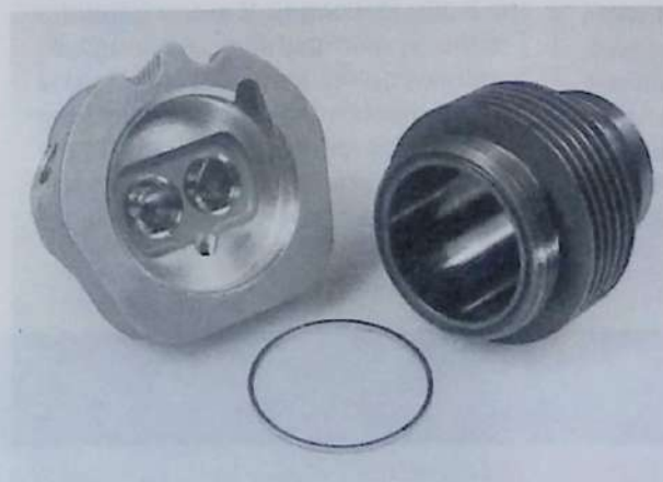
Left: Bath-tub combustion chamber is also used by the Kavan FK-50. The aluminum head screws onto the investment cast steel cylinder with a buttress thread.
