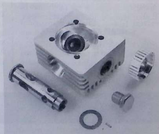
Left: Bath-tub combustion chamber is also used by the Kavan FK-50. The aluminum head screws onto the investment cast steel cylinder with a buttress thread.
