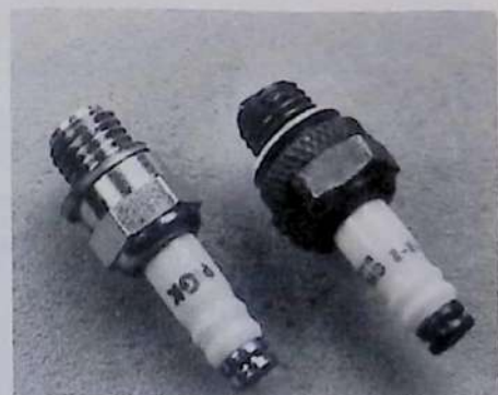
In the heyday of the spark-ignition model two-stroke, miniature spark-plugs were provided by many leading manufacturers, including Champion (example right), AC, KLG, etc. Production ceased with the rapid acceptance of the glowplug after 1948. Modern successor (left) is the Japanese NGK ME-8.
