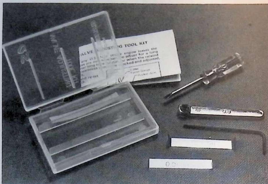
Useful valve adjusting kit from O.S. It consists of a miniature screwdriver, box-ended wrench, Allen key and two feeler gauges with angled tips for dealing with recessed rockers as in, for example, O.S. FS-40, FS-61 and FS-120.
