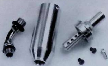
Most model four-stroke engine mufflers are simple non-baffled expansion chambers. Improved O.S. type shown has internal diffuser and gives better noise attenuation with minimal power loss.
