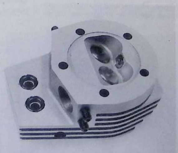
An example of good cylinder head design. Laser 75 combines efficient wedge-shaped combustion chamber with 30-degree valve inclination and straight ports for unimpeded gas flow. Plug location and generous squish area provide combination of short flame travel and good squish turbulence to minimize detonation despite relatively high compression ratio.
