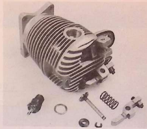
Right: Cylinder-heads are almost invariably detachable. Exceptions are to be found in some later model Saito engines such as this cylinder from the FA-90T Mk.II which has a steel liner and an integral head.
