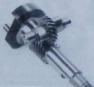
O.S. engines with front mounted valve gear employ a transverse camshaft driven directly from the crankshaft through crossed-helical "skew" gearing. Example shown here is from small FS-20 model.
