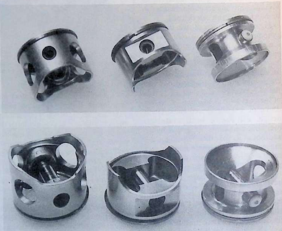
Three types of modern four-stroke piston. Left to right they are: (a) O.S. FS-90 semi-slipper type with lightening holes; (b) Enya 80-4C slipper type and (c) Laser 75 hourglass pattern.
