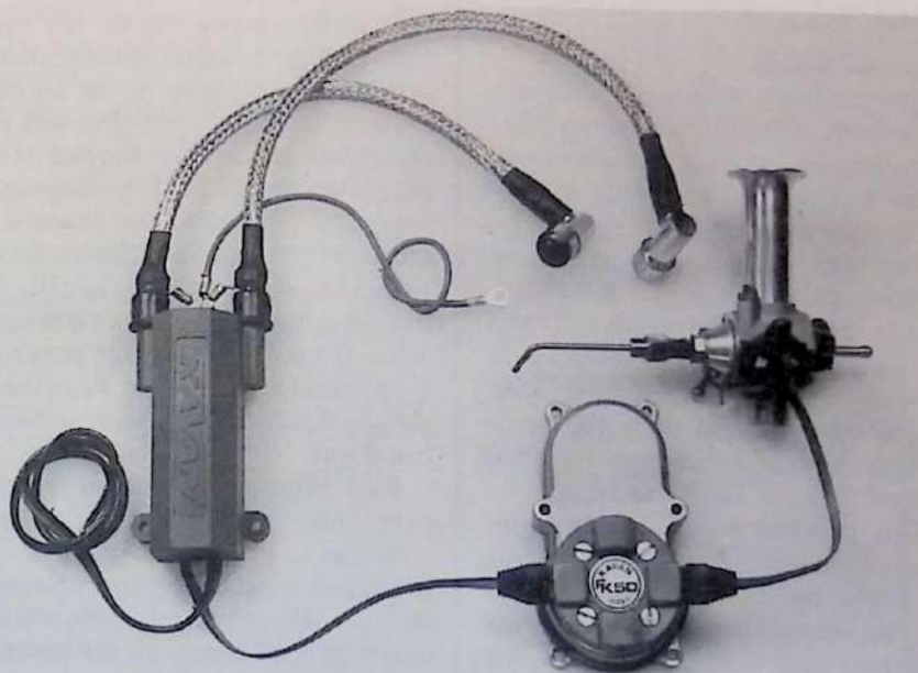
The Kavan Twin electronic spark ignition system. It has two Hall Effect pickups, one advanced and one retarded, with selection via a microswitch actuated by the throttle.
