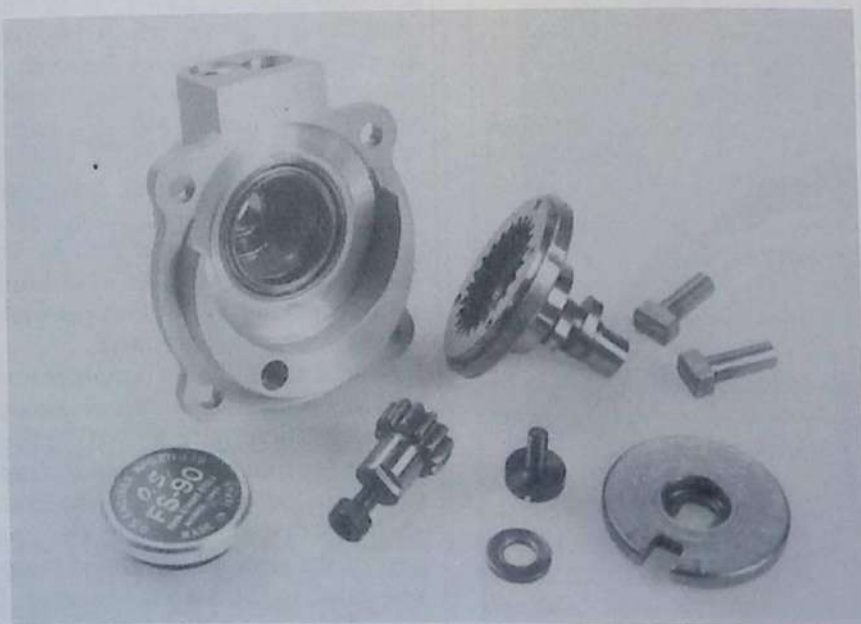
In the O.S. FS-90, the camshaft drive is the same as in the original FS-60 but cam profiles are considerably modified and operate special hammer-head shaped cam followers.
