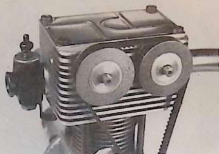
Twin overhead camshafts used by Schillings-PL engines are driven directly from a rear crankshaft take-off pulley by a toothed belt. Such a simple arrangement eliminates the need for separate timing gears.
