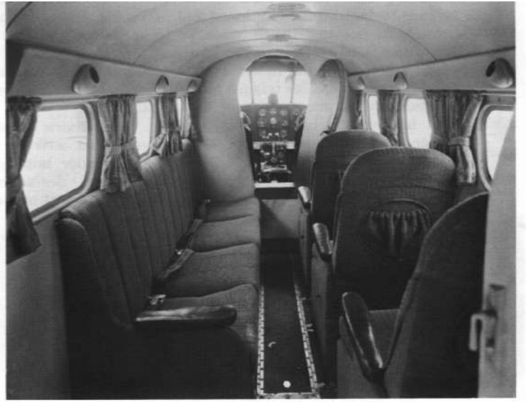
Cockpit and cabin interior of the original Beech 18. All succeeding civil versions varied little in general arrangement.
