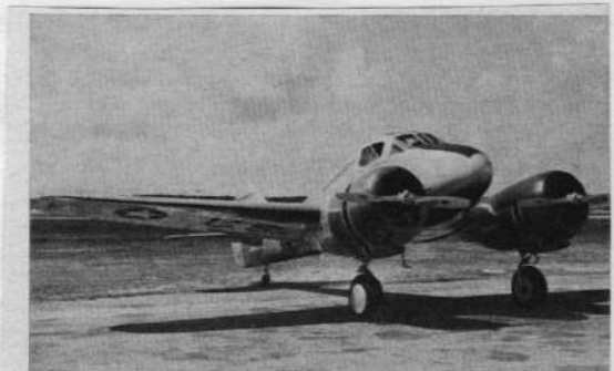
AT-9 Curtiss, twin-engine. In advanced training, cadets begin simulated combat work, cross-country night flying, fixed-gun shooting, tight-formation flying, landing on small fields
