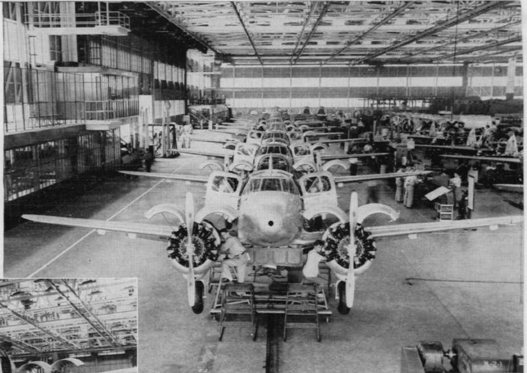
Twin-engine AT-9 Transition Trainers are assembled on a continuously moving, block long line. The wheel dollies on which the airplanes are mounted are pulled along by a powered chain, motor for which is seen in foreground.
