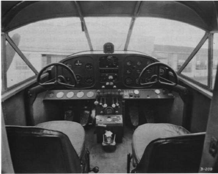
Cockpit and cabin interior of the original Beech 18. All succeeding civil versions varied little in general arrangement.
