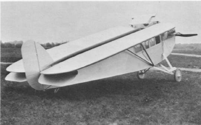
Below, with wings folded and detail of tail surfaces.
