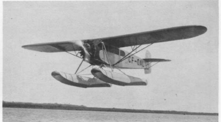
Canadian CF-OAL Model 71, had spill-plate fairings on outer wing struts.
