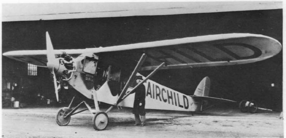
Above, OX-5 powered FC-1 with a golf sportsman about to "fly" to his favorite course. Aileron-flap pulleys on wing are prominent. Right, modified with a Wright J-4 engine, it became the FC-1A. Fred Weymouth by rear door. Ailerons and flaps are now operated separately.
