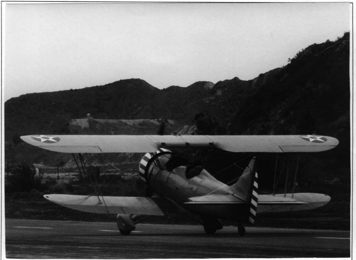
UPF-7 with different paint scheme with cowling and wheel pants.
