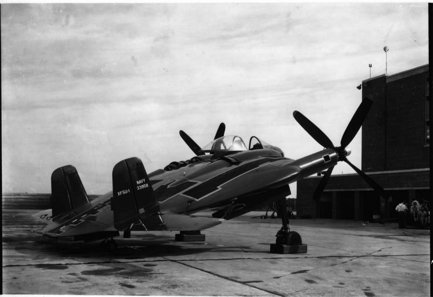
CV-21649 XF5U-1 BU. #33958 - 1ST FLIGHT MODEL 3/4 REAR VIEW WITH AIRPLANE IN STATIC 3 POINT POSITION - PRIOR TO INITIAL ENGINE GROUND RUN - (STD. HYDROMATIC (F4U-4) PROPS) 8/20/45
