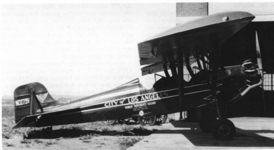
City of Los Angeles established a unique endurance record in November 1930. Owned by J. Warren MacClatchie and powered by an engine of his own development, it flew some 27,667 miles without an engine shut down or maintenance of any kind. It was the sole Timm M-150 Collegiate, c/n 105. Power was the MacClatchie X-2 Panther engine of 150 hp. Colors were overall red with black trim and white pin striping.
