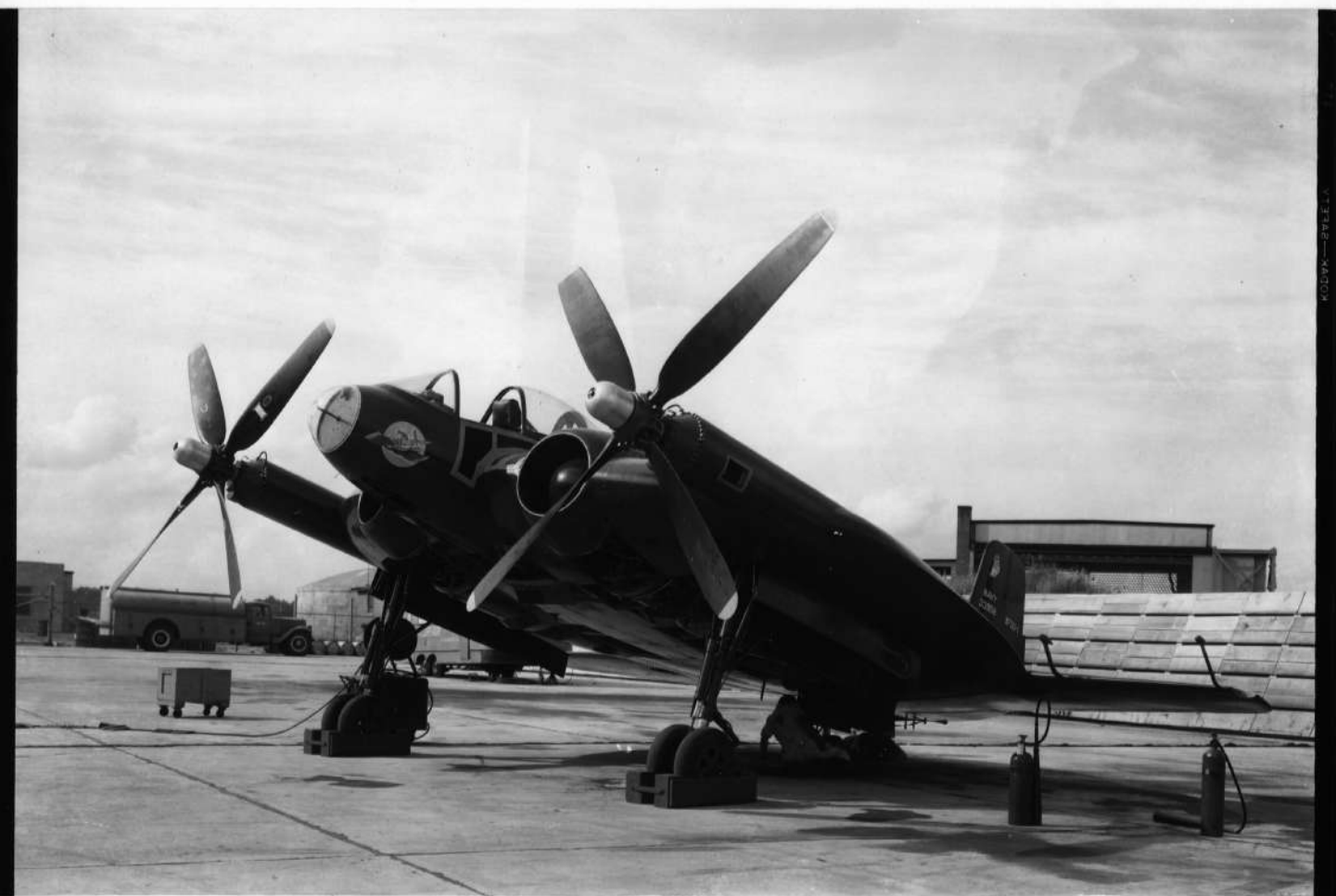
CV-21650 XF5U-1 BU. #33958 - 1ST FLIGHT MODEL 3/4 FRONT VIEW WITH AIRPLANE IN STATIC 3 POINT POSITION - PRIOR TO INITIAL ENGINE GROUND RUN - (STD. HYDROMATIC (F4U-4) PROPS) 8/20/45
