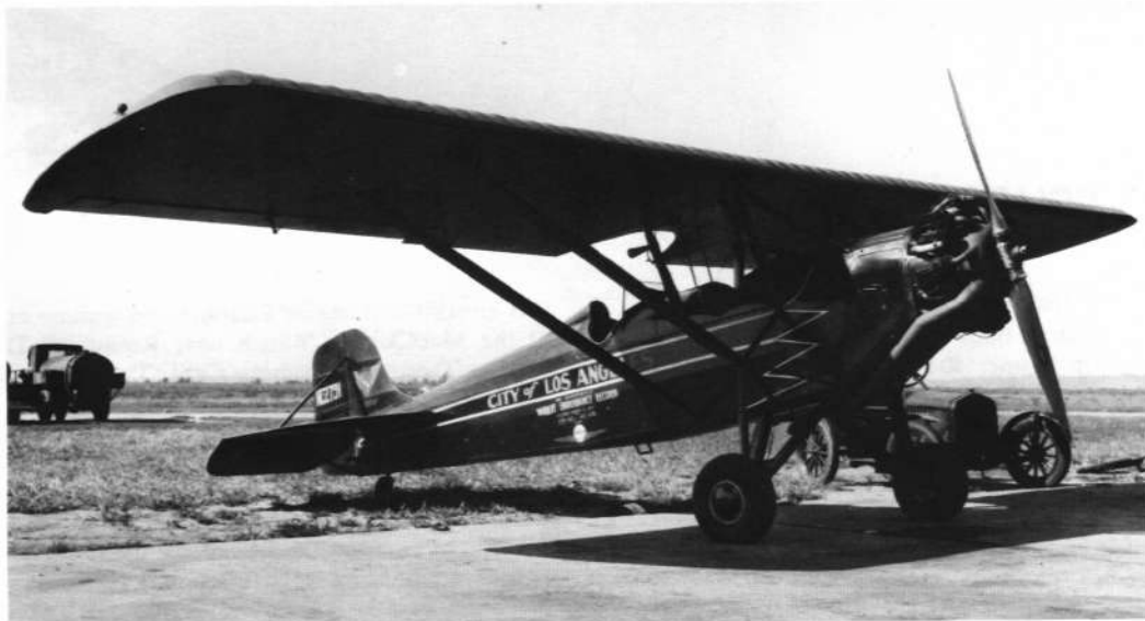
City of Los Angeles established a unique endurance record in November 1930. Owned by J. Warren MacClatchie and powered by an engine of his own development, it flew some 27,667 miles without an engine shut down or maintenance of any kind. It was the sole Timm M-150 Collegiate, c/n 105. Power was the MacClatchie X-2 Panther engine of 150 hp. Colors were overall red with black trim and white pin striping.
