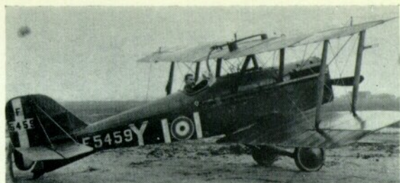
It had served with No. 60 Squadron, R.F.C. Like B4890 it had the steel-tube undercarriage, but its engine drove a two-blade airscrew. An S.E.5a (above) of No. 24 Squadron with reduced dihedral. The headrest has been removed and the windscreen modified. Although the engine is a Viper, the aircraft retains the higher Foster mounting that was standard on S.E.5a's with geared engines.
