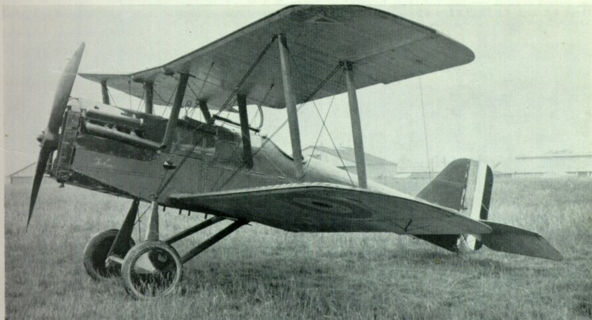
The small number 98 stencilled on the side of the forward fuselage indicates that this S.E.5a is C1148. This aircraft passed its final inspection on September 28th 1918, when it had engine No. 2297/W.D.33397. In February 1919 it was fitted with a Royal Aircraft Establishment variable-pitch airscrew. This photograph is dated June 11th 1920, and shows the aircraft with standard Viper installation and fixed-pitch airscrew; it has short exhaust pipes and the wooden undercarriage.
