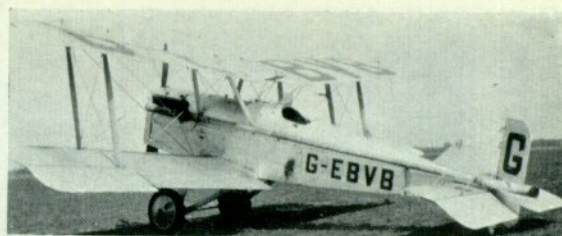
G-EBVB was one of the skywriting S.E.5a's. Their extended exhaust pipes met in a single outlet, to clear which a cut-out was made in the rudder.
