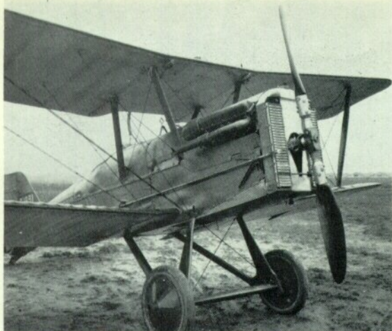
C1091, photographed on April 26th 1920, with an experimental variable-pitch airscrew. (Photo: Crown copyright)
