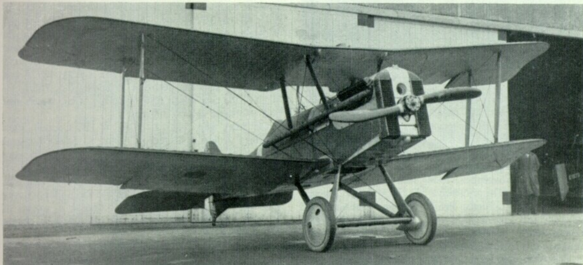
Apparently an early installation of a Wolseley Viper engine. The top of the radiator is not of the shape that became standard, and the under-fairing is shallower than on production Viper-powered aircraft.
