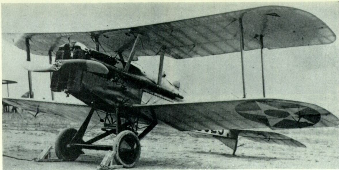
An S.E.5a in American service and markings, seen at Quantico in June 1921. The under-fairing of the nose has been removed and the structure under the fuselage may have been a bomb rack. (U.S. Navy photo)
