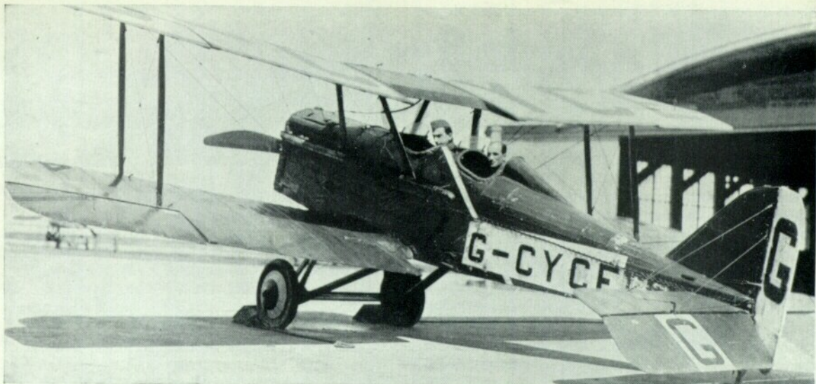
The Canadians also made a two-seat conversion of the S.E.5a. G-CYCF was originally F9117. It appears that a modified centre section, possibly containing a gravity tank between the spars, was fitted. (Photo: K. M. Molson)
