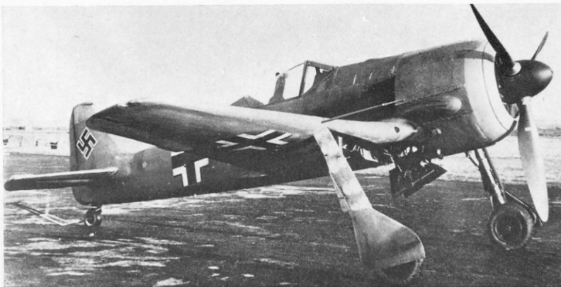
The third prototype Focke-Wulf Fw 190. Designated Fw 190V5k, this aircraft had the short span wing. (Photo: Imperial War Museum)
