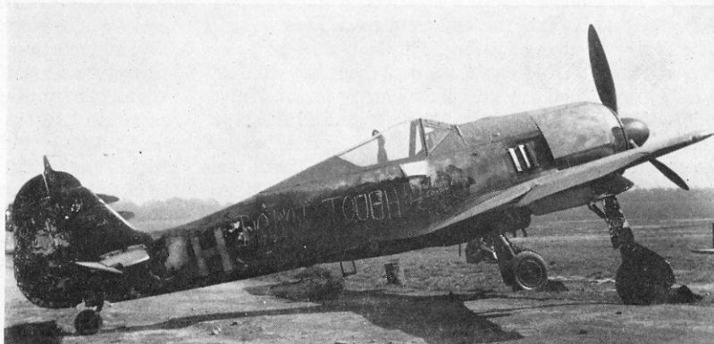
An Fw 190A-4/U8 of SKG 10 which landed at R.A.F. West Malling on the night of July 16th 1943. A matt-black temporary finish was applied to the aircraft for night intruder sorties.
