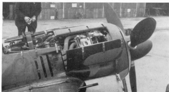
Power-egg of Fw 190A-3 showing MG 17 Mgs. ('Flight' photo)
