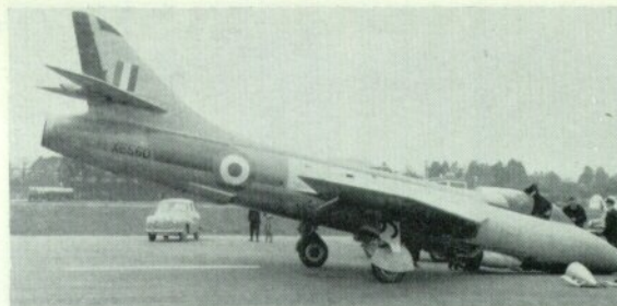
A nosewheel-up landing by a C.A. Trial Hunter 6 caused by fatigue failure of the operating mechanism during intensive gun firing trials.
