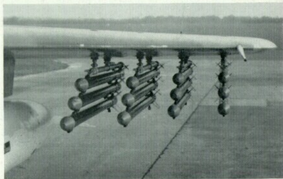
Below: The Hunter 6 with alternative weapons and stores, including practice bombs, H.E. bombs, 230-gal. and 100-gal. drop tanks and napalm bombs, 5-inch, 3-inch and 2-inch (folding fin) rockets. Top left: The pilot's view of the port pair of 100-gal. drop tanks. Right: Close-up view of 3-inch rocket triple-tier mountings. When fitted with 60-lb. warheads, only a single bank of rockets could be carried.
