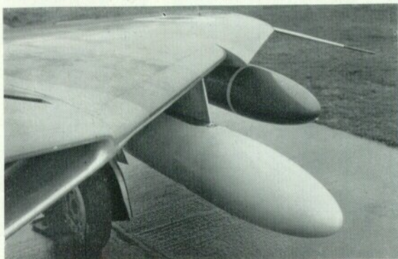
Below: The Hunter 6 with alternative weapons and stores, including practice bombs, H.E. bombs, 230-gal. and 100-gal. drop tanks and napalm bombs, 5-inch, 3-inch and 2-inch (folding fin) rockets. Top left: The pilot's view of the port pair of 100-gal. drop tanks. Right: Close-up view of 3-inch rocket triple-tier mountings. When fitted with 60-lb. warheads, only a single bank of rockets could be carried.
