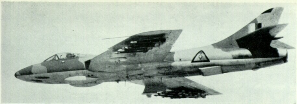
An Iraqi Hunter 6 equipped with practice bomb carriers and 3-inch rockets.
