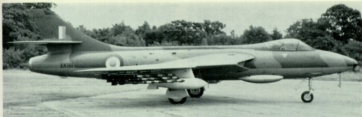
XK161 fitted with 1,000-lb. bombs on the inboard pylons and 24 rockets outboard.
