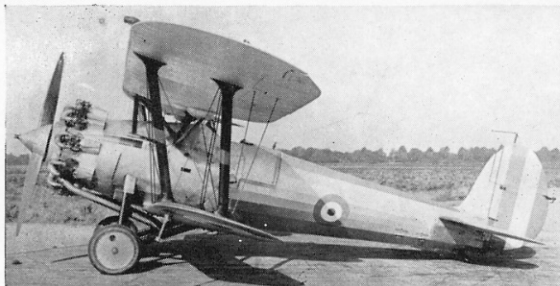
Left: Prototype Bulldog II, c/n 7235, serial J9480. First flew on 21st January 1928. Right: 11th production Bulldog II, c/n 7332, serial J9576, in No. 3 Squadron colours. No. 3 was the first squadron to operate Bulldogs. Note amended fin shape.
