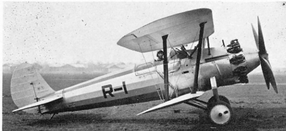
Left: Bulldog II, c/n 7399, SBAC number R.1. Test bed for Mercury III engine fitted with four-blade propeller. Right: R.1 with Geome-Rhône Jupiter VI engine. Registered G-ABAC on 30th May 1930 and destroyed on 4th June.
