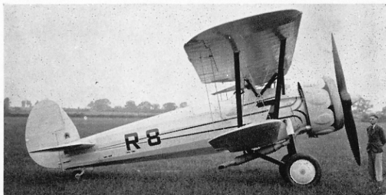
The second Bulldog IVA, R-8, c/n 7808. Registered G-ACJN and built to test Mercury VIS.2 engine. Later fitted with this engine, but first used for testing Perseus IA. Seen here painted ready for the 1934 SBAC Show.
