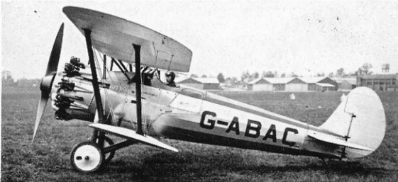
Left: Bulldog II, c/n 7399, SBAC number R.1. Test bed for Mercury III engine fitted with four-blade propeller. Right: R.1 with Geome-Rhône Jupiter VI engine. Registered G-ABAC on 30th May 1930 and destroyed on 4th June.
