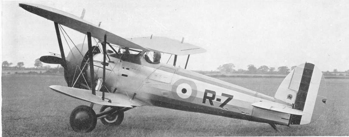
The second Bulldog IIIA, R-7, c/n 7745, private venture aircraft. Registered G-ABZW on 3rd October 1932 but never carried marks. Narrow-chord ailerons on upper and lower wings as standardised on Marks IV and IVA.
