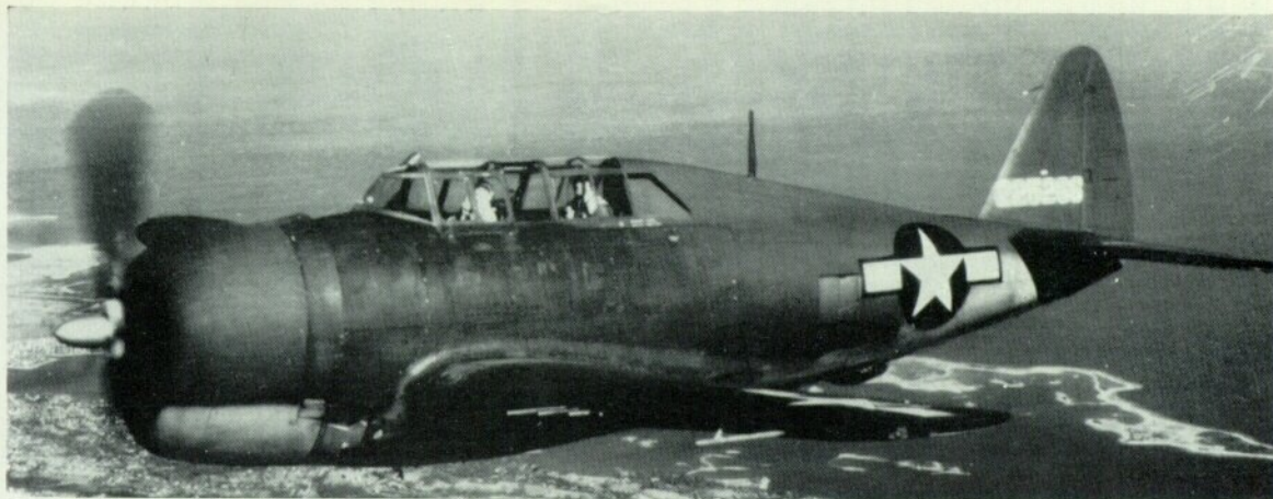
Curtiss-built two-seat TP-47G trainer. Began life as a P-47G-15-CU of the 5th and final batch built at Buffalo. Converted to trainer configuration during 1942. (Photo: Richard Ward)
