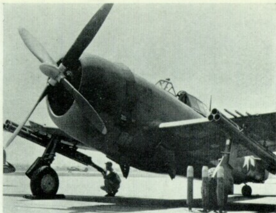
Early P-47D-20RA showing three-tier 'bazooka-type' rocket tubes and folding fin rockets. (Republic Aviation photo)
