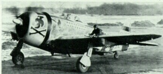
P-47D-30-RE of the 18th and final batch built by Republic at Farmingdale. Operated with 353rd Fighter Squadron, 354th Fighter Group, 9th Air Force. (Photo: Imperial War Museum)
