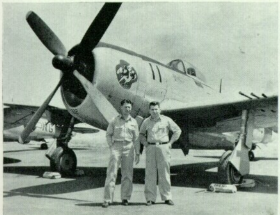
P-47D-40-RA of the Maryland Air National Guard. Pilot, Major 'Bob' Tyler, flew the aircraft with one prop blade white to get the stroboscope effect. To spectators it appeared that the blade remained static. (Photo: Major Robert Tyler, U.S.A.F.)
